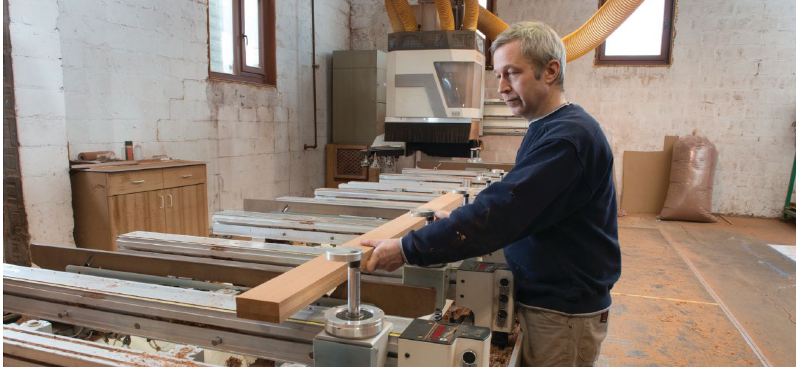
John Proulx loads the SCM Routech CNC router at Architectural Openings in Somerville, Mass.
