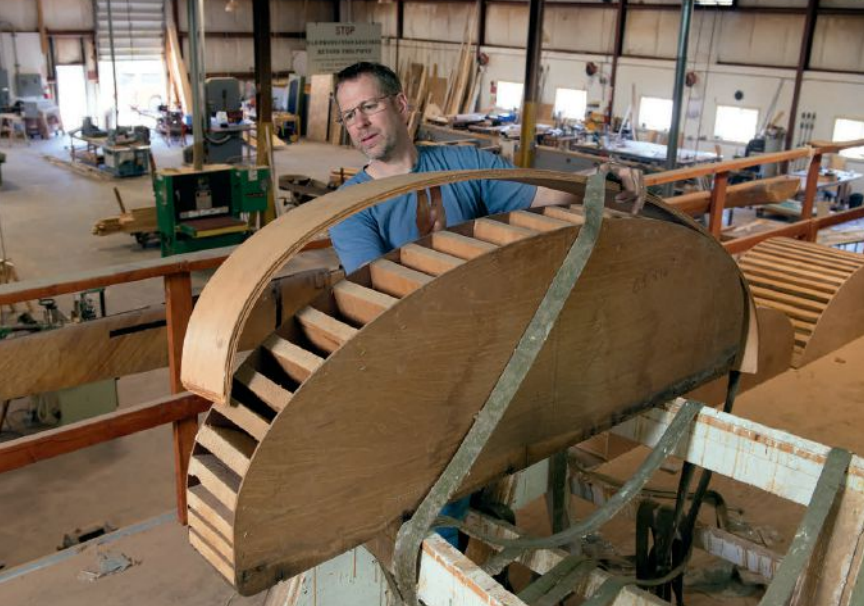
The shop has dozens of jigs to form curved products.
