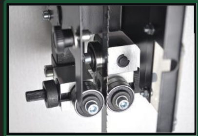
Tool-less Micro-Adjustable Blade Guide Bearings.
