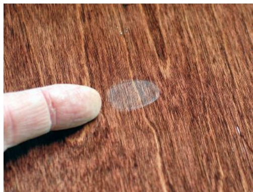
When finishes dry slower than expected, press marks, like the one shown here with a fingerprint, are often the result.
