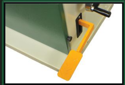
Foot Brake with Built-in Power Off Switch.
