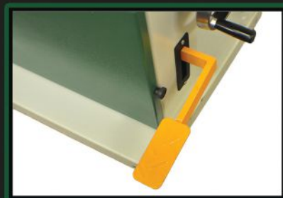
Foot Brake with Built-in Power Off Switch.
