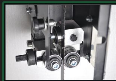
Tool-less Micro-Adjustable Blade Guide Bearings.
