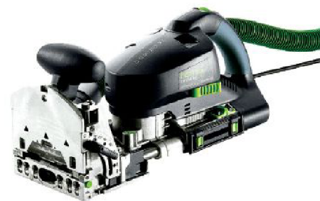
The Domino from Festool cuts two mortises and a separate, floating tenon is used to complete the joint. The machine comes in two sizes for regular (above) and large work.
