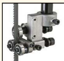
UPPER AND LOWER BALL BEARING BLADE GUIDES
