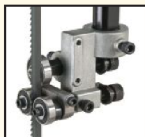
UPPER AND LOWER BALL BEARING BLADE GUIDES
