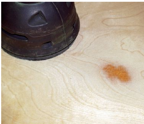
When replacing panels and top, some plywood imports have paper-thin hardwood veneer that is very easy to sand through.
