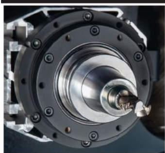
Main spindle 13.5 HP (10kW) main spindle - HSK F63 (24.000 rpm), ceramic bearings, pressurized system
