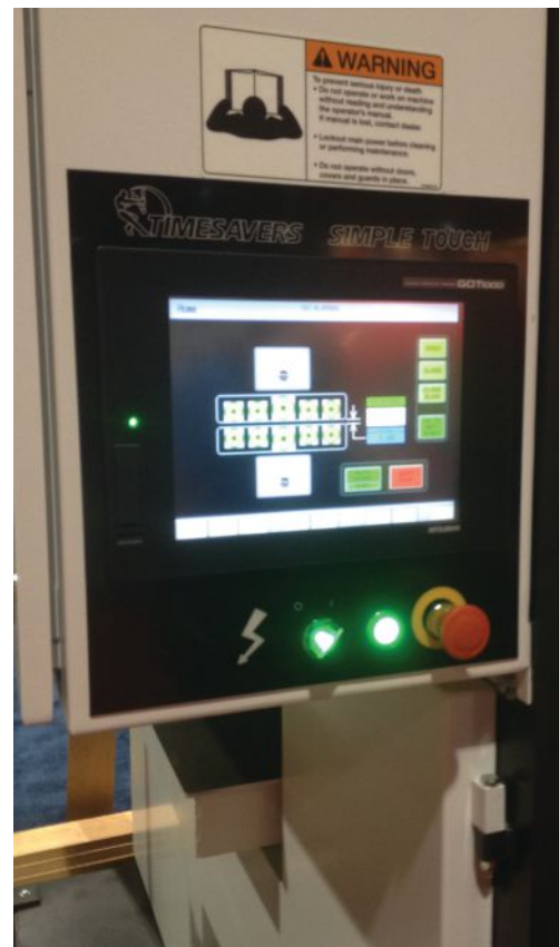
The controls of Timesavers' Yieldsaver-24, a rough lumber planer.
