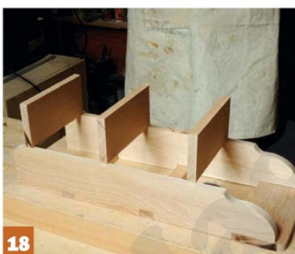
18 I laid the components out for a last check before cutting the housings
