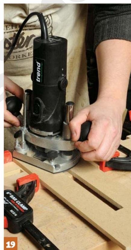
19 I used a router and guidebush in a slot cutting jig to cut the housing joints
