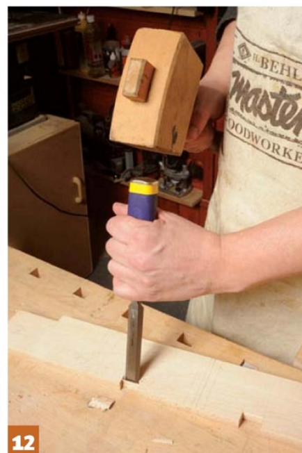
12 Remove the housing waste with a sharp chisel and mallet
