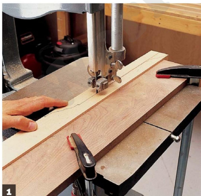
1 Rip the stepped board on the bandsaw. A simple fence helps you make a straight cut. Stop the cut at the top of the ogee curve, withdraw the board, remove the fence and cut out the ogee
