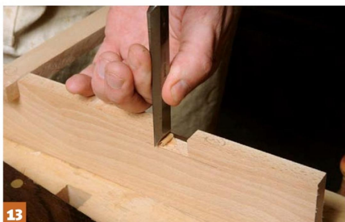
13 Pare the sides vertically to clean up the sawn sides
