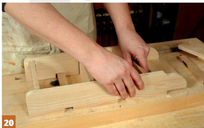
20 I dry fitted the joints to make sure everything went together
