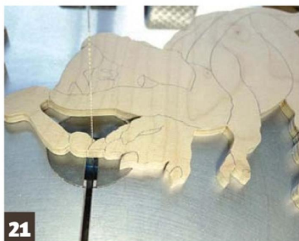
21 Using the No. 3 blade, cut around the backing and drill an entry hole
