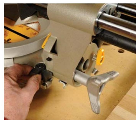
The tri-knob changes the bevel angle and the flip-out stops then limits the bevel
