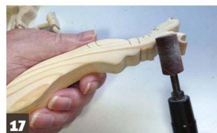
17 Use a drum sander to refine the shapes and remove scratches left from the sander
