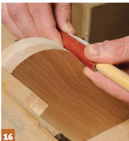
16 I ganged the two sides together in a vice and finished the curves with abrasive
