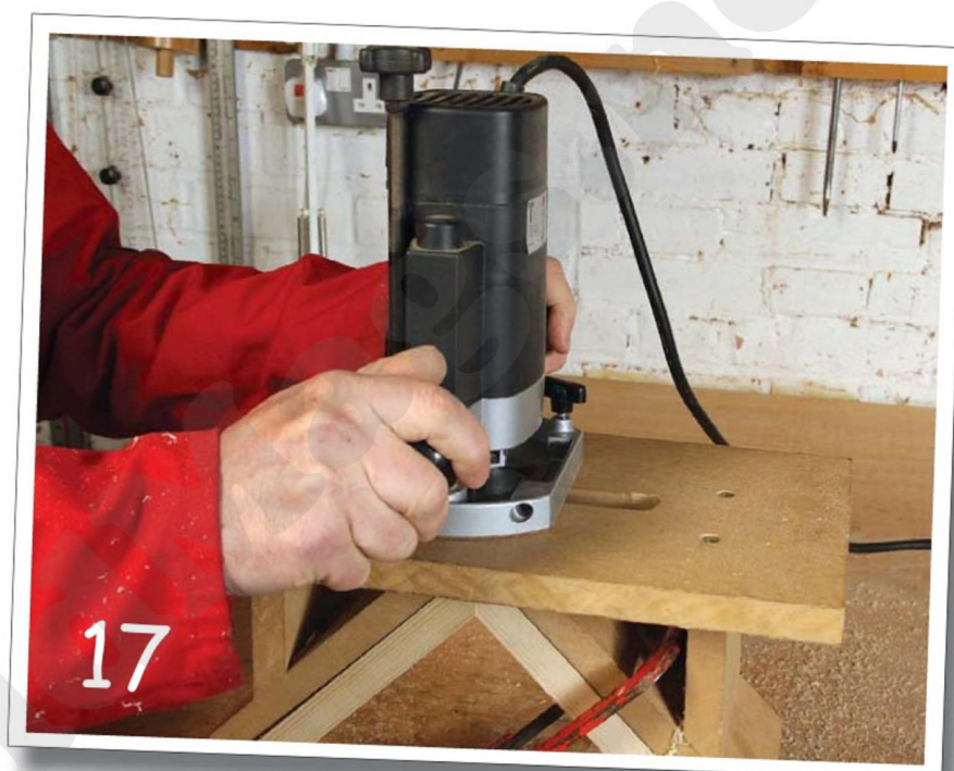
Place your router on the jig and make sure that the cutter is securely locked down. It must not be raised as it might damage the cutter and/or the guidebush. Start the router and gently push it forward to cut the joint. Switch off and do not lift the router out until the cutter has stopped revolving
