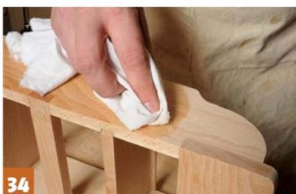
I applied a coat of sanding sealer before de-nibbing with 120 grit
