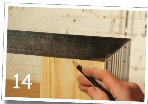
The dovetails will only be inserted on the mitred corners, so mark their positions with a pencil
