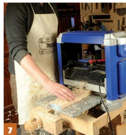
7 Flat off one side and use this as the reference surface on the thicknesser
