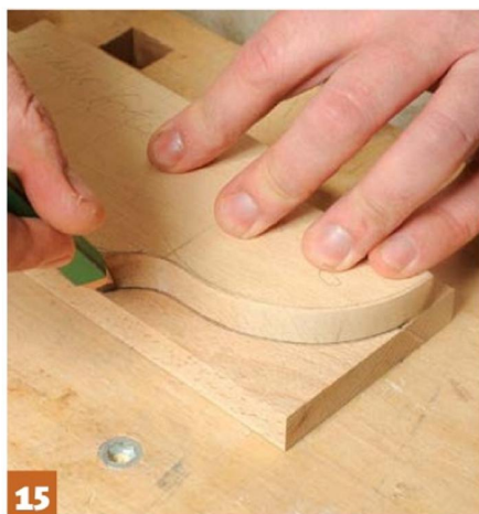
15 I cut the curve out on the bandsaw, using it as a template for the opposite face
