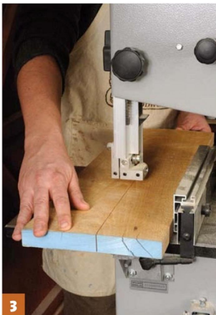
3 I ripped the boards to width on the bandsaw with a fence
