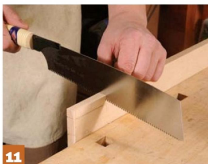
11 For cuts that don't fit on the bandsaw, the Japanese saw is very useful
