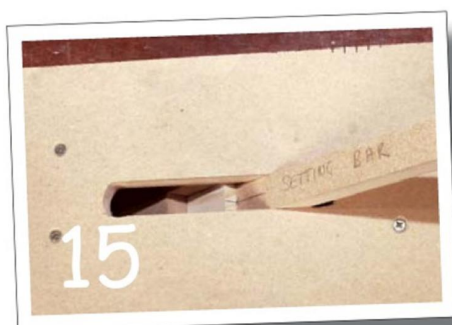
Clamp the box in a bench vice and, using the setting bar, align the jig with one of the marks
