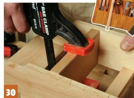
30 Then I positioned the front edges and clamped them in place
