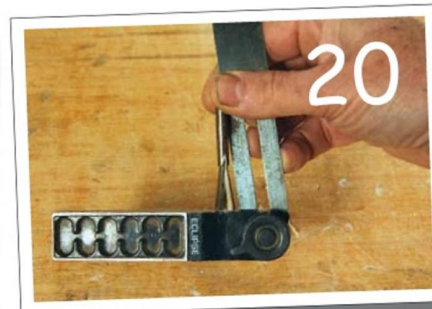
Remove the dovetail cutter from your router and use it to set the angle of your sliding bevel. Use this to set the tilt on the blade of the table saw
