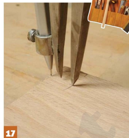
17 I marked the rounded corners on the front bottom corner with a compass
