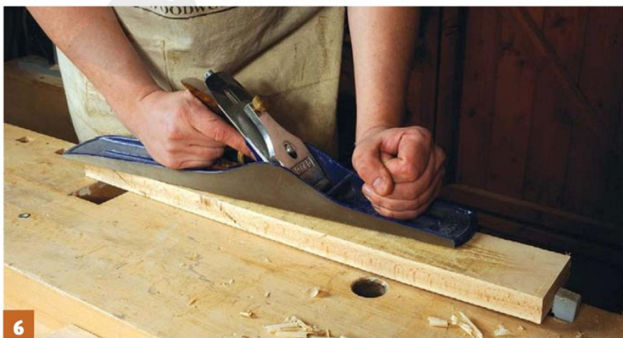
6 The bow was too pronounced to use the thicknesser so it was time get the jointer out
