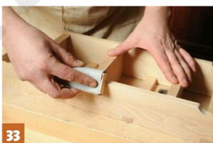
I used 120 grit and a wooden block to cut the smallest hint of a bevel
