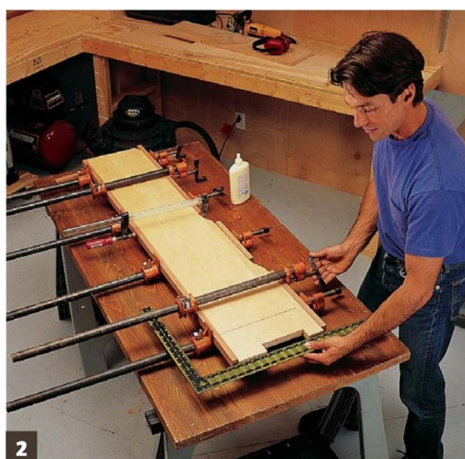
2 Glue the upper case sides from 1 in thick rough boards that are planed to \frac{7}{8} in thick. This leaves some untouched low spots, but that's OK. Align the outside boards so their bottoms are even
