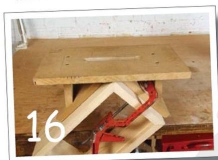
Clamp the box in a bench vice and, using the setting bar, align the jig with one of the marks
