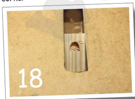
To prevent breakout as the cutter exits, make a cut at the rear of the slot by standing the router at the end of the jig, start the motor and gently pull it back to the box corner. Push it back and forward, switch off and remove the router and cut
