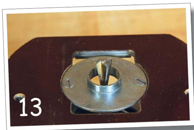
The router fitted with dovetail cutter and guidebush
