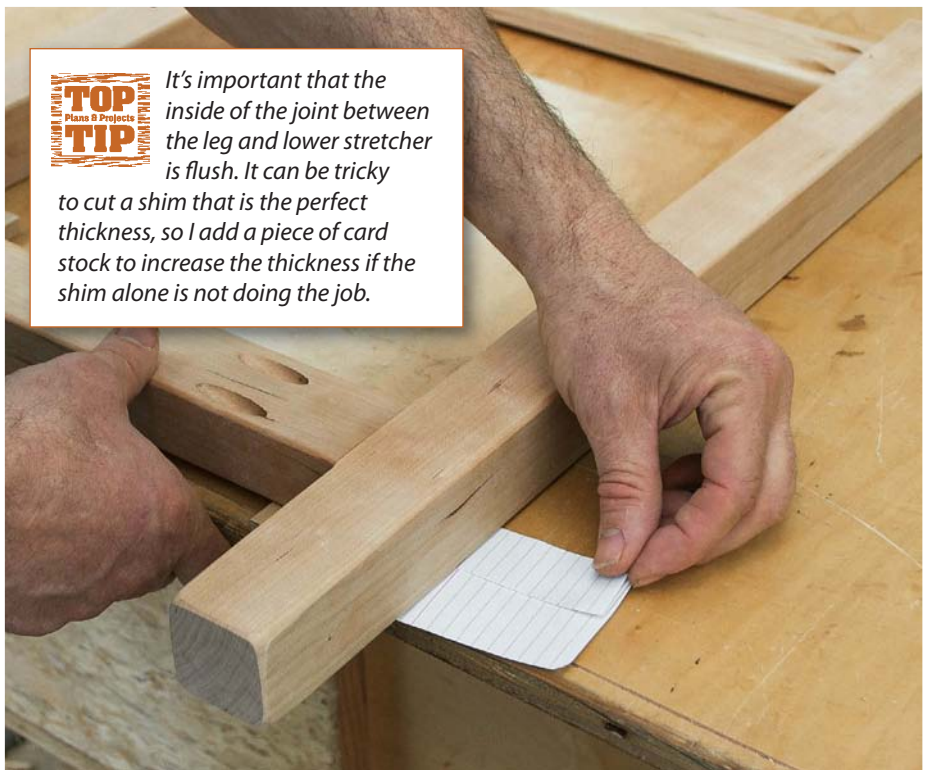
With bar and face clamps holding the assembly, slowly drive the long screw through the lower stretcher and into the leg
