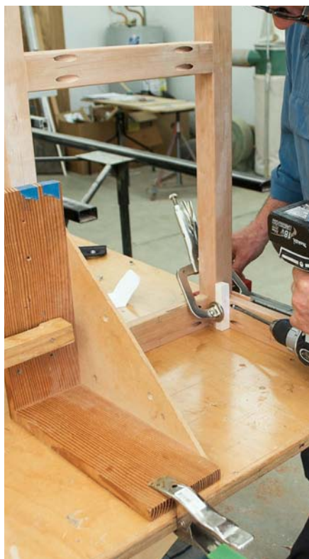
You'll need the right-angle jig to hold the sides upright during assembly
