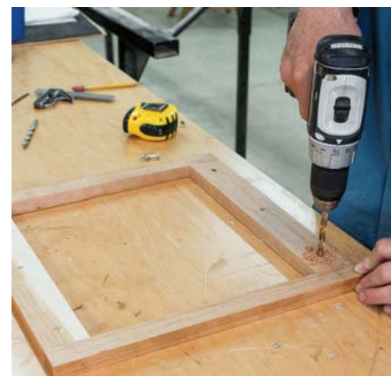
Drill oversize holes in the spacer frame to allow for wood movement of the top at the edges
