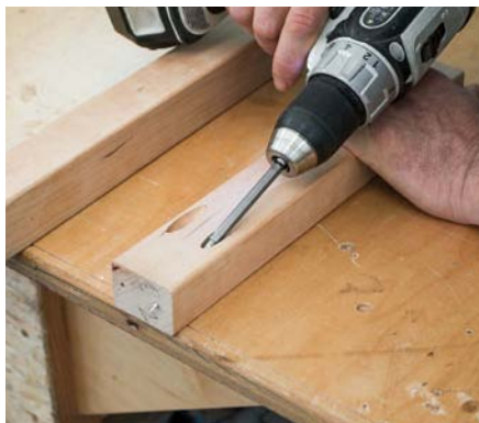
Drive the 2in screw through the hole in the stretcher to mark it for reaming with the extra-long \frac{1}{8} in bit
