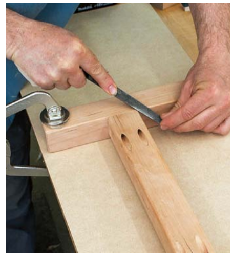
With the lower stretcher installed, finish the roundover on the leg above and below the stretcher
