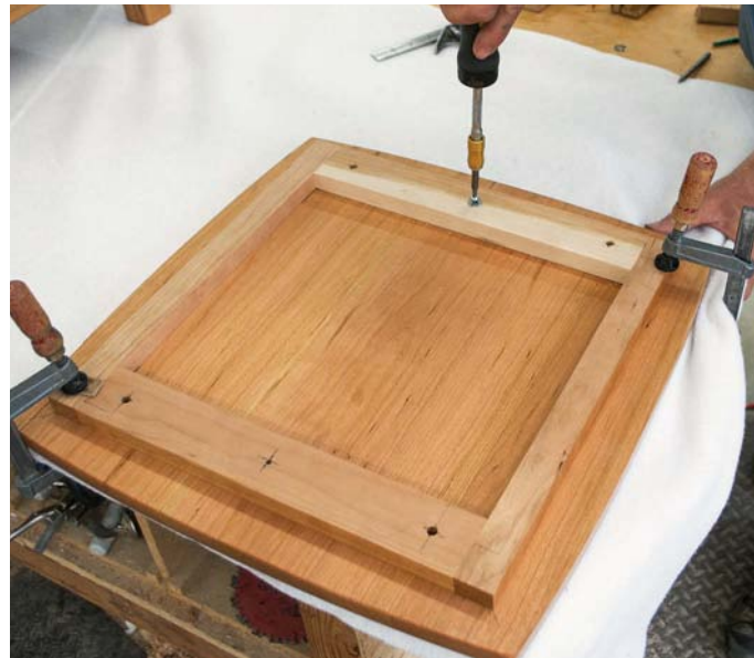
Attach the spacer frame to the tabletop with pocket screws and No.10 washers, driving the screws by hand
