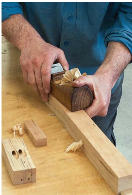
Nothing gets rid of machine marks faster than a sharp hand plane
