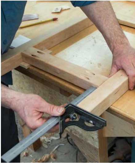
Use a square to locate the lower stretcher on the legs
