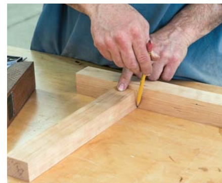
Mark the stretcher location on the legs to help you know where to stop and start the roundover edge on the leg
