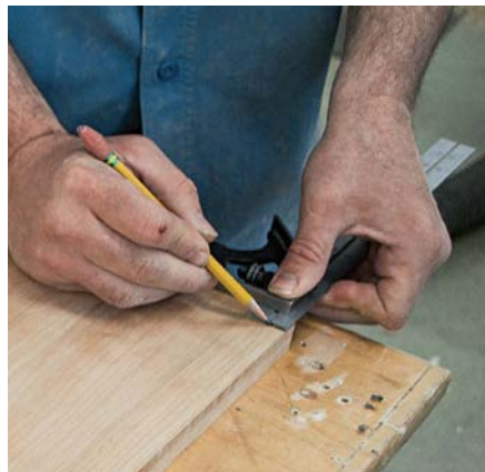
Measure in \frac{1}{2} in on both sides of the corner to mark the point that the curve will pass through
