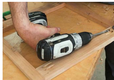
Hold the spacer frame joint with the face clamp while driving the pocket screws
