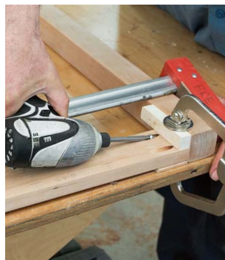
Use a bar clamp and a face clamp to hold the leg/skirt assembly in place while driving the pocket screws
