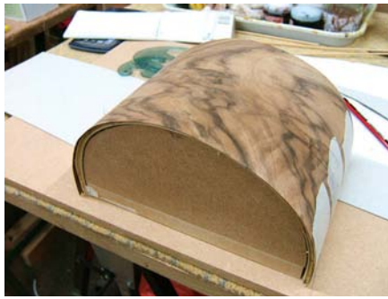
Once the glue had set the arch was cut to length and width
