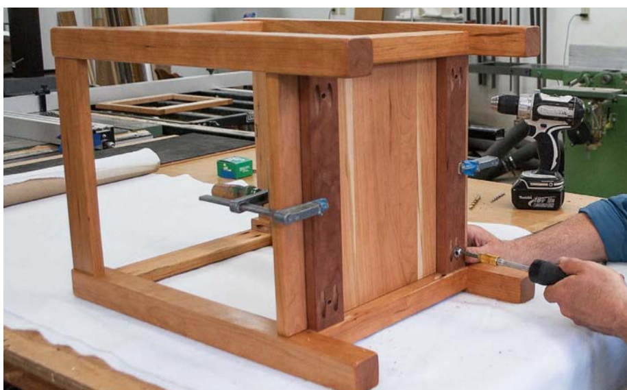
Attach the lower shelf with pocket screws and No.10 washers. Drive the screws by hand to ensure the holes don't get stripped out
