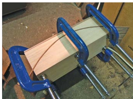
The case side and former block with the walnut laminate between
