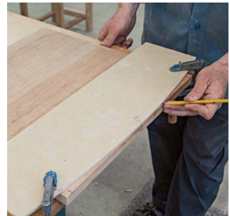
Align the template on the tabletop so that the centre and end marks match. Trace the outline onto the top
