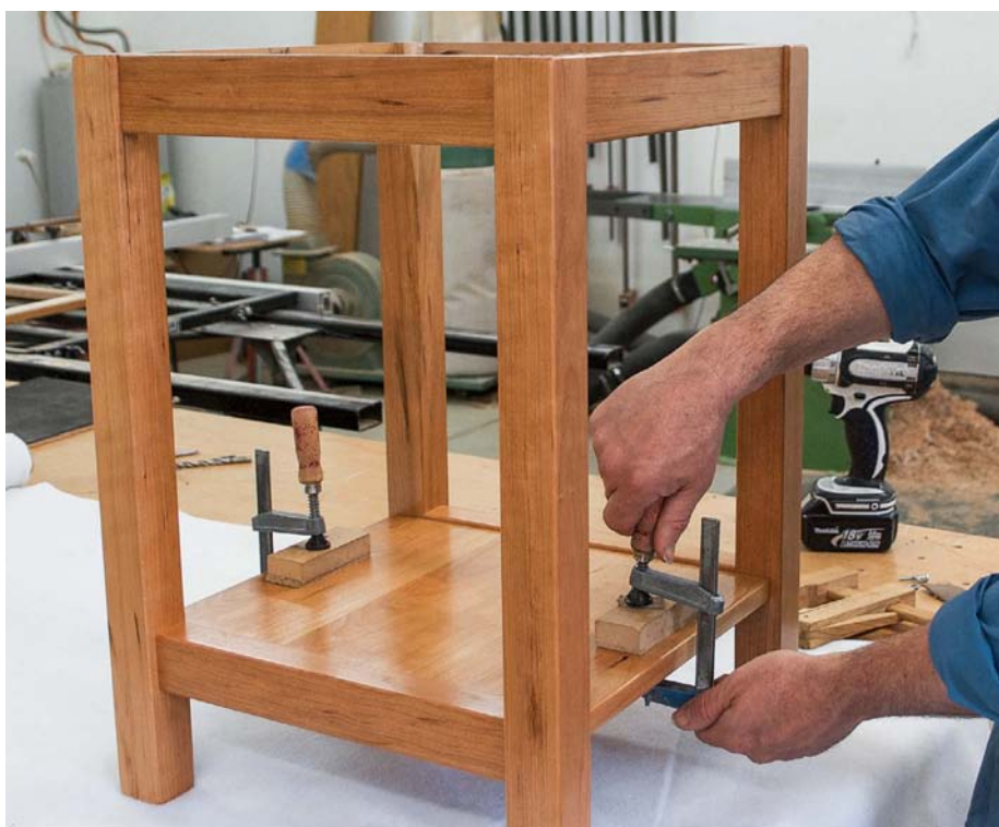
Clamp the shelf in place using protective cauls against the finished surface
