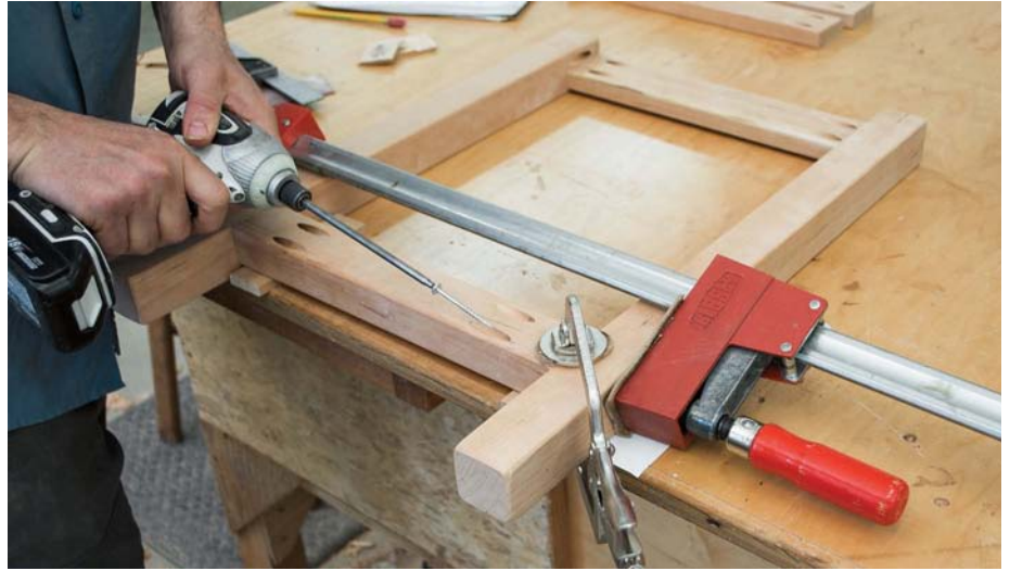
With bar and face clamps holding the assembly, slowly drive the long screw through the lower stretcher and into the leg
