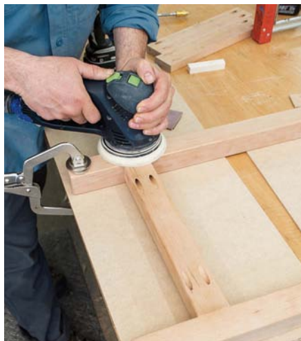
Flush-sand the butt joint between the leg and the stretcher after assembly
