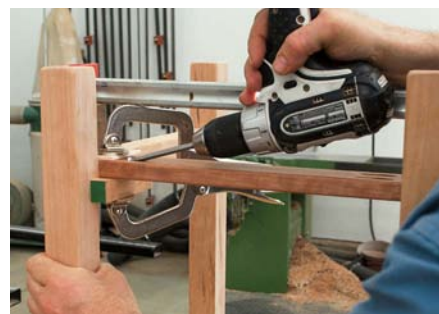
With the face clamp holding the shims in place, drive pocket screws through the shelf support into the lower stretcher. A bar clamp across the support provides added security against slippage
