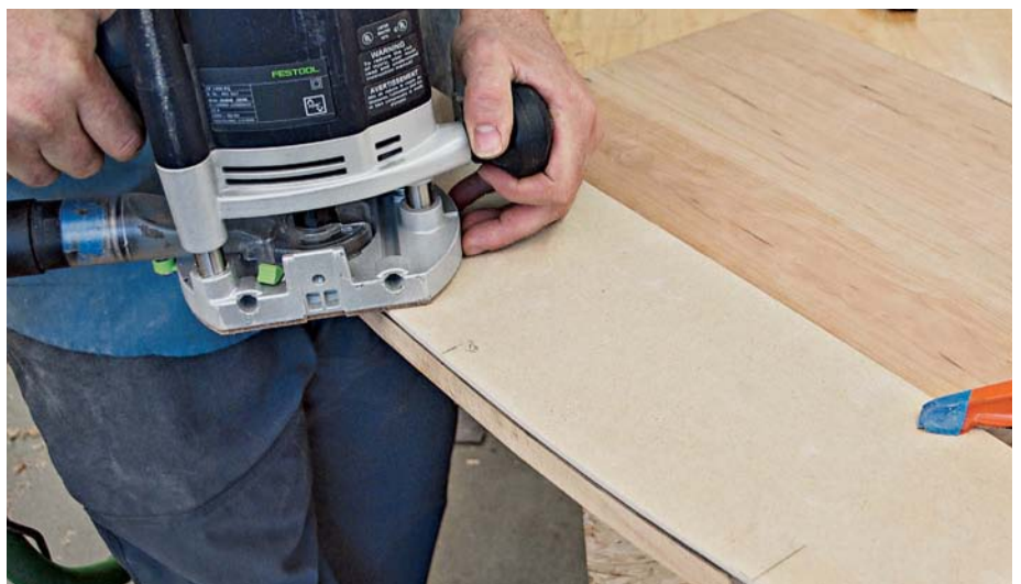
Use a router with a bearing in the middle; this will allow you to follow the template and clean up any saw marks
