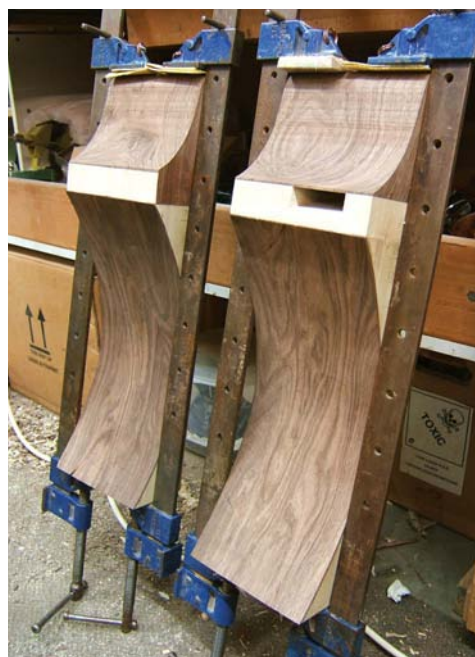
The sides clamped with the top rebates protected and chime cutout shown
