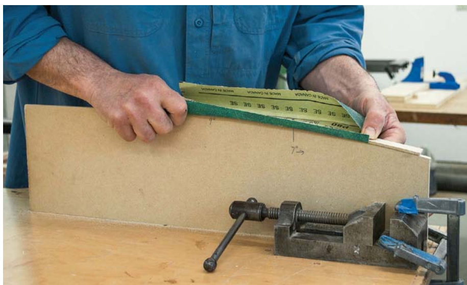
Clean up the cut marks on the half template using a strip of wood wrapped with 80 grit sandpaper
