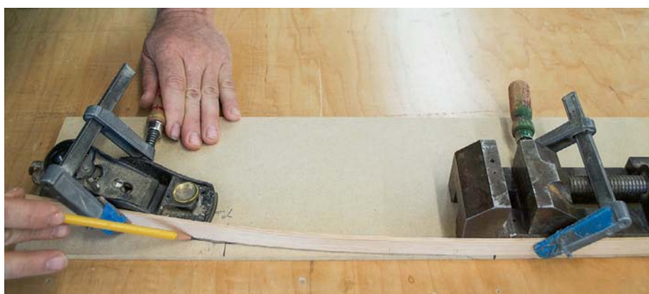
Clamp the batten to some heavy shop objects to help create a curve and to hold it in place while tracing the template
