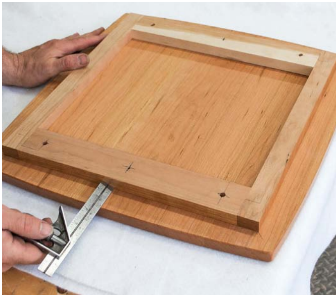
Mark the diagonals on the underside of the top to help locate the spacer frame, then use the diagonal marks and a square to centre the frame on the top
