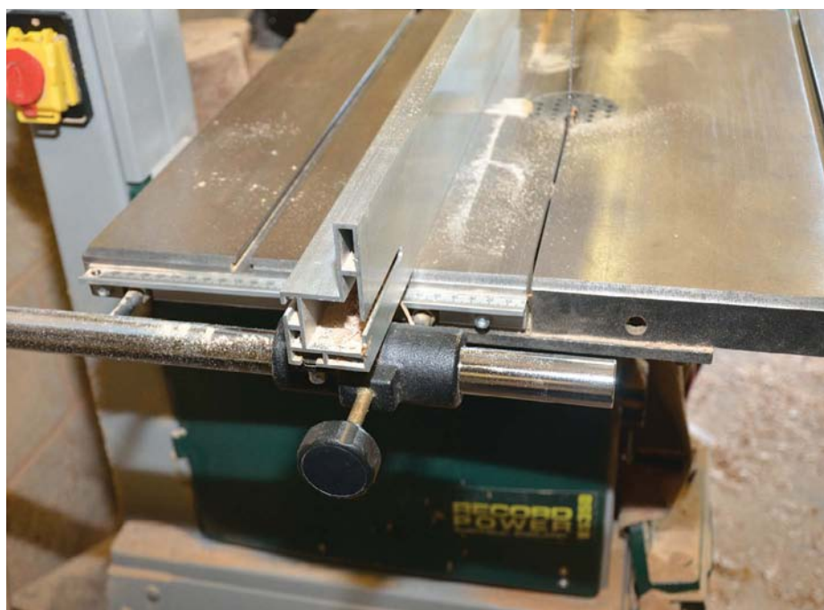
The chromed fence bar is very rigid and easily adjustable for accuracy
