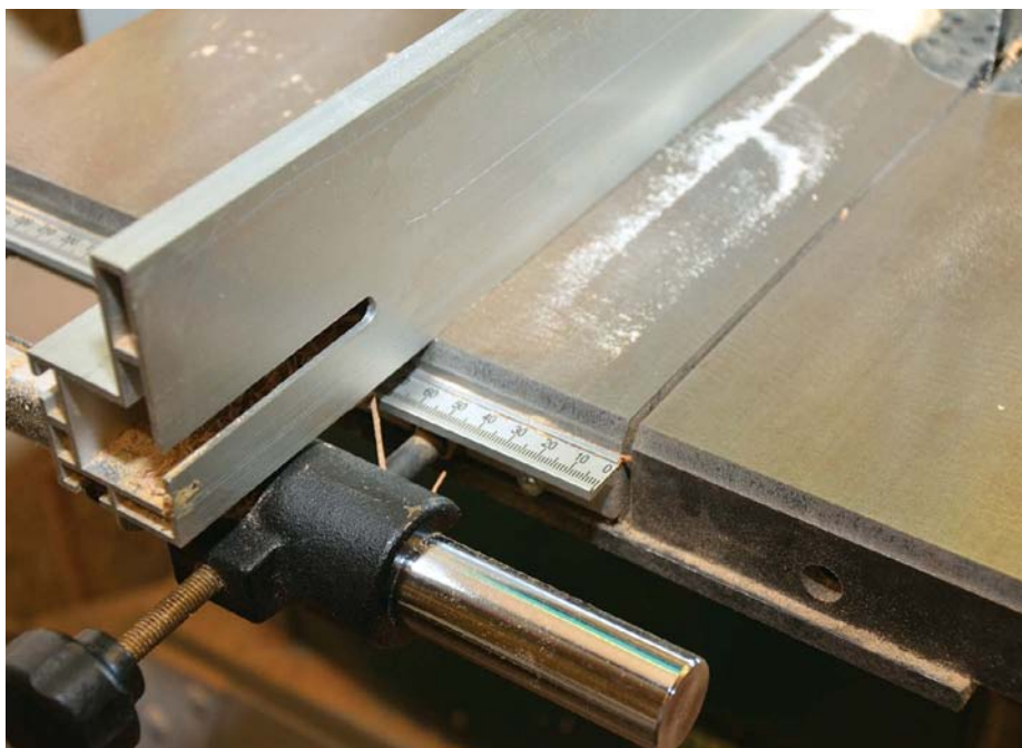
Rip width scale is accurate and easy to see
