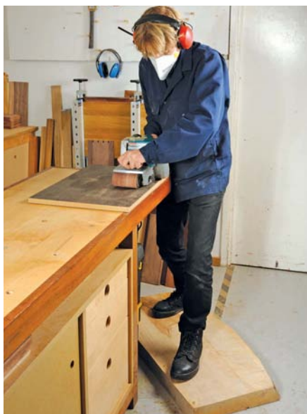
An ergonomic platform for sanding operations, using a thick board
