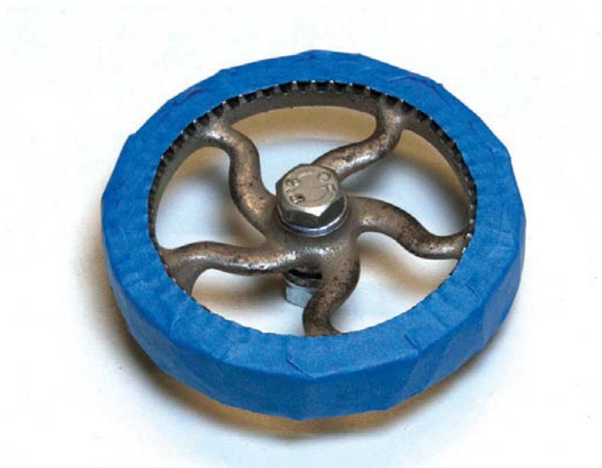
Masking tape was used to prevent spray paint getting on unwanted areas
