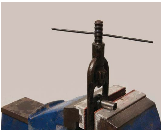
Two more dowel pins had to be removed before the handle could be removed
