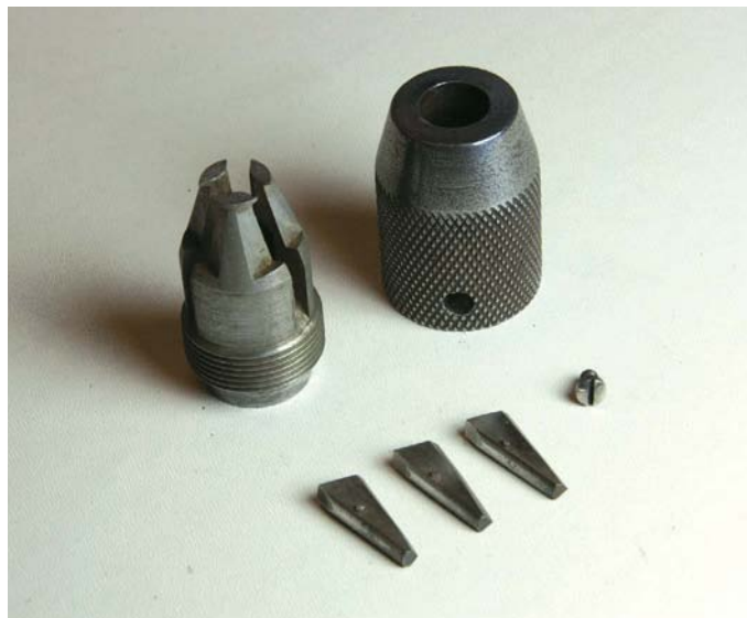
100 years' worth of dirt and rust was removed by hand
