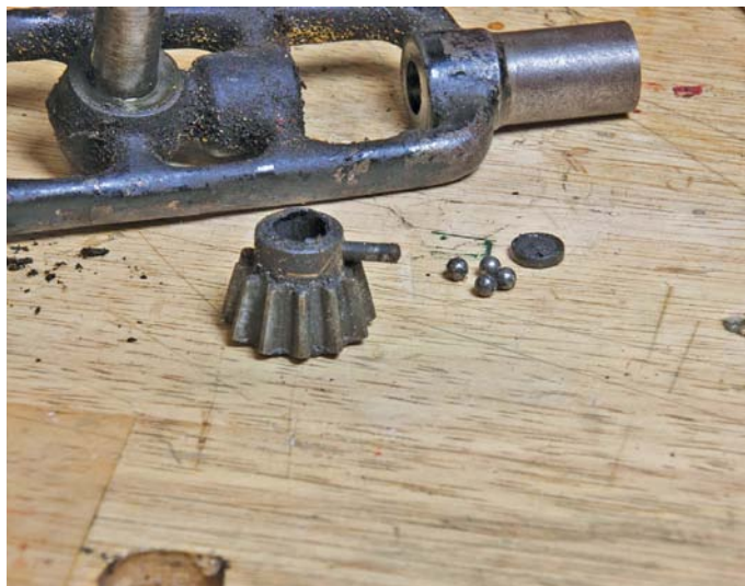
I made sure to keep an eye on the small components of the thrust bearing
