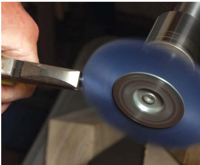
To hold nails and other small components steady, pliers came in handy
