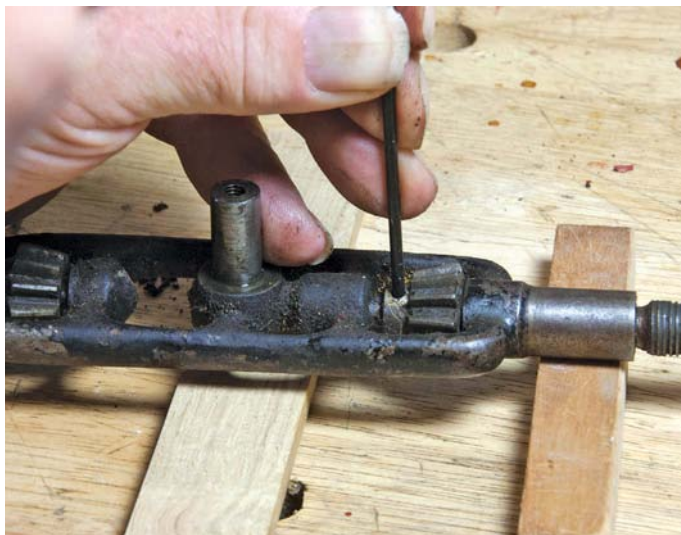
Dismantling the tool was mostly done through the unscrewing of components
