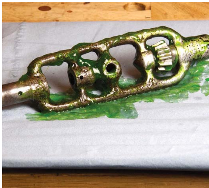
Rust removing gel was used
