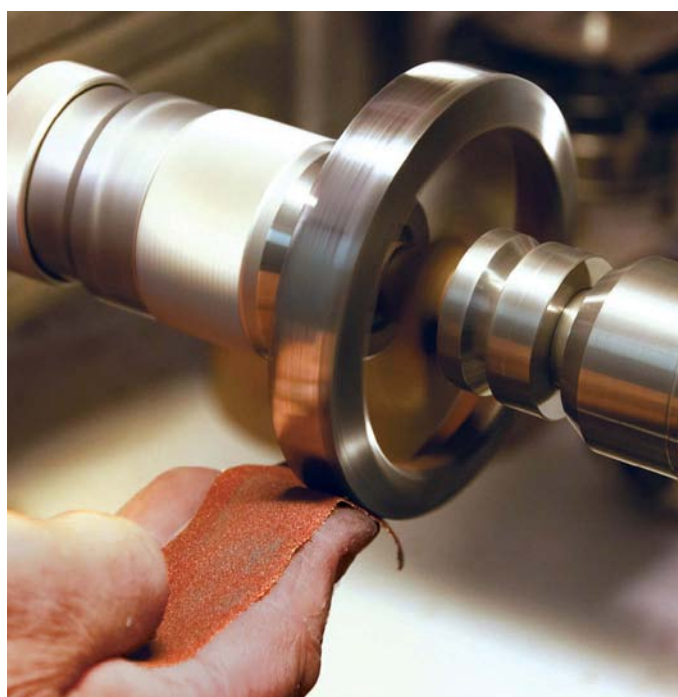
Removing the ‘patina’ or rust
