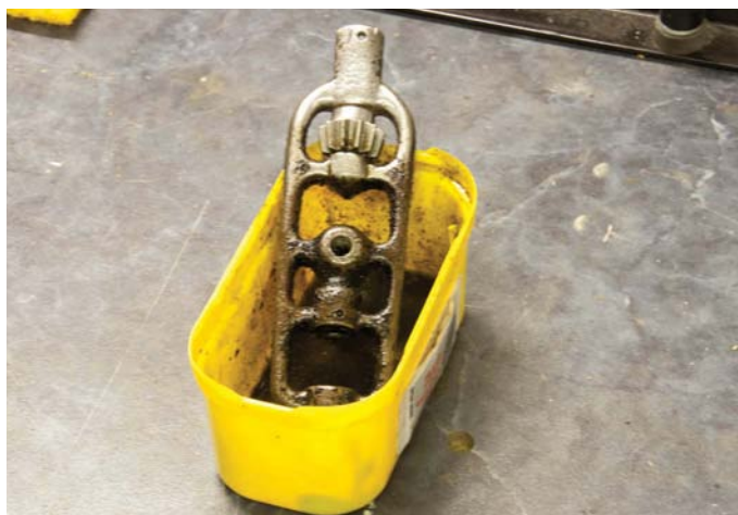
The remnants of finish were removed with a combination of stripping gel and scrubbing
