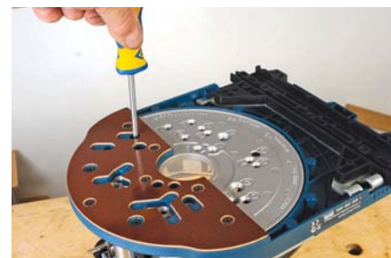
The accessory kit includes an adaptor base for Bosch and other router makes, so you can use the guiderail system
