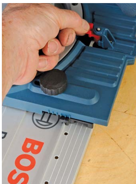
The adaptor base includes an accessory drop-pin to use with the holes in the special piece of guiderail, which features exactly 32mm spaced carcass drillings
