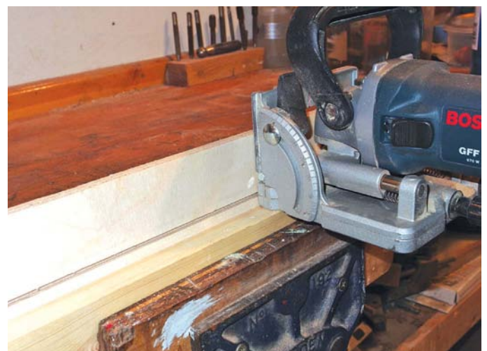
The doors were slotted by mounting them in the vice
