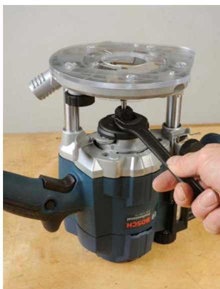
One spanner plus spindle lock makes cutter changing easy
