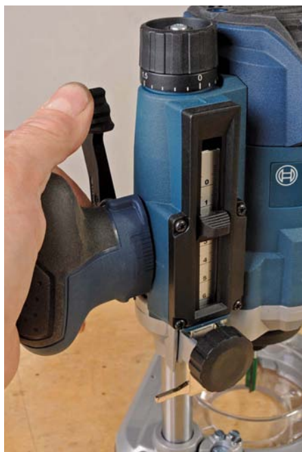
This plunge lock has much more sprung leverage than previous iterations
