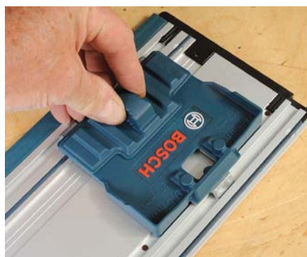
There is even a sprung fit end stop so you can get the positioning exact on each carcass panel
