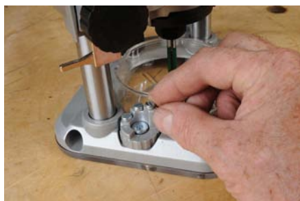
Some things never change – Bosch's standard five-stage depth turret
