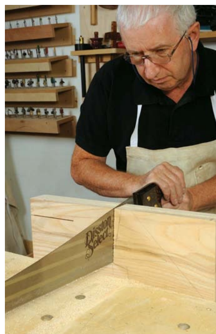
Making a quick clean cut in some 50mm thick ash
