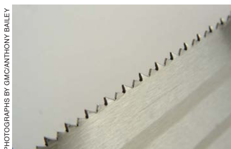
The saw features carefully crosscut sharpened and set teeth
