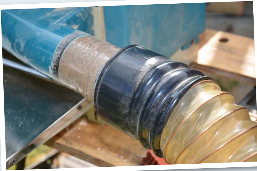
100mm adaptor cuff allows flexible use
