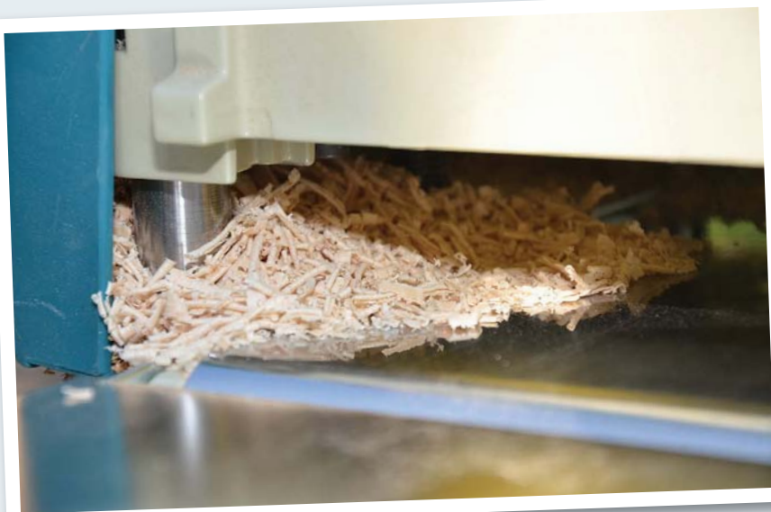
Chippings can sometimes stop cutter head movement so needs vacuuming out
