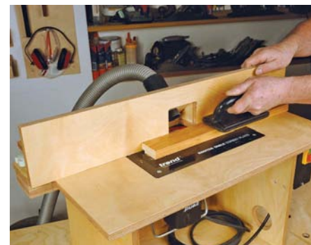
Wider boards can be easily rebated
