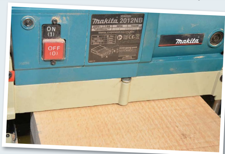
Pin is a quick guide to depth of cut setting
