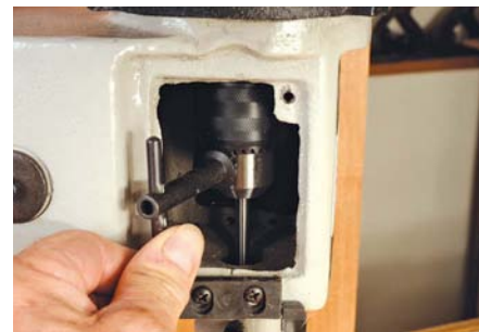
Accessing the CM2's chuck to tighten the drill bit
