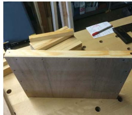
Edge detail of the drawer construction
