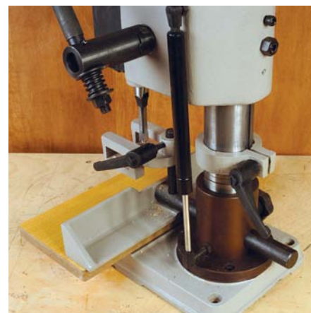
The piston that supports the mortiser head of the machine
