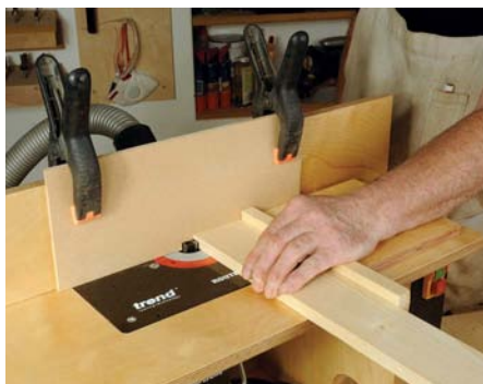
Use a 'breakthrough' fence and pushblock
