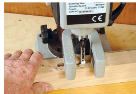
A downward work clamp holds the workpiece securely
