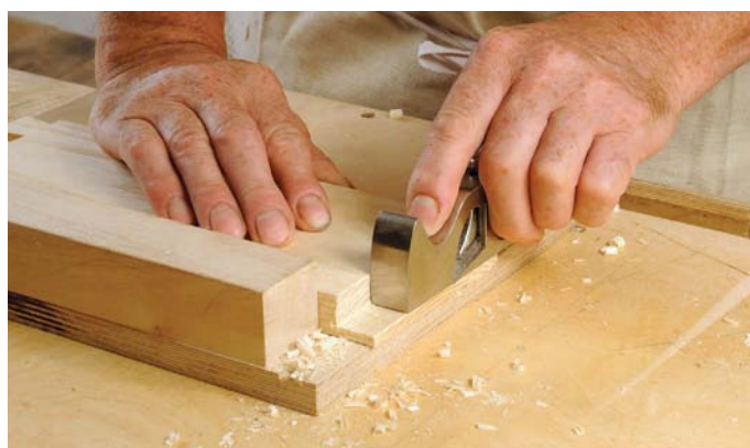
Cleaning up a rebate is quick and easy
