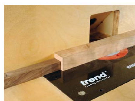
First, an outfeed support to fit the rebate
