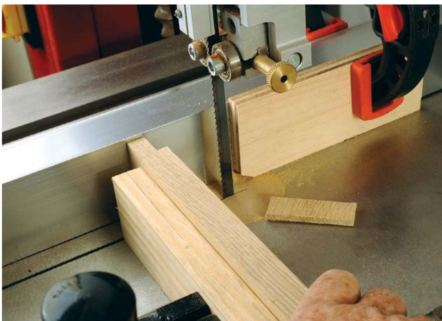
Here an end stop is in place for the rip cut, shoulder cut taking place
