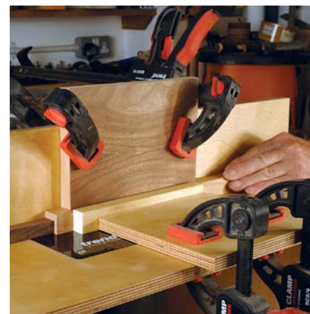
Followed by hold-downs to enclose the workpiece
