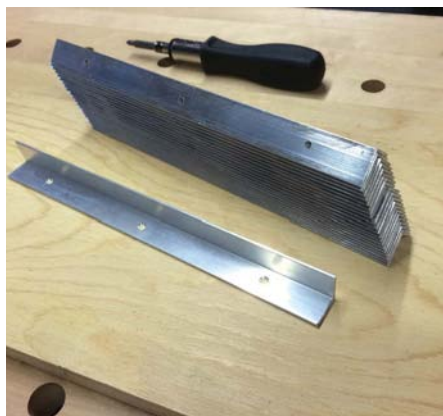
'L'-section aluminium was cut to length and drilled
