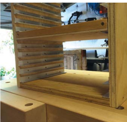
A test fit was required to make sure the drawers would slide
