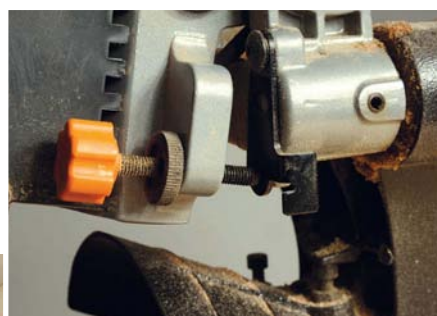
Clamp it in place before making cuts
