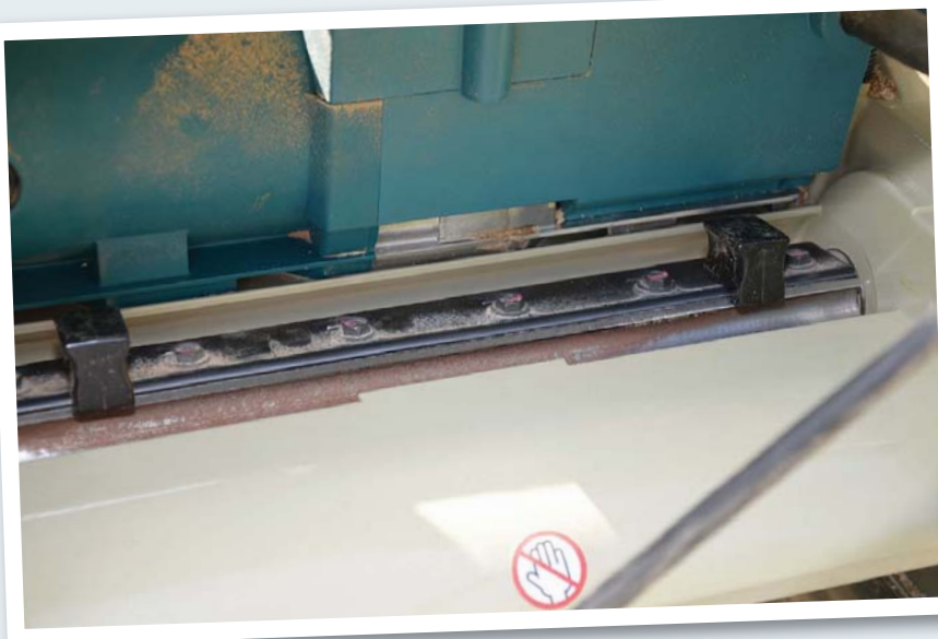
use magnets to set cutters in groove
