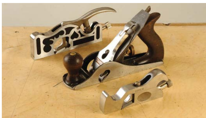
From top to bottom: cabinetmaker's shoulder rebate, carriage maker's rebate and a small shoulder rebate
