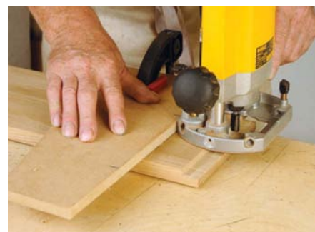
Clamp it in place before making cuts
