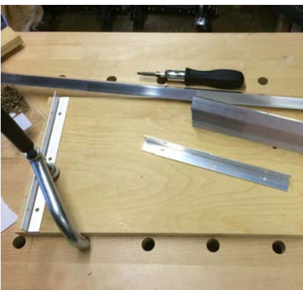
Setting out the first runner
