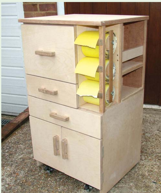
You can use a mixture of drawers and cupboards for greater versatility. This unit provides easy access to a range of abrasives and sanders
