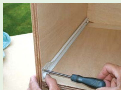
An alternative to using frames is to use a plywood or MDF carcass, with one part of the drawer runners attached to each side. This method can be used for static or mobile units
