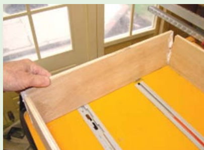
Drawers can be made by cutting 12mm thick plywood sides and using biscuits to join them
