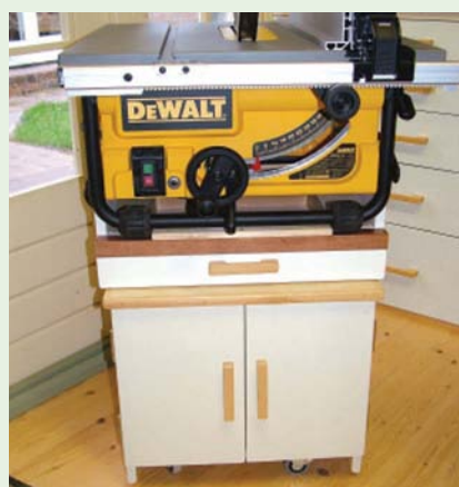
This bench saw unit incorporates a cupboard below to store associated items, as well as a pull-out tray to collect dust that falls through the saw
