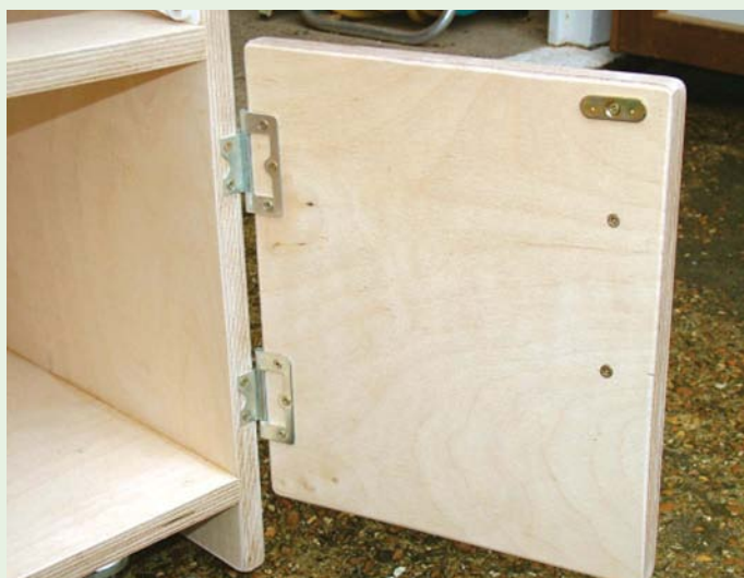
A simple door can be made from a panel of MDF or plywood
