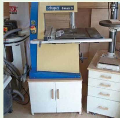
Even heavy-duty machines can be mounted in this way; this bandsaw weighs 69kg, so the mobile unit must have a sufficient footprint for stability
