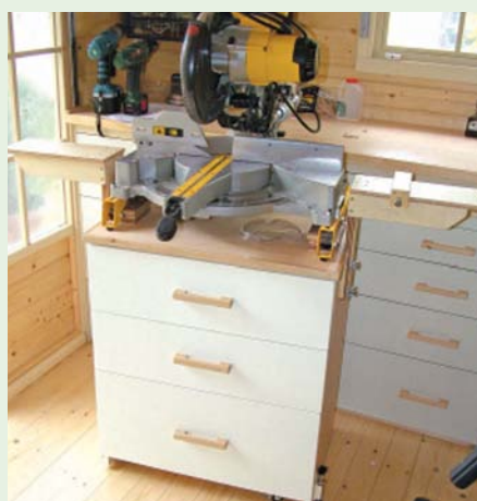
This sliding chop saw is mounted on a mobile drawer unit, incorporating removable extension tables
