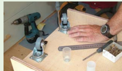
Fitting castors to the base of the mobile unit
