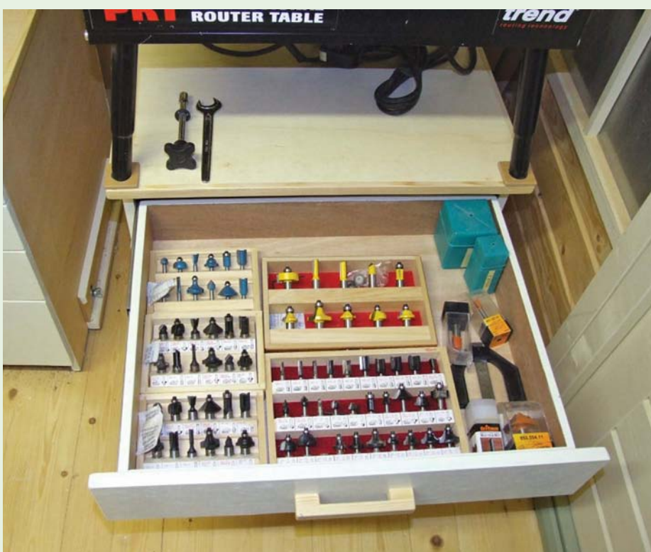
Fully extending drawer runners allow better access to contents
