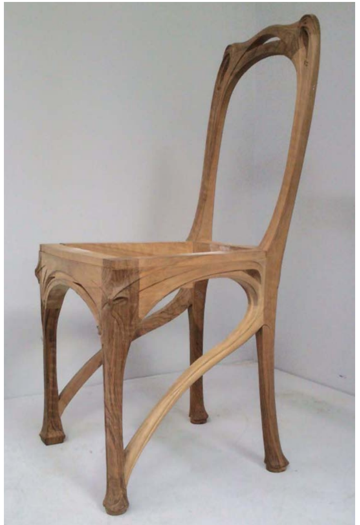
Left: Patrick elected to use standard PVA glue for the joint assembly of the final piece
