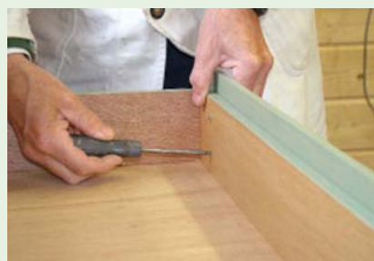
Check that all the drawers open and close and maintain the correct spacing. Then, use the screws to attach the handle and the drawer front to the false front
