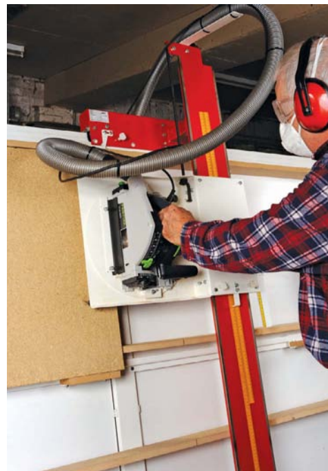
The ZM uses a portable standard saw
