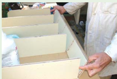
A simple shelving unit can be made using lengths of plywood attached with biscuits, screws and adhesive
