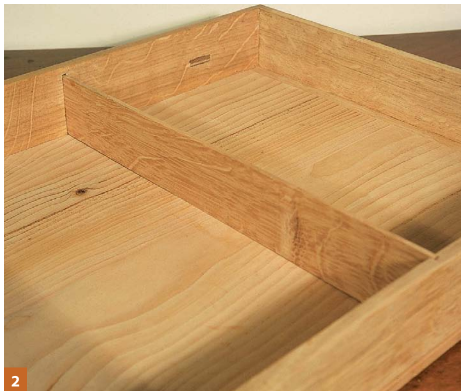
Here is a completed drawer. Note the mortised handles, removable divider and flush drawer slips
