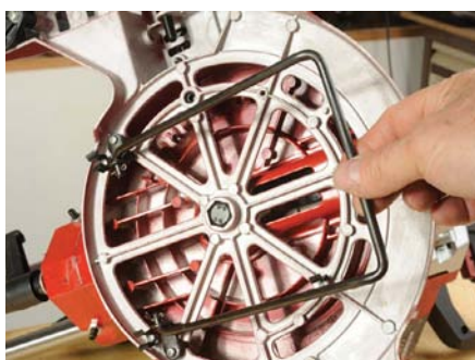
A flip-out anti-tilt frame
