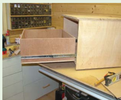
An alternative ball-bearing drawer runner type allows full opening
