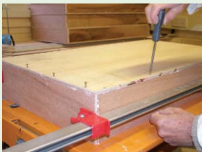
Screw the bottom to the drawer frame, ensuring that the resulting drawer is square
