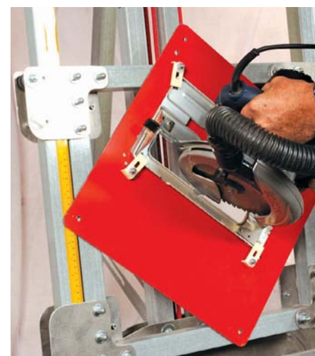
The panel is turned when converting to rip cuts
