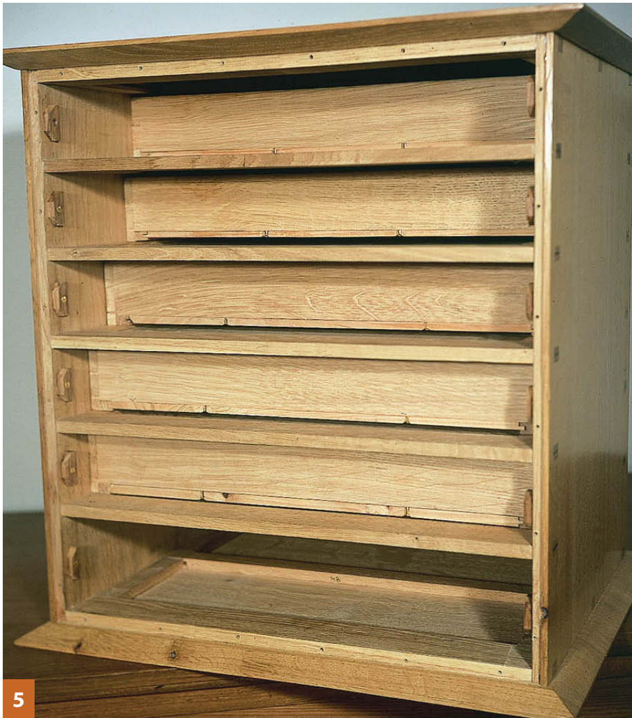
5 Rear view with back removed. Unconventionally placed drawer stops are technically incorrect but work well in a piece this small. Slots for screws securing solid cedar drawer bottoms allow seasonal movement
