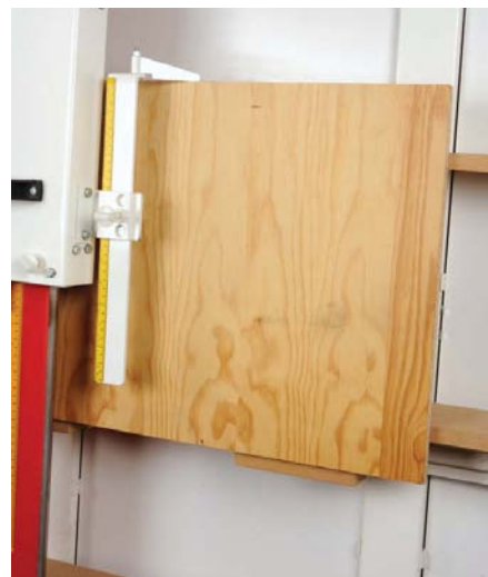
Repeat rip cuts are made with this scale
