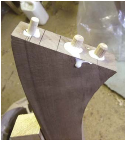
Left: Patrick elected to use standard PVA glue for the joint assembly of the final piece
