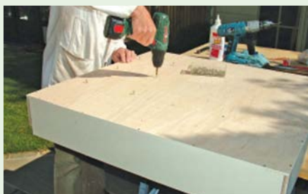
Adding a backing will greatly strengthen the assembly
