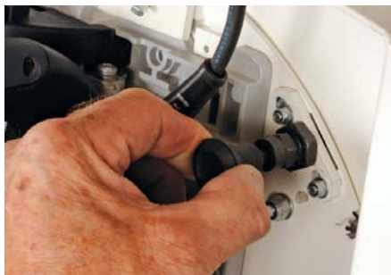
A lock pin allows changing from cross-cut to rip cut
