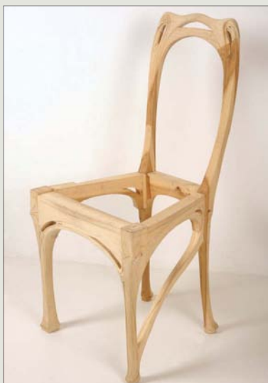
Patrick made a wise decision to do a basic prototype in tulipwood
