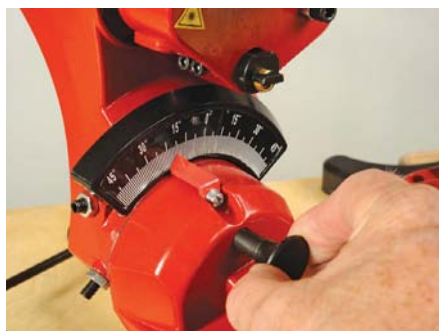
The spring lock pin allows the saw head to move to the right
