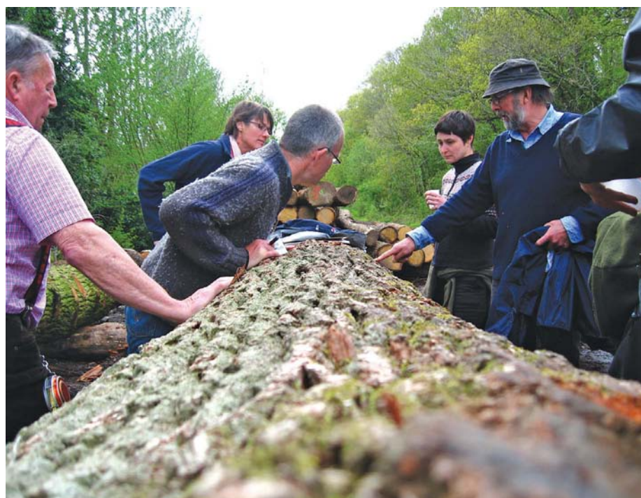
Tutors, Gavin Munro (left) and Will Bullough (right) explaining defects in an oak butt
