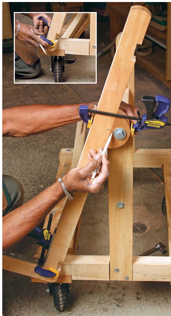
Locate the panel support. After marking the two L-shaped pieces and notching them for the crosspieces, but before gluing in the crosspieces, you need to locate the Ls on the uprights. To do this, bold a semicircle pivot block to its upright and clamp one of the Ls to the top of the base so its lower crosspiece will hit the base about 5in from the upright. Mark the block's location on the L
