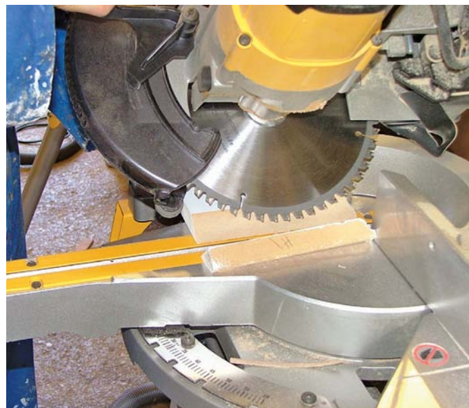
Cut the required mitres for the corner joints
