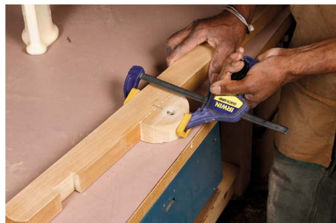
Glue on the pivot block. With the pivot block marked for position, glue and clamp one to each L. Now you can glue in the crosspieces to complete the panel support frame
