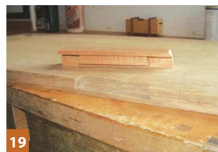
19 The handle is dovetailed to the lid
