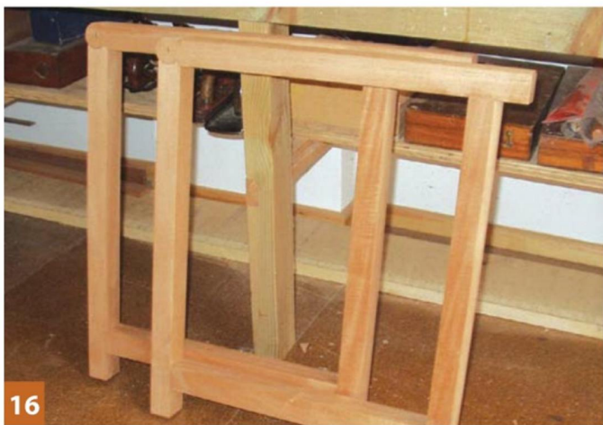
16 The frames dry-assembled
