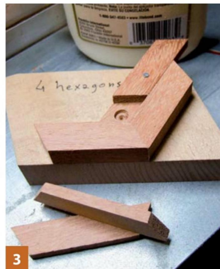
3 The jig is used initially for gluing up
