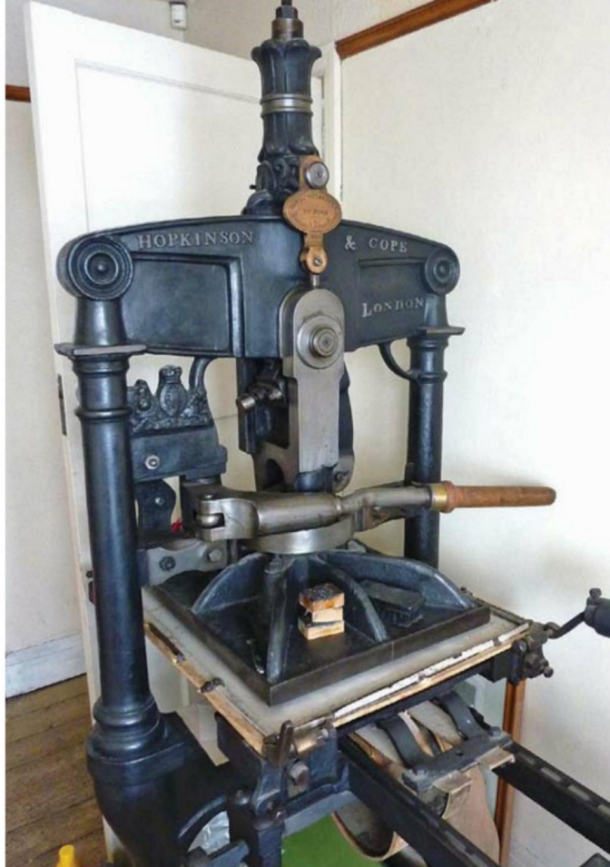
The Albion press, manufactured in the 19th century by Hopkinson and Cope of Finsbury, London
