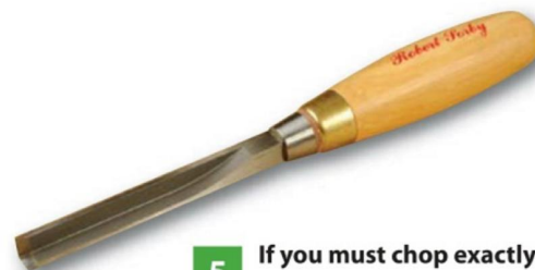
4 These skew chisels need to be bought as a pair. The points are quite dangerous so care is needed
