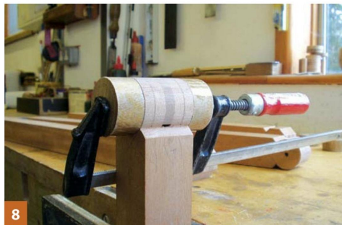
8 Spaces between knuckles are filled during shaping; the plane catches the Sellotape when you have gone far enough
