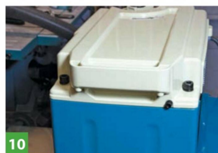
10 You can carry a 'portable' thicknesser but take care as they are heavy. A trolley is the safer option
