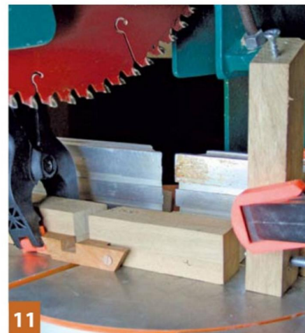
11 The jig is moved sideways between cuts
