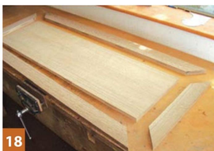
18 The lid is made up of a solid frame biscuitied to the central veneered panel
