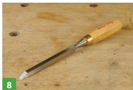
8 Note the hefty, thick blade metal on this sash mortise. If more force is needed, use a hooped 'registered' pattern instead
