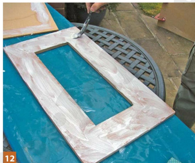
12 The frame is then coated with adhesive
