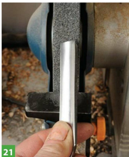
There is a knack to rolling the tool on the abrasive wheel so you get a regular curved grind
