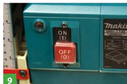
9 It won't restart itself after the power cuts out, but still unplug it for maintenance
