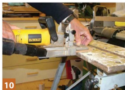
10 Cutting size 20 biscuit slots to join the rails and stiles
