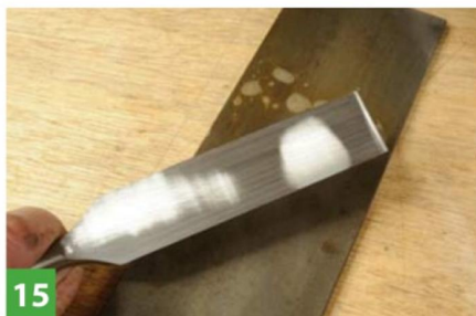
A new chisel can be surprisingly uneven when you try flattening the back
