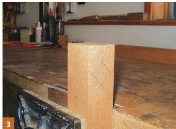
3 Marking the barrel, shoulders and V-shaped clearance
