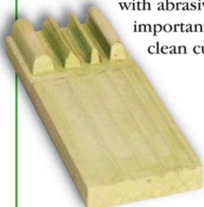
This waterstone is shaped to match carving tool and gouge profiles
