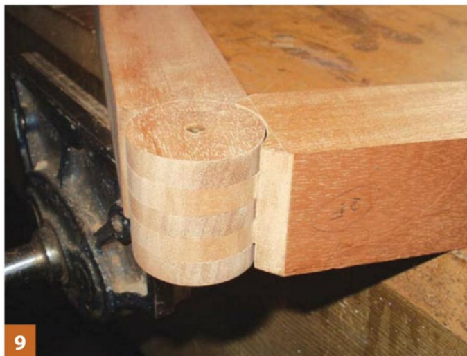
9 The completed joint prior to cleaning up
