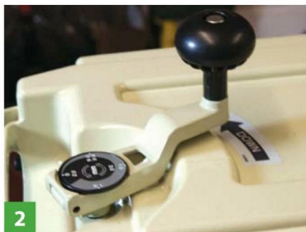
2 This indicator plate can be turned to zero, there's a front scale and pointer too
