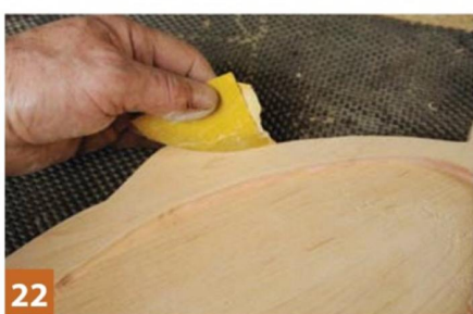
22 'Break' the edges with abrasive so the platter is safe and pleasant to the touch
