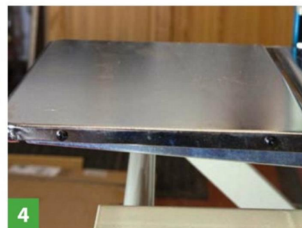
4 Experiment with setting the infeed and outfeed table heights
