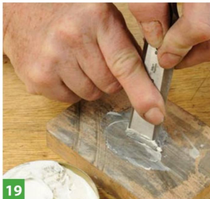
After polishing both back and micro bevel it is worth dragging the edge vertically to give a last polish to the edge
