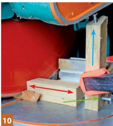
10 The vertical piece – on the right – has an adjustment screw
