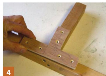
4 A plywood T-piece for added strength
