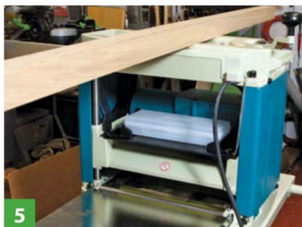
5 The machine top is normally intended to take boards being passed back ready for the next cut pass. Some tops have rollers
