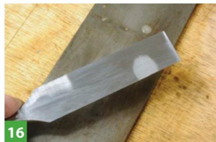
This chisel is nearly flat, even the edge has a slight dip to be removed
