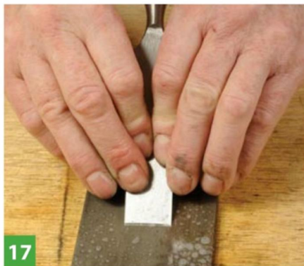
A honing guide is essential for obtaining a flat micro bevel at the correct angle
