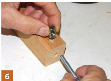
6 To further improve the joint of the frame members use a cross dowel
