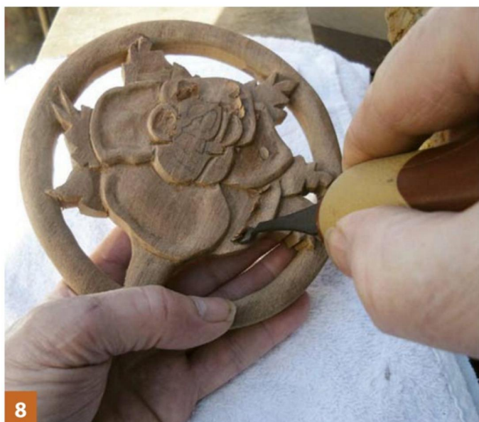
8 A spoon gouge affords easy control on concave surfaces
