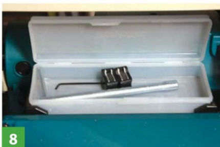
8 The toolkit will be needed eventually when blade blunting or scoring occurs
