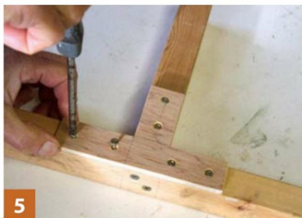
5 Screw the T-piece to the frame to reinforce the adhesive joint
