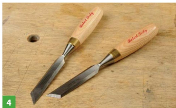
4 These skew chisels need to be bought as a pair. The points are quite dangerous so care is needed
