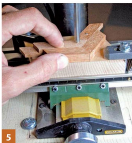
5 Drilling the magnet holes using the jig
