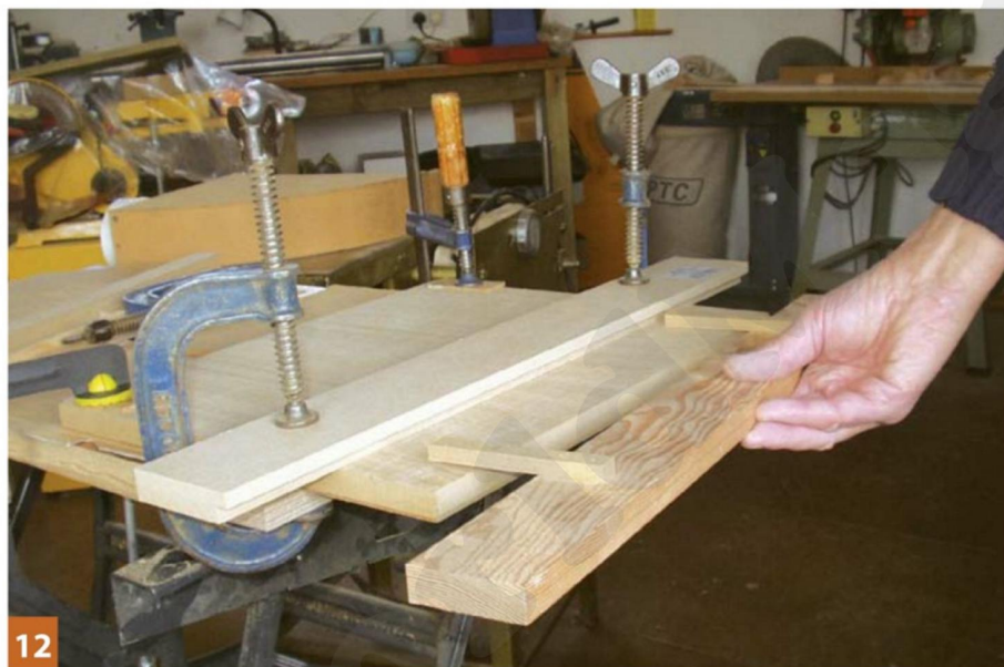
12 A simple jig is made to set the guide bar the exact distance in from the end of the board for each mitre
