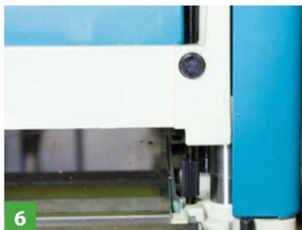
6 A depth stop is useful for refinding an exact finish thickness, but retract it when not required
