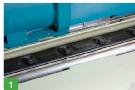
1 When blade changing the power must be disconnected
