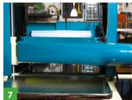
7 Extraction is pretty essential unless you don't mind your workshop being sprayed with chippings!
