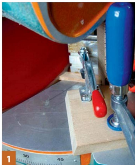
1 The workclamp is essential for safe working
