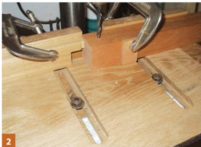
2 The drill is constantly withdrawn to clear the waste
