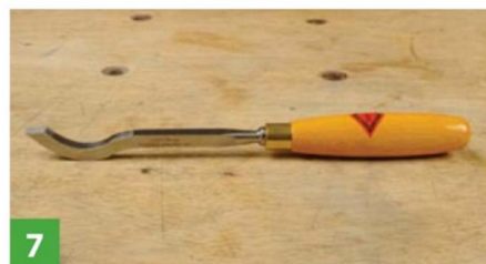
7 The swan neck chisel is very much a levering tool, not intended to be struck
