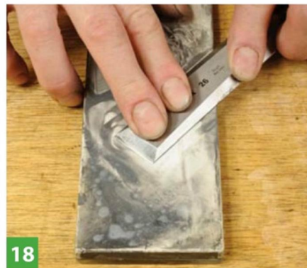
Ceramic stones give a subtler finish to the cutting edge
