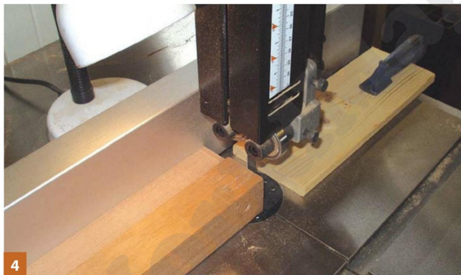
4 The waste was cut out from the knuckle using a bandsaw with a sharp, new blade
