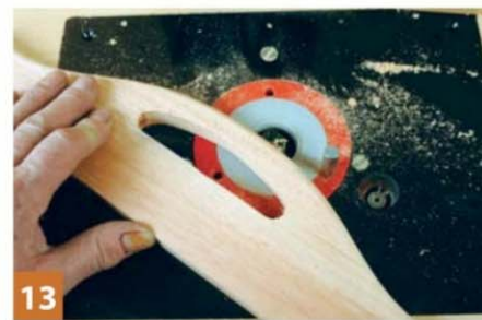
13 You will need the lead-in pin here to avoid any kick-away by the cutter
