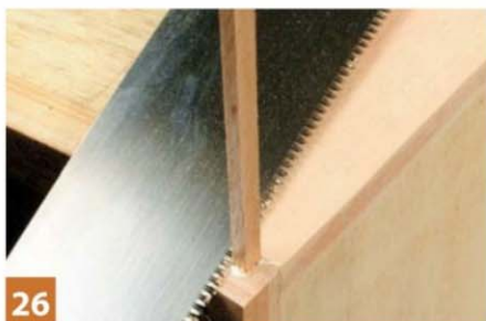
26 Once this fillet is trimmed off and sanded the groove will become invisible
