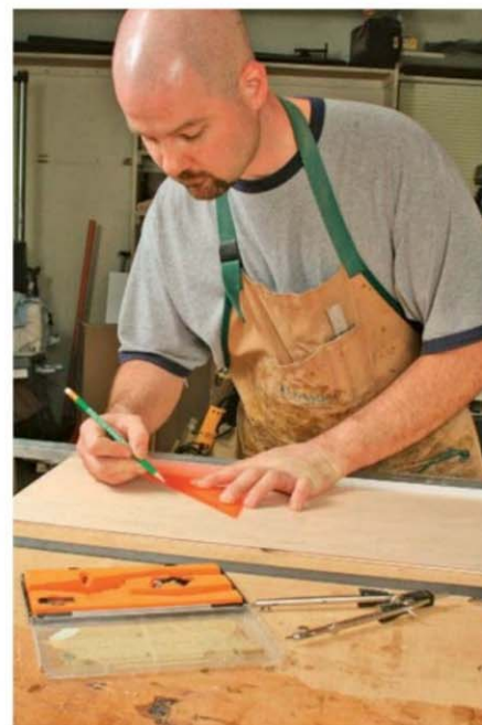
Lay out the slots. Align the template and the triangle against a straightedge clamped to the bench to draw the shelf outlines from
