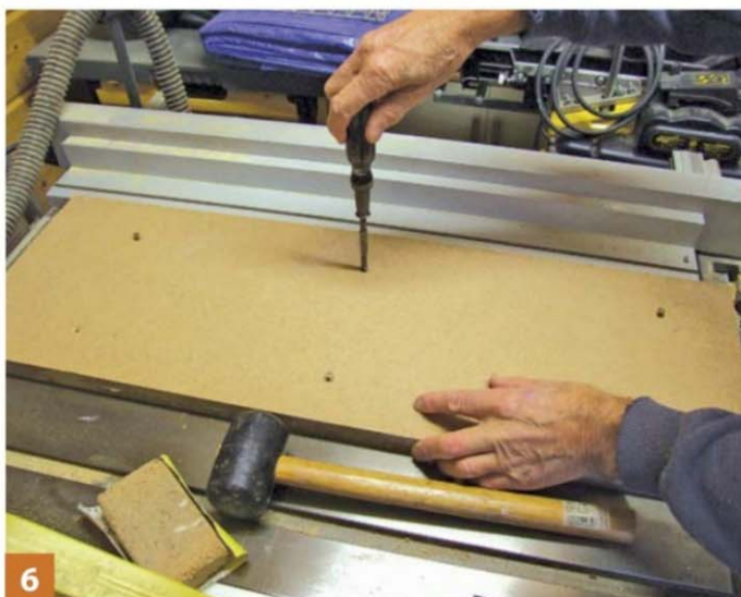
6 Screws help to ensure the two sheets are fully pressed together
