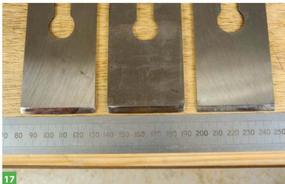
Edge profiles L to R: No.5 Jack - camber edge, No.3 and No.4 Smoothing - relieved corners, No.6 Fore, No.7 and 8 Jointer - straight
