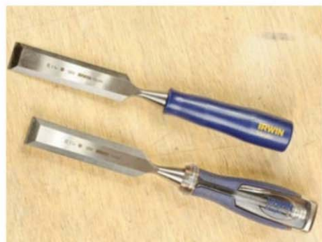
The Blue Chip on the left is meant for benchwork, whereas the High Impact version on the right has a striking cap and the blade metal continues as a rod right up to the cap
