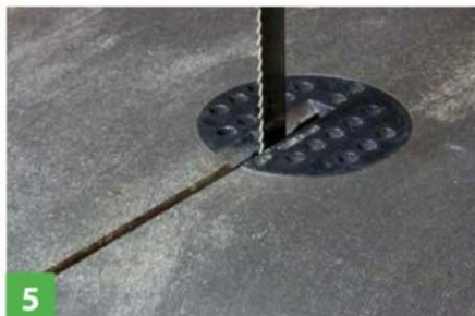
5 The cast table has a removable insert to access the lower guides
