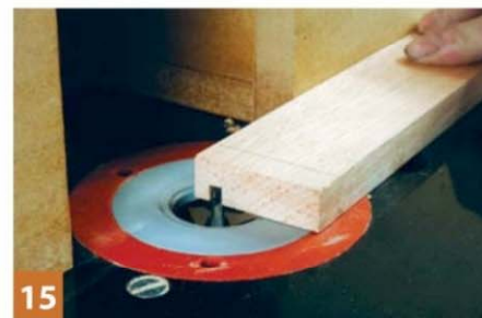
15 Do repeated passes to clear the tightly packed chippings
