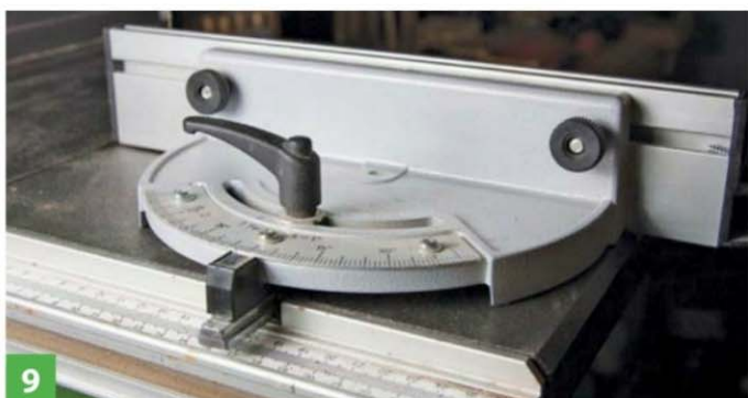
9 A mitre gauge is useful for cross cutting and angled cuts
