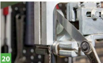
20 Use a feeler gauge to check the thrust bearing clearance
