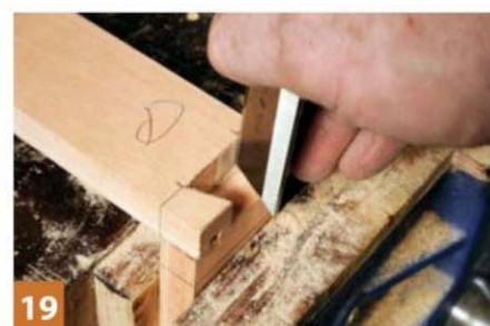
19 The chisel is being used to transfer the socket shape to the dovetail portion
