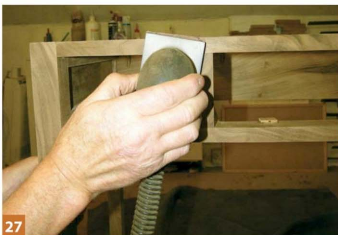
27 Hand sanding to a final finish
