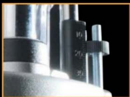
3-Stage Turret with direct reading scales for precise pre-set cut depths
