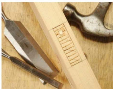
Always indent a chisel line all around the mortise markings so it delineates the cut area and severs the surface fibres neatly before chopping out
