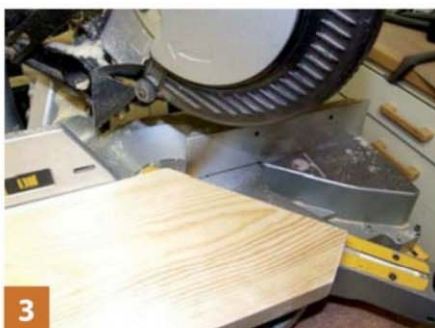
3 A piece is biscuit jointed on the underside of each stringer to take the weight evenly
