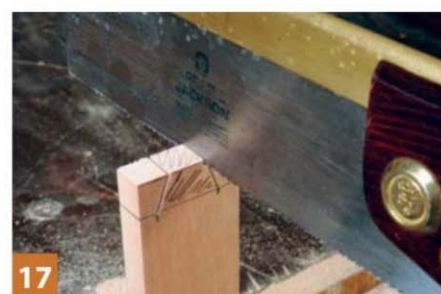
17 If you have a dovetail saw use it for a finer cut finish
