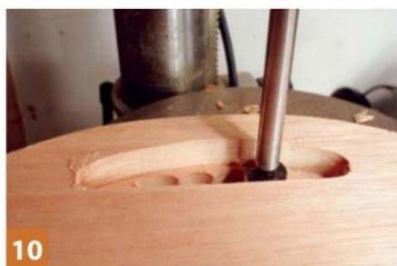
10 The Forstner will only take out a limited amount of material
