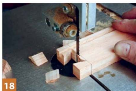
18 Repeated slices will take out the waste, or use a coping saw
