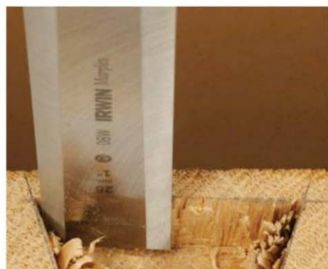
Square edge firmer chisels cannot undercut whereas a bevel edge chisel can
