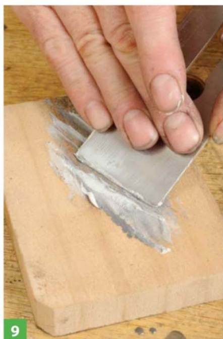
9 If you want to finesse the edge completely, then stropping it will give a polished finish
