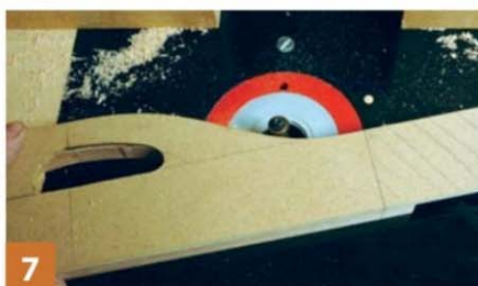
7 Machine from the left running down to the right – this will avoid tearout
