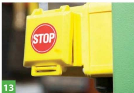
13 The NVR switch is a useful safety feature
