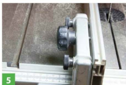
5 These adjusters enable the fence to be aligned for blade drift
