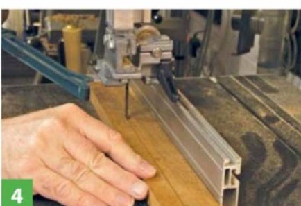
4 Always use a pushstick when ripping
