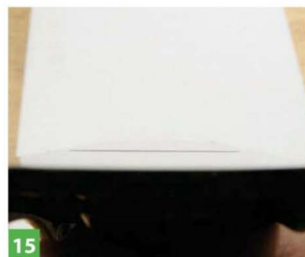
A razor thin, even line of 'blade show' is what you should achieve
