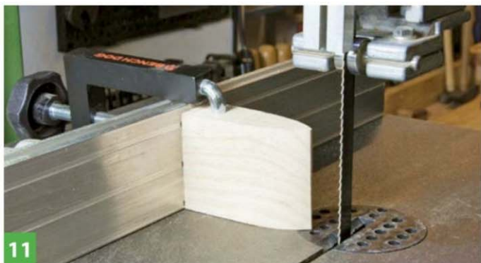
11 A single point fence is useful for curves
