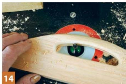
14 The machining direction is the opposite to an external cut
