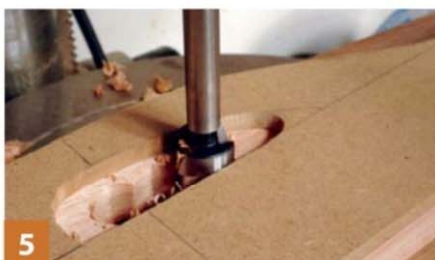
5 Do not let the Forstner clip the edge of the template. Start with it lower than the template but not touching the wood
