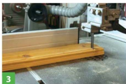
3 The mitre gauge helps with accurate crosscutting
