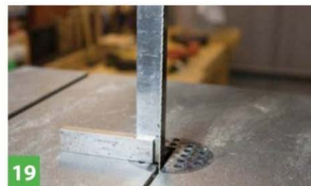
19 An engineer's square is useful for checking the blade is true
