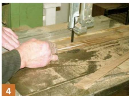
4 Sawing tapers on the inside faces of the legs using a pre cut ply taper jig against the fence
