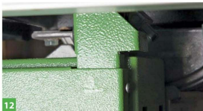
12 A guard protects fingers under the table
