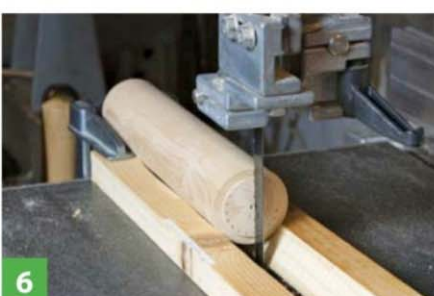
6 Round stock must be well supported
