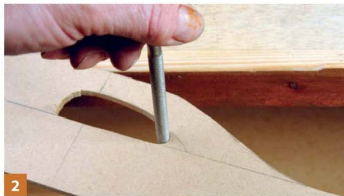
2 Standard metal files are quite suitable for cleaning up the shape
