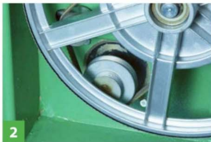
2 Speed is changed by moving the belt to a different pulley set
