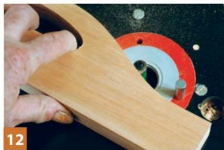
12 If you start from the middle of the handgrip a lead-in pin is not essential
