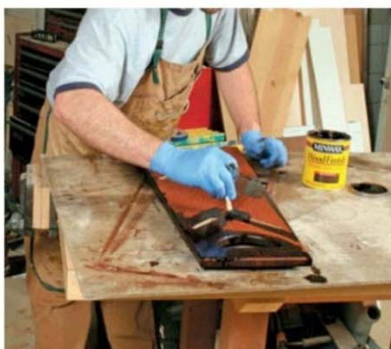
Dye, then stain. A brownish dye, followed by a darker oil stain, produces a finish that's very close to fumed oak. Mask the tenons to keep finish off glue surfaces. When applying the finish, work carefully to keep the stain out of the mortises
