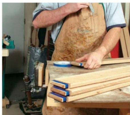
Dye, then stain. A brownish dye, followed by a darker oil stain, produces a finish that's very close to fumed oak. Mask the tenons to keep finish off glue surfaces. When applying the finish, work carefully to keep the stain out of the mortises
