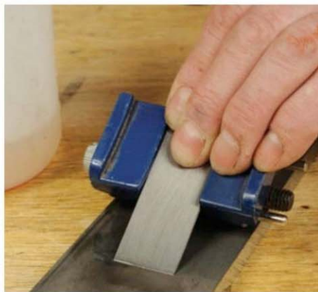
A 600 grit diamond plate with lapping fluid and a standard honing guide will give you the required 30° micro bevel very quickly
