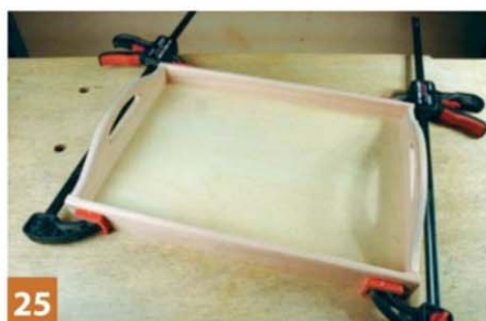
25 Care in clamping should result in tight, well-fitting joints
