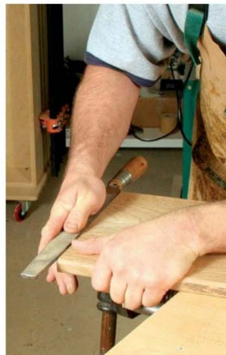
Fine-tune the fit. The tenons should fit into the mortises with hand pressure. At the end, you may need to remove a small amount of excess with a coarse file or alternatively a shoulder plane
