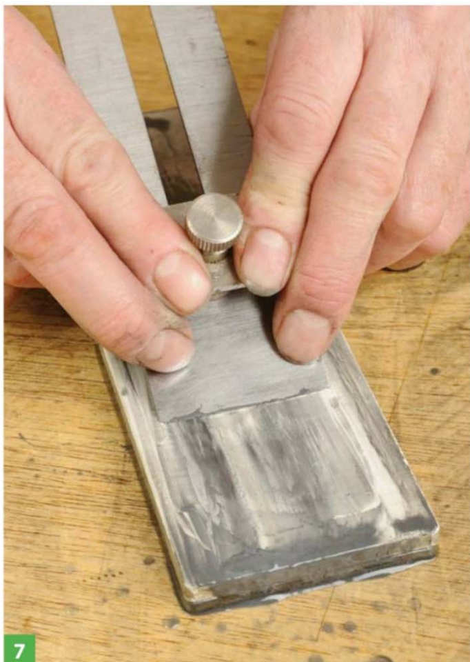
7 I like using a ceramic stone after diamond because it improves on the slightly raw sharpness left by diamond honing
