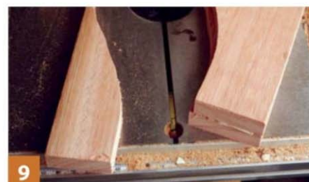
9 Leave about 2-3mm overhang to machine off later
