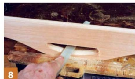
8 The file needs to push at a diagonal to cut both across and lengthways so the curve is smooth
