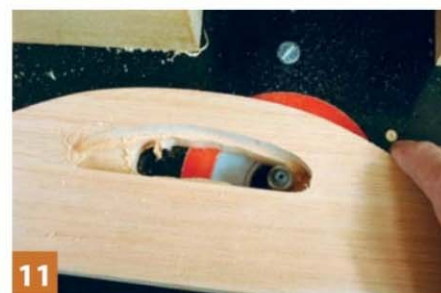
11 'Grouse', my term for width-wise removal layer by layer, allows you to sculpt out the waste ready for a final run around the template
