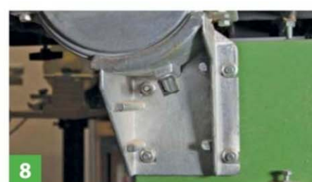
8 The tilt mechanism for table adjustment which allows it to be positioned to enable bevel cuts.
