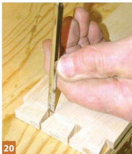
Trimming the dovetails after bandsawing the majority of the waste out
