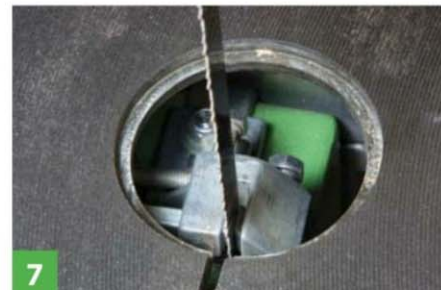
7 The lower guides may be blocks or bearings
