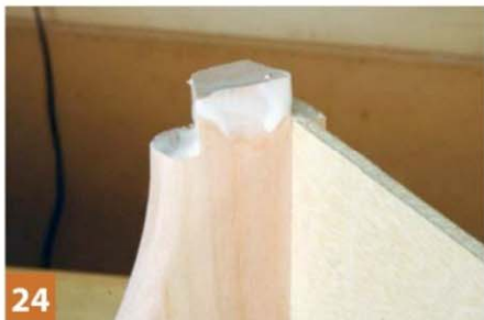
24 Aliphatic resin glue gives a good quick bond
