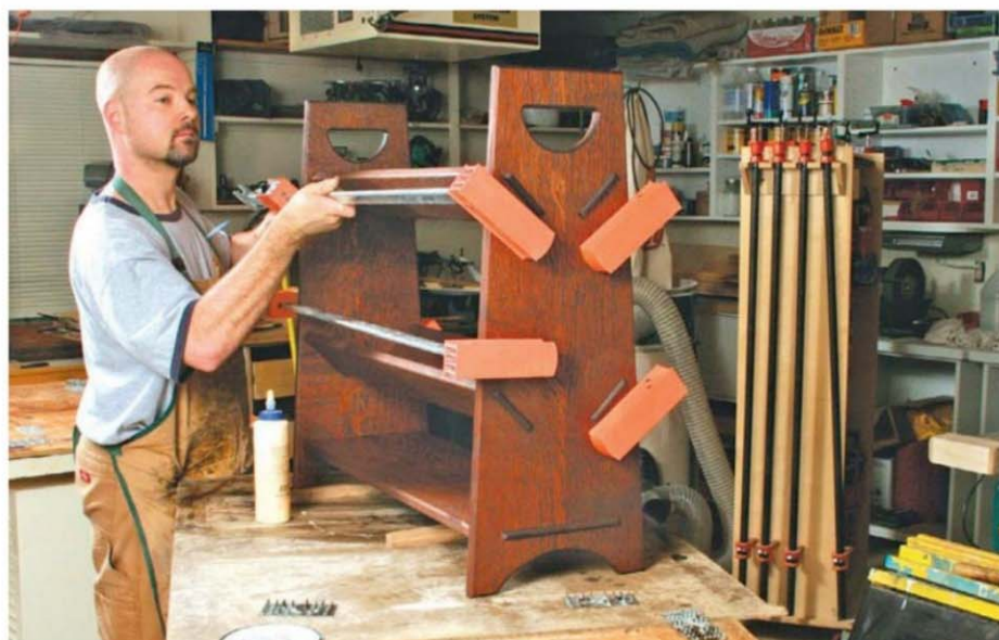
Glue, then shellac. To reduce squeeze-out, put most of the glue on the tenons and only a dab in the mortises. When the glue has cured, apply several coats of thinned shellac. As a final step, rub out the finish
