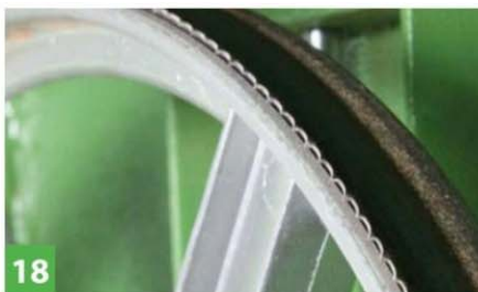
18 This 15mm wide blade is tracked towards the front of the wheel
