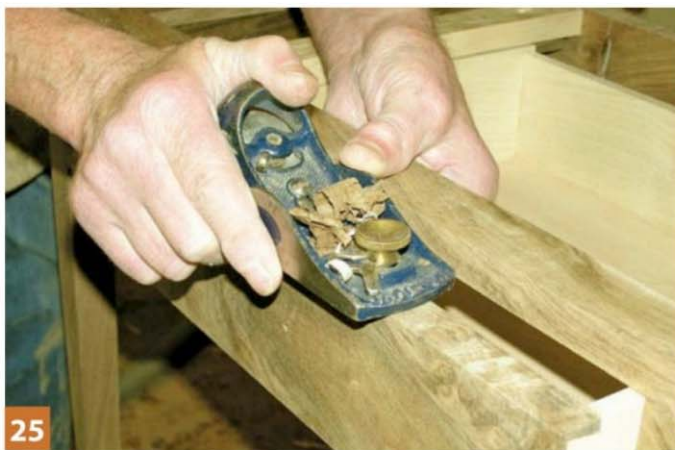
25 Trimming the drawer fronts to fit with a block plane
