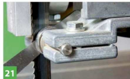
21 The guides should be about 0.1mm from the blade
