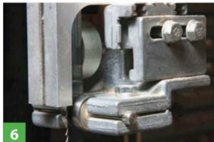
6 Quality machines will be fitted with bearings for the upper guide system
