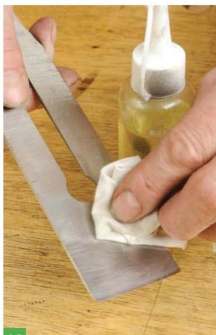
10 A light coating of oil on all bare metal tool parts is important
