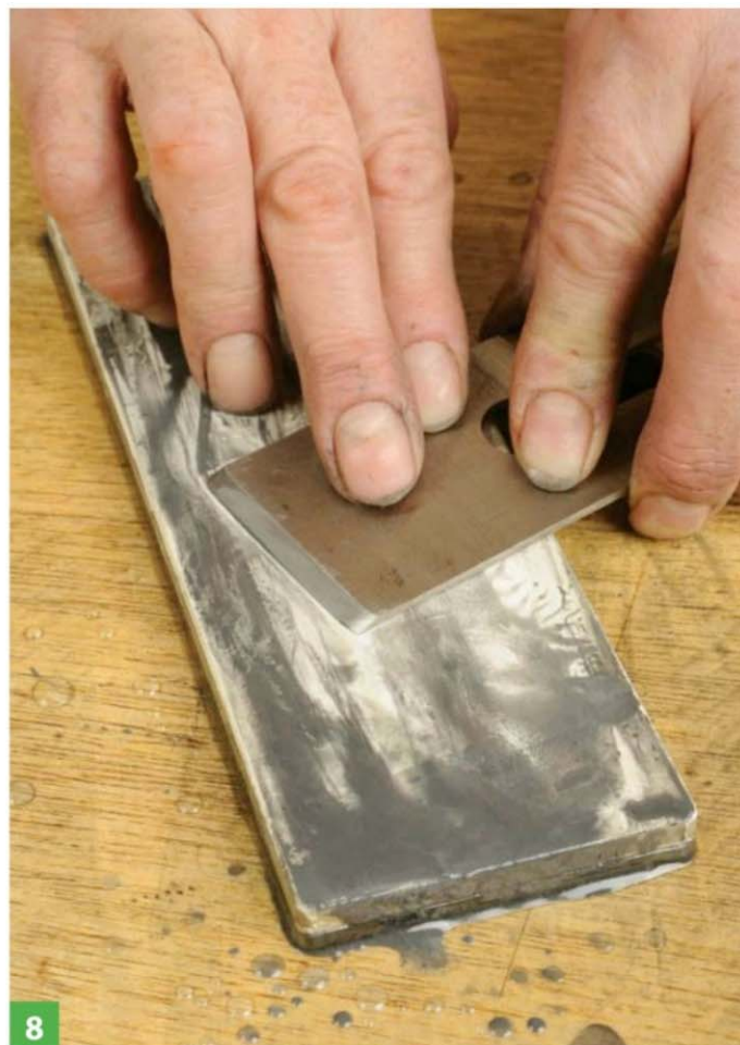
8 The same procedure for the back as before; you should now have a very sharp cutting edge. Note this blade has had its corners rounded for a No.4 smoother
