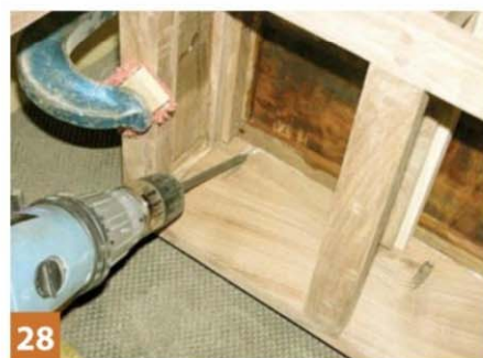
28 Driving screws into pockets in the back to fix the top to the frame
