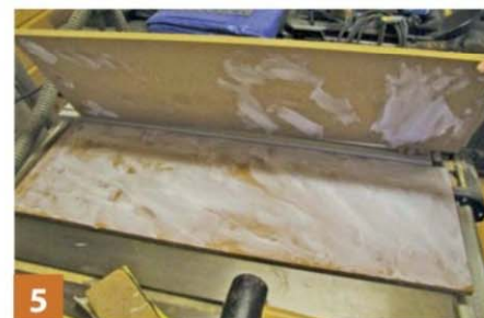
5 For adequate thickness you will need two 12mm MDF boards bonded together
