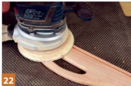
22 Use a fine abrasive to avoid obvious scratches
