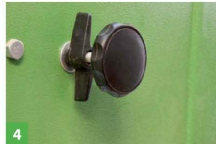
4 Tracking is adjusted by a knob that alters the tilt of the top wheel
