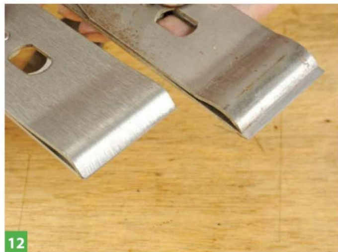
The blade edge is barely visible on the left while the extreme opposite shown at the right. Some early blades are very thin and need to be set forward partly to prevent shavings jamming under the cap iron
