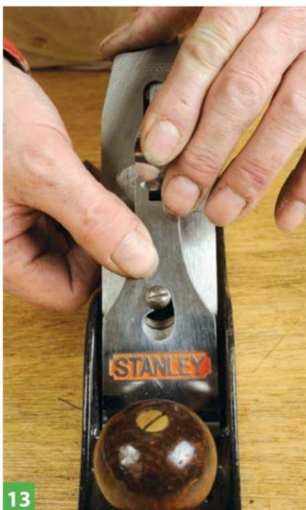
Make sure the blade assembly is seated on the adjustment peg and sitting vertically
