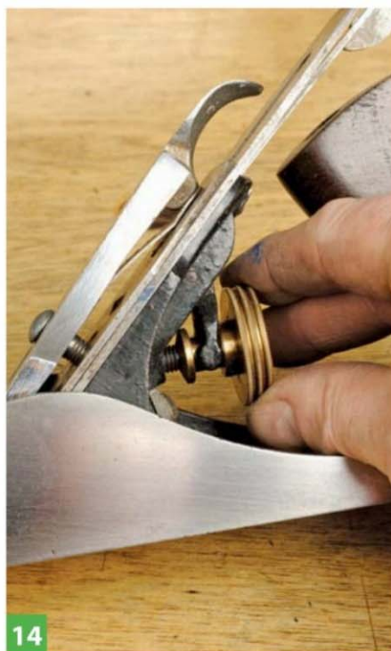
Antique planes often have a small knob which is hard to turn unlike this more modern example
