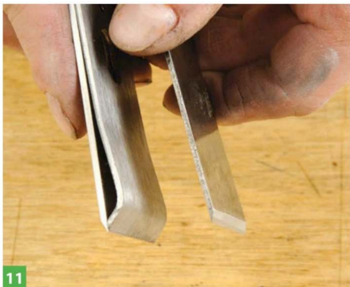
A bench plane blade and cap iron on the left, block plane blade on the right
