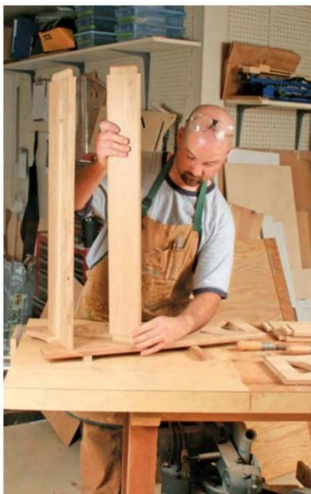
Fine-tune the fit. The tenons should fit into the mortises with hand pressure. At the end, you may need to remove a small amount of excess with a coarse file or alternatively a shoulder plane
