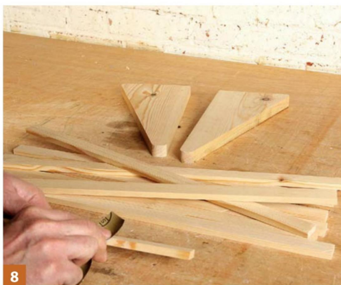
Soften the edges of the shelf slats with abrasive paper
