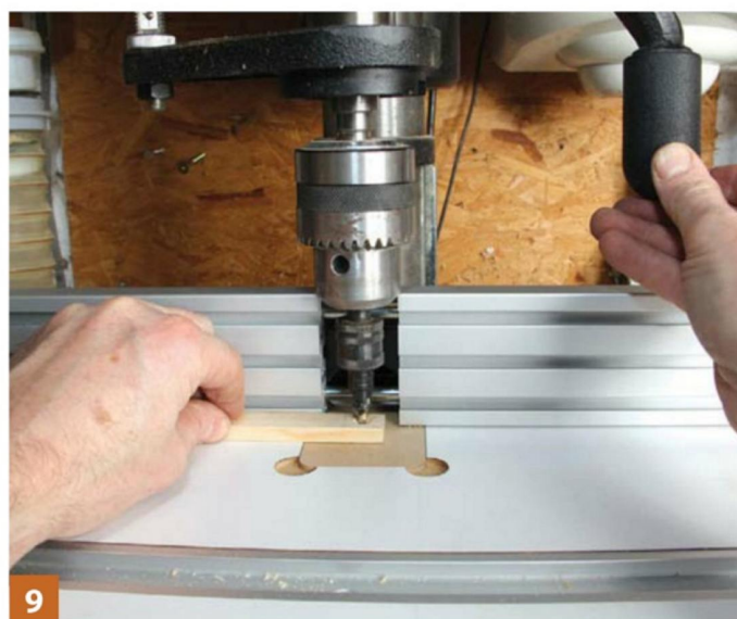
Drill and countersink the end of each slat; a pillar drill is ideal for this repetitive job
