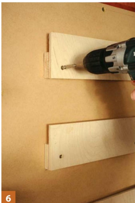
6 Next, I glued and screwed some ply upstands in place
