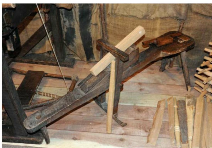
The shave horse traps the roughly split timber just by the action of sitting on it, then a drawknife is used to round it off sufficiently to mount it on the lathe. The timber is 'green' i.e. wet
