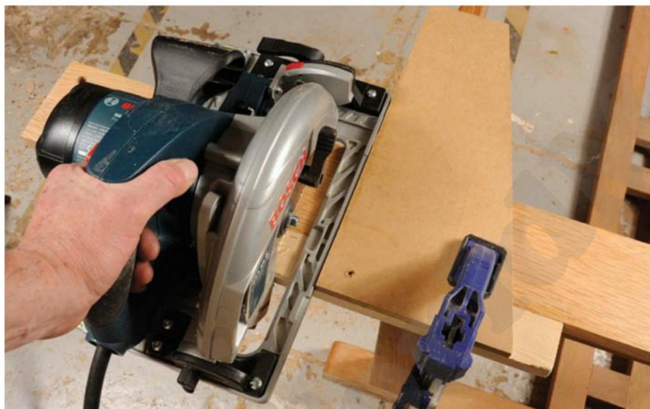
A homemade 'T' square makes cross cuts easy
