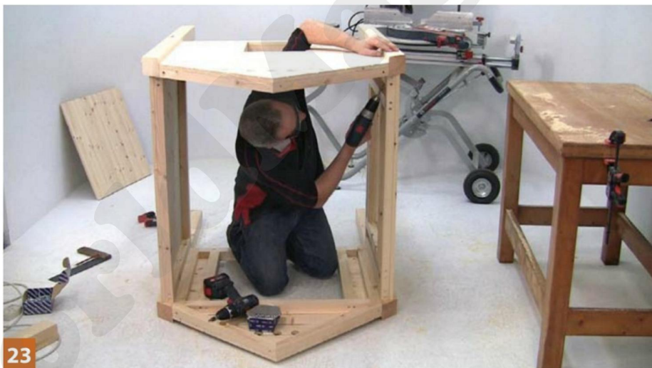
23 It is relatively easy to line everything up with the edge of the leg on the inside
