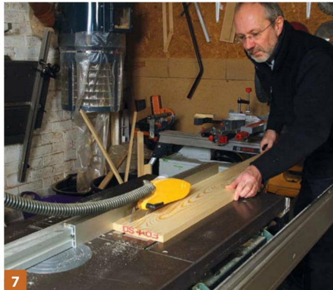
Rip two lengths for the legs and 10 narrow strips for the slats on the top shelf
