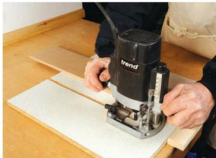
Slotting using a T-square
