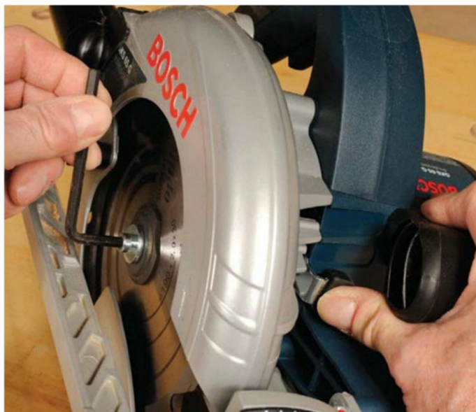
Using the spindle lock to change the blade
