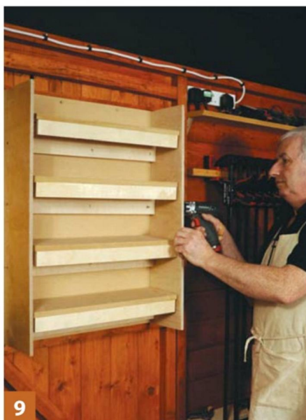
9 The sides were glued and screwed to the ends of the 'L' pieces
