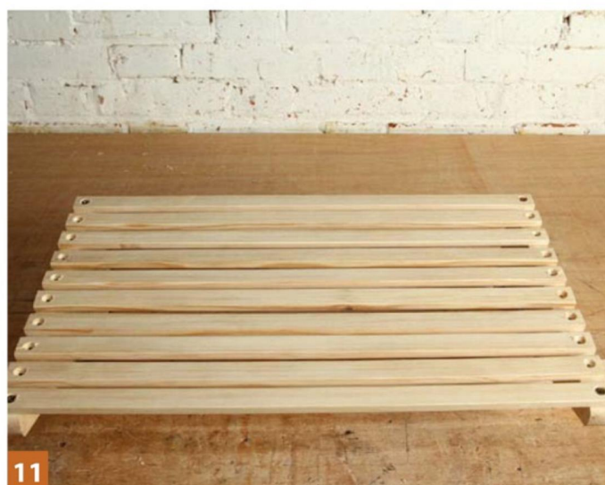
Arrange the other slats evenly across the middle, you can do this by eye, or, if you are really meticulous, make a spacer to equalise all the gaps
