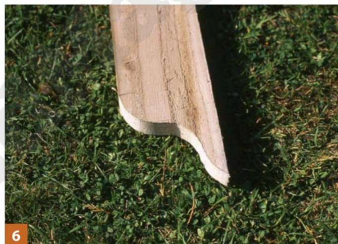
The detail was cut out with a jigsaw
