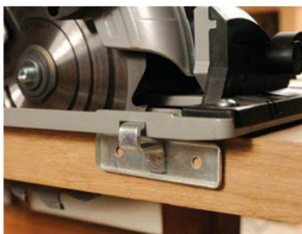
Always use a fence or guide rail
