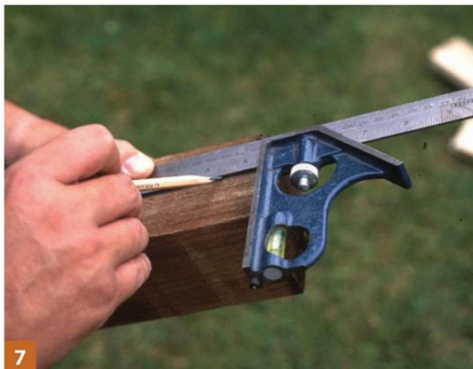
Creating a flat face to take the beam
