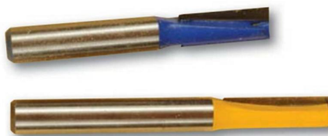
Use a longer shank cutter in a table
