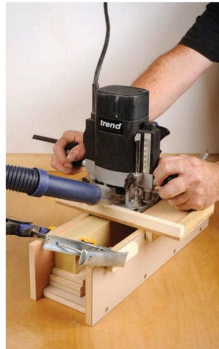
A mortise box makes joints easy to do
