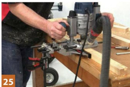
25 Rout an 18mm groove in the other piece of framing
