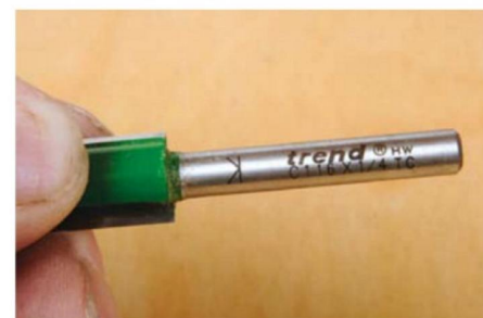
Safe working shank depth mark
