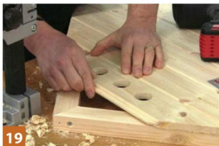
19 Using the router, trim back both the external and internal overhangs
