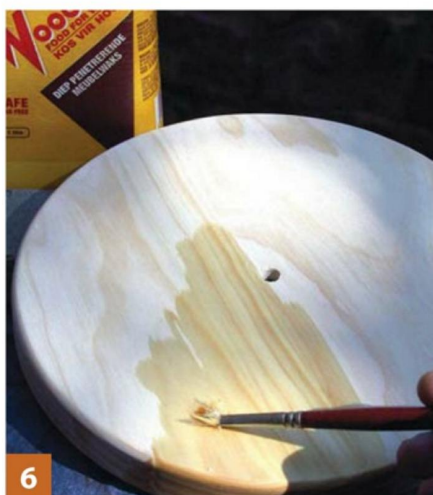
6 Use a small paintbrush to apply deep-penetrating furniture wax liquid or Danish oil to the backing piece
