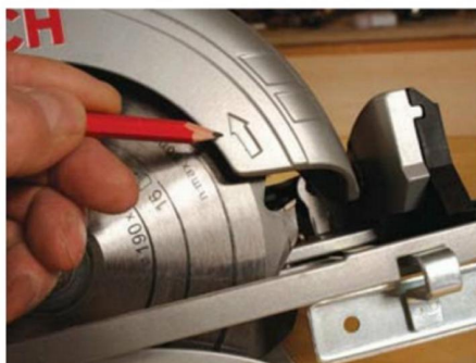
The arrow indicates tooth and cut direction
