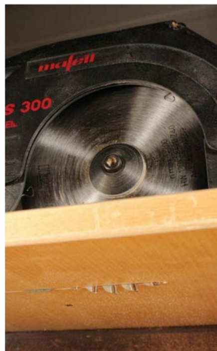
The teeth should just project when cutting faced board
