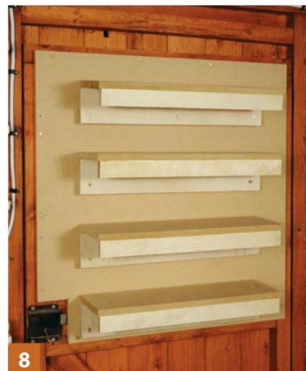
8 The cutter racks simply drop into the 'L' shapes and stay there
