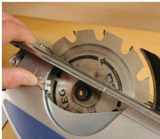
The riving knife is correctly set
