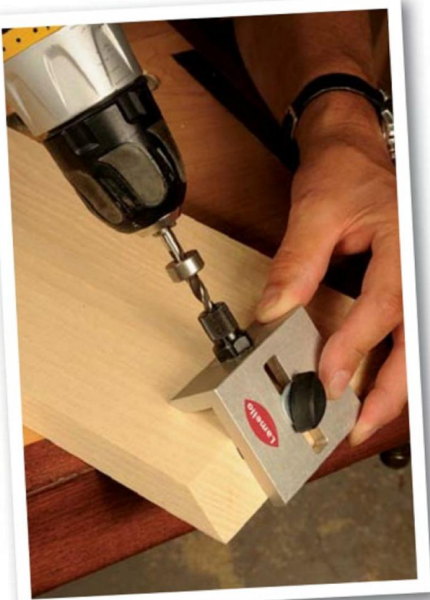
Lamello supply a drilling jig to make location of the 6mm hole precise
