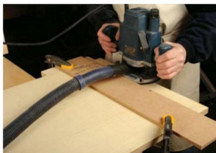
If the cut is too rough then clean up with a router afterwards
