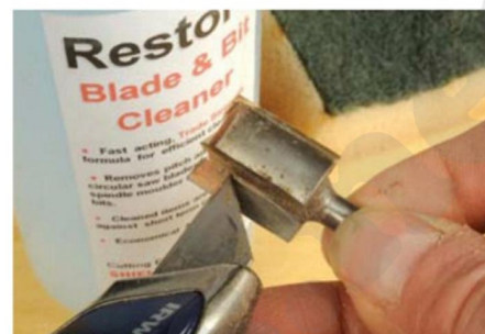
Scraping deposits off a cutter
