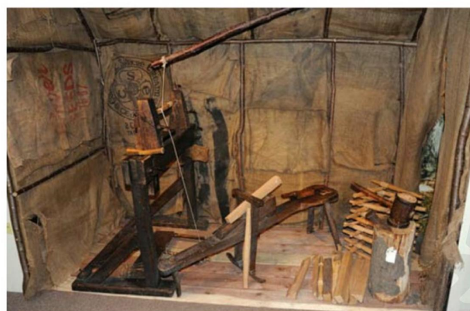
A reconstruction of a sack-lined hovel in the Wycombe Museum showing the pole lathe and shave horse – used to roughly shape the legs before turning – a large timber filled mallet, an iron wedge and a stack of finished components. Bodgers lived in 'hovels' or huts in the Chiltern hillside
