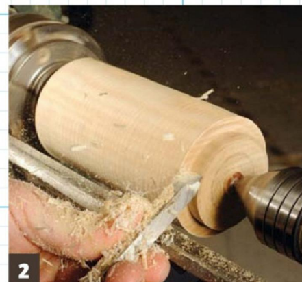
2 The beading parting tool cutting your spigot, here with a bevel-rubbing cut
