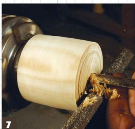
7 Making the drilling cut with the spindle gouge to the box's full inside depth
