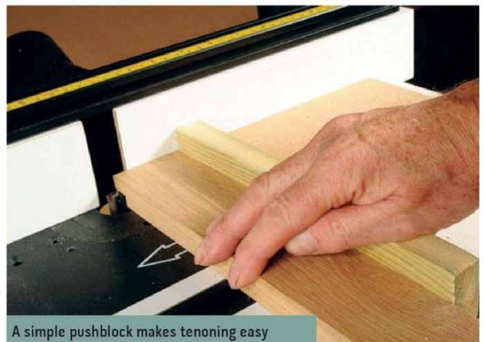
Machining the bevels on a tenon
