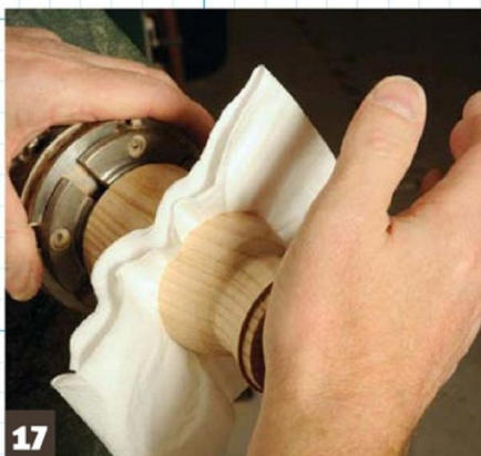
17 Jamming the lid on with kitchen paper and hand pressure
