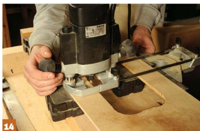
14 Straightening up the template sides with a router and fence
