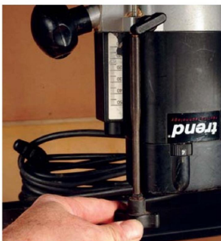
A fine height adjuster is essential for table working
