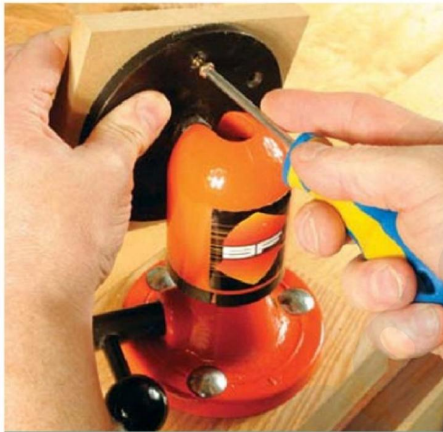
Waste wood blocks give more fixing options for tricky pieces of work
