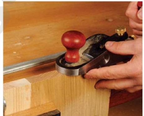
End grain is not a problem. Just protect the front edge
