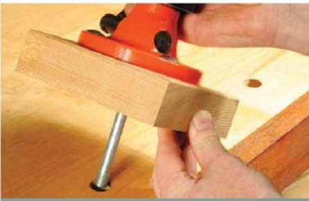
A standard long-reach bolt can help with fixing the clamp in place
