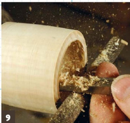
9 The French curve scraper finishing off the bowl interior to full width and depth
