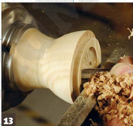
13 ... before hollowing out the lid, as with the body, but leaving a 3mm thick lip
