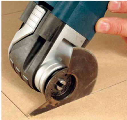
The disk blades make it easy to plunge cut and follow a straight line freehand
