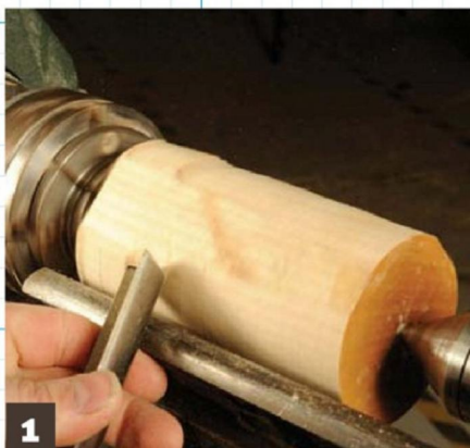
1 Turn your blank to a cylinder with the spindle roughing gouge
