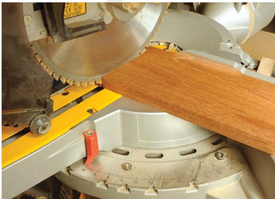
The chop saw is the easiest way to cut the stretcher ends to an angle of 10°
