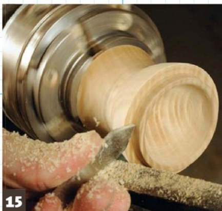
15 The 3mm parting tool being used to slightly undercut the lid edge
