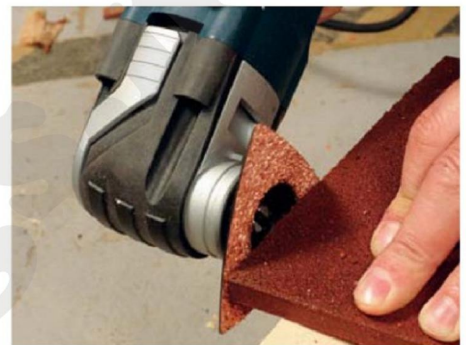
With the right tool ceramics can be trimmed with your multi-tool
