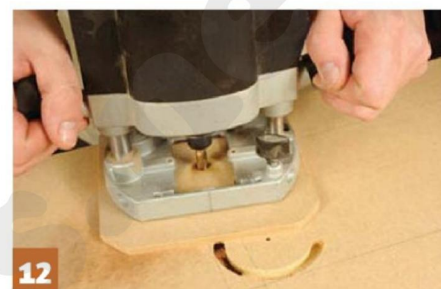
12 Locate the jig pin in this hole. Plunge your router in, then rout out the curve
