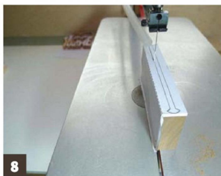
8 When cutting the stem, cut through the tall, thin side first
