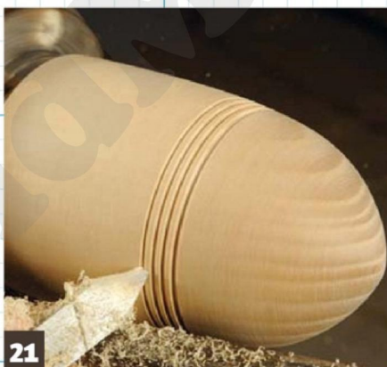
21 The 3mm parting tool is used to cut the bead curves with a scraping cut
