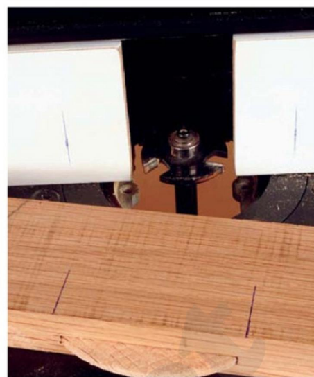
Slotting is easy after fence marks are made
