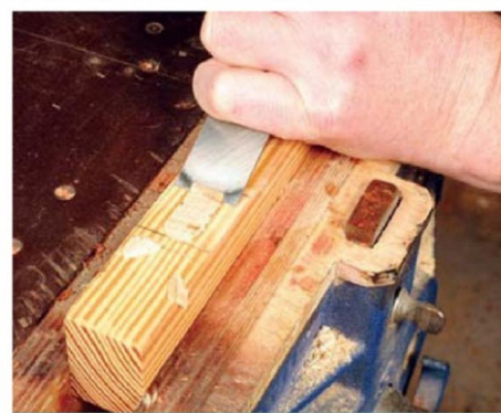
Cut in from both ends when paring off work
