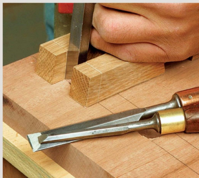
...and a 19mm chisel to clean up the walls
