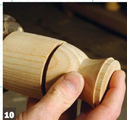
10 Make a test fit of the box lid, to ensure it is a nice fit, but not too tight
