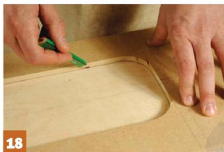
18 Mark the opening on your birch ply using the template as a guide
