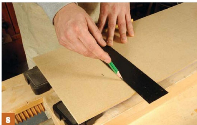
8 Mark up a piece of 6mm MDF which will be your router template
