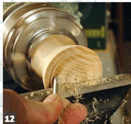
12 Cleaning up the front face of the lid with the spindle gouge...
