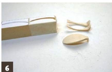
6 Back up the blade and cut along the other side. Slide the petal out from the block
