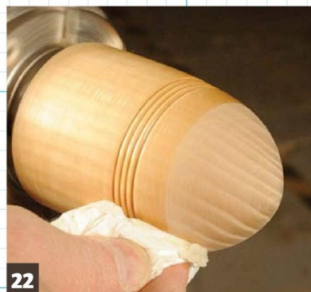
22 Applying the first coat of finishing oil with kitchen paper
