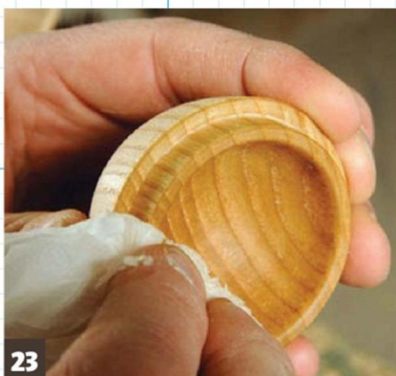
23 After removing the lid, apply oil to the inside, and the body inside too
