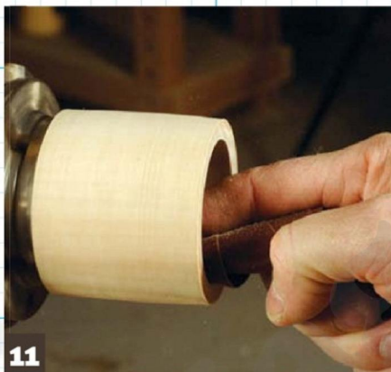
11 Sand the interior through the grits, in the lower left quadrant of the bowl
