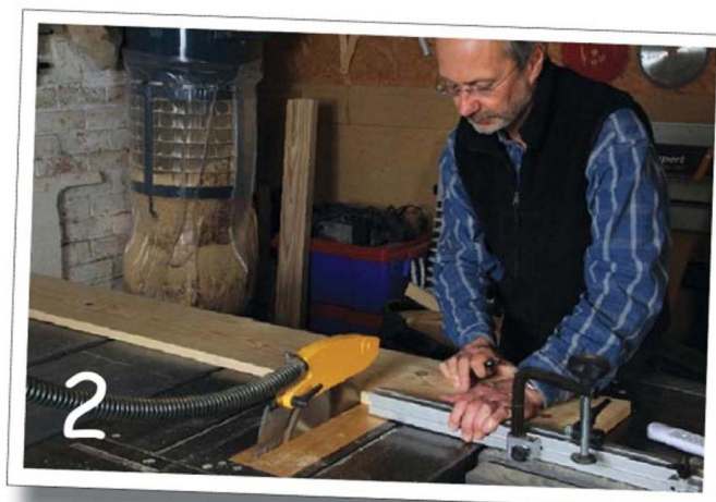
2 Crosscut the components to length
