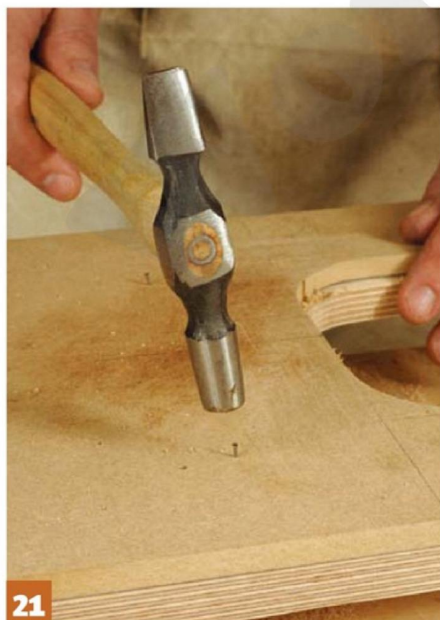
21 Tack the template in place, ready to use the router to finish off the opening
