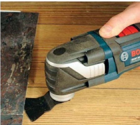
An oscillating knife tool can help lift material that's been stuck down
