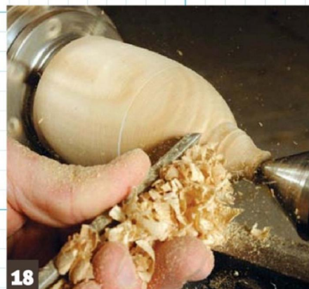
18 Shaping the lid and body with the spindle roughing gouge...
