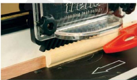
When using a support strip, ensure pressure is applied to the workpiece side
