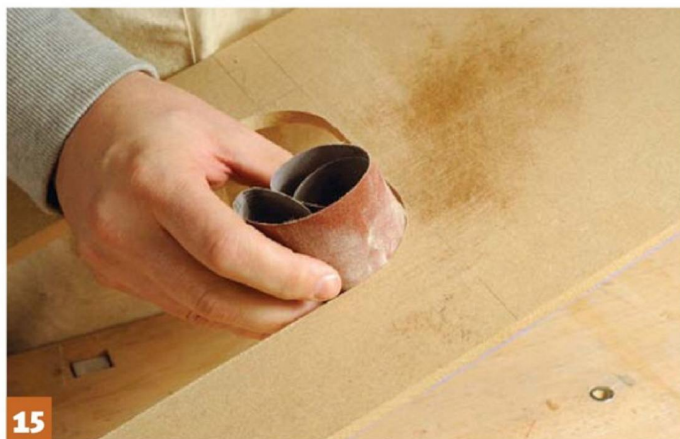
15 Clean up the inside faces of your template with abrasive
