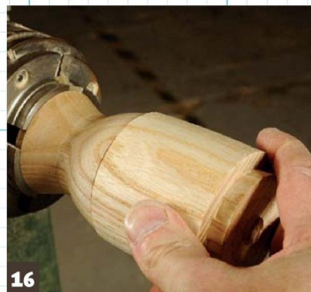
16 A test fit ensures the edges meet with no gaps
