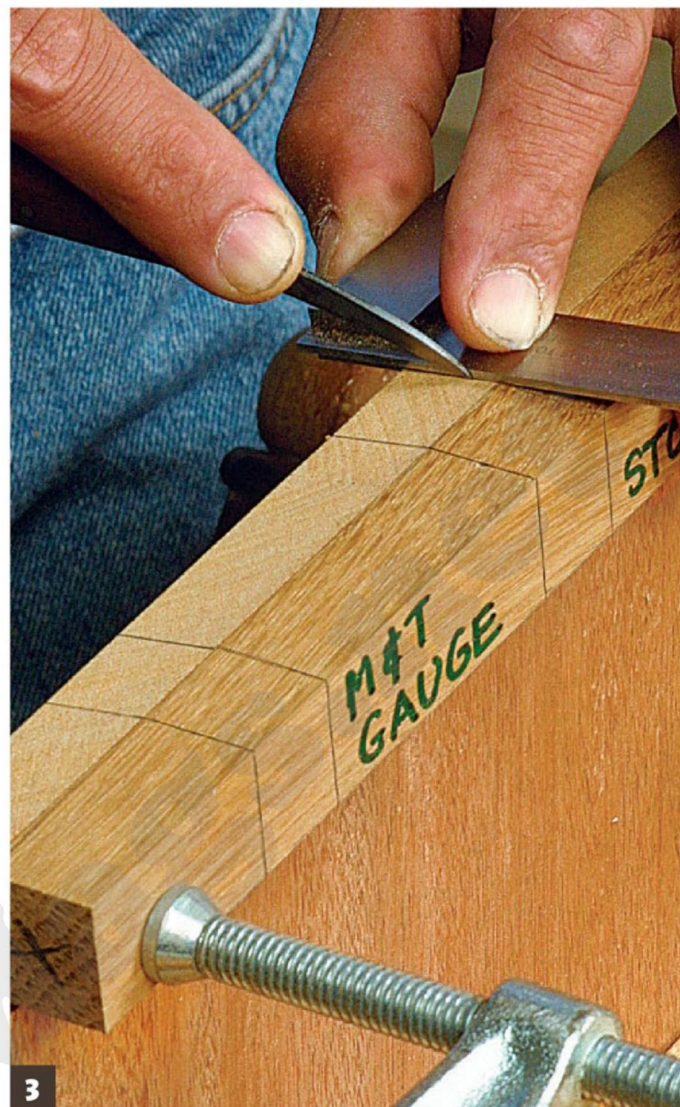
3 Use the same layout gauge for the tenons. There is no room for error here, and the layout gauge will ensure that the tenons match the mortises
