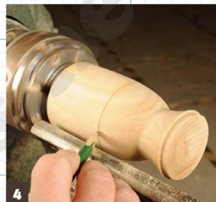
4 Marking the lid onto the blank with a pencil
