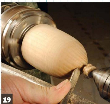
19 ... before refining the shape with the spindle gouge
