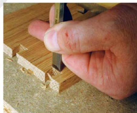
Sacrificial boards can save damaging your workbench
