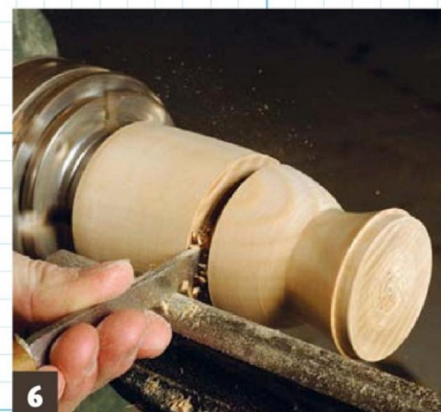
6 Removing the lid with the 3mm parting tool
