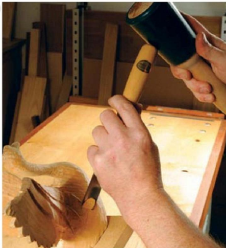
Make sure your clamp is substantial enough to be used with heavy-duty shaping cuts
