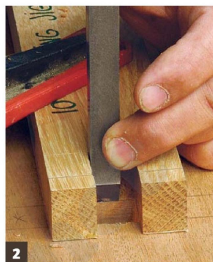
...a 12mm mortising chisel to rough out the rest
