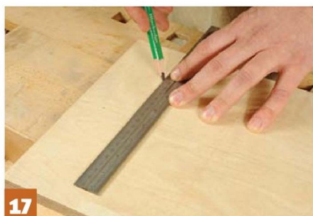
17 Also mark a centre line and the top of each opening on to the birch ply
