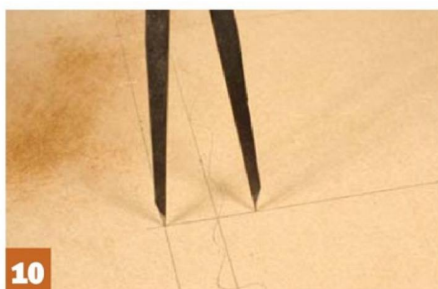
10 And use this to find the centre of the radii for your template curves
