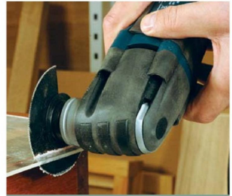
Cut Perspex with your multi-tool
