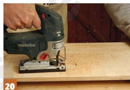
20 And then jigsaw out the opening, leaving a few millimetres of waste inside the line
