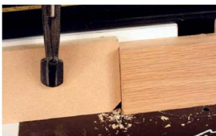
You can use a stop block on the in-feed or out-feed fences or both
