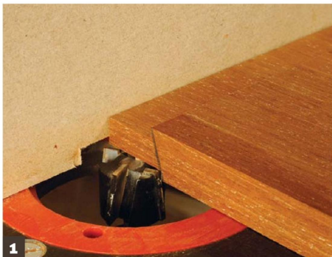
1 Cut the cheeks of the tenons with a router and tenoning cutter, using your router table and a sub fence. Note the different shoulder heights on each side
