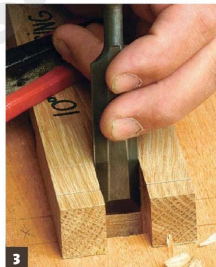
...and a 19mm chisel to clean up the walls
