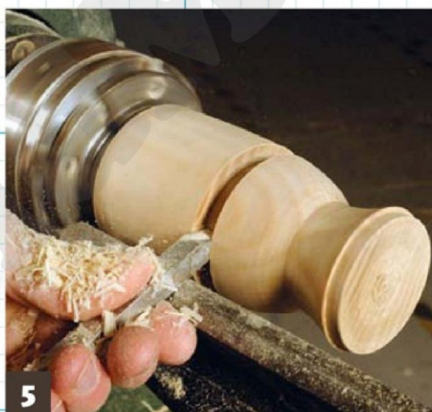
5 Forming the lid bottom with the beading/parting tool
