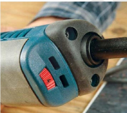
A machine with variable speed opens up the range of tools you can use with your multi-tool
