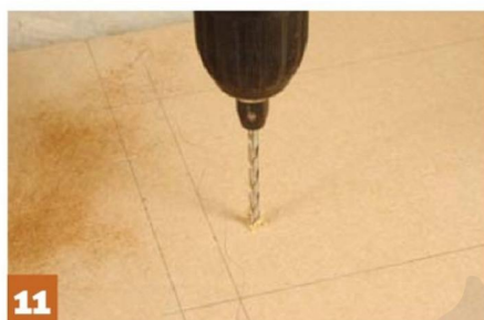
11 Drill a hole to take the in-board trammel jig pin
