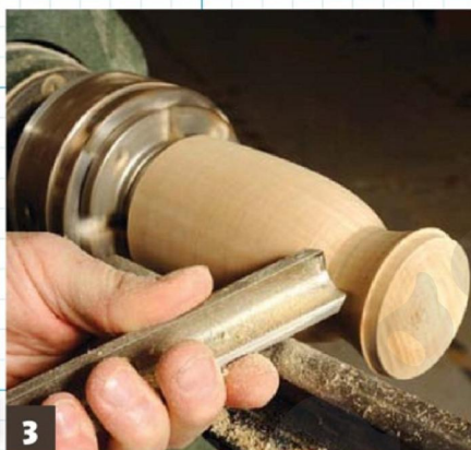
3 Shape as much of the box lid as possible with the spindle roughing gouge
