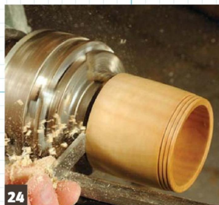
24 Then simply part off, undercutting slightly to let the box stand securely
