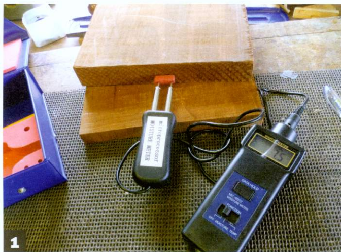
1 Make sure your timber is at the right moisture content
