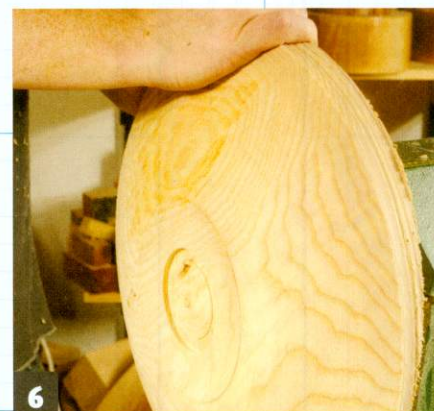
6 Remount the blank on the lathe with the scroll chuck, using the recess cut earlier
