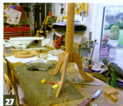
27 The dovetails needed trimming, to create a nice neat joint
