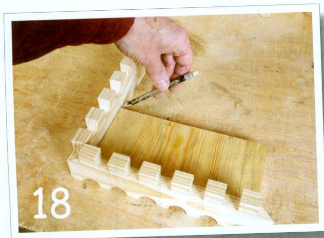
18 Arrange the parts around the top panel and mark the length
