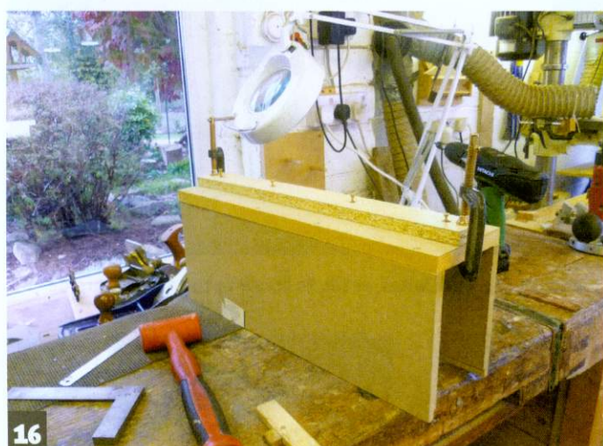
16 A further batten was screwed to the base, to locate in the lathe
