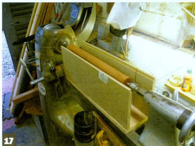
17 Here the jig and blank are in position, ready for routing
