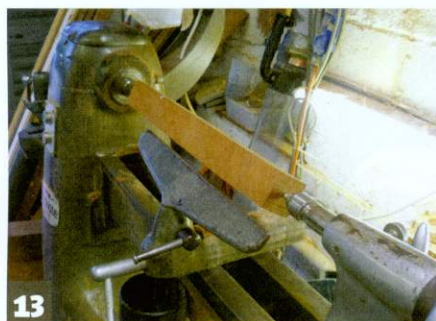
13 The 50mm square blank was mounted between centres
