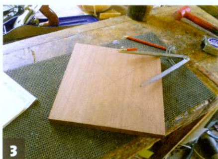
3 Find the centre of your top, and mark the diameter with a compass
