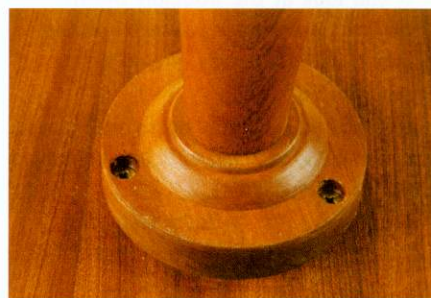
Here's a detail shot of the stem brace on the underside of the table top
