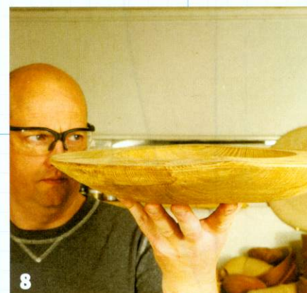
8 A blank left to dry for a year or two has warped an incredible amount
