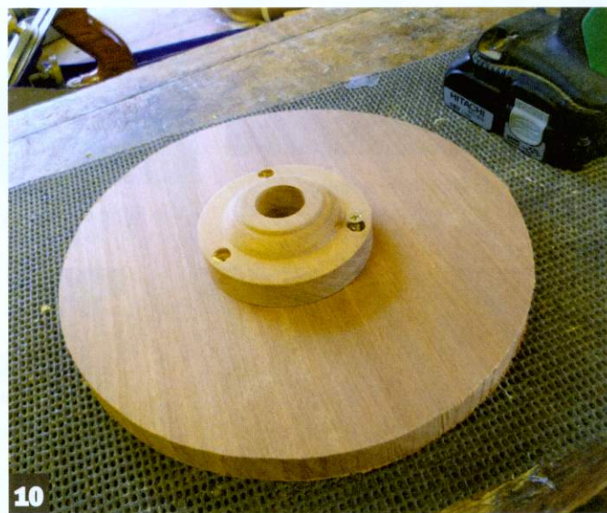
... and countersink holes, ready to screw to the top underside
