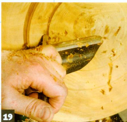
19 When happy with the rim, hollow out the platter with the bowl gouge
