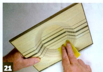
21 Sand the rim and inner walls once dry
