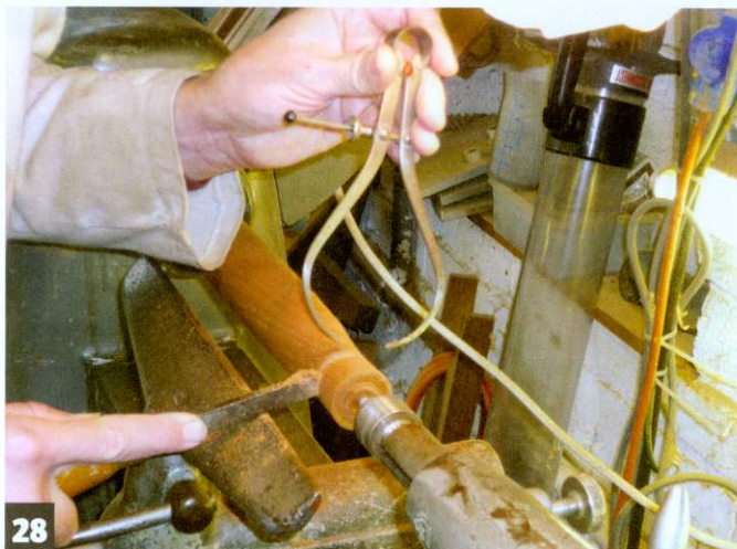
28 I remounted the stem and turned the top tenon, and stem shape
