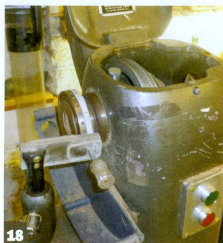
18 Andy's lathe has an indexing feature, perfect for this job
