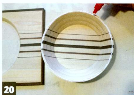
20 Glue the bowl section's top edge to the top piece, clamp and allow to dry
