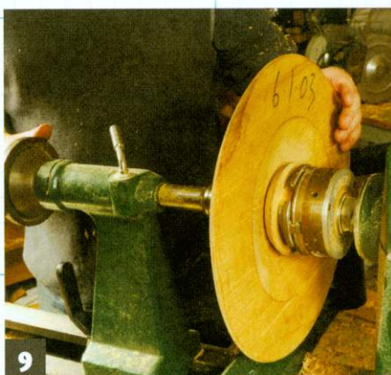
9 Mount the blank between centres with a friction drive in the scroll chuck
