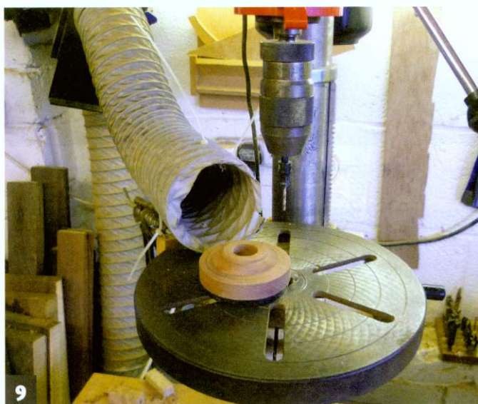
9 After turning the cove on the brace, drill your screw pilot...
