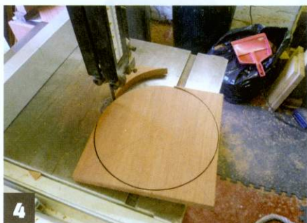
4 The top is rough cut on the bandsaw, just over the final diameter
