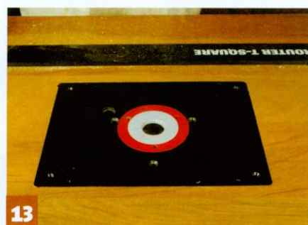
13 Here, you can see the insert fits neatly in to the router table
