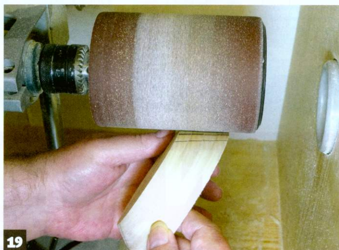
19 Align and glue the sides to the base, then sand once dry
