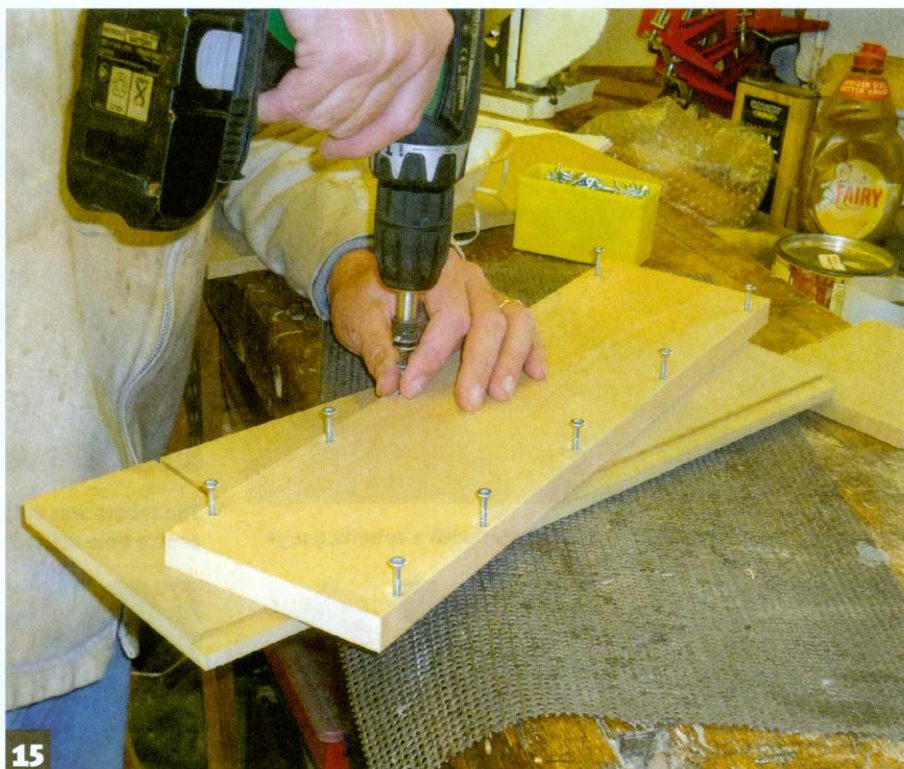
15 The jig to cut the dovetails is 'U'-shaped, with the bottom and sides screwed together
