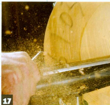
17 After remounting the blank, round up the outside edge...
