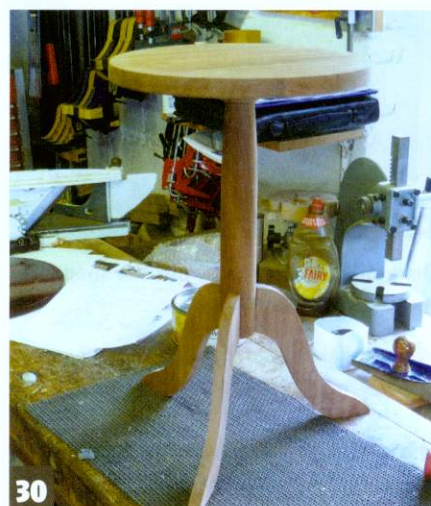
30 And there's the table put together before finishing, and before the stem cap's fitted
