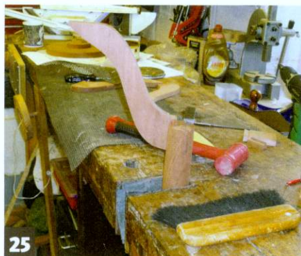
25 I fitted the legs one at a time, with a little gentle persuasion
