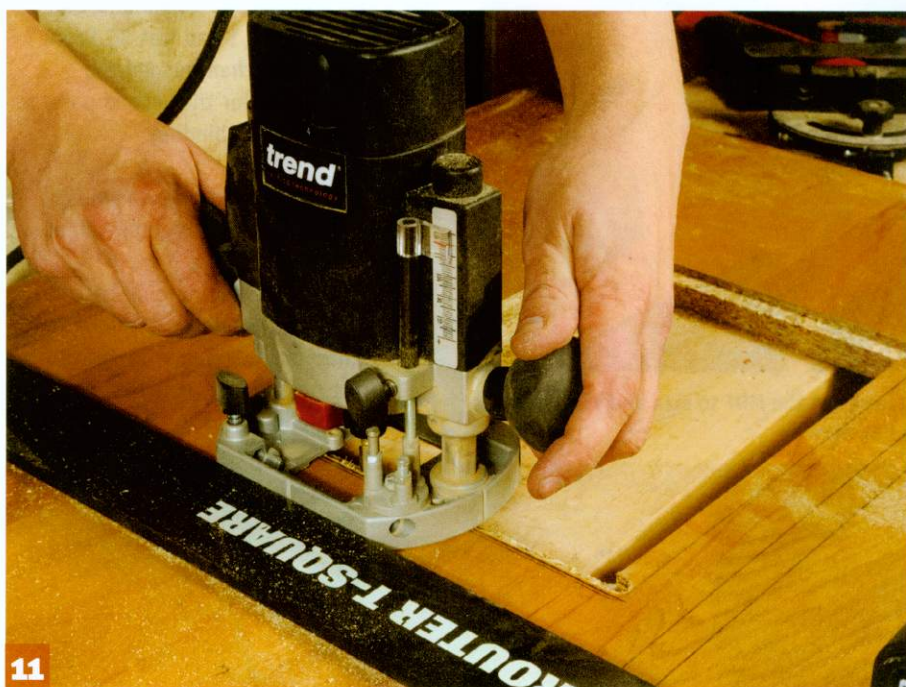
11 Now, rout out the insert recess around the opening, being careful to get the depth exact
