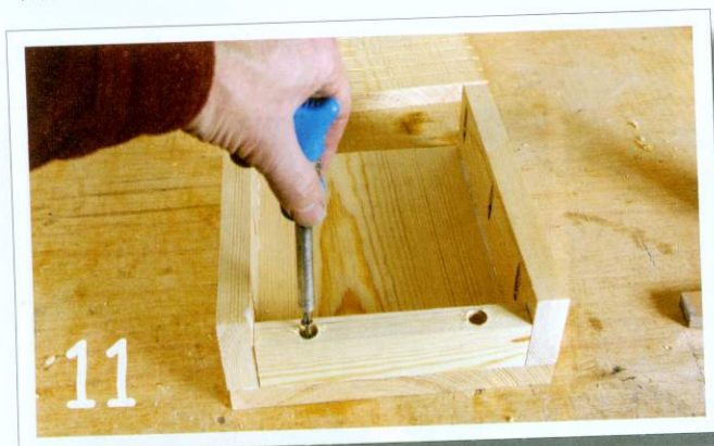
Screw the bottom board in place. It must be 20mm narrower than the sides to allow a small space for the bats to squeeze through
