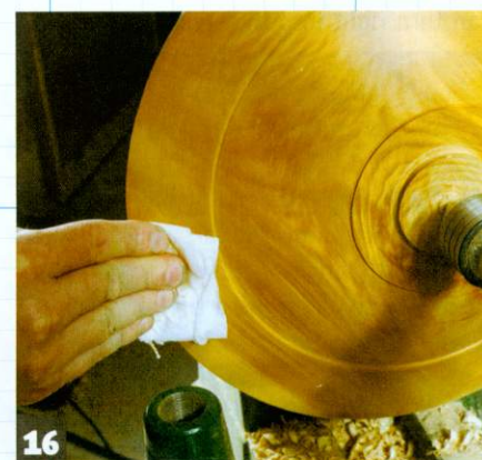
16 After sanding apply a few coats of finishing oil, burnishing the last coat
