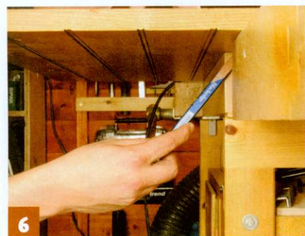
Mark the position for the batten under the table, which will be held by the tail vice
