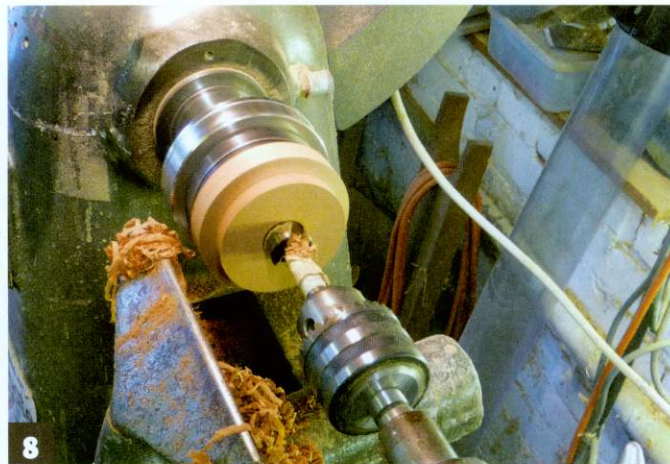
The rebate was cut with the beading/parting tool, before the centre hole drilled with a Forstner bit and chuck in the tailstock
