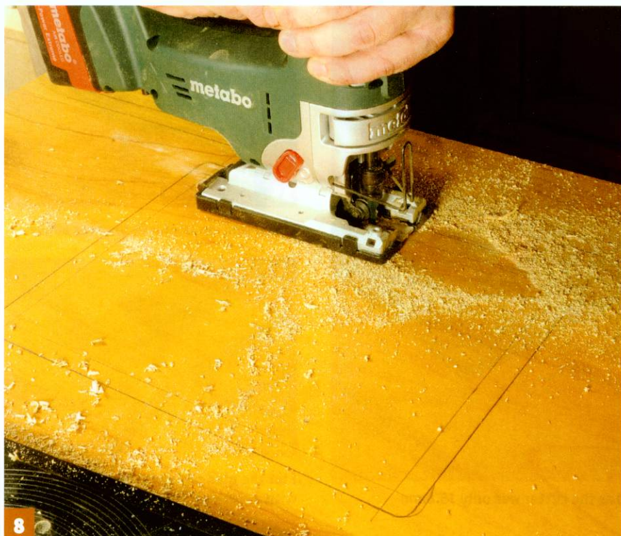
8 Then cut inside the inside face of the insert rebate using your jigsaw
