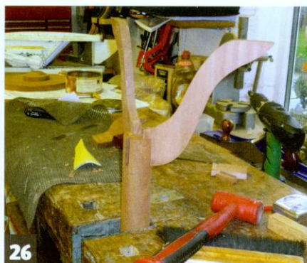
26 Note, how the dovetails pins are longer than the sockets in the stem
