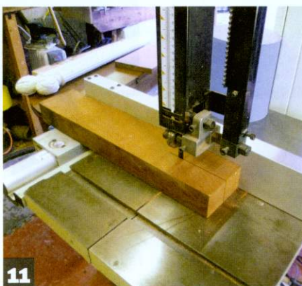
11 A 50mm square blank is prepared for turning
