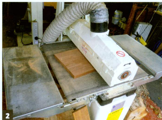
2 Thickness your table top, with a planer, sander, or by hand
