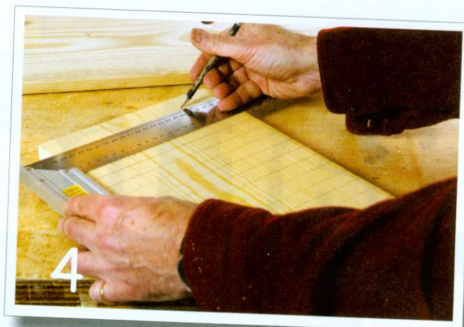
The backboard needs to have grooves cut into it so that the bats will have something to grip on to. Mark out a series of lines with a try square, about 20mm apart
