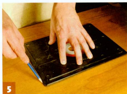
Draw round the insert ready for cutting the recess in the table
