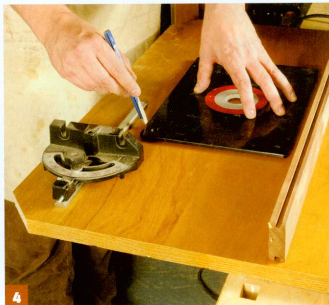
Clamp the table to the bench to lay out the router table components
