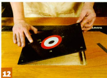
12 Getting the width correct can be difficult, so do a test fitting as you go
