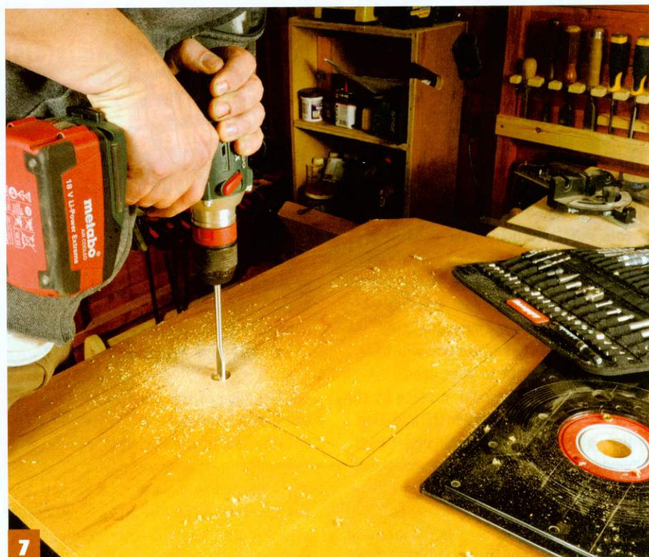
After marking the insert, drill a hole in one corner, with which to start your jigsaw cut
