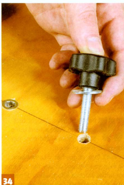
The fence adjusting knob goes through the top to hold the router table securely
