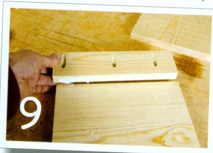
Use exterior grade waterproof glue to fix the sides
