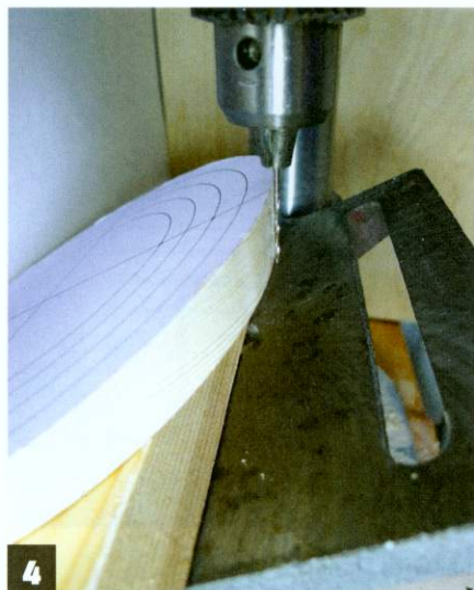
4 Check the bit runs true down the bowl
