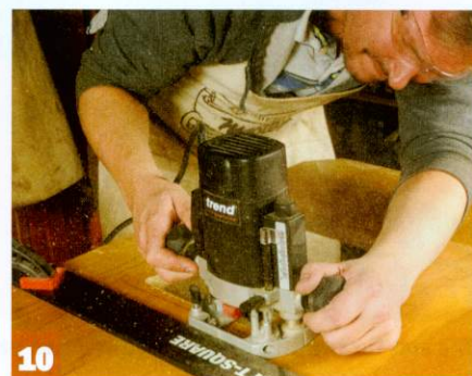
10 Be careful when getting near the corners, as the router can bite
