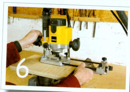
When routing the grooves, be sure to hold the side fence tight against the edge of the board to keep the grooves straight. The board is supported here on a vacuum clamp
