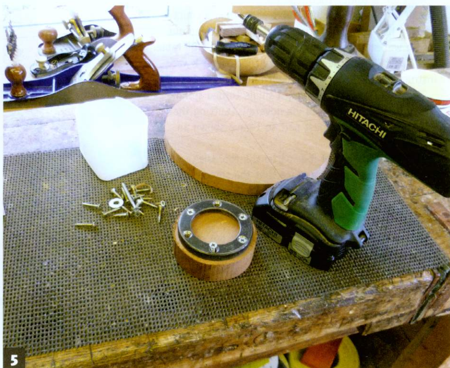
5 A blank for the brace is screwed to a metal ring... the screw holes will be hidden
