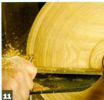
11 Next turn the shape of the underside with a bevel rubbing cut and the bowl gouge
