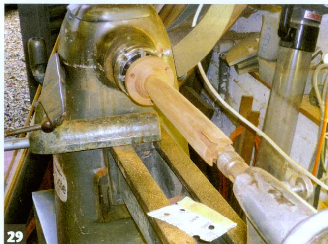
29 For sanding, I mounted the stem with a brace in the lathe
