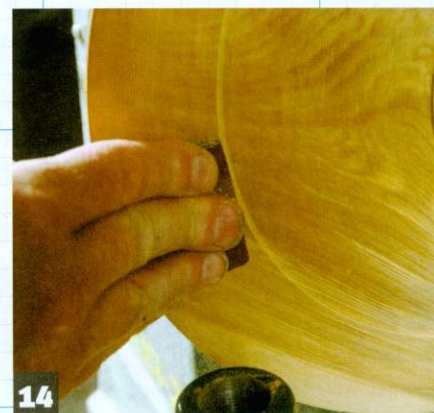
14 Hand sand through the grits when working close to your quirk and stand
