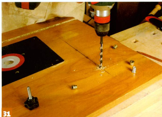
After drilling the holes, cut a countersinking hole for the inserts
