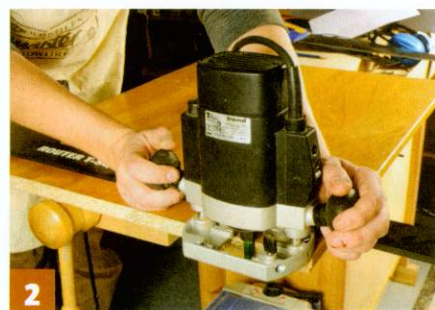
... then clean up the edge with a router, straightcutter and a straight edge
