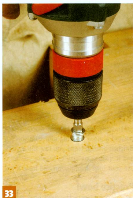
Drill your hole in the bench top, before countersinking and screwing in the insert
