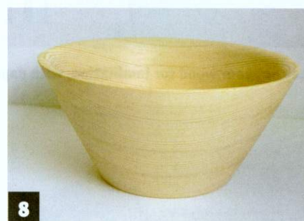
8 Then glue the bowl sides, sand the inside walls, attach the base and apply a finish
