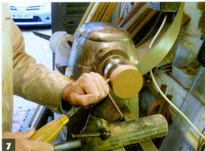
7 Cutting your blank to the correct diameter with a spindle gouge
