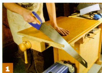
First of all, square up the edge of the table with a handsaw...
