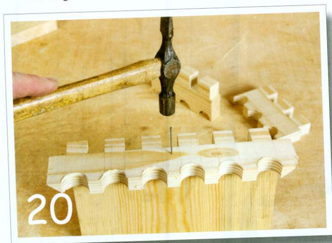
20 Glue and pin the pieces around the top panel. Set the base of the cut-outs flush with the top of the panel
