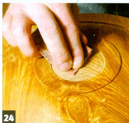
24 Clean up the recess, before cutting off the nib, sanding and oiling. Job done!
