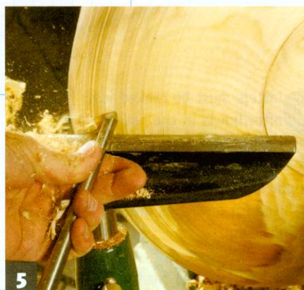
5 Then using a bevel-rubbing push cut, shape the underside of the platter
