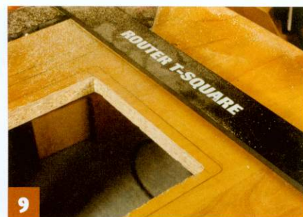
9 Tidy up your jigsaw cut with a straight cutter and straight edge
