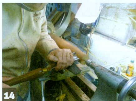
14 And roughed down with a spindle roughing gouge to a cylinder
