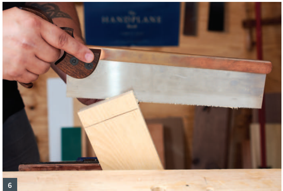
2 Go as wide as you can to make paring the mortise easier 3 Forget the numbers and determine the depth of the mortise referentially 4 & 5 This small groove will give you all the guidance you'll need 6 Start with angled cuts to ensure great cheeks
