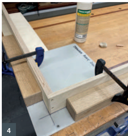
1 The case was installed in the frame using trim screws 2 The cherry boards were surfaced and then the best ones were chosen to make the drawer fronts 3 The drawers were constructed using a dowelled rabbit corner construction 4 I used a jig to ensure the drawers were square
