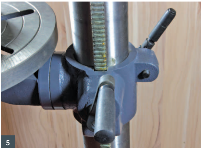
Parts of the pillar drill: 1 Motor 2 Belts and pulleys 3 Quill 4 Table 5 Rack and pinion 6 Clamping 7 Chuck
