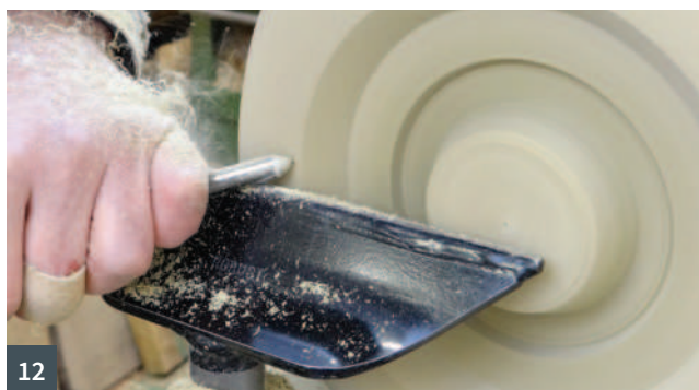
7 Reducing the thickness to suit the toy cars 8 Shaping the car's boot and rear windscreen 9 Checking progress with the template 10 Working out the detail positions on the face of the blank 11 Cutting the slope of the windscreen 12 Shaping the curve of the roof
