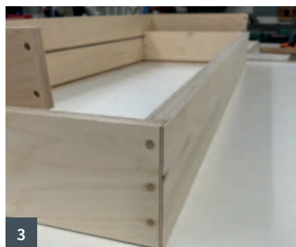
1 The case was installed in the frame using trim screws 2 The cherry boards were surfaced and then the best ones were chosen to make the drawer fronts 3 The drawers were constructed using a dowelled rabbit corner construction 4 I used a jig to ensure the drawers were square
