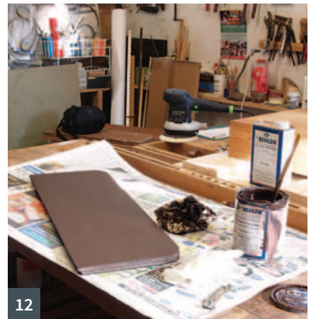
7 The Festool sander did an excellent job of removing the previous sander marks 8 Two flaps side by side. The one on the right is as it arrived; the one on the left is off the Festool 9 Picking the paint out of the rim mouldings. Note the clamp marks from Victorian needlework accessories 10 The three leaves before any colouring 11 Applying grain filler to a leaf 12 The filled leaf left to dry
