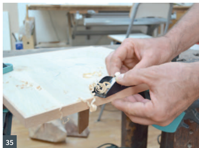
33 & 34 With the saw, I removed the two rear corners of the seat to allow for the legs 35 With the plane, I trimmed the beech edging flush with the birch of the seat
