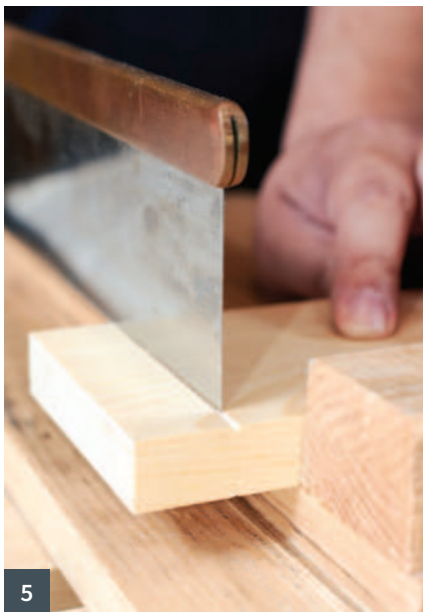
2 Go as wide as you can to make paring the mortise easier 3 Forget the numbers and determine the depth of the mortise referentially 4 & 5 This small groove will give you all the guidance you'll need 6 Start with angled cuts to ensure great cheeks
