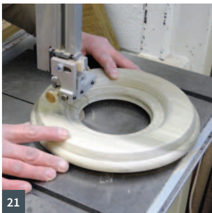
19 Once I begin to cut through, the ring easily lifts away from the hub 20 The ring looks promising 21 Cutting the car from the ring 22 It actually looks like a car! 23 Comparing the car to my sketches and templates
