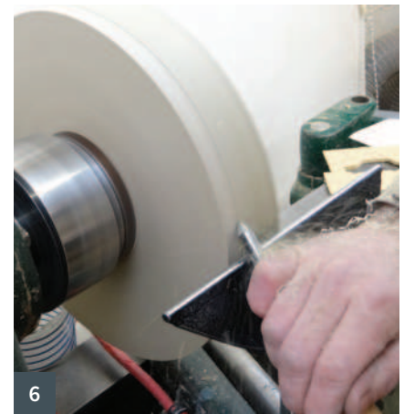
1 Making sketches of the car profile 2 The sketches were transferred onto the working templates 3 Cutting the templates on the bandsaw 4 Refining the bandsaw cuts with rasps and files 5 Reassembling the templates to check the shapes 6 Truing the edge
