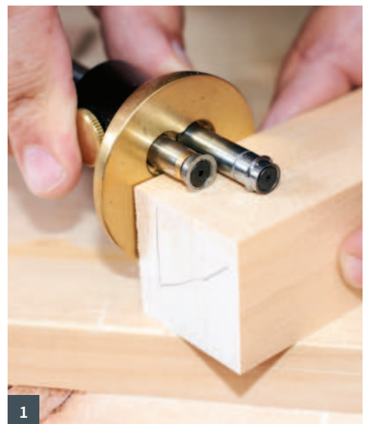
1 A marking gauge with two cutters makes easy work of marking this joint
