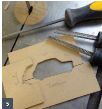
1 Making sketches of the car profile 2 The sketches were transferred onto the working templates 3 Cutting the templates on the bandsaw 4 Refining the bandsaw cuts with rasps and files 5 Reassembling the templates to check the shapes 6 Truing the edge
