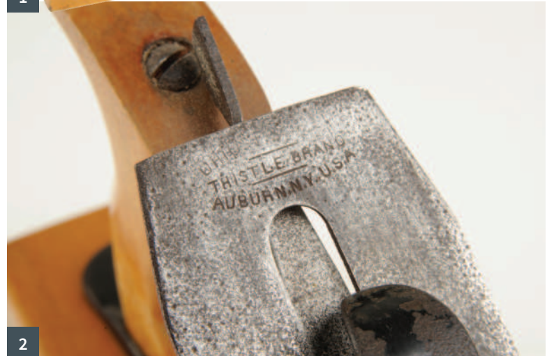
1 & 2 A strange combination of Bailey-type mechanism and wooden body 3 & 4 The tapered laminated blade and cap iron
