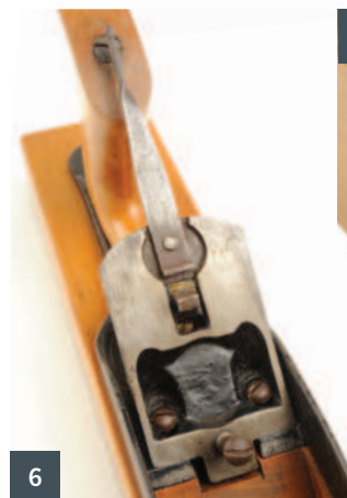
5 The manufacturer's name and serial number are clearly visible 6 Ohio Tool Company's rather basic frog design
