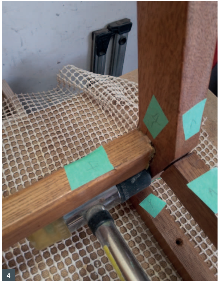
1 The top of the table was cracked 2 The top was unscrewed from the base 3 Mating parts were labelled to make reassembly easier 4 Most of this repair could be done using a mallet ...
