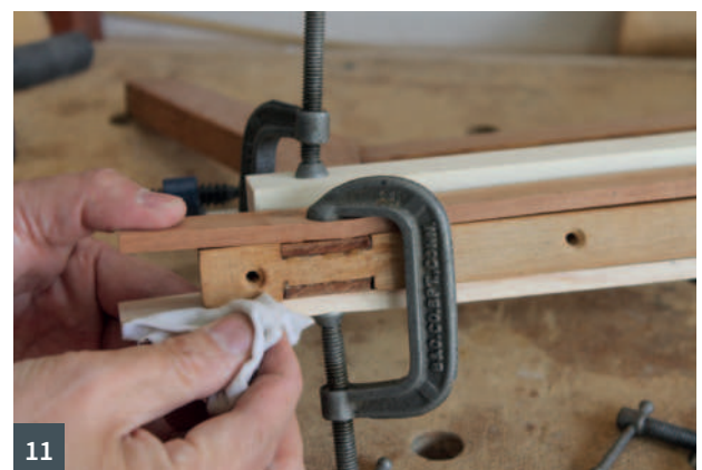
5 ...although a heat gun was needed to loosen the joints 6 The top was glued and clamped... 7 ...and the screw holes on the aprons elongated to prevent the crack from re-emerging 8 & 9 Glue was removed from the leg joints using a scraper and sharp chisel 10 A veneer was glued to the mortise wall, which was held in place with a wedge while the glue dried 11 The mating parts were glued back together
