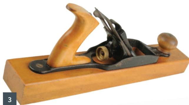
1 & 2 A strange combination of Bailey-type mechanism and wooden body 3 & 4 The tapered laminated blade and cap iron
