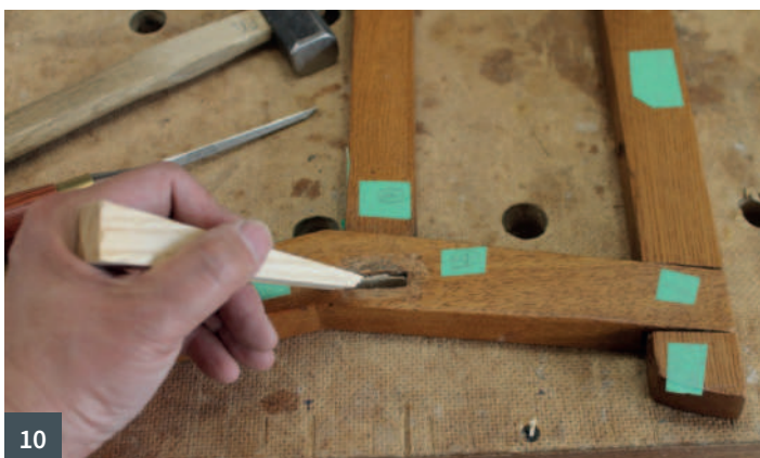
5 ...although a heat gun was needed to loosen the joints 6 The top was glued and clamped... 7 ...and the screw holes on the aprons elongated to prevent the crack from re-emerging 8 & 9 Glue was removed from the leg joints using a scraper and sharp chisel 10 A veneer was glued to the mortise wall, which was held in place with a wedge while the glue dried 11 The mating parts were glued back together
