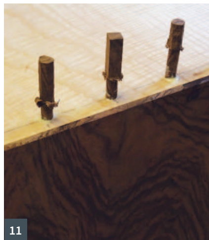
7 Walnut dowels being sized on a dowel plate over a dog hole 8 Carefully marking the pin positions 9 Lightly dampening the area to be drilled helps to avoid tear-out 10 Drilling holes as accurately as possible using a depth stop on the drill bit 11 Pegs ready to be cut off and carefully mushroomed 12 With a piece of veneer placed beneath the flush cutting saw the dowels are trimmed to 1.5mm proud of the ash top 13 Planing the plugs flush
