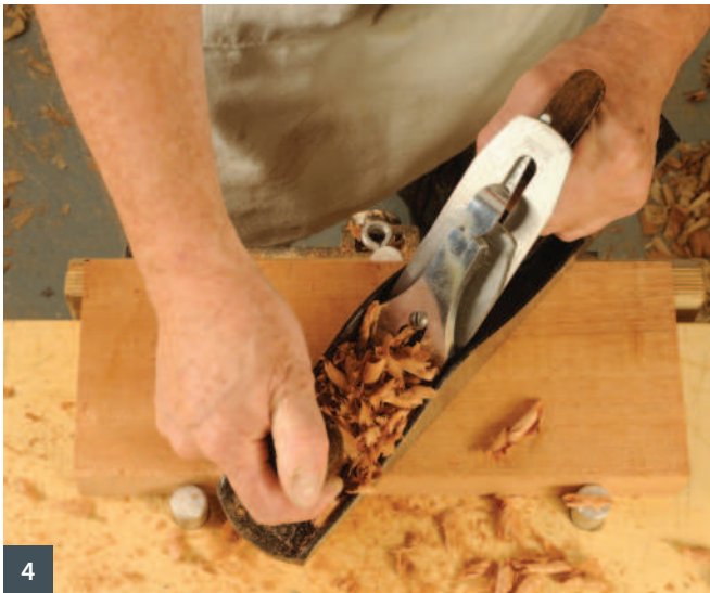
1 Just two hand planes will allow you to 'flat' wide boards 2 & 3 Skew planing is quicker but you need to finish 'on the straight' 4 The same process works well with wide boards 5 Finishing with a No.4 smoothing plane 'with the grain'
