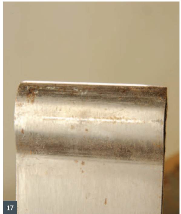
14 A cambered edge, ready to strop 15 An automotive grinding paste will polish the edge 16 The difference between straight and cambered 17 A smoothing blade with rounded ends. As you can see, the cap iron is set back slightly
