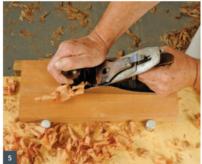
1 Just two hand planes will allow you to 'flat' wide boards 2 & 3 Skew planing is quicker but you need to finish 'on the straight' 4 The same process works well with wide boards 5 Finishing with a No.4 smoothing plane 'with the grain'
