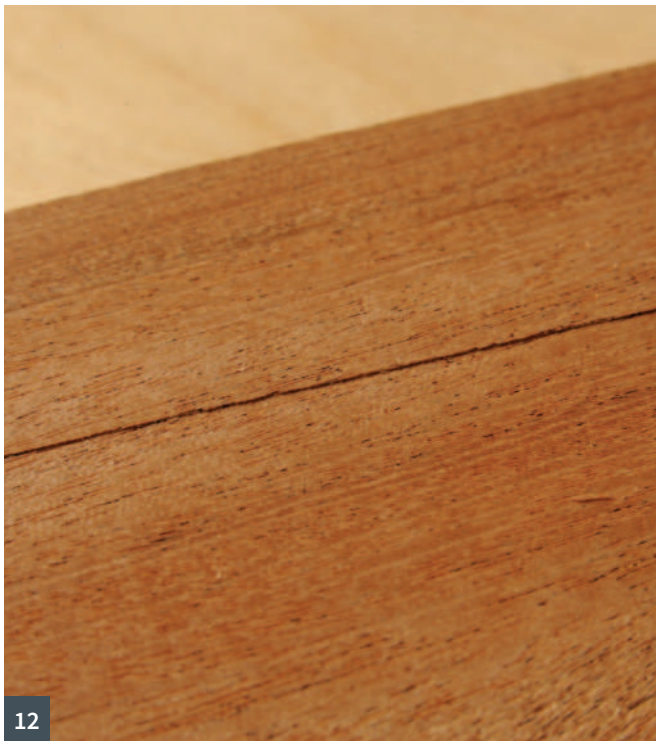
10 Grinding a camber can cause the edge to overheat 11 A secondary micro bevel is the one that performs the cuts 12 A straight-edged blade will 'dig in' 13 A straightedge is needed for trimming end grain
