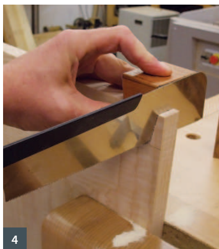
1 The two boards planed up and ready to cut to length 2 Assessing the proportions, so important with such a simple piece 3 Using white spirit to reveal the finished colours of the end and flat grain. A marked difference in colours would have ruled out the use of plugs 4 Using my magnetic guide to cut the tails. Note the shortened spine on the saw enabling me to cut to the 32mm depth required 5 Marking out the pins 6 Removing the waste, note the backing board at the rear to give support
