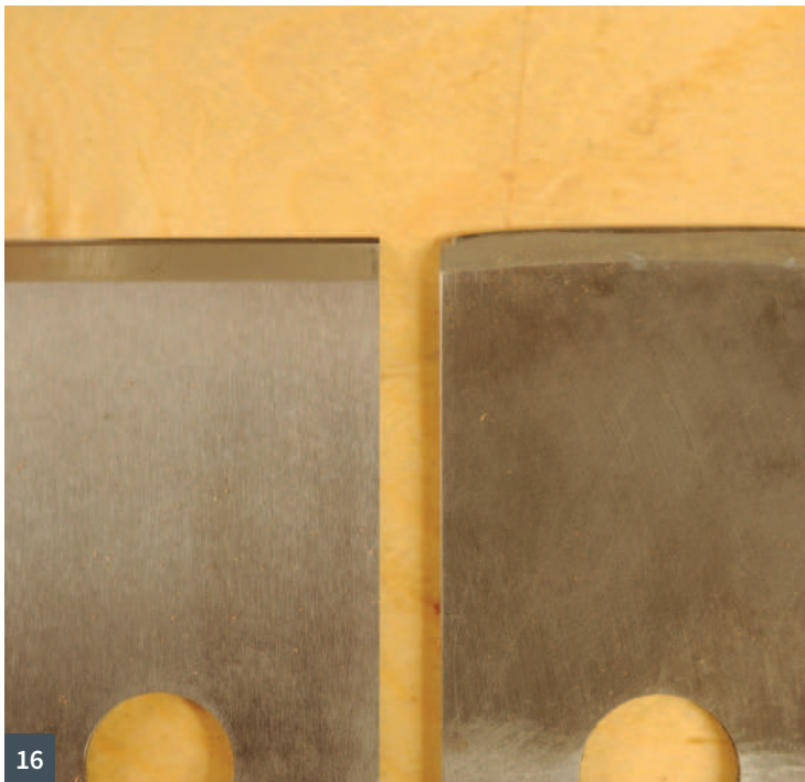
14 A cambered edge, ready to strop 15 An automotive grinding paste will polish the edge 16 The difference between straight and cambered 17 A smoothing blade with rounded ends. As you can see, the cap iron is set back slightly
