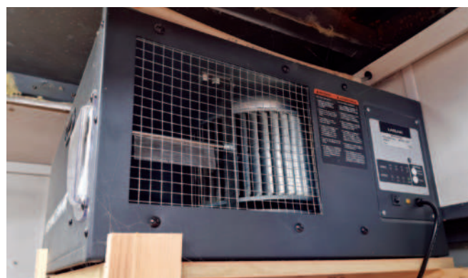
A dust filter is essential in a woodworking workshop
