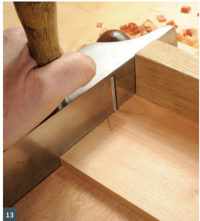
10 Grinding a camber can cause the edge to overheat 11 A secondary micro bevel is the one that performs the cuts 12 A straight-edged blade will 'dig in' 13 A straightedge is needed for trimming end grain
