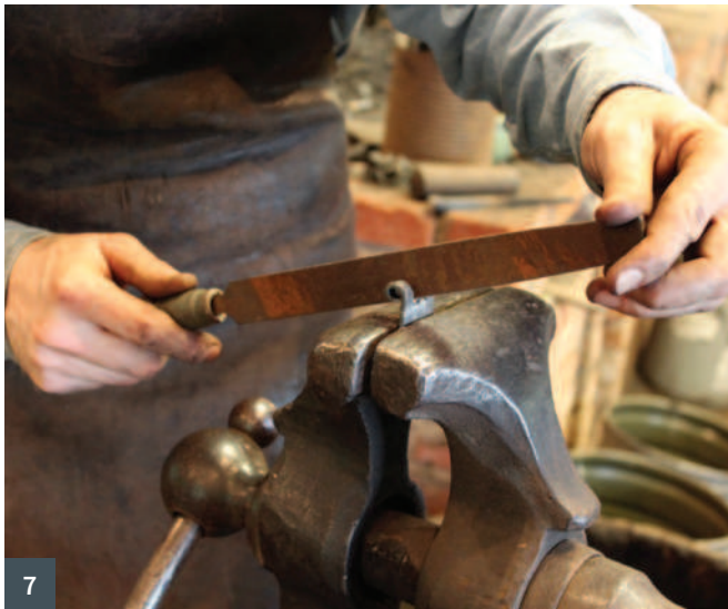
5 Forming the leaf 6 Forming the hinge 7 Cleaning the cut 8 Fitting the hinge
