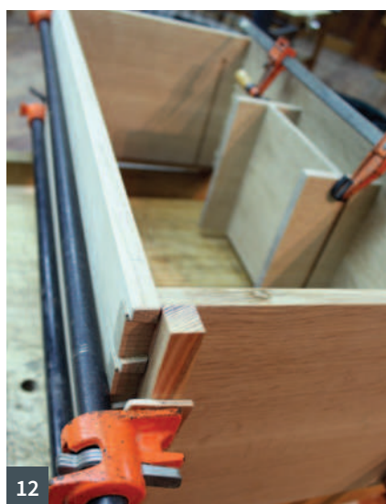
9 The false floor solves problems 10 Refining the sliding dovetail 11 The interior joinery 12 Clamps and cauls in all the right places 13 Gang marking saves time and increases accuracy
