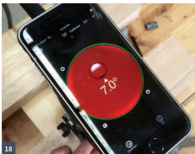
15 Rail fitted to table leg 16 Tilting base angled to that over the dovetail cutter 17 Routing the sliding dovetail 18 Clinometer app showing the router tilt base angle 19 Using layers of masking tape can help with fine adjustment of cutter depth
