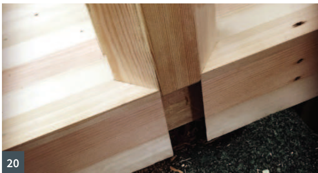
15 Laying out and marking the leg mortises on the top 16 Trimming the bench's other end before installing the legs 17 First cut for the sliding dovetail 18 Breaking out the waste from the sliding dovetail socket with a chisel 19 Roughing out the through mortise with a Festool Domino 20 Test fitting the first leg 21 Marking the stretcher shoulders direct from the legs
