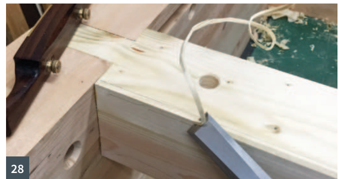
22 Drilling the waste with a 40mm Forstner bit 23 Failed trial drawbore joint with too much offset 24 Successful trial drawbore joint with curve to 1/2in ash peg 25 All joints glued and all pegs hammered home 26 Fitting the face vice 27 Solid brass dogs – on left – and prairie dogs – on right 28 Cutting a chamfer on the front of the legs and stretchers with chisel, spokeshave and block plane
