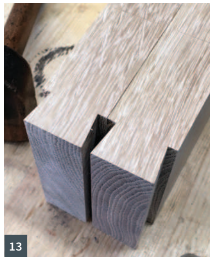
9 ... used to set the fence spacing on the workpiece 10 Marking out the joint can help with depth and fence alignment 11 Dovetail cut in one pass leaving a small ridge on the end ... 12 ... which was easily cleaned up with a block plane 13 End result, clean sliding dovetails 14 The fence is flipped over and spacer used to align the second cut
