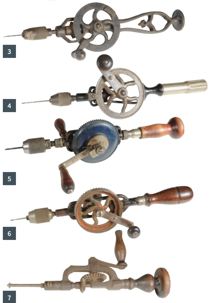
1 & 2 This Millers Falls drill, made around 1920, has two gears, an improved chuck with a thrust race, and drill storage in the handle 3 8in Goodell-Pratt 4 10in Goodell-Pratt 5 13in Millers Falls 6 16in Yankee with several speeds and ratchet system for use in restricted places 7 An early iron wheel brace
