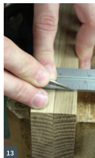
9 The false floor solves problems 10 Refining the sliding dovetail 11 The interior joinery 12 Clamps and cauls in all the right places 13 Gang marking saves time and increases accuracy
