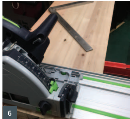
1 Laminating the main slab for the bench top 2 Keeping the slab under 410mm wide allowed rapid planing of the top 3 Wagon vice moving block 4 Cross drilling the salvaged vice nut 5 Marking the dovetails for the end cap 6 Trimming the slab to length 7 Shoulder cut with the track saw
