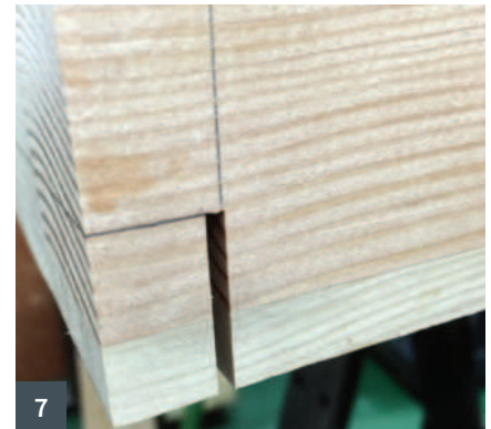
1 Laminating the main slab for the bench top 2 Keeping the slab under 410mm wide allowed rapid planing of the top 3 Wagon vice moving block 4 Cross drilling the salvaged vice nut 5 Marking the dovetails for the end cap 6 Trimming the slab to length 7 Shoulder cut with the track saw
