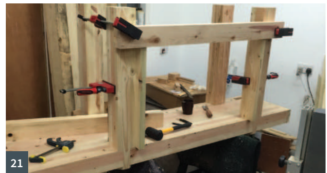
15 Laying out and marking the leg mortises on the top 16 Trimming the bench's other end before installing the legs 17 First cut for the sliding dovetail 18 Breaking out the waste from the sliding dovetail socket with a chisel 19 Roughing out the through mortise with a Festool Domino 20 Test fitting the first leg 21 Marking the stretcher shoulders direct from the legs
