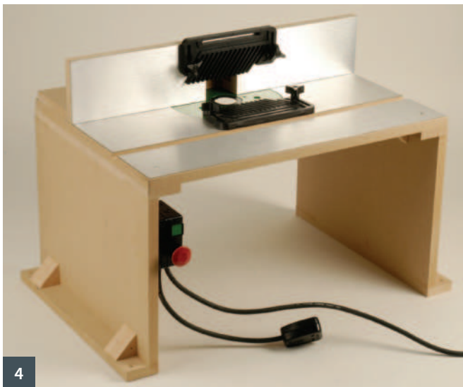
2 The basic carcass of the large table 3 The carcass with the insert plate added 4 The main fence added 5 A rear view showing the dust port and the fence adjustment
