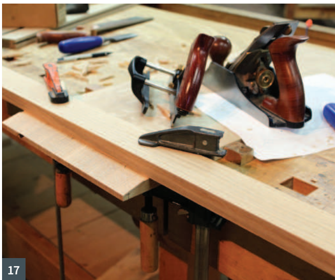
14 Jonathan critiquing my sawing technique 15 Ploughing the grooves 16 The plough plane defines the straight edge 17 The sacrificial board protects the edge 18 This chest is the result of a wonderful collaboration between woodworkers
