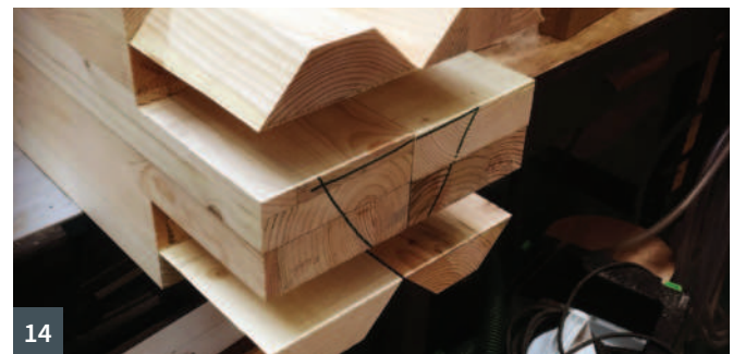
8 Cheek cut with the track saw 9 Fettle the fit of the breadboard endcap and tongue 10 Laminating the final section to the main slab top 11 The 8in radius curve ground on blade for No.3 12 Short and light No.3 as a scrub 13 All four legs together marked with the marriage mark 14 Legs after cutting the joints on the bandsaw
