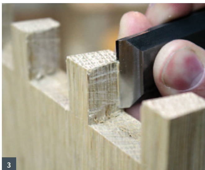
1 The wood was laid out in different orientations to find the best way to put it together 2 The measured drawing 3 Cutting the dovetails 4 Caleb's hand-smithed hardware
