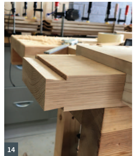
9 ... used to set the fence spacing on the workpiece 10 Marking out the joint can help with depth and fence alignment 11 Dovetail cut in one pass leaving a small ridge on the end ... 12 ... which was easily cleaned up with a block plane 13 End result, clean sliding dovetails 14 The fence is flipped over and spacer used to align the second cut
