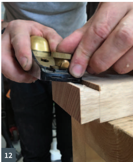
9 ... used to set the fence spacing on the workpiece 10 Marking out the joint can help with depth and fence alignment 11 Dovetail cut in one pass leaving a small ridge on the end ... 12 ... which was easily cleaned up with a block plane 13 End result, clean sliding dovetails 14 The fence is flipped over and spacer used to align the second cut
