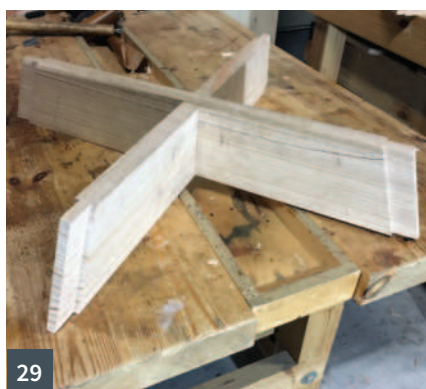
22 Test fit of housing and mortise 23 Turning the legs on the lathe 24 Lathe work-holding jig with sacrificial insert 25 Lathe jig with leg in position 26 Half-lap knife lines marked out 27 Ryoba saw cutting almost to the line 28 A little extra light can help with sawing 29 The half-lap joint cut, pared and test fitted 30 The bandsaw table angled to match the half-lap
