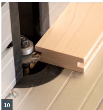
7 Cutting a 45° bevel on the French cleat 8 French cleat fitted to the upper rear of the cabinet 9 Plywood corner fillets glued and screwed 10 Grooving the door's mid rail using a slot cutter 11 Door rail stub tenons cut using a 'tenon-jig' 12 The door assembly glued and clamped
