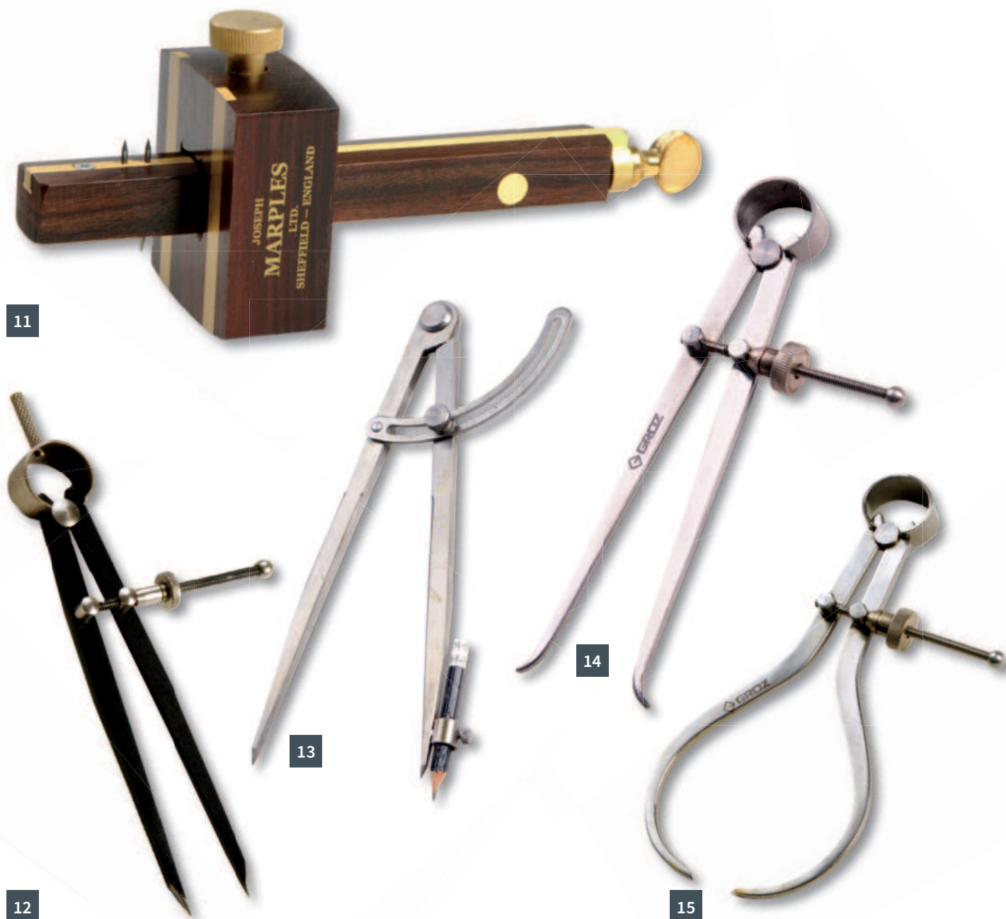
11 A combination mortise marking gauge with screw adjustment 12–15 A pair of dividers, also dividers with a mount for a pencil to be used as a compass, and internal and external callipers
