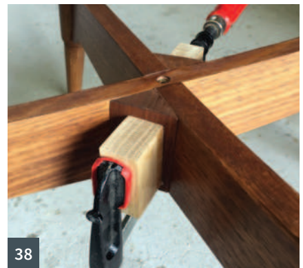
31 Cleaning up bandsaw marks with spokeshaves 32 Fitted to the reupholstered top 33 Setting a marking gauge 34 Rail curves after being cut and tidied 35 Taped up and stained 36 You can never have enough clamps 37 Shop-made liquid hide glue 38 Corner blocks glued and clamped 39 The finished bases
