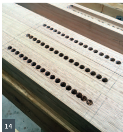
10 Jig-centring jig 11 The centring jig locating in the router jig slot 12 Jig fences clamped in position 13 Marking out the legs 14 Leg blanks, mortises drilled out 15 Routing the rail shoulder housing
