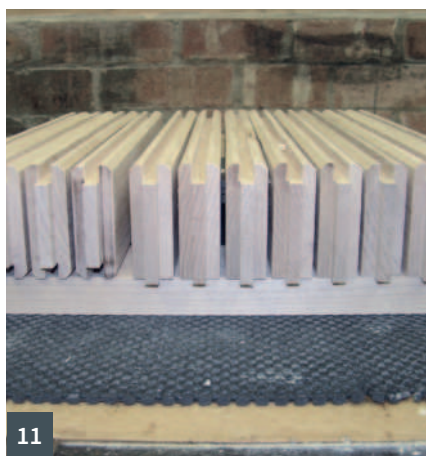
7 Cutting a 45° bevel on the French cleat 8 French cleat fitted to the upper rear of the cabinet 9 Plywood corner fillets glued and screwed 10 Grooving the door's mid rail using a slot cutter 11 Door rail stub tenons cut using a 'tenon-jig' 12 The door assembly glued and clamped
