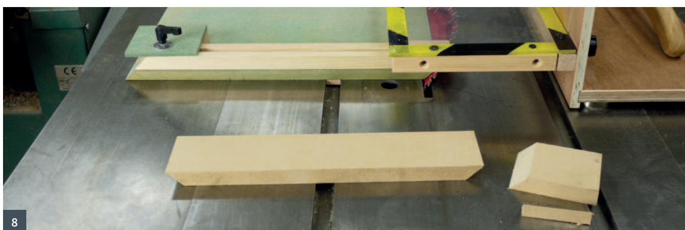
6–8 After making the first cut, position the stop for the desired length, rotate the pieces and make the opposite cut
