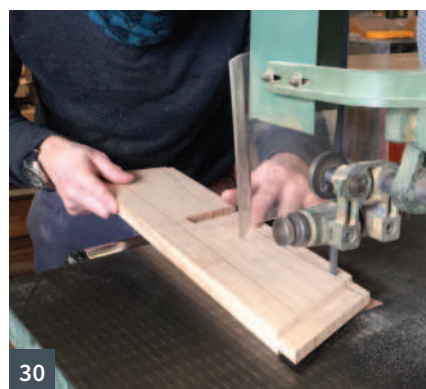
22 Test fit of housing and mortise 23 Turning the legs on the lathe 24 Lathe work-holding jig with sacrificial insert 25 Lathe jig with leg in position 26 Half-lap knife lines marked out 27 Ryoba saw cutting almost to the line 28 A little extra light can help with sawing 29 The half-lap joint cut, pared and test fitted 30 The bandsaw table angled to match the half-lap
