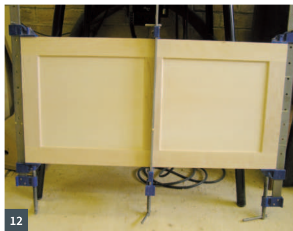
7 Cutting a 45° bevel on the French cleat 8 French cleat fitted to the upper rear of the cabinet 9 Plywood corner fillets glued and screwed 10 Grooving the door's mid rail using a slot cutter 11 Door rail stub tenons cut using a 'tenon-jig' 12 The door assembly glued and clamped
