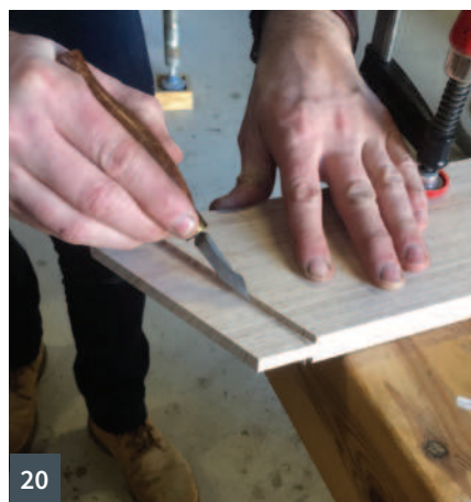
16 Material added to reduce the slot size for mortising 17 Cutting out the legs. Note the use of an independently mounted crown guard 18 The angled tenon shoulders cut on the saw 19 The rail itself is used to reset the fence angle 20 Knife run along the shoulder 21 Paring for a fine fit
