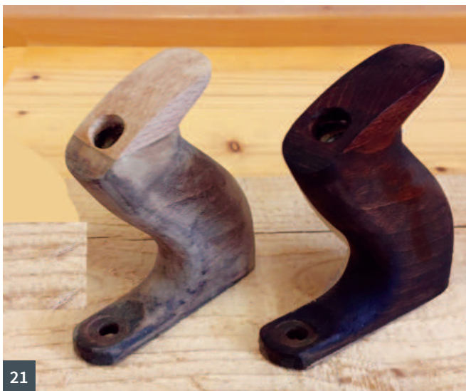
18 The broken handle of the No.5 19 A new ear was made from beech and glued and clamped in place 20 Shaping the tote with a rasp 21 A dark wood dye was applied to complete the handle 22 A homemade hybrid plane
