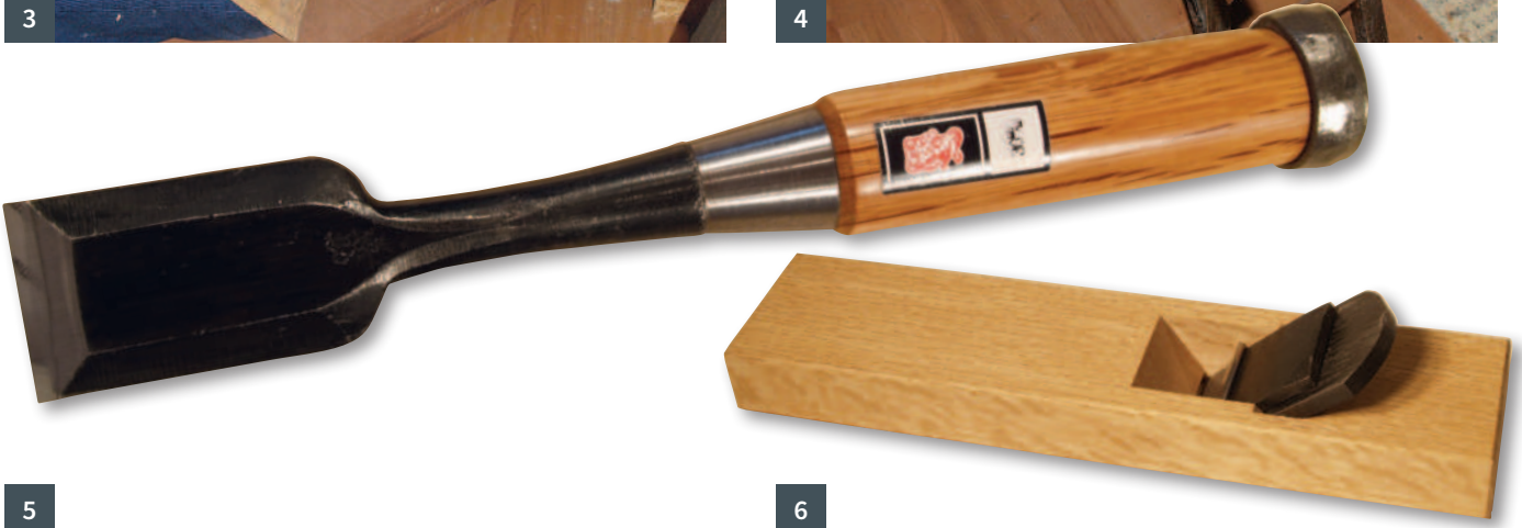
1 As with all Japanese saws the dozuki backsaw cuts on the pull stroke 2 The ryoba saw has cross-cut and rip teeth 3 The ryoba in rip mode for a big plank 4 The ryoba in cross-cut mode being used to cut the project shelf top to length 5 Large flat chisel 6 A Japanese plane is high maintenance but gives perfect results
