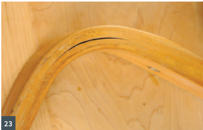
21 The de-waxing solution removes only dirt and grime leaving the existing finish intact 22 Button polish was used to bring the areas of bare wood up to the same colour as the rest of the trolley 23 Out of eight tight corner bends half were showing signs of de-laminating 24 Look closely and you can see the diagonal glue lines where the complete hoop was joined
