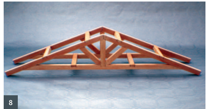
1 Marking the angles on the tie beams 2 Cutting the tie beam end 3 Cutting the slots for the bracing bars 4 Clearing the slots with a detail knife 5 Roof frames assembled 6 Gluing and clamping the roof truss over the full-size front elevation drawing 7 Joining and gluing the two roof trusses together with the bracing bars 8 The completed roof frame
