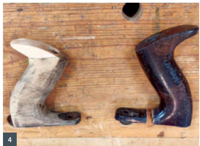
1 UK hybrid No.2690/91 by Marples 2 Modified wooden Chinese (L) and standard Czech Horned plane (R) 3 Exclude all planes with any damage to the body casting, like this metal plane 4 Broken wooden plane handles, showing impact damage
