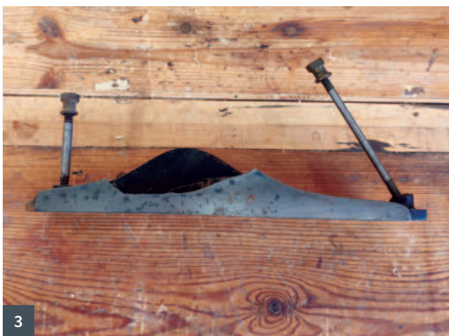
1 UK hybrid No.2690/91 by Marples 2 Modified wooden Chinese (L) and standard Czech Horned plane (R) 3 Exclude all planes with any damage to the body casting, like this metal plane 4 Broken wooden plane handles, showing impact damage
