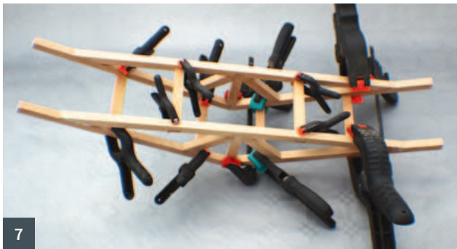
1 Marking the angles on the tie beams 2 Cutting the tie beam end 3 Cutting the slots for the bracing bars 4 Clearing the slots with a detail knife 5 Roof frames assembled 6 Gluing and clamping the roof truss over the full-size front elevation drawing 7 Joining and gluing the two roof trusses together with the bracing bars 8 The completed roof frame
