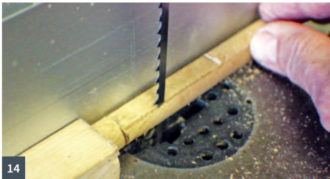
9 Drilling the holes for the support dowels 10 Wood for the dowels 11 Making the dowels 12 Making the horizontal support dowels 13 Forming the flat regions on the support dowels with a gouge... 14 ...or the bandsaw 15 The completed back post
