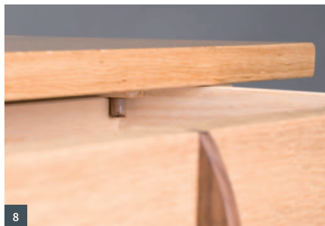
7 The central divider in the drawer 8 The walnut dowel in use as a drawer stop
