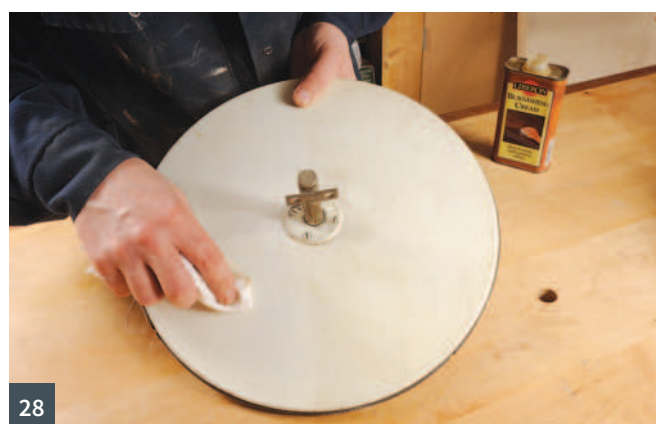
25 These little markings give an indication of how the trolleys were manufactured 26 The old laminate was used as a template to cut the new linoleum with an additional couple of millimetres for fine trimming 27 A plane can be used to trim the linoleum to get good, clean edges 28 Burnishing cream was used to blend the chips that had been touched up using white shellac with the existing paint
