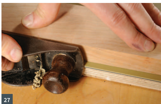
25 These little markings give an indication of how the trolleys were manufactured 26 The old laminate was used as a template to cut the new linoleum with an additional couple of millimetres for fine trimming 27 A plane can be used to trim the linoleum to get good, clean edges 28 Burnishing cream was used to blend the chips that had been touched up using white shellac with the existing paint
