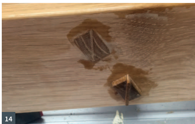
11 Wedging the tenons – the fixture in use on the shooting board 12 Showing the wedge to the mortise and marking the length 13 Glue-up with angled clamp head packers to allow clamping without bruising the timber 14 Trimming the tenons flush with a flushcut saw before smooth planing the outsides of the ladder section 15 The ladder section shimmed up by 6mm to allow the angle and length of the rear section to be scribed to exact length and angle with a 6mm block
