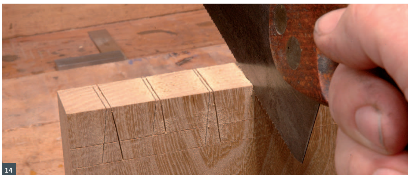
13 The finger and thumb pinch the board to guide the blade at the start of a cut 14 Cuts on marking lines that are made with a knife are normally guided down the waste side of the line while pencil lines are split
