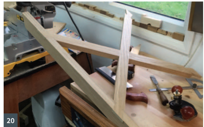
16 Marking the dovetail sockets with the rear section clamped to the ladder section over 2mm spacers for clearance in the final assembly 17 Cutting the sockets and kerfing the waste prior to chopping out 18 Cleaning the base of the dovetail sockets with a router plane to final depth 19 Dovetail socket cleaned out ready for dry fitting 20 Dry fitting a pair of dovetails together changed the fit of the joint slightly and tightened everything up
