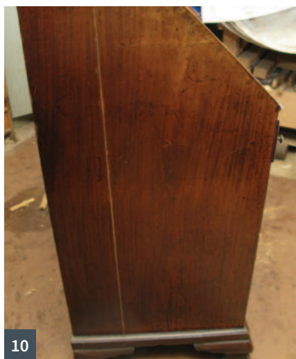
8 Clamping the glue-injected rail joints 9 The kicker being glued in place; sprung lathes hold it in place 10 The vertical fillet fitted to the left-hand side 11 The worn and damaged drawer sides and nailed runner
