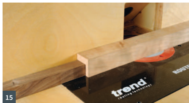
9 Hand tools for making rebates, from top to bottom: cabinetmaker's shoulder rebate, carriage-maker's rebate and a small shoulder rebate 10 Cleaning up a rebate is quick and easy 11 There are different ways to machine rebates 12 Routing using a 'breakthrough' fence and pushblock 13 Wider boards can be easily rebated 14 Narrow stock needs safe support 15 First, an outfeed support to fit the rebate
