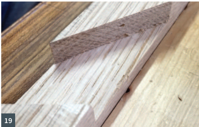
16 Marking the dovetail sockets with the rear section clamped to the ladder section over 2mm spacers for clearance in the final assembly 17 Cutting the sockets and kerfing the waste prior to chopping out 18 Cleaning the base of the dovetail sockets with a router plane to final depth 19 Dovetail socket cleaned out ready for dry fitting 20 Dry fitting a pair of dovetails together changed the fit of the joint slightly and tightened everything up
