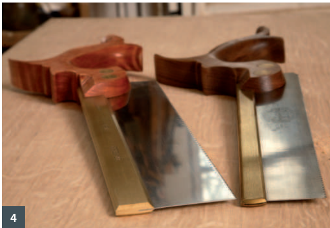
1 This tenon saw has a 350mm-long, 75mm-deep blade with a D handle while the dovetail saw (right) has a 230mm-long, 30mm-deep blade and a pistol-grip handle 2 Although all described as pistol grips and looking similar, the dimensions and feel of different handles can vary a lot 3 Sighting along the blade and then the back of a saw confirm that both are straight 4 Brass backs can be milled or folded (right) in manufacture; some are made from steel 5 The blade must be firmly gripped before it can be sharpened, ideally in a saw vice
