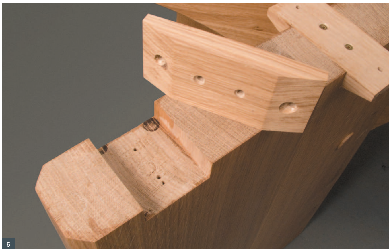
6 The fixing blocks are screwed into sockets
