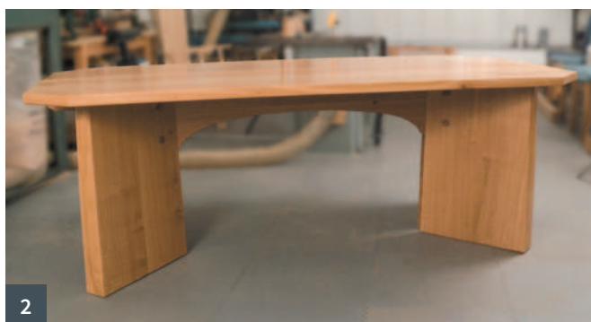
1 The central stretcher beam is an integral part of the top 2 Only seven components make up the very direct, simple concept
