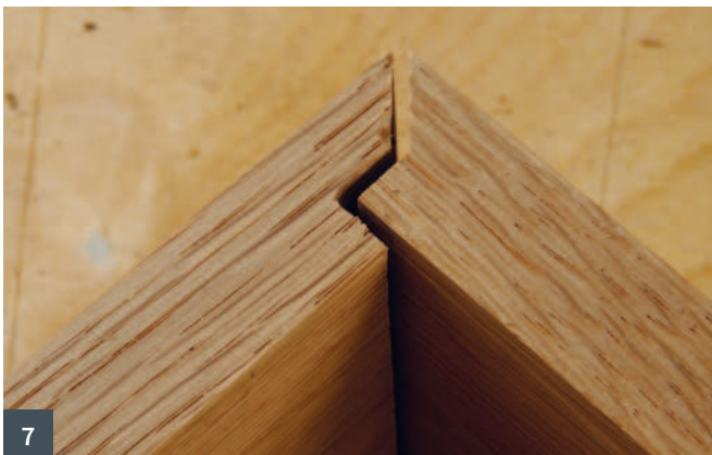
1 Here I am fitting a glazing bead into the rebate 2 A useful set, but why have a dovetail cutter? 3 I find that I can do a lot more with these cutters 4 Frame rebate 5 Corner rebate 6 Lap rebate 7 Mitred rebate 8 Rebated tongue and groove
