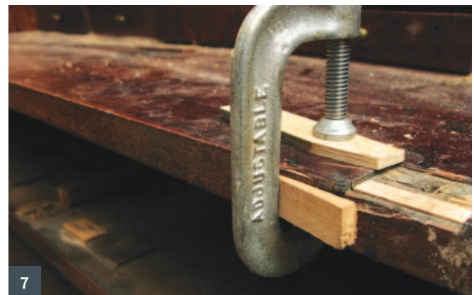
1 Damage to the left hand of the flap; note the worn screw holes 2 Trimming off the dowels inserted to strengthen the repair to the left of the flap 3 Damage to the hinge point at the right side 4 Preparation for cutting the recess to repair the broken hinge area 5 Clamping on the replacement in the recess 6 Clamping an additional piece around the screw area 7 The improvised edge clamp
