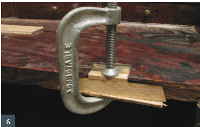
1 Damage to the left hand of the flap; note the worn screw holes 2 Trimming off the dowels inserted to strengthen the repair to the left of the flap 3 Damage to the hinge point at the right side 4 Preparation for cutting the recess to repair the broken hinge area 5 Clamping on the replacement in the recess 6 Clamping an additional piece around the screw area 7 The improvised edge clamp
