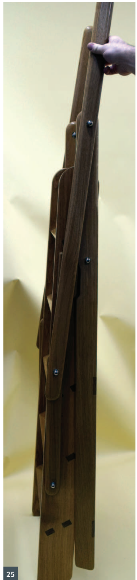
21 Dovetailed back brace being glued up 22 Fitting the stops with Dominoes and hide glue 23 Final assembly with nylon bearing washers 24 Detail of the stops and clearance cutouts 25 The folded steps
