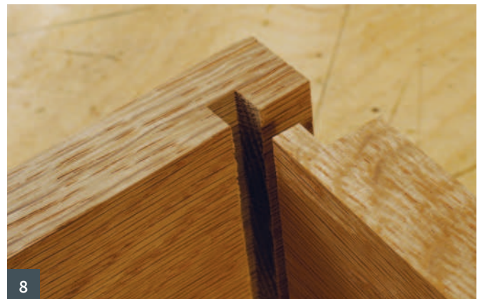
1 Here I am fitting a glazing bead into the rebate 2 A useful set, but why have a dovetail cutter? 3 I find that I can do a lot more with these cutters 4 Frame rebate 5 Corner rebate 6 Lap rebate 7 Mitred rebate 8 Rebated tongue and groove
