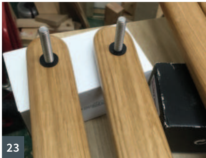
21 Dovetailed back brace being glued up 22 Fitting the stops with Dominoes and hide glue 23 Final assembly with nylon bearing washers 24 Detail of the stops and clearance cutouts 25 The folded steps
