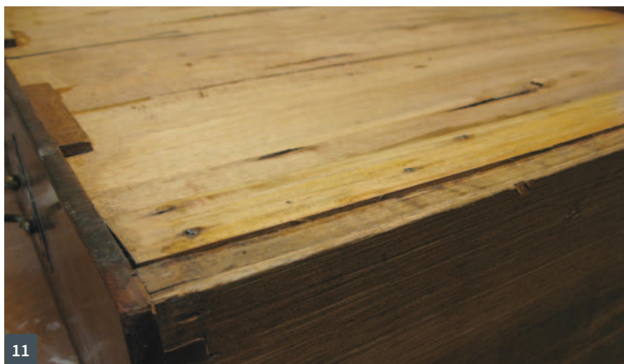
8 Clamping the glue-injected rail joints 9 The kicker being glued in place; sprung lathes hold it in place 10 The vertical fillet fitted to the left-hand side 11 The worn and damaged drawer sides and nailed runner
