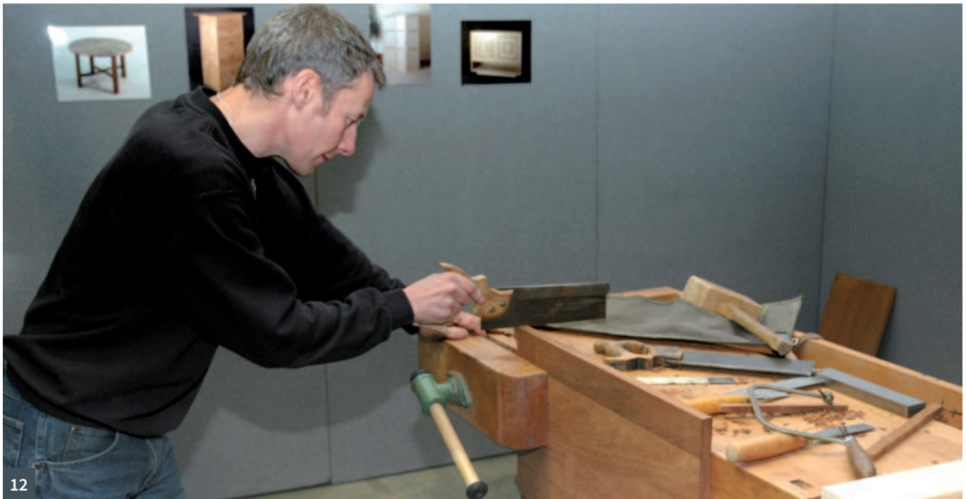
10 Martin Grierson examines the teeth and feels the amount of set on a new dovetail saw 11 Martin's arm and sawblade form a straight line as he crosscuts a piece of walnut against a bench hook 12 Andrew Lawton stands with his feet well back from the bench while sawing in the vice
