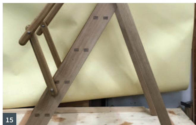
11 Wedging the tenons – the fixture in use on the shooting board 12 Showing the wedge to the mortise and marking the length 13 Glue-up with angled clamp head packers to allow clamping without bruising the timber 14 Trimming the tenons flush with a flushcut saw before smooth planing the outsides of the ladder section 15 The ladder section shimmed up by 6mm to allow the angle and length of the rear section to be scribed to exact length and angle with a 6mm block
