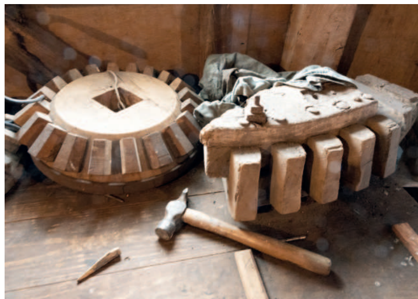
Internal gears are usually wooden too, often apple wood or hornbeam
