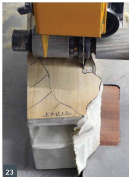
19 Cut the simplest side first 20 Now cut the opposite side 21 Dust off and mask together 22 Cut along lines E and then S (from nose) 23 Cut from lower S up to E 24 The completed two-profile form
