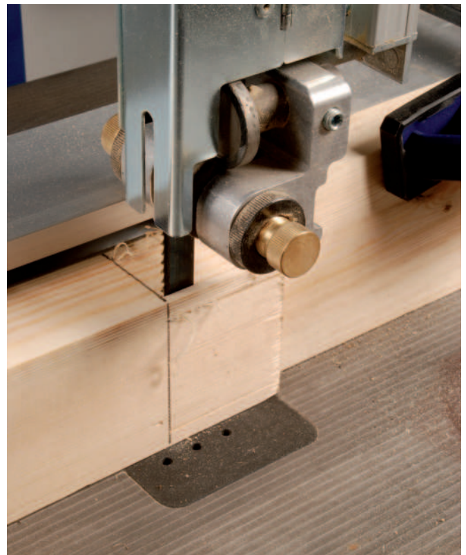
Clamp a stop to the blade when making tenon cuts
