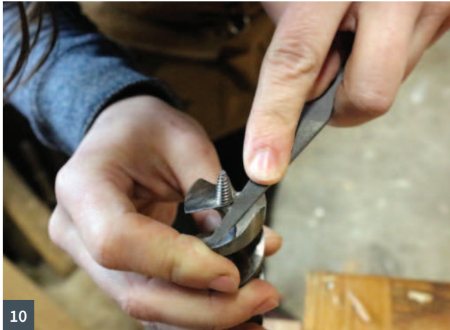
6 TX Heritage auger roll, made by Jason Thigpen 7 The beautifully restored eggbeater drill 8 My collection of boring tools 9 & 10 Sharpening an auger bit 11 Drilling benchdog holes is a great exercise
