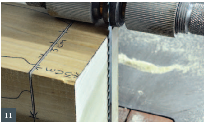
7 A 6mm skip-toothed 4tpi blade 8 The blade guide set 1mm above the timber 9 Cut directly along the lower edge of the line 10 Cut up to the 30mm mark 11 Adjust the blade guides for the front view 12 Repeat the previous steps
