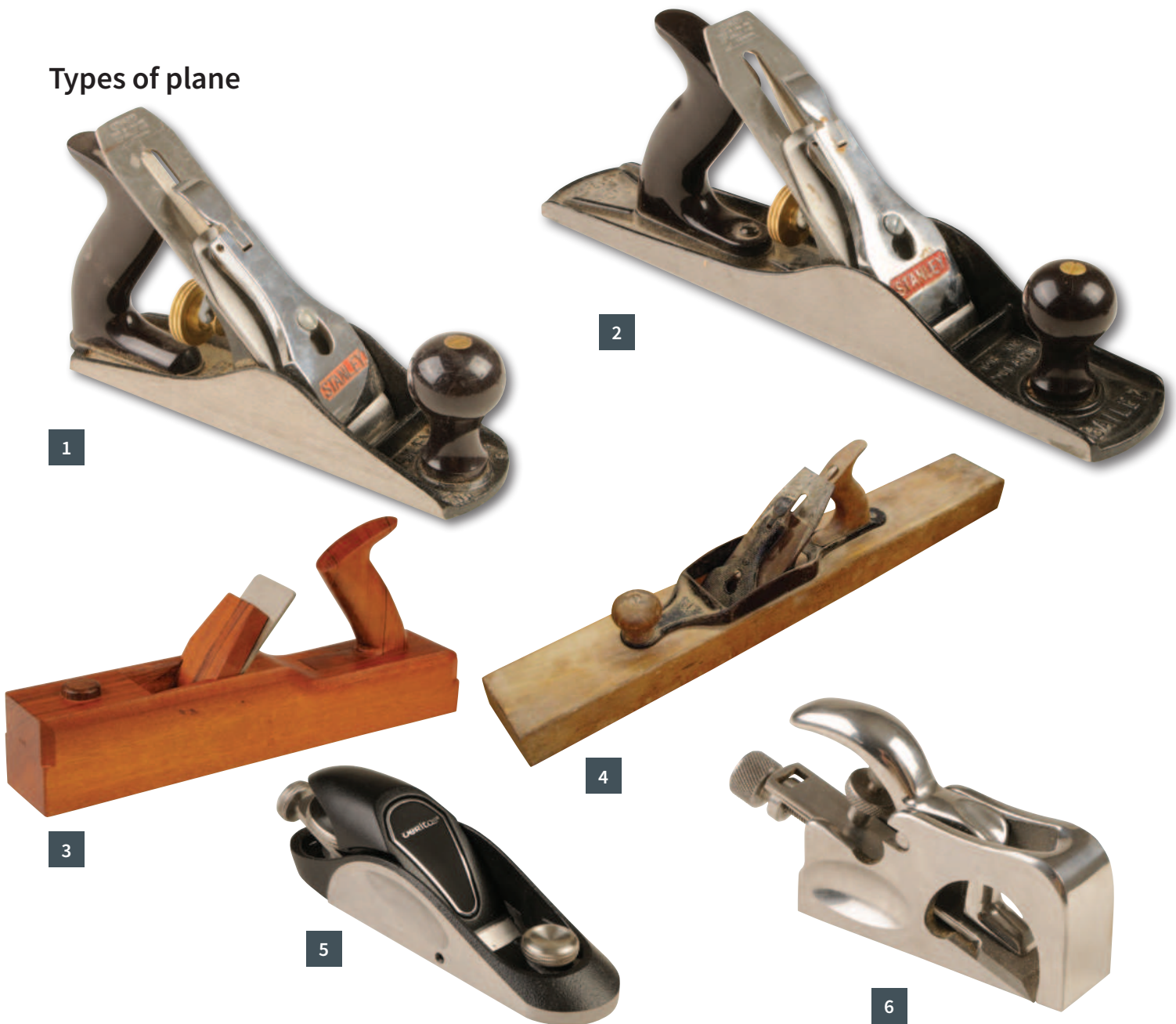
1 A smoothing plane 2 A Stanley No.5 Jack plane made of a cast-iron bed with steel, brass and wood components 3 A wooden Jack plane made by Phil Edwards of Philly Planes 4 An antique Stanley No.32 transitional jointer plane, which is a whopping 660mm (26in) long 5 A Veritas DX60 block plane with a bed length of about 165mm (6½in) 6 A bull nose rebate plane
