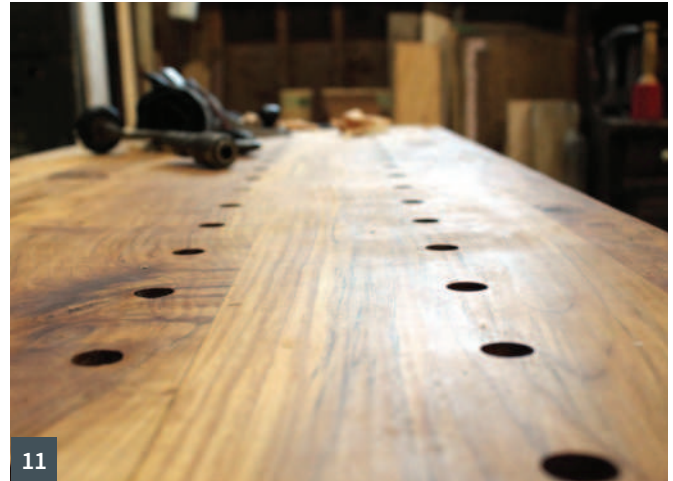
6 TX Heritage auger roll, made by Jason Thigpen 7 The beautifully restored eggbeater drill 8 My collection of boring tools 9 & 10 Sharpening an auger bit 11 Drilling benchdog holes is a great exercise
