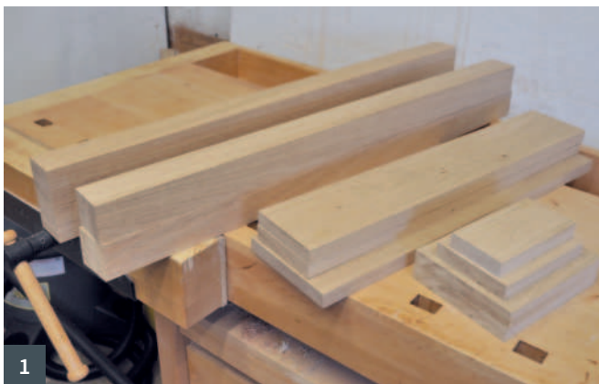
1 The pieces for the construction of the framework were machined simultaneously in order to obtain consistent sizes 2 The taper was marked out on the legs in pen to make it easier to follow
