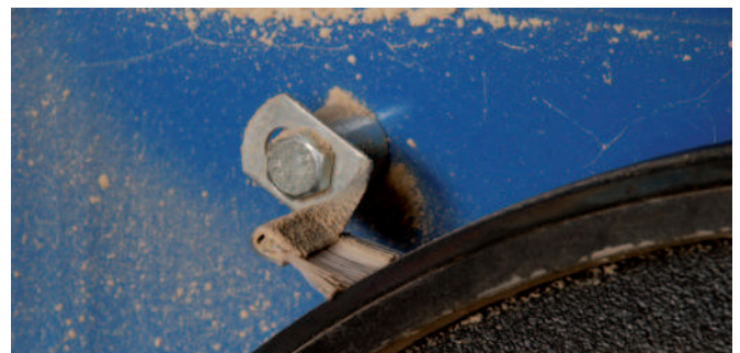
Regular cleaning of the bandwheel is important
