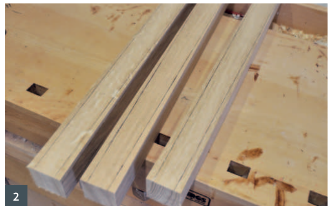
1 The pieces for the construction of the framework were machined simultaneously in order to obtain consistent sizes 2 The taper was marked out on the legs in pen to make it easier to follow
