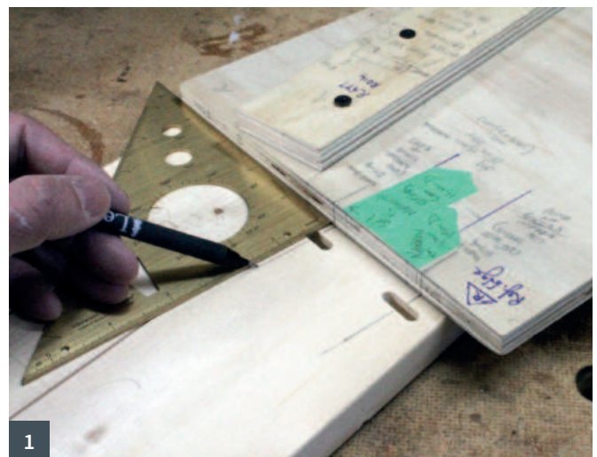
1 The placement lines were changed on the jig to make sure the mortises were spaced further apart
