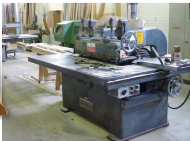
This Wadkin straight-line edger with caterpillar track and autofeed dates from the 1950s and is still in use at Woodworks of Lewes
