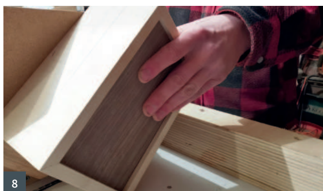
4 ... before tilting the blade to cut the mitres 5 & 6 The box was assembled and secured with tape before the glue-up 7 I measured the diagonals to ensure everything was square 8 & 9 A jig was used to hold the box on in position when cutting the keyed corners
