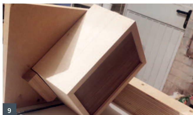
4 ... before tilting the blade to cut the mitres 5 & 6 The box was assembled and secured with tape before the glue-up 7 I measured the diagonals to ensure everything was square 8 & 9 A jig was used to hold the box on in position when cutting the keyed corners
