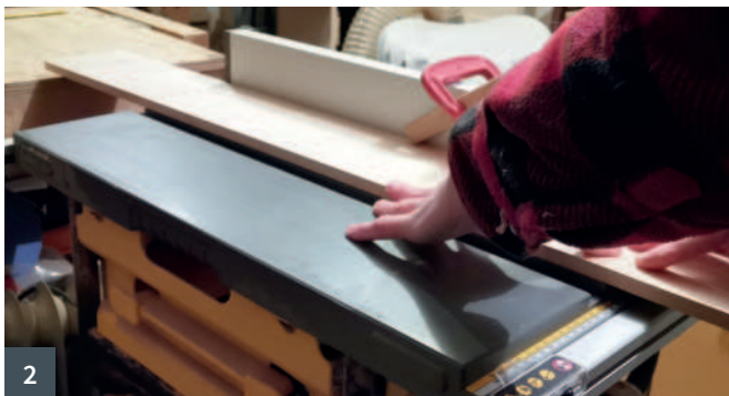
1 The box carcass was made from boards of rippled sycamore 2 Grooves were cut along the lengths of the sycamore boards prior to cross-cutting 3 The boards were cross-cut square ...
