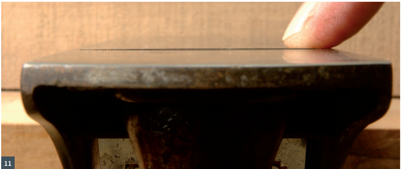
8 A good viable alternative is to use a honing guide to clamp a chisel 9 The same guide can be opened out to take plane irons and, by careful measurement of the protruding end, the same angle can be honed each time 10 Tramlines caused by sharp corners on a plane cutter 11 Curving the cutting edge guarantees there will be no tramlines
