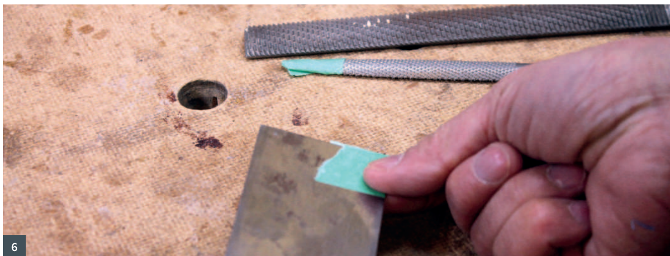
2 Highlighting where to stop cuts 3 A handy installation marker 4-6 Tape can protect surfaces from tool marks
