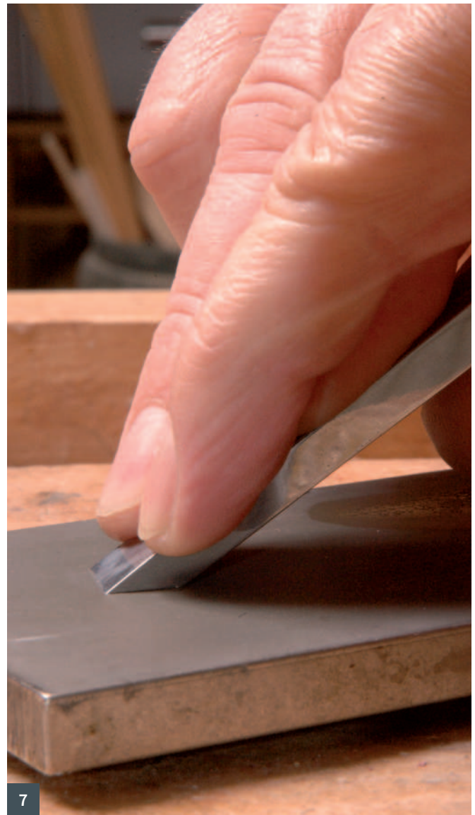
5 The waterstone wheel produces a hollow grind with a small 'wire edge' 6 Two polished areas are visible on the hand-honed chisel – one on the cutting edge, the other on the 'heel' which holds a constant angle 7 After hollow grinding, honing by hand on a flat stone produces an accurately repeatable angle on the working edge
