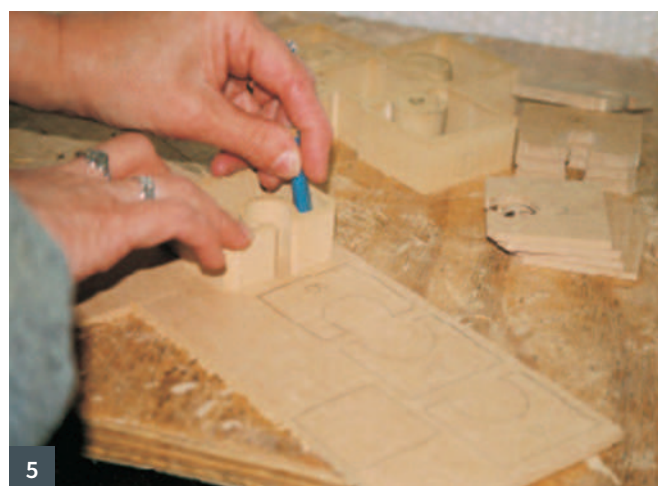
1 Stick the pieces of MDF together using double-sided tape 2 Cut around the outside of the boxes 3 Next, carefully cut out the jigsaw shapes 4 Mark and cut out the box cavities 5 Use the box body to mark out the lid
