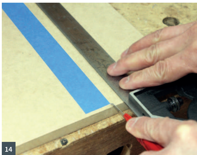
11 Tape can improve sawing accuracy 12–15 Using tape for extra precision
