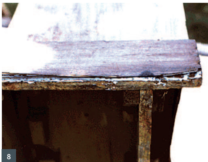
7 The black ring was removed by scraping carefully with the tip of a chisel 8 PVA glue was applied to both the pine ground and the mahogany veneer 9 A clean cloth was used to apply an even stain to the whole cabinet
