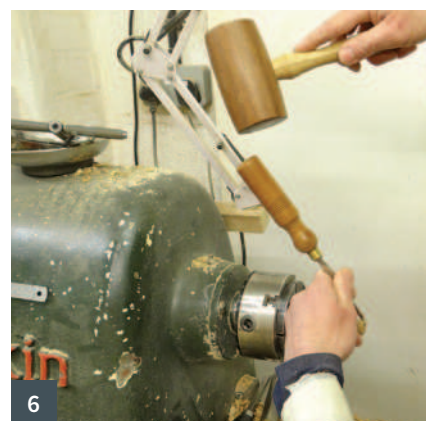
1 Rook samples in tulip 2 Turning the rook 3 Marking the crenellations 4 Using my dovetail saw on the crenellations 5 Enlarging the saw cuts with a chisel 6 Squaring them with a 3mm chisel
