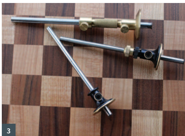
1 Traditional 'pin' marking gauges 2 Hamilton Woodworks' wooden 'cutting' gauges are small and lightweight 3 Modern 'wheel' cutting gauges can often come with fine adjusters and multiple locking mechanisms 4 A relatively crude pin gauge can be transformed into something more accurate with the help of a safe edge file 5 A mortise gauge enables you to capture and translate key reference lines in pairs
