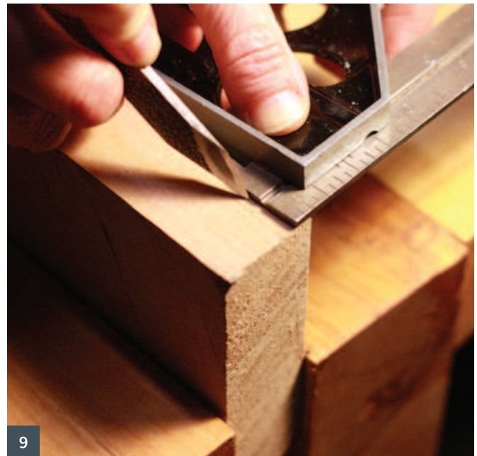
6 A bench hook provides a sturdy support for marking out 7 A wheel gauge has less tendency to split out at the edge 8 The chisel registers within the knife line 9 Marking gauge in a pinch
