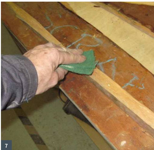
5 I avoided using the bevel side of the chisel when levering the components apart to avoid denting the wood 6 The worn looking tenons, the original dowel peg holes are visible in one tenon 7 Using a scouring pad to clean the edges of dirt and dust ready for re-gluing 8 An interesting glimpse into the table's history – a warehouse storage sticker, judging by the number one of many pieces of furniture that were kept in store
