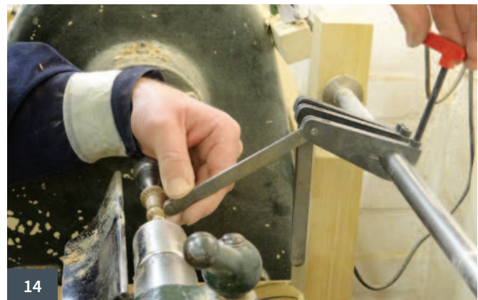
11 Turning one of the oak queens 12 Sample and finished kings 13 Turning one of the kings 14 Setting the duplicating fingers
