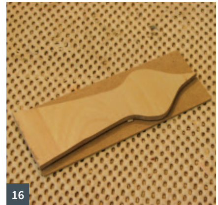
9 Test cut for the top leg joint 10 Stop block and fence set-up 11 The leg top joints 12 The legs being sanded 13 Legs chamfered and glued to the table apron 14 The template for corner braces 15 The corner braces blank affixed to double-sided tape 16 The template stuck to the brace blank with the tape
