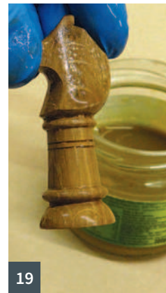
15 Marking the details with the storyboard 16 The moment the duplicating finger drops and I reach the correct diameter 17 Rolling the ball-shaped head 18 The completed oak set 19 After dipping in the ebonising solution, the oak colour immediately begins to change 20 Oiling the piece
