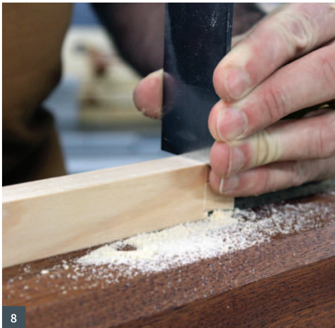
6 A bench hook provides a sturdy support for marking out 7 A wheel gauge has less tendency to split out at the edge 8 The chisel registers within the knife line 9 Marking gauge in a pinch
