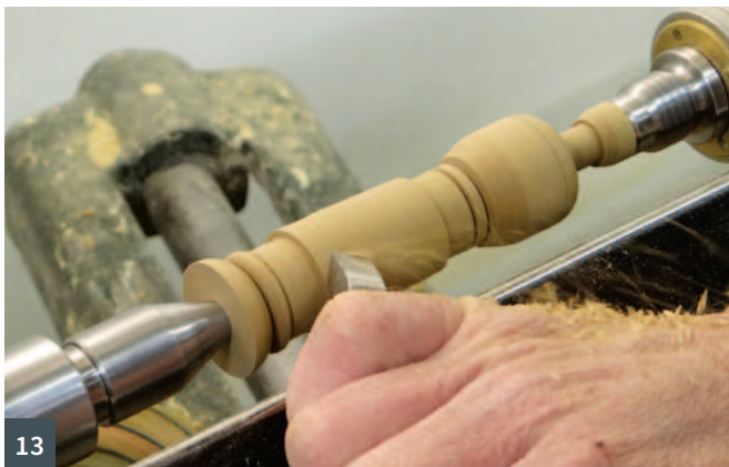
11 Turning one of the oak queens 12 Sample and finished kings 13 Turning one of the kings 14 Setting the duplicating fingers
