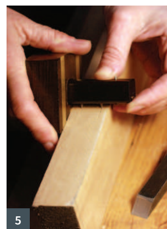
1 Traditional 'pin' marking gauges 2 Hamilton Woodworks' wooden 'cutting' gauges are small and lightweight 3 Modern 'wheel' cutting gauges can often come with fine adjusters and multiple locking mechanisms 4 A relatively crude pin gauge can be transformed into something more accurate with the help of a safe edge file 5 A mortise gauge enables you to capture and translate key reference lines in pairs
