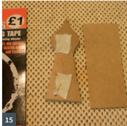
9 Test cut for the top leg joint 10 Stop block and fence set-up 11 The leg top joints 12 The legs being sanded 13 Legs chamfered and glued to the table apron 14 The template for corner braces 15 The corner braces blank affixed to double-sided tape 16 The template stuck to the brace blank with the tape
