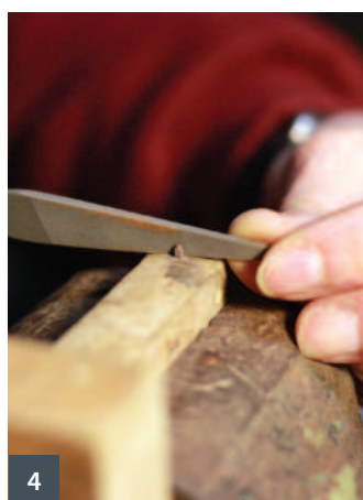
1 Traditional 'pin' marking gauges 2 Hamilton Woodworks' wooden 'cutting' gauges are small and lightweight 3 Modern 'wheel' cutting gauges can often come with fine adjusters and multiple locking mechanisms 4 A relatively crude pin gauge can be transformed into something more accurate with the help of a safe edge file 5 A mortise gauge enables you to capture and translate key reference lines in pairs
