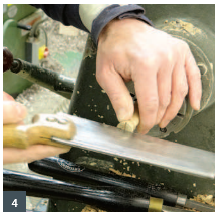
1 Rook samples in tulip 2 Turning the rook 3 Marking the crenellations 4 Using my dovetail saw on the crenellations 5 Enlarging the saw cuts with a chisel 6 Squaring them with a 3mm chisel
