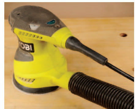
Extraction is better than using a dust bag
