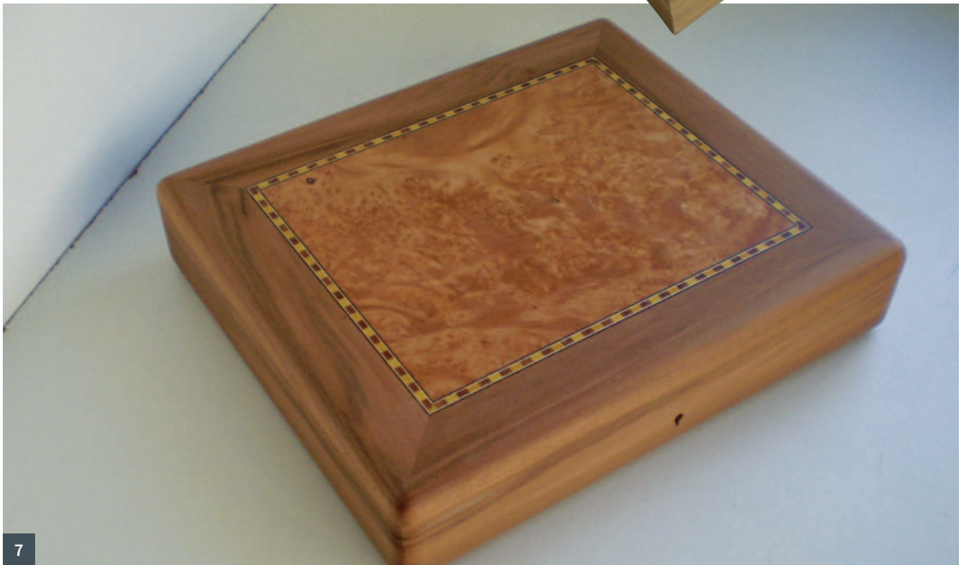
5 The lid frame was secured with a band clamp 6 The bottom panel was glued into its rebate 7 Inlay banding sits between the maple burr panel and the walnut lid frame
