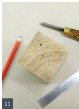
7 & 8 Adding pencil lines front and back before profiling 9 My sanding jig, which holds my belt sander safely on its side 10 The progression of my prototypes to the final sample on the right 11 The 15mm offset to produce the profile with the ray fleck on each side 12 Turning the shape prior to offsetting
