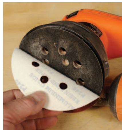
Hook-and-loop makes sheet changing very fast
