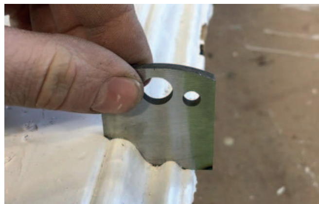
Cutters are ground in house to machine new custom mouldings
