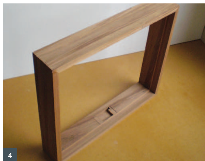
1 These walnut drawer fronts came from an old chest of drawers 2 Stringing surrounds the maple burr 3 The mitres needed hardly any adjustment 4 The recess for the box lock should be cut at this stage
