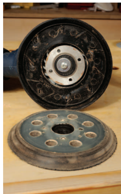
The eccentric plate in the centre is clearly visible
