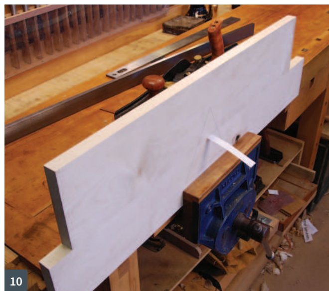
6 First 'stop' shaving 7 Second 'stop' shaving 8 Third 'stop' shaving 9 Board is slightly hollow so that the paper can slip in underneath 10 Both boards planed slightly hollow
