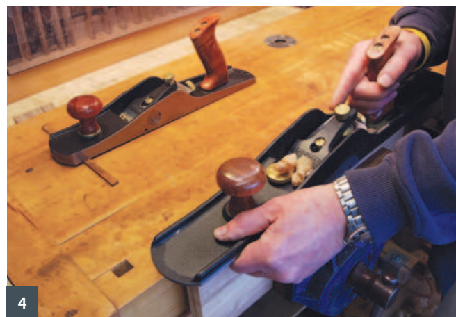
1 Walnut end grain – showing the joints 2 Bench level in both planes 3 Hand position for edge planing. Note the position of the lead hand 4 Planing two thin boards together. The position of the lead hand ensures constant pressure across the length of the stroke 5 Planing a board dead straight is only one option
