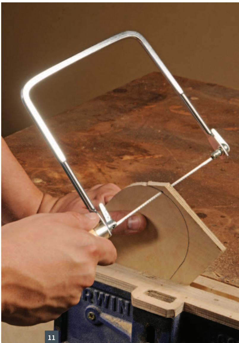
11 A coping saw in action cutting out a curve 12 A close-up look at a coping saw 13 A hacksaw 14 A Japanese pull saw 15 Irwin's hardpoint variation of a Japanese pull saw
