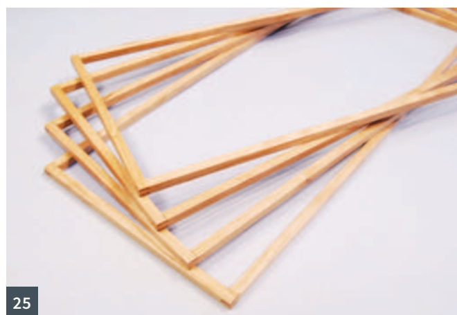
19 The equipment prepared for hot acrylic bending 20 The bending jig in use 21 The heating mask jig 22 The bending jig ready 23 Routing 2.5mm bridge joints for the shoji panels 24 The lamp fitting inside the framework 25 Four shoji panels, polished and ready for paper
