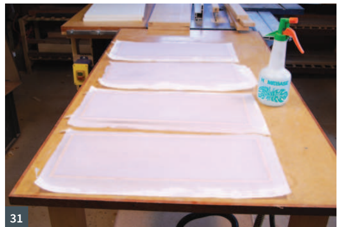
26 Paper taped to bench, frame under 27 Rice glue bottle, frame and paper 28 Paper glued to the frame 29 Stacked between boards 30 The panels weighted down 31 Panels sprayed with water
