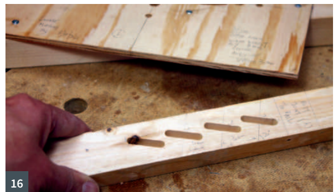
7 Marking a centre line as the alignment line on the inside strip 8 The hole for the index pin CUTTING THE ANGLED SLOTS: 9 Marking the angled lines for the slots 10 Clamping the stile in place 11 Plunge the Joiner to make the mortise 12 Realigning the stile 13 Milling the second and third slots 14 Positioning the stile using the index pin 15 Milling the slot 16 The mortised slots
