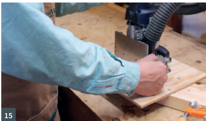
7 Marking a centre line as the alignment line on the inside strip 8 The hole for the index pin CUTTING THE ANGLED SLOTS: 9 Marking the angled lines for the slots 10 Clamping the stile in place 11 Plunge the Joiner to make the mortise 12 Realigning the stile 13 Milling the second and third slots 14 Positioning the stile using the index pin 15 Milling the slot 16 The mortised slots
