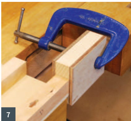
1 The practice joint 2 The practice joint exposed 3 Hand planing to 22mm 4 Marking out, with the aid of three clamps 5 Using the indexing jig 6 The indexing jig for the first Domino mortise 7 The first mortise cut, with the leg turned through 90° 8 Using 'mock' Dominos to test the fit and alignment 9 Using a cabinetmaker's triangle to mark the position of each piece on each side
