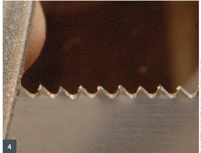
1 My old Disston handsaw, which is about 20 years old and still going strong after numerous re-sharpenings 2 A joiner's panel saw 3 Crosscut saw teeth have a pointed profile 4 Rip saw teeth are sharpened to a chisel edge, not to a point
