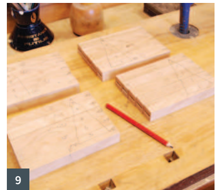
1 The practice joint 2 The practice joint exposed 3 Hand planing to 22mm 4 Marking out, with the aid of three clamps 5 Using the indexing jig 6 The indexing jig for the first Domino mortise 7 The first mortise cut, with the leg turned through 90° 8 Using 'mock' Dominos to test the fit and alignment 9 Using a cabinetmaker's triangle to mark the position of each piece on each side
