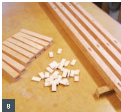
1 The practice joint 2 The practice joint exposed 3 Hand planing to 22mm 4 Marking out, with the aid of three clamps 5 Using the indexing jig 6 The indexing jig for the first Domino mortise 7 The first mortise cut, with the leg turned through 90° 8 Using 'mock' Dominos to test the fit and alignment 9 Using a cabinetmaker's triangle to mark the position of each piece on each side
