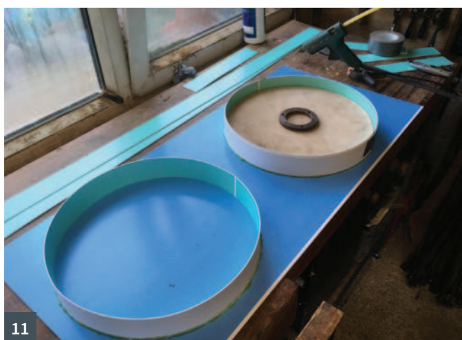
8 Pressure pot with compressor 9 Using a small blowtorch to remove bubbles 10 Using a torch to see the bubbles 11 Moulds ready for use for casting bedside tables 12 Multiple moulds ready for small castings
