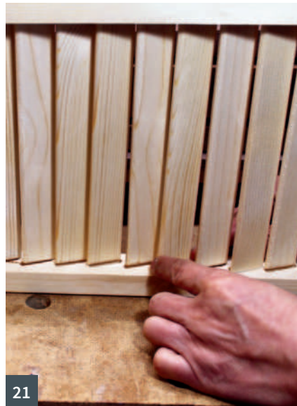
MILLING THE JOINTS: 17 Joining the rails and stiles with a butt joint MAKING THE SLATS: 18 The slats were cut to size 19 Rounding the edges of the slats 20 The edges of the shutter frames can also be rounded ASSEMBLY AND FINISHING: 21 Dry-fitting the slats in the frames 22 Hanging the shutters in place
