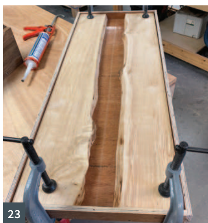
19 Burr elm is cut and planed square and flat to make a lamp 20 Different effects on two resin lamps 21 Yew planks for the river table 22 The finished tables 23 Bigger pieces should be clamped down 24 Removing from the mould
