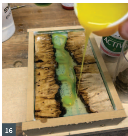
13 Ready-made, reusable, take-apart moulds 14 A homemade mould being put to good use 15 Resin is used to enhance the timber for these pendants 16 Adding yellow pigment to the main pour 17 A selection of cast and cut pendant blanks 18 The two-colour 'Aurora Borealis' effect
