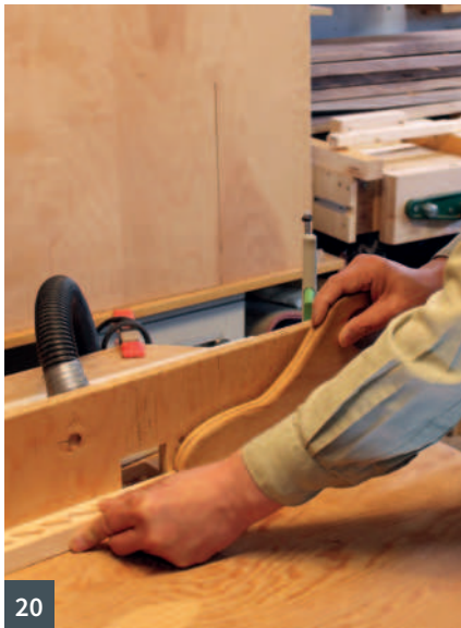
MILLING THE JOINTS: 17 Joining the rails and stiles with a butt joint MAKING THE SLATS: 18 The slats were cut to size 19 Rounding the edges of the slats 20 The edges of the shutter frames can also be rounded ASSEMBLY AND FINISHING: 21 Dry-fitting the slats in the frames 22 Hanging the shutters in place
