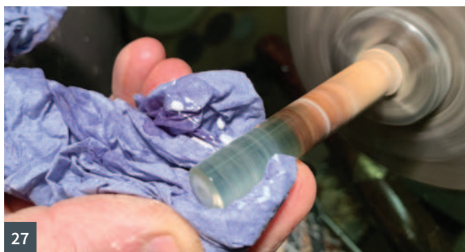
25 Sanding the resin to finish off 26 Polishing resin on a polishing mop 27 Using micro-fine abrasive on the resin with a cloth pad
