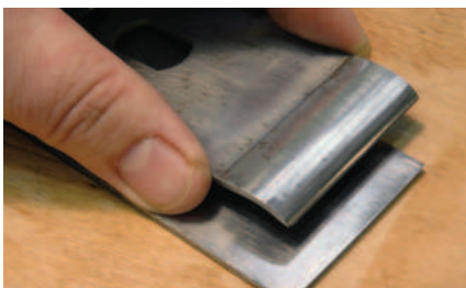
A well set up chipbreaker is essential
