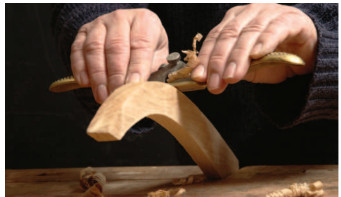
Be careful to plane to the arc when using a spokeshave to smooth a curve
