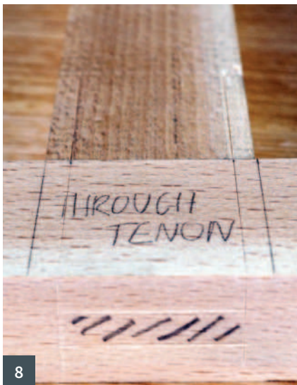
6 ... as the opposing part of the joint 7 A mortise gauge will help to standardise the marking out for this joint 8 Project the mortise width from the tenon component 9 Single crisp knife marks will help with your joinery 10 Gauge marks for a 6mm chamfer all round
