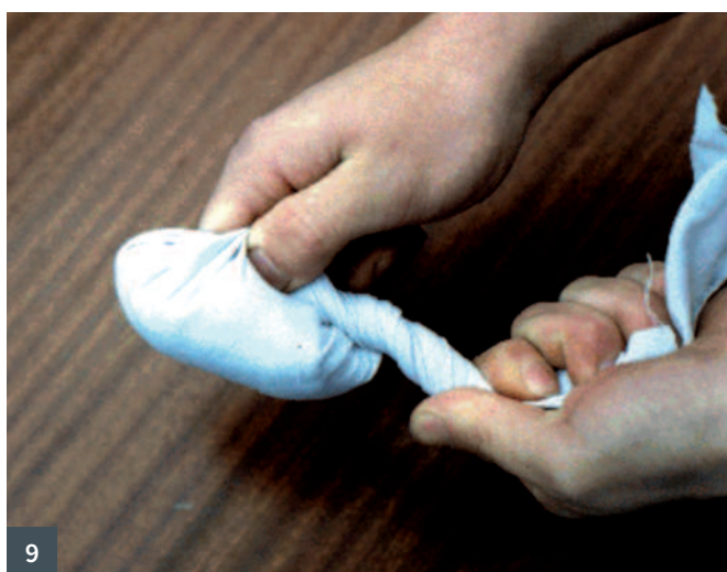
7 Place the fad in the centre of another square of cotton cloth, then move it 25mm closer to a corner, as shown 8 Pull the sides of the outer material up around the fad to cover it 9 Twist the loose material above the fad 10 You have now created a rubber, which should be held as shown here
