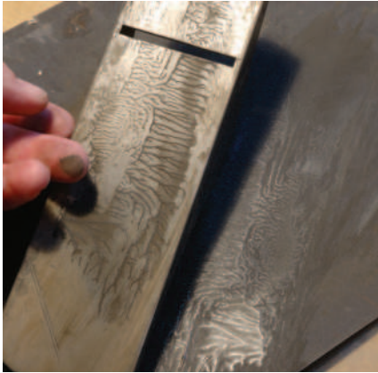
Rub the sole firmly to remove rust
