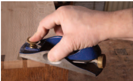
Block planes are ideal for trimming joints
