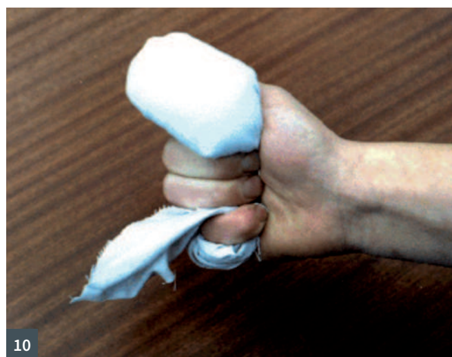
7 Place the fad in the centre of another square of cotton cloth, then move it 25mm closer to a corner, as shown 8 Pull the sides of the outer material up around the fad to cover it 9 Twist the loose material above the fad 10 You have now created a rubber, which should be held as shown here
