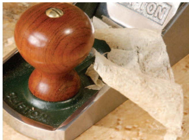
A difference in the thickness of shavings suggests the need for adjustment
