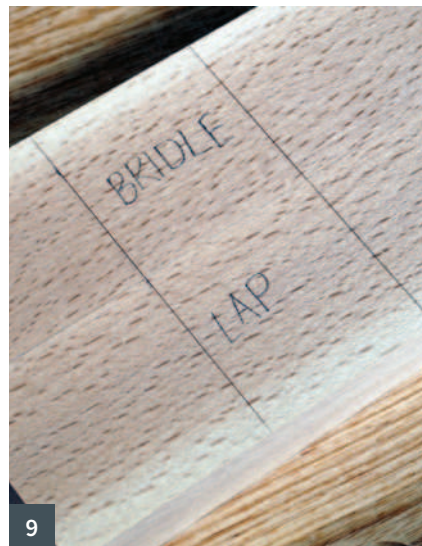
6 ... as the opposing part of the joint 7 A mortise gauge will help to standardise the marking out for this joint 8 Project the mortise width from the tenon component 9 Single crisp knife marks will help with your joinery 10 Gauge marks for a 6mm chamfer all round
