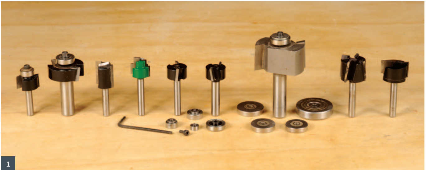
1 Rebate cutters, left-right: 4mm width rebater; 12.7mm width rebater; 19mm dia. straight; 19mm dia. Tonk; 21mm dia. up-shear and 21mm dia. down-shear plus bearings; 50mm dia. multi-bearing rebater with five bearings; 25mm dia. tenoning; 25mm dia. bottom trim
