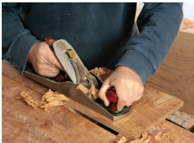
Plane with the grain – look for ‘even’ shavings to confirm this
