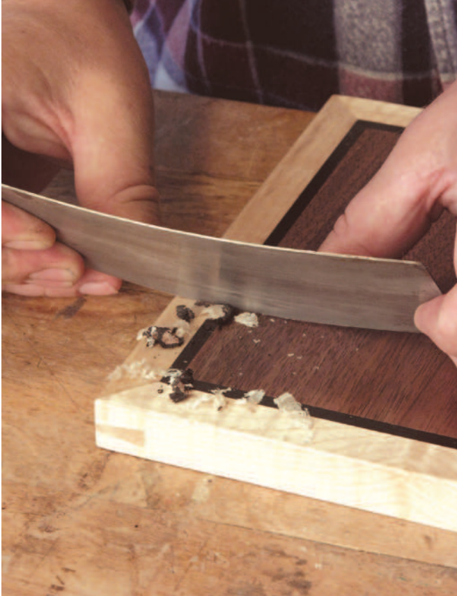
Cabinet scrapers are useful for smoothing difficult surfaces
