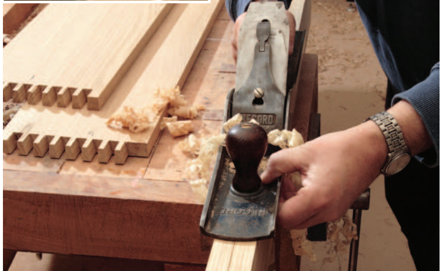
A sharp plane shouldn't need much in the way of downward pressure
