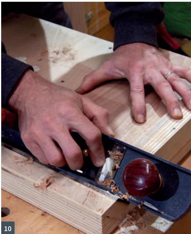
8 Cutting the corner joints by hand instead of using a mitre saw 9 The mitre shooting jig used to create precise joints 10 The jig in use using a No.5 jack plane and a good, sharp blade 11 Biscuit jointing the corners close to the inside edge to avoid breakthrough
