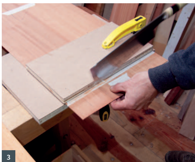
1 The raw materials, blockboard and thick veneers 2 Marking a line along the blockboard to cut to size 3 Sawing cross grain using a board offcut as a saw guide 4 Using a block plane to obtain a clean straight edge
