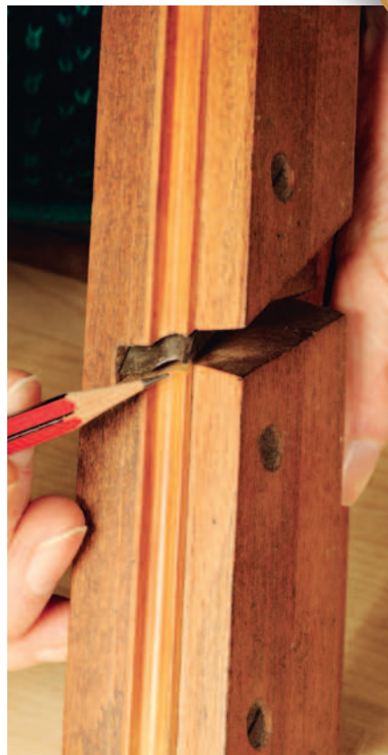
The mouth of this beech moulding plane is still crisp and has plenty of life left in it
