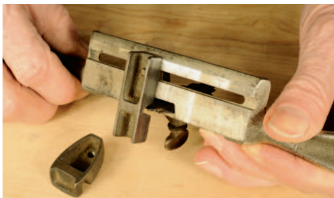
The blades are interchangeable and can be set against a choice of two fences
