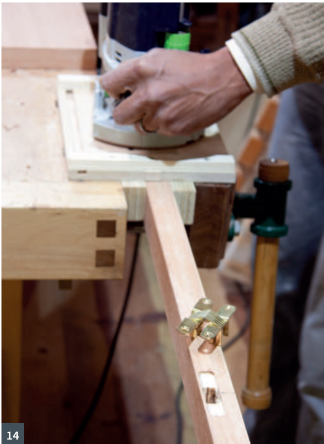
12 Applying a finish to the bottom panel prior to assembly 13 The carcass glued and clamped and then allowed to cure 14 Machining the slots for the recessed hinge mechanism 15 Biscuit slots are needed on three sides for the lid frame
