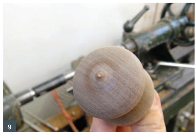
8 Parting off with the spindle gouge 9 A small nib can be pared off and sanded smooth
