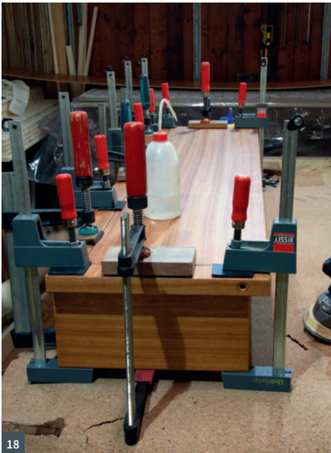
16 The frame in position and working out the locking dowel placement 17 Shaping the knob end of the dowel resting against a stop 18 The frame glued and clamped on to the carcass, note the dowel hole
