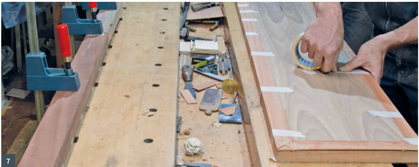
5 Edging a board with the same material, using PVA glue 6 Marking and laying the border veneer. Note the perforated veneer tape 7 Taping the whole veneer assembly together
