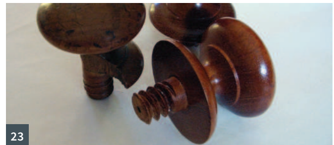
17 Cleaning the face 18 Sanding 19 The difference between the cross grain (top) and end grain (bottom) knobs 20 Fixing methods for knobs and pulls 21 The wedged tenon before fitting 22 Cross section of a wedged tenon fixing 23 Replacement threaded knobs
