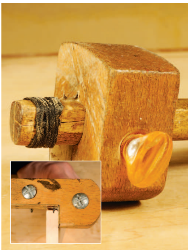
These two homemade scratch stocks are perfectly serviceable and won't cost the earth to make
