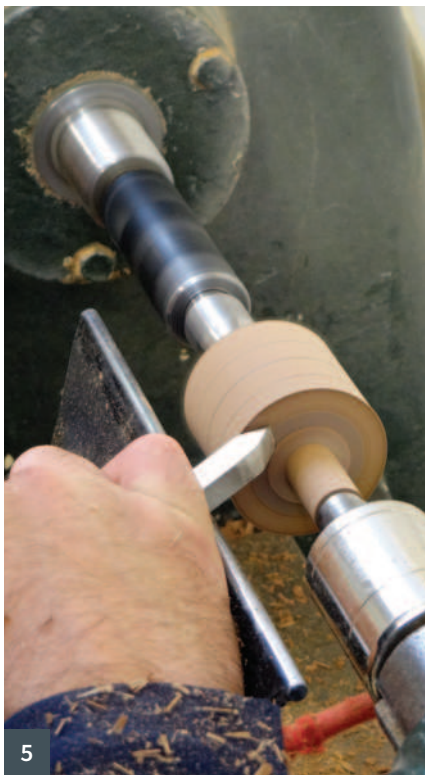
5 Slicing the base of the knob to form a clean undercut 6 Shaping the knob 7 Forming the narrow cove
