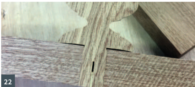
17 Cleaning the face 18 Sanding 19 The difference between the cross grain (top) and end grain (bottom) knobs 20 Fixing methods for knobs and pulls 21 The wedged tenon before fitting 22 Cross section of a wedged tenon fixing 23 Replacement threaded knobs
