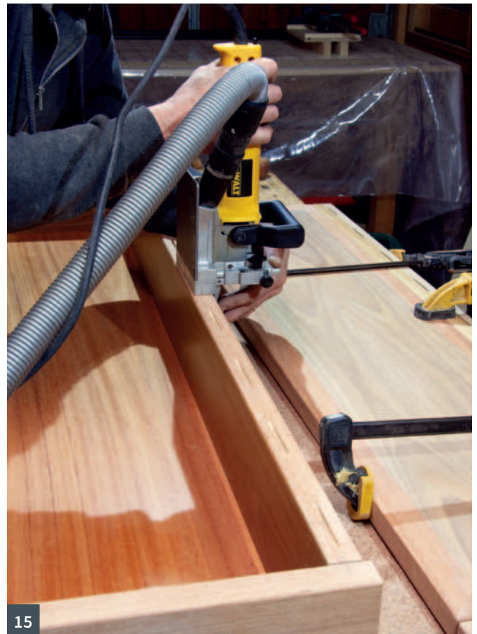
12 Applying a finish to the bottom panel prior to assembly 13 The carcass glued and clamped and then allowed to cure 14 Machining the slots for the recessed hinge mechanism 15 Biscuit slots are needed on three sides for the lid frame
