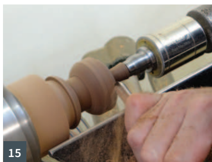
10 Cross grain knob mounted on the screw chuck 11 The cross-grain knob and screw chuck, showing the spacer block 12 Roughing out with the spindle gouge 13 Sizing the fillet with a scraping cut 14–16 The shaping process of the cross grain knob with the wing of the spindle gouge
