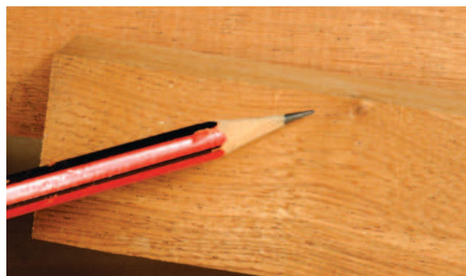
Even a pip like this can throw you off course when running beads by hand
