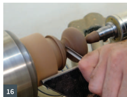
10 Cross grain knob mounted on the screw chuck 11 The cross-grain knob and screw chuck, showing the spacer block 12 Roughing out with the spindle gouge 13 Sizing the fillet with a scraping cut 14–16 The shaping process of the cross grain knob with the wing of the spindle gouge
