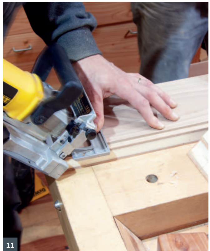
8 Cutting the corner joints by hand instead of using a mitre saw 9 The mitre shooting jig used to create precise joints 10 The jig in use using a No.5 jack plane and a good, sharp blade 11 Biscuit jointing the corners close to the inside edge to avoid breakthrough
