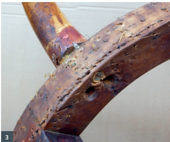
3 Screws and dowels through the seat rails and into the arm upright
