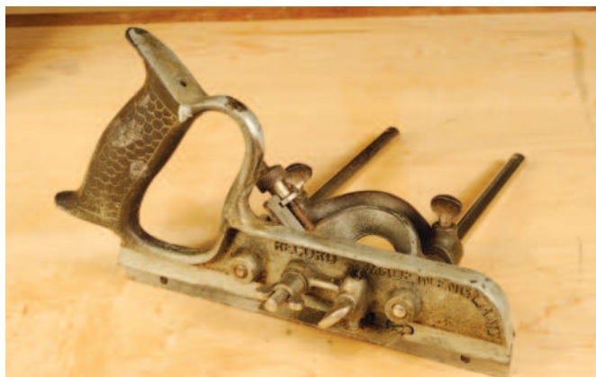
This Record 45S first appeared in the 1938 catalogue and is the same as the Stanley 45 with the addition of a simple screw adjustment added to the cutter blade
