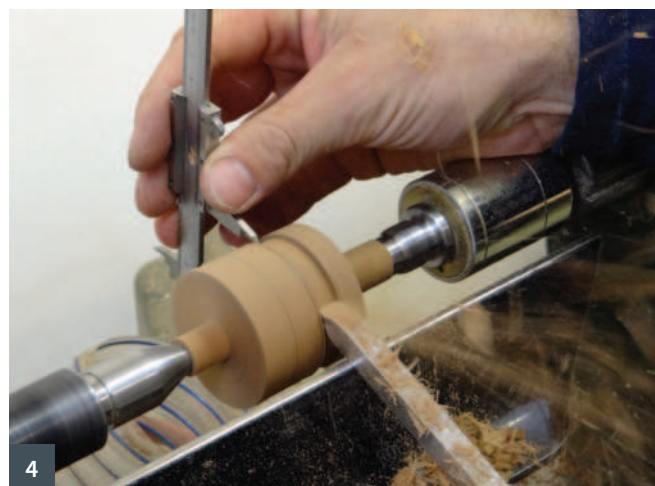
1 Almost any screw can be used to make a screw chuck 2 The screw chuck ready for action 3 Marking out with a story board 4 Sizing the fillets
