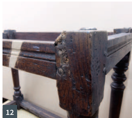
7 The new infill being fitted to the stretcher 8 Carving in the moulded profile 9 Strengthening dowels through the broken joint area on the leg 10 The first stage of forming the new tapered pegs 11 Tapering the pegs to match the existing ones and the holes 12 The stretcher and pegs fitted and the pegs squared off just proud of the frame 13 One of the cleats being removed from the leaf 14 Drilling the cleat for the replacement pegs 15 The bearer rails fitted in position
