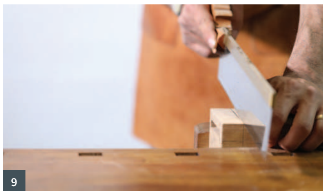
7 The base with the hole cut out 8 Mortising the block by the mortiser machine 9 Cutting out the cantilever by the crosscut saw 10 Cutting out the inside of the lamp hole with the drill press for better access
