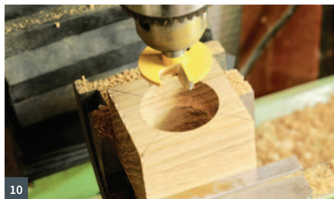
7 The base with the hole cut out 8 Mortising the block by the mortiser machine 9 Cutting out the cantilever by the crosscut saw 10 Cutting out the inside of the lamp hole with the drill press for better access
