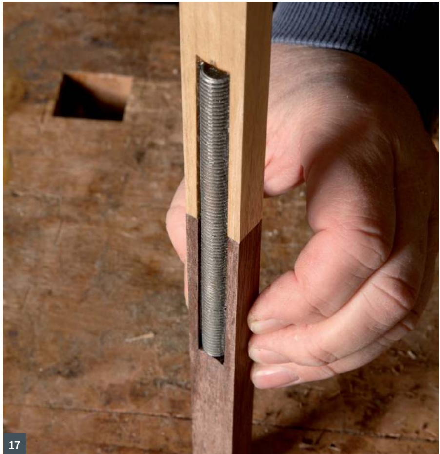
17 More in common with bone implants than conventional woodworking, a steel rod is set in epoxy resin to produce this strong joint in a fine-section leg
