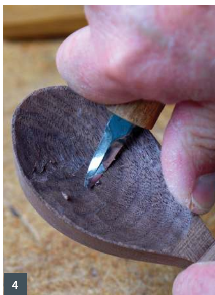
1 Mark out the shape of the spoon 2 Blank marked and ready to cut 3 Starting to shape the bowl of the spoon 4 A curved knife or a curve-bladed gouge will help refine the inside shape 5 Abrasives help refine the surface if you are after a smooth feel 6 The difference between a tool and sanded finish
