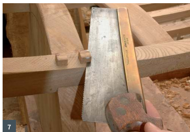
7 Pegged mortise and tenons on country furniture are resistant to glue failure in damp conditions
