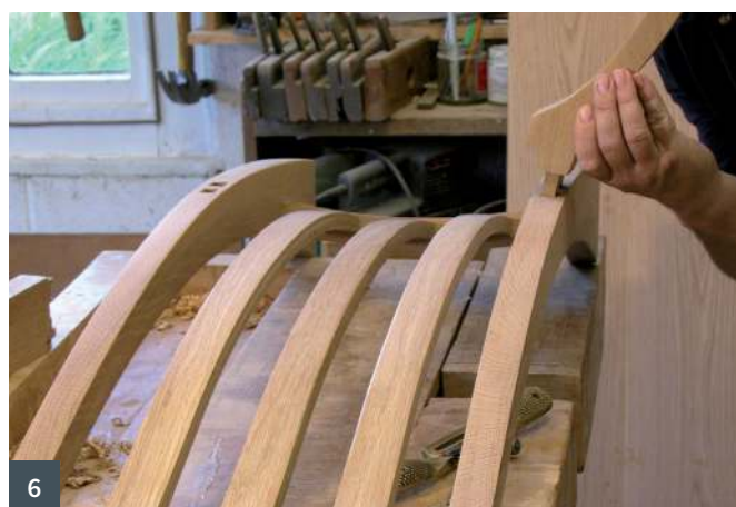
6 Twin tenons have the advantage of offering extra mechanical strength against racking
