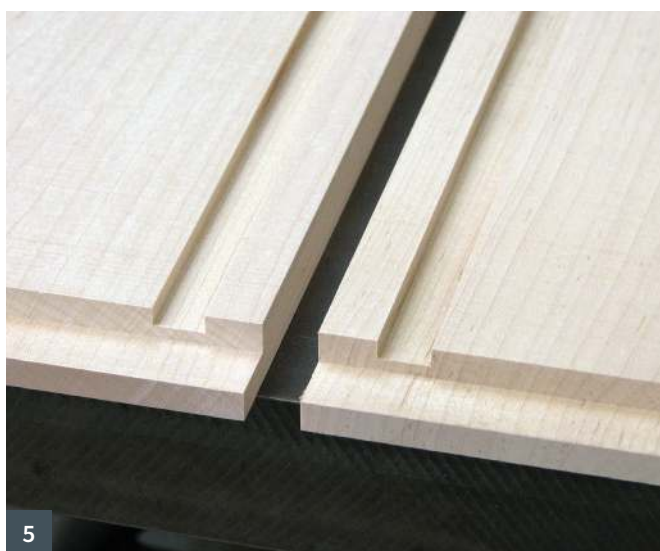
2 Four drawers need replacing, two on each side of the kitchen, plus two faux drawers in front of the sink 3 Cutting the rabbet joints at the front of the drawers with a dado set and sacrificial fence 4 Dado joints at the back of the drawer are cut in a similar manner 5 Grooves for the drawer bottoms run right through the rabbetted area 6 Four clamps complete the glue-up. No need to insert the drawer bottom yet
