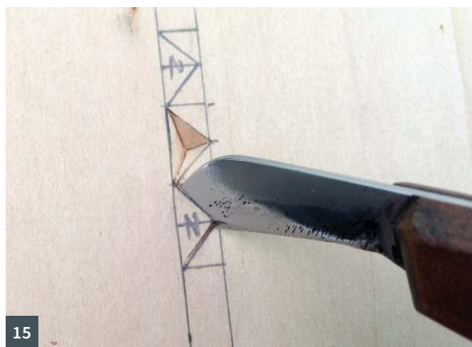
14 The three cuts to release the chip: cut 1 15 Cut 2 16 Cut 3
