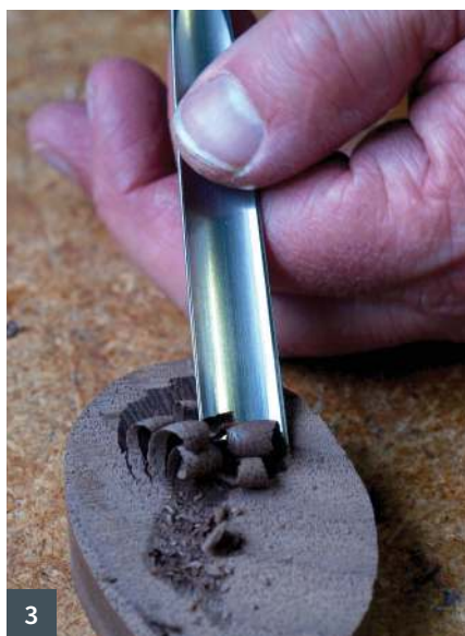
1 Mark out the shape of the spoon 2 Blank marked and ready to cut 3 Starting to shape the bowl of the spoon 4 A curved knife or a curve-bladed gouge will help refine the inside shape 5 Abrasives help refine the surface if you are after a smooth feel 6 The difference between a tool and sanded finish
