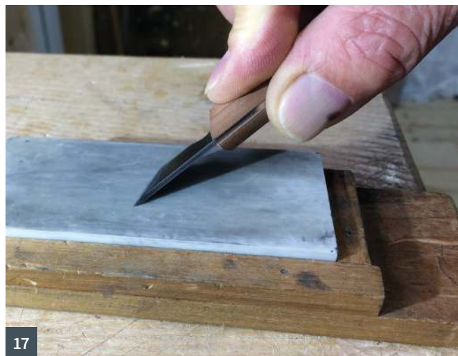
17 Sharpening the stab knife at 30° each side 18 Using the stab knife
