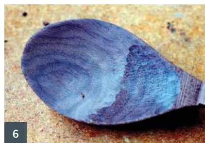
1 Mark out the shape of the spoon 2 Blank marked and ready to cut 3 Starting to shape the bowl of the spoon 4 A curved knife or a curve-bladed gouge will help refine the inside shape 5 Abrasives help refine the surface if you are after a smooth feel 6 The difference between a tool and sanded finish
