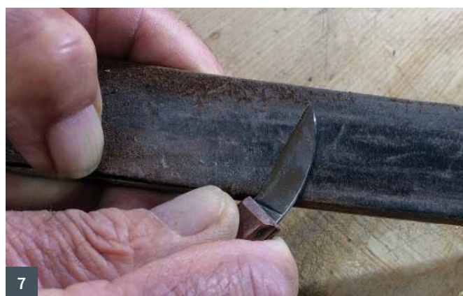
4 Keeping an even pressure on the blade 5 Using a raised block, put your blade flat on the ceramic stone, then raise the back edge no more than 1mm 6 Testing for the burr 7 Stropping a blade 8 Testing the blade sharpness on some wood
