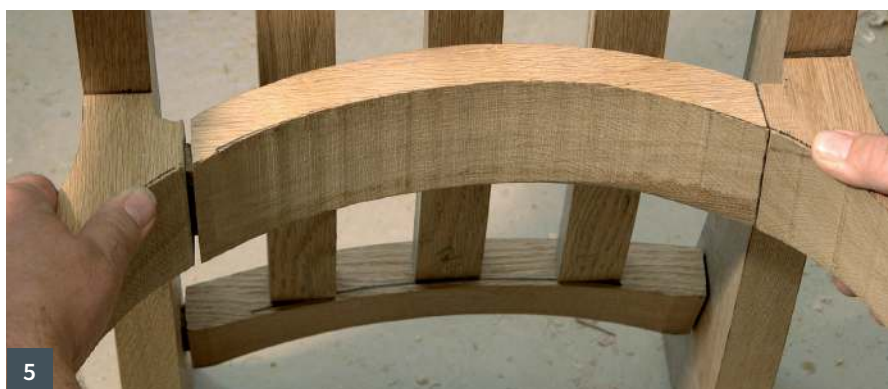
4 The bandsaw produces the cheeks of tenons on a solid seat. The waste is then removed with coping saw and chisel 5 Angled joints, in this case cut on a frame mortise-and-tenon jig, normally use a slanting tenon to fit a straight mortise
