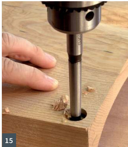
14 Turned ends on legs can produce joints with accuracy for a tight fit 15 Good-quality Forstner bits produce an accurate round mortise hole 16 Carving the finished joint can produce a form that is diverse from the construction
