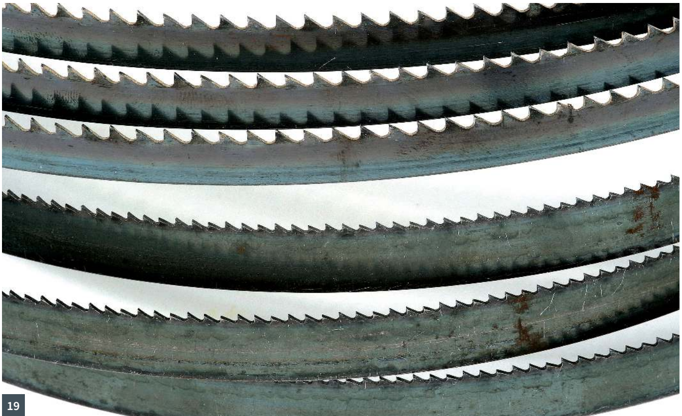
17 Blade width is more important than its thickness 18 The fewer the teeth, the coarser the cut will be 19 Tooth pattern is the determinant for cutting speed and quality
