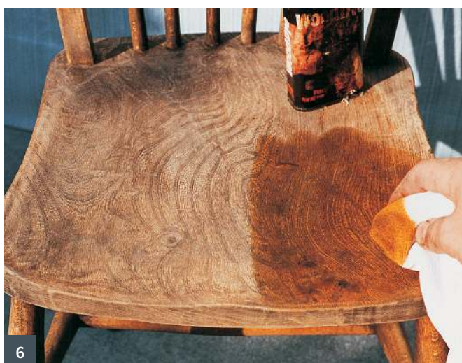
4 Stripping between the spindles 5 Using wire wool to strip the spindles 6 Applying an oil stain to even up the colour of the chair 7 End grain will soak up more stain than the rest of the wood, resulting in dark patches
