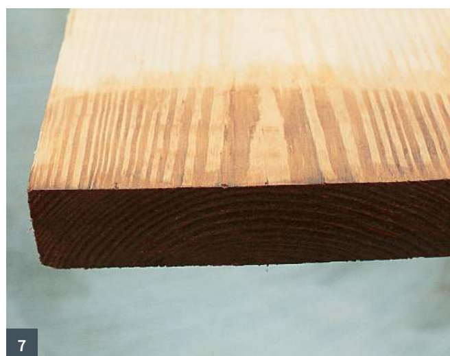
4 Stripping between the spindles 5 Using wire wool to strip the spindles 6 Applying an oil stain to even up the colour of the chair 7 End grain will soak up more stain than the rest of the wood, resulting in dark patches
