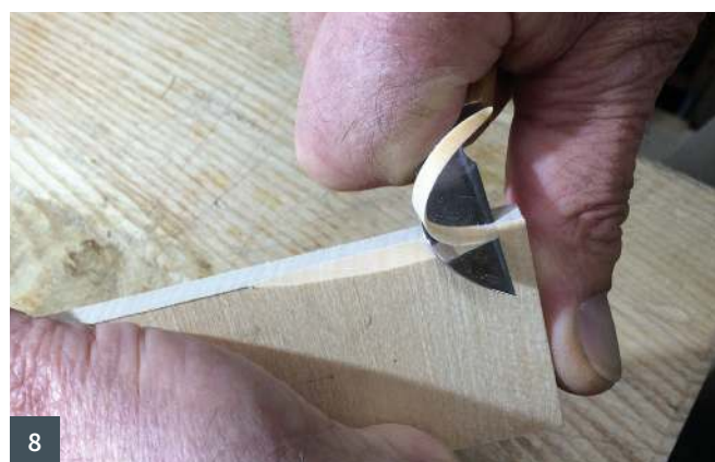
4 Keeping an even pressure on the blade 5 Using a raised block, put your blade flat on the ceramic stone, then raise the back edge no more than 1mm 6 Testing for the burr 7 Stropping a blade 8 Testing the blade sharpness on some wood
