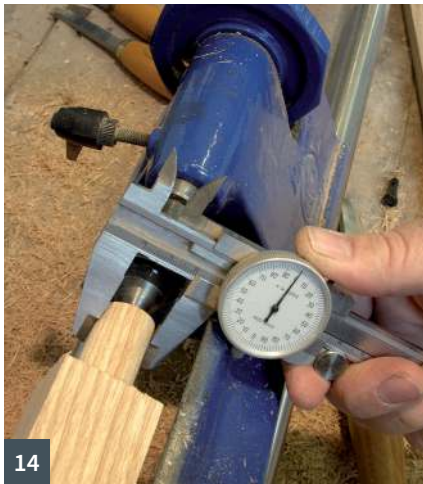
14 Turned ends on legs can produce joints with accuracy for a tight fit 15 Good-quality Forstner bits produce an accurate round mortise hole 16 Carving the finished joint can produce a form that is diverse from the construction
