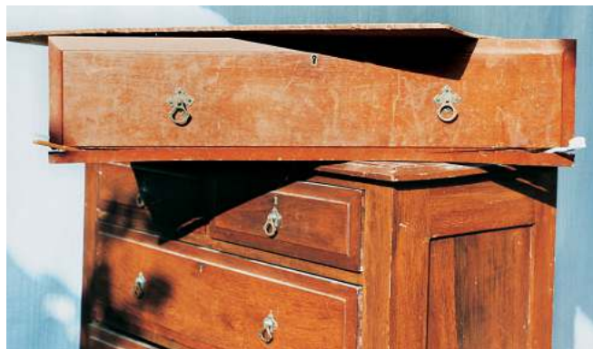
The two big splits in the drawer front
