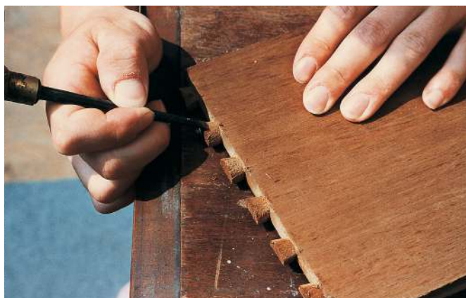
Scraping all the old glue from the joints
