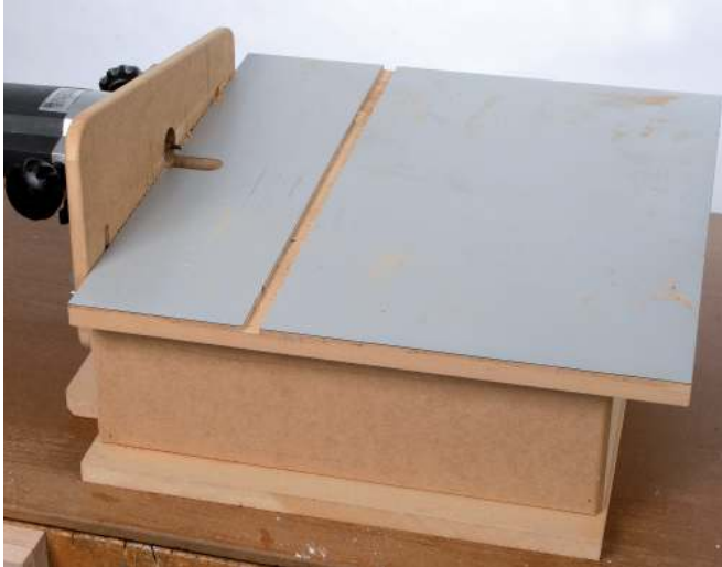
Grooving and jointing work calls for a horizontal routing table
