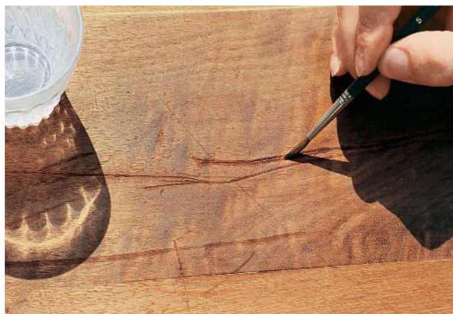
Applying water to the minor dents to 're-inflate' the wood fibres
