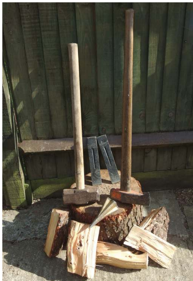
Clockwise from top: two splitting wedges, a splitting maul, a 'log grenade' and a sledgehammer
