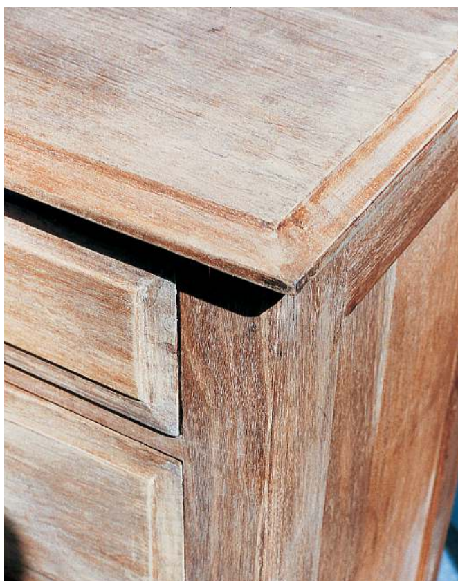
The surface of the wood after stripping
