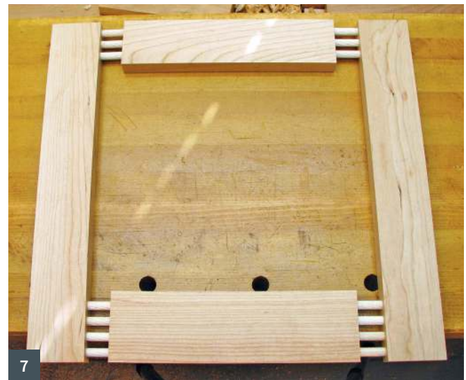
3 Detail of the frames, glazing and handles 4 Karelian birch veneer is incredibly beautiful and light in colour 5 Using a precision Dowelmax jig to create the frame joints 6 Using a rose countersink to ease the dowel entry 7 A dry alignment check of the dowel joints
