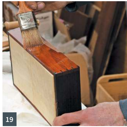
18 Sanding the long sides of the box after flushing the aluminium pins 19 The last oil finishing on the long sides 20 Fitting the base with four micro screws was followed by applying four rubber dots on top of the screws, which will allow the box to stay a little bit raised
