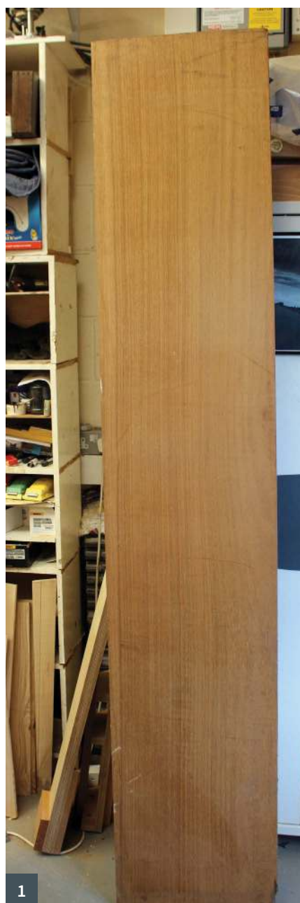
1 A large board of Iroko 2.5m long x 405mm wide x 50mm thick 2 All the parts planed and cut to length 3 Square hole, cut on the tablesaw, to take the 12mm threaded bar 4 Dominoes were used at each end for alignment 5 Gluing up the top with plenty of clamps
