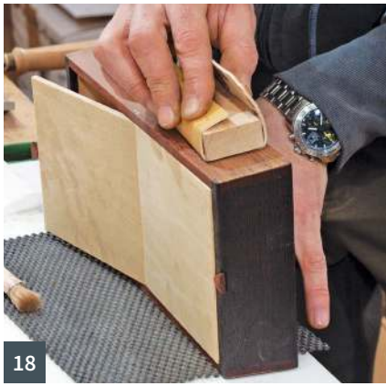
18 Sanding the long sides of the box after flushing the aluminium pins 19 The last oil finishing on the long sides 20 Fitting the base with four micro screws was followed by applying four rubber dots on top of the screws, which will allow the box to stay a little bit raised
