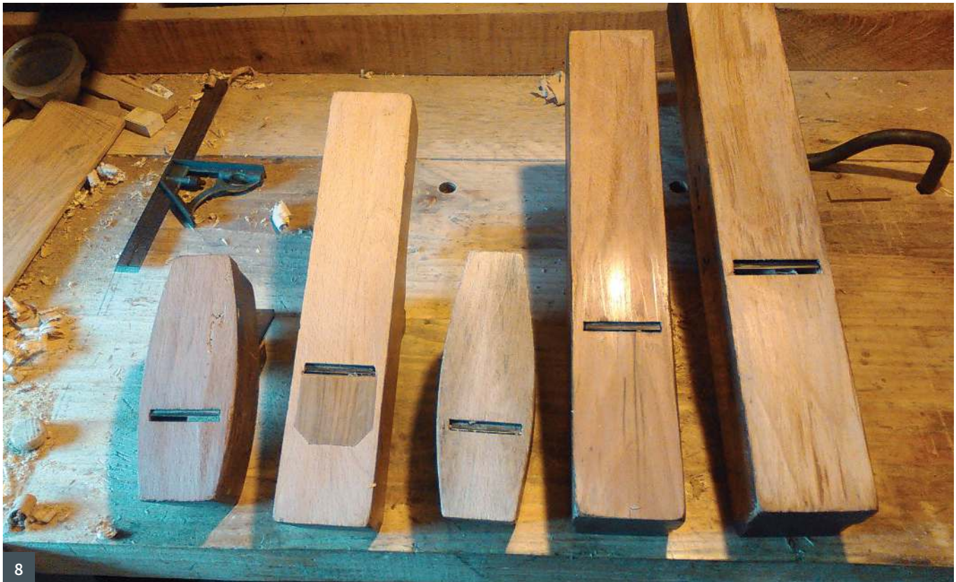
8 A variety of planes used to create different levels of finish
