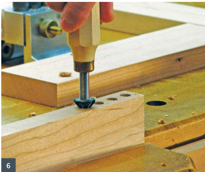
3 Detail of the frames, glazing and handles 4 Karelian birch veneer is incredibly beautiful and light in colour 5 Using a precision Dowelmax jig to create the frame joints 6 Using a rose countersink to ease the dowel entry 7 A dry alignment check of the dowel joints
