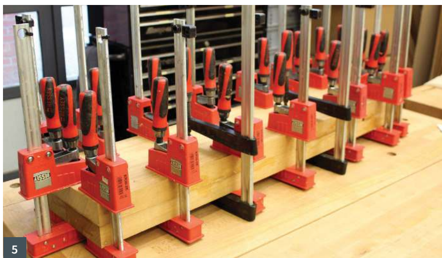
1 A large board of Iroko 2.5m long x 405mm wide x 50mm thick 2 All the parts planed and cut to length 3 Square hole, cut on the tablesaw, to take the 12mm threaded bar 4 Dominoes were used at each end for alignment 5 Gluing up the top with plenty of clamps
