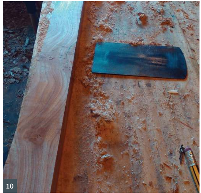
A card scraper produces a higher level of finish
