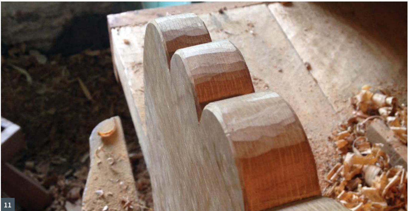
The faceted effect created with a chisel
