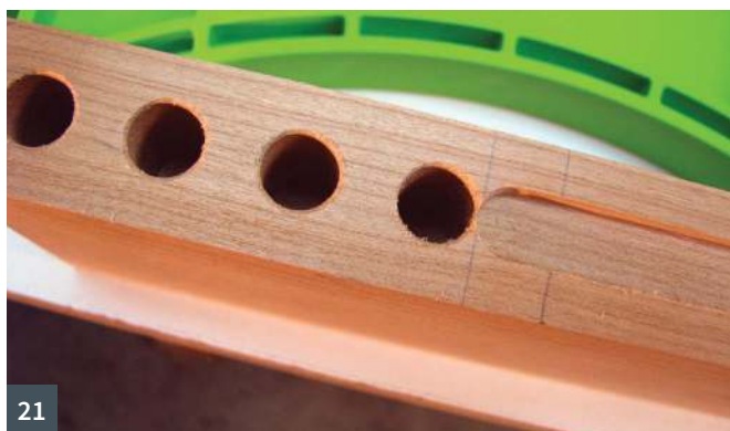
16 Setting up to machine the panel slots in the stiles and rails 17 Using removable shims to increase the slot width 18 The shims removed for a second widening pass 19 The finished slots are shallow as the plywood panels will not shrink 20 The stiles need a drop-on, lift-off method to avoid slotting the joint areas 21 Slot overrun so the panel will fit in properly 22 Checking the panel fit next to the dowel joint
