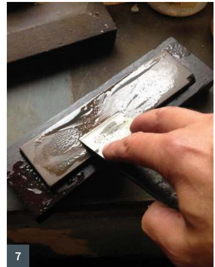
7 Creating a cambered blade profile
