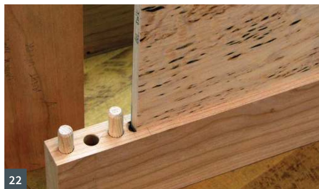
16 Setting up to machine the panel slots in the stiles and rails 17 Using removable shims to increase the slot width 18 The shims removed for a second widening pass 19 The finished slots are shallow as the plywood panels will not shrink 20 The stiles need a drop-on, lift-off method to avoid slotting the joint areas 21 Slot overrun so the panel will fit in properly 22 Checking the panel fit next to the dowel joint
