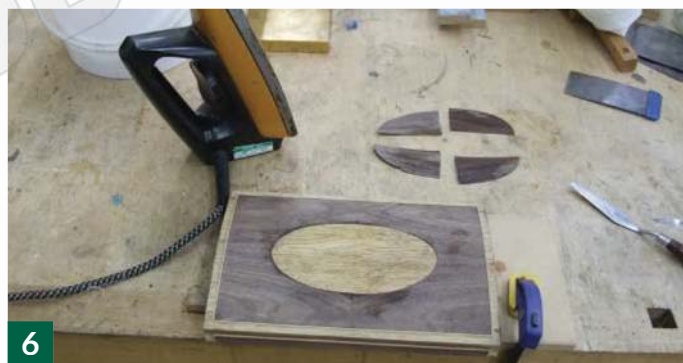
Marquetry based on Mieczyslaw Piotrowski's drawing is glued on top of the lid
