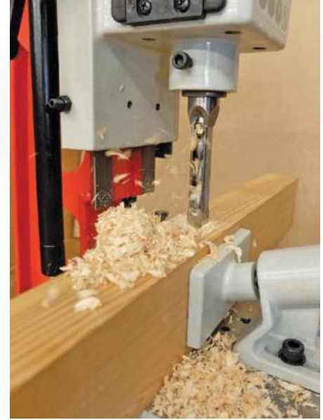
The Japanese chisel cut cleanly and easily
