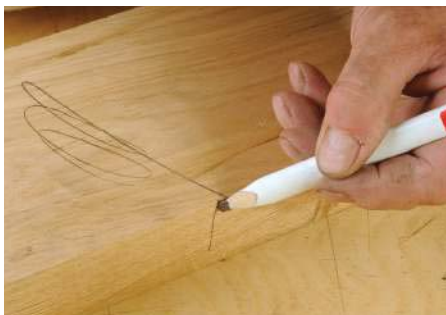
Using a precision grip to make face and edge marks
