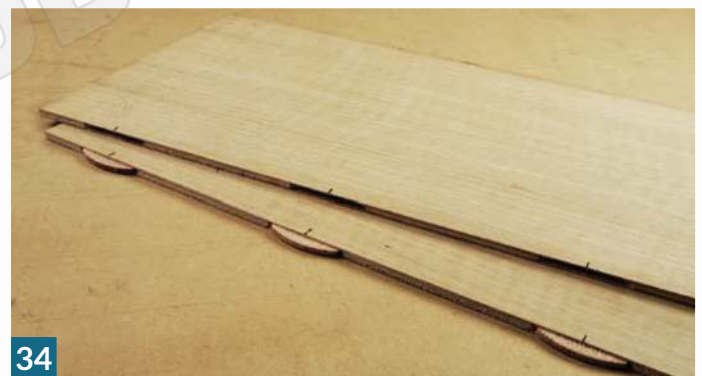
9mm veneered ply being extended widthwise using carefully placed biscuits
