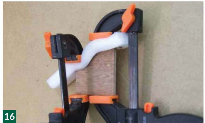
The edges of the pigeonhole dividers were veneered as well
