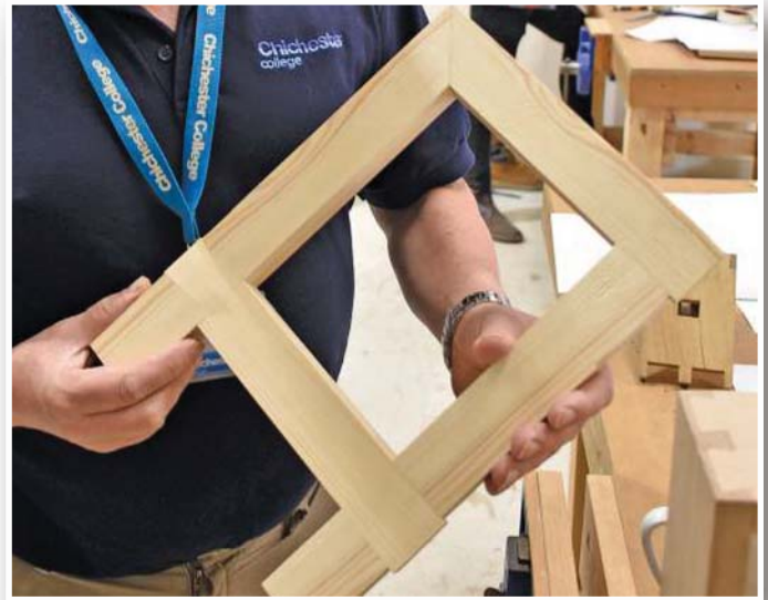
How a neatly finished joint frame should look when done correctly
