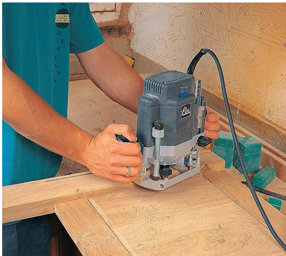
Routing internal chamfer on leg
