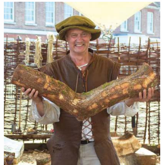
For maximum strength, naturally L shaped pieces of timber are used to make a boat's knees
