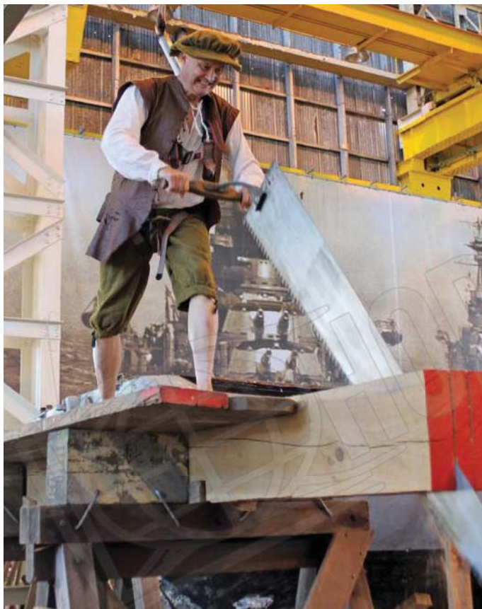
A two-man pit saw being used to cut through a squared off log
