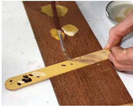
Using light brush strokes in a diagonal direction to blend the colours using sanding sealer
