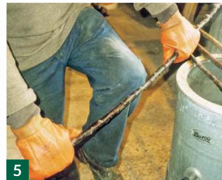
Flex the heated stick gently over your knee to straighten it
