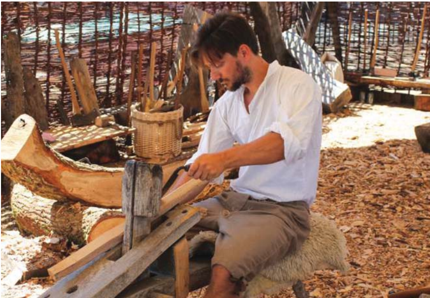
Working with a drawknife on a shaving horse
