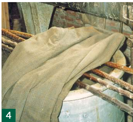
For heating a number of sticks, a water boiler is ideal. A draped coat will concentrate the heat where you want it
