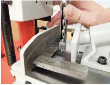
Making sure the chisel is square to the fence
