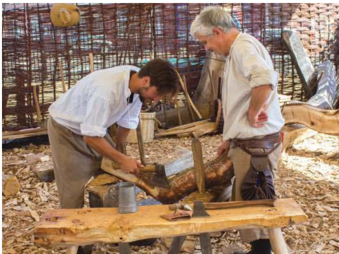
Using a hand axe to transform a naturally L shaped piece of wood into a knee for fitting in a boat
