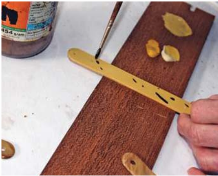
Applying the spots and streaks of each colour to match the original handle
