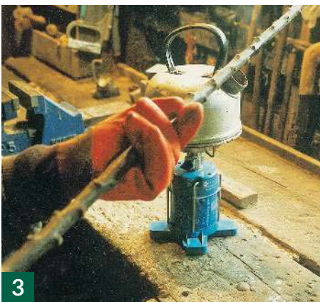
The steam from a kettle is sufficient to heat a single stick
