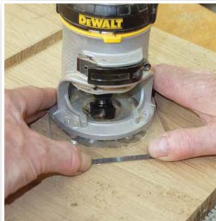
A swap-body router can allow different ways of working from freehand...
