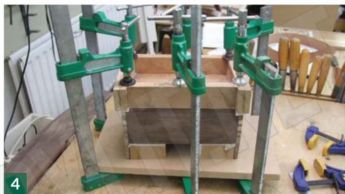
The laminated lid was glued on to the case and held in place with clamps
