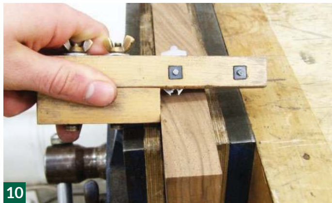
Mouldings were made with a scratch stock...
