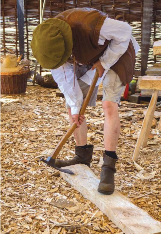
Taking careful aim with an adze to level a piece of timber
