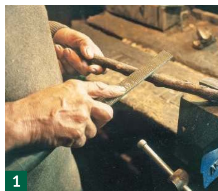
Smoothing down the knots left after trimming
