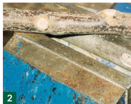
Do not file the knots flat – they should be left nicely rounded
