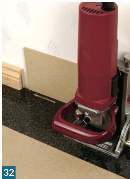
A packer behind the jointer ensures the slots avoid a slight gap at the back of the worktop
