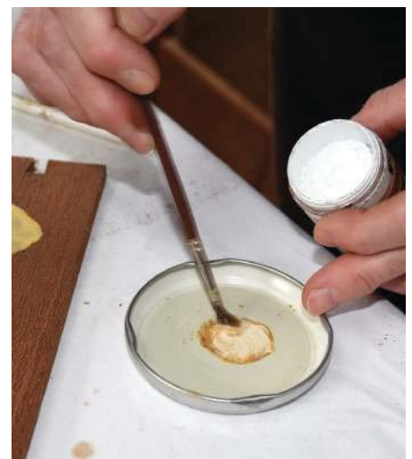
Mixing the flake white with a little yellow ochre and sanding sealer
