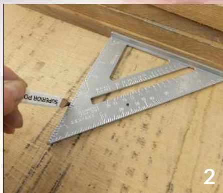
A Speed square is really handy for rough marking out with its raised edge
