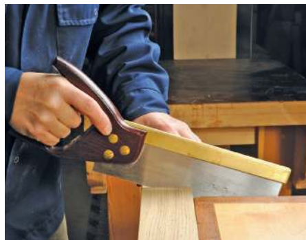
Continue to cut while holding the waste piece to avoid breakage
