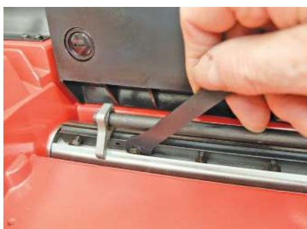
Tightening up a bolt holding a blade. Note the height-setting jig
