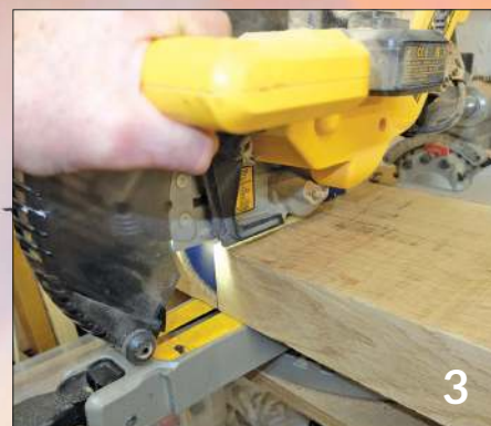
Cut depth at maximum on the compound mitre saw with a top-quality blade
