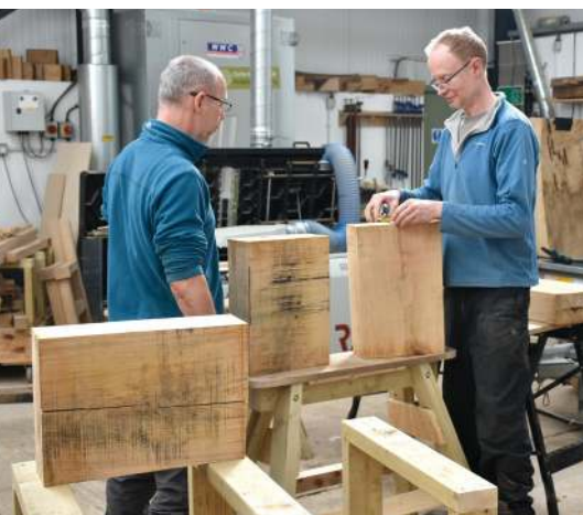
Legs for a heavy, oak garden bench being readied for thicknessing
