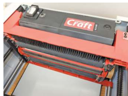
The anti-kickback pawls, rubber drive rollers and the cutter block
