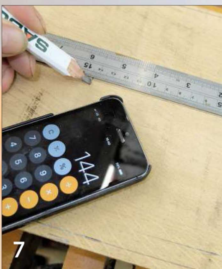
7 Attempting to work out key datum points for the crest rail curvature
