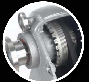
Heavy-duty spindle lock and 24 point indexing
