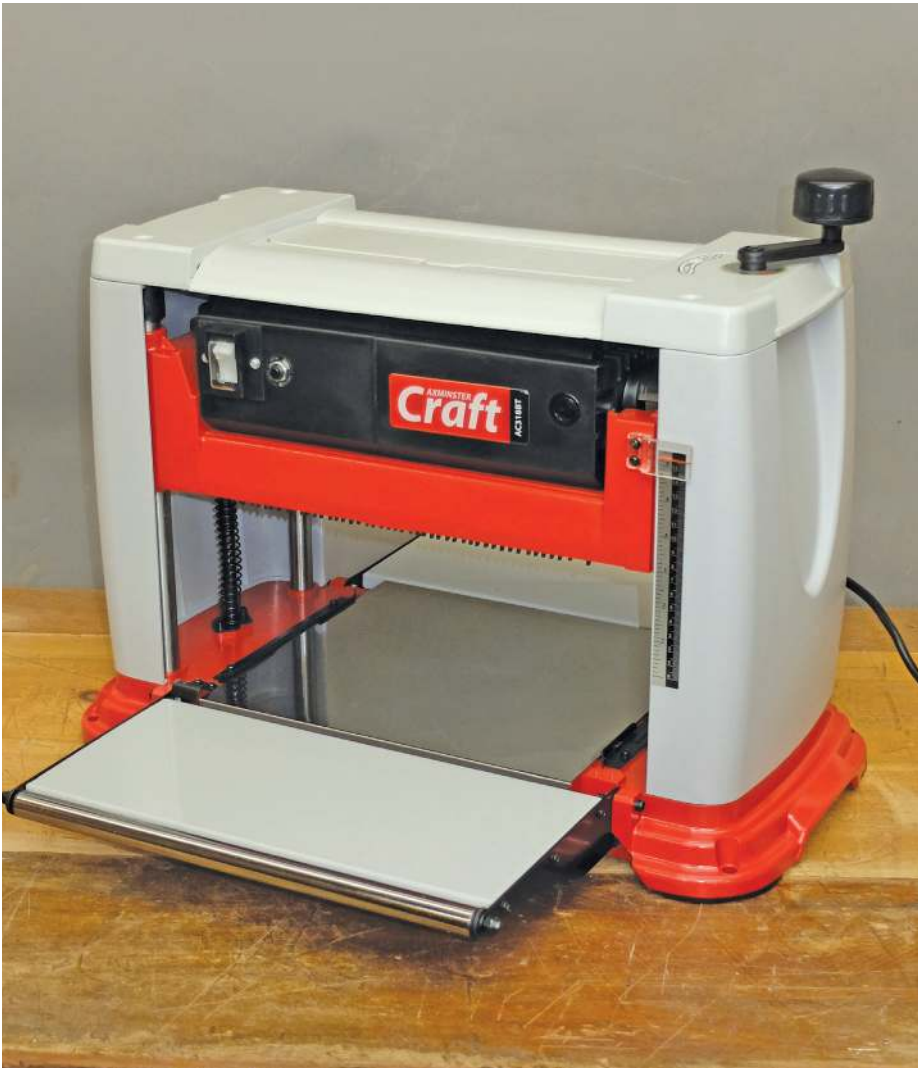
Checking how level the beds and rollers are to each other
