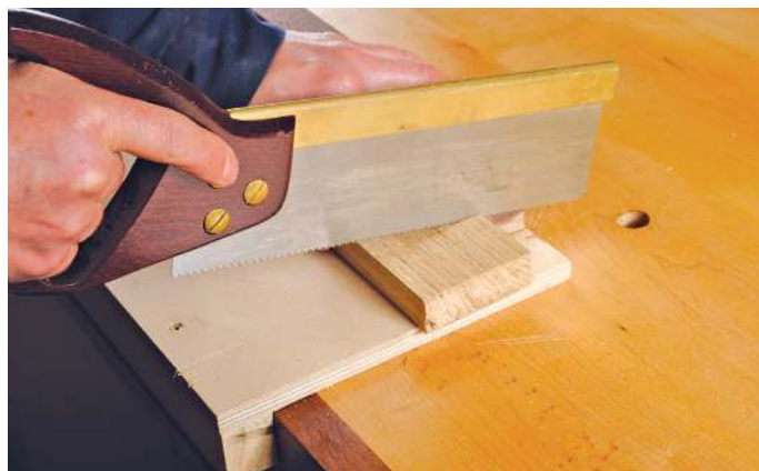
Pull the saw backwards to graze the wood and start the kerf
