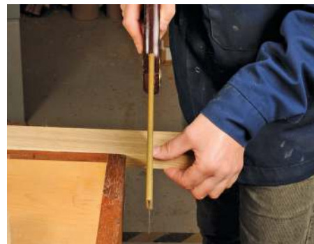
Sight along the 'good' side to make sure you follow the pencil lines
