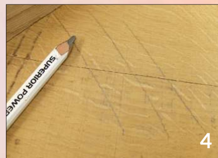
Each split board had different marking to allow quick re-matching together
