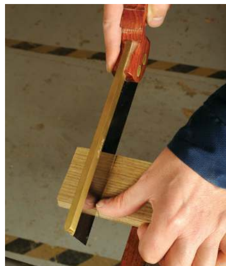
Use your thumb as guidance but above the tooth line to avoid injury
