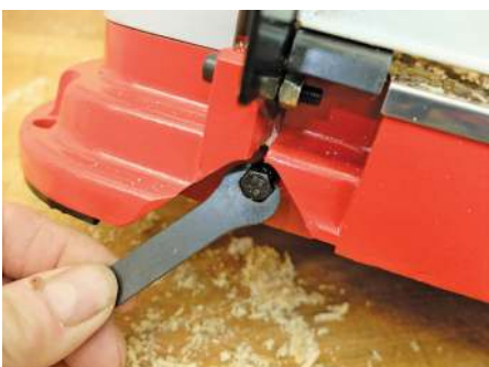
One of the bed adjusting bolts – very easy to alter the height
