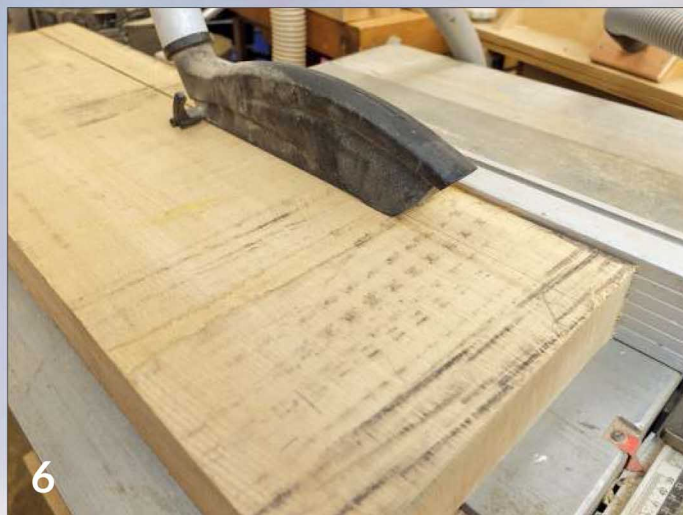
6 Cutting the initial rectangle needed to cut out the crest rail running at maximum cut depth (blade stationary for photo)
