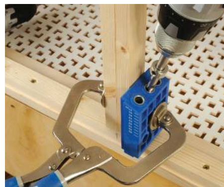
Just one of the methods for securing a butt joint easily
