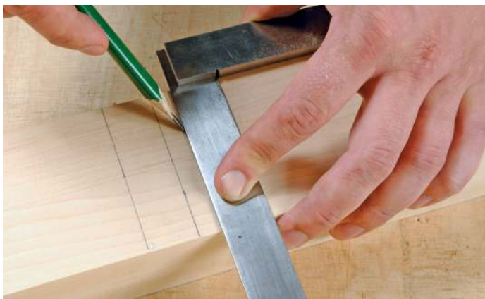
Always mark all around the workpiece so you can see where to cut
