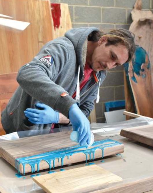
Creating a resin infill chopping board to be sanded and polished when the resin cures
