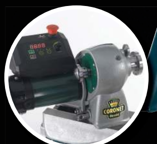
Rotating headstock features accurate angle stops and can swivel 360°
