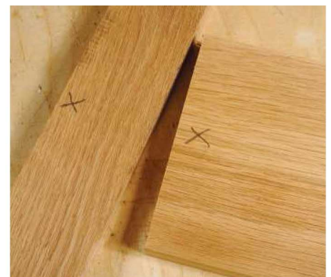
Marked-up oak framing ready to be butt jointed
