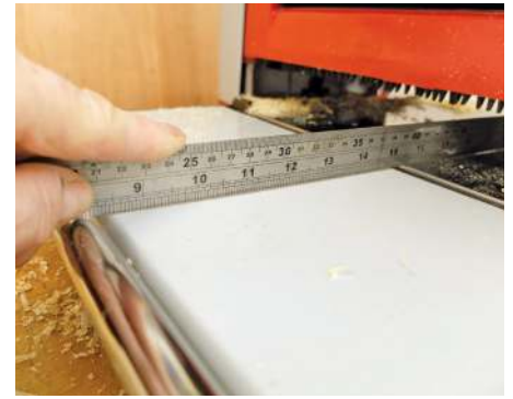
Checking how level the beds and rollers are to each other
