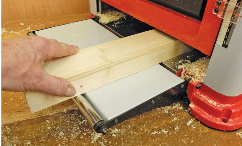
First a piece of softwood for a trial cut with rather a lot of chippings
