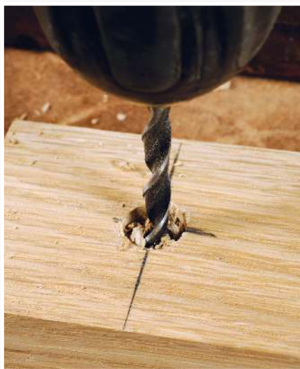
Shallow drill for the bolt head first, then drill right through for the bolt hole
