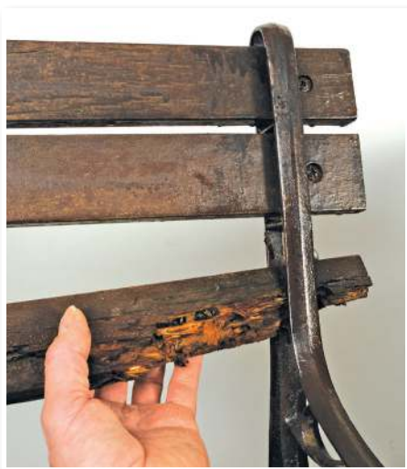
A slat with rot which has been hidden for years by the thick exterior coating
