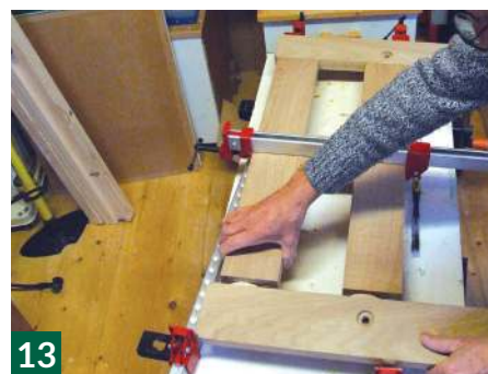
13 Join the legs and cramp to set. Add the side attachments and the supporting blocks
