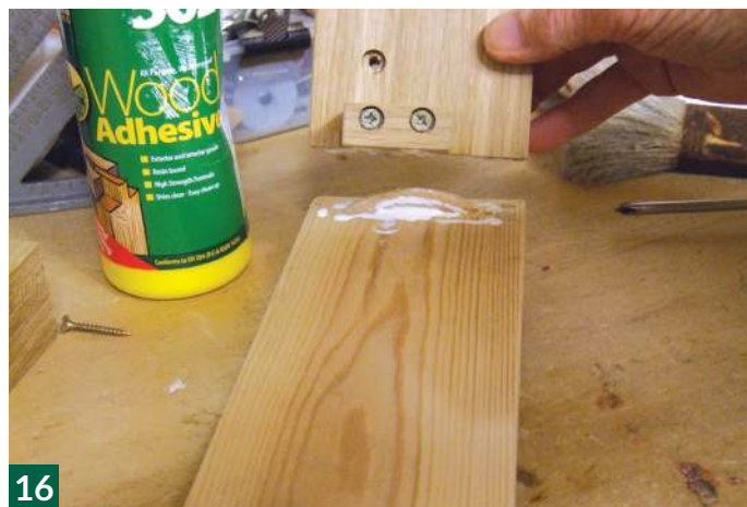
16 Attach to the end of the side rail using a size 20 jointing biscuit and adhesive. Repeat for other ends
