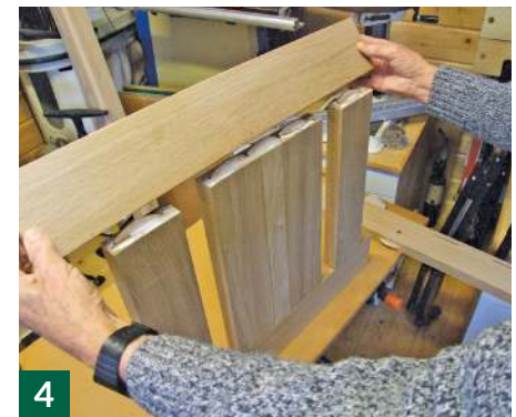
4 Using adhesive and size 20 biscuits, join the top rail to the infill pieces. Repeat with the bottom rail
