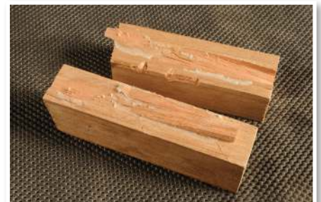
This wood broke because the hot-melt glue was very hot when first applied
