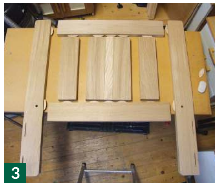
3 Mark and cut matching biscuit slots to join the top and bottom rails to the infill pieces and to the legs. Dry-fit to check
