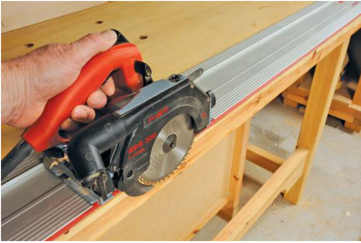
A small, dedicated guide rail saw
