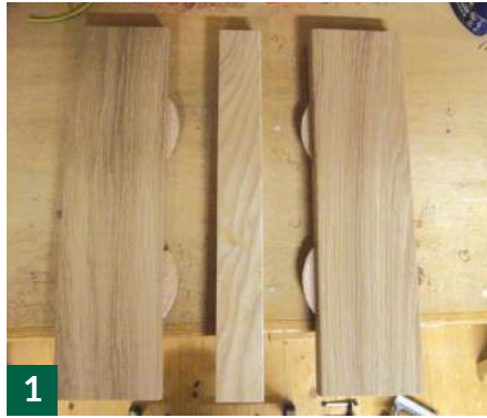
1 Mark matching jointing biscuit slot positions. Cut slots and dry-fit to check
