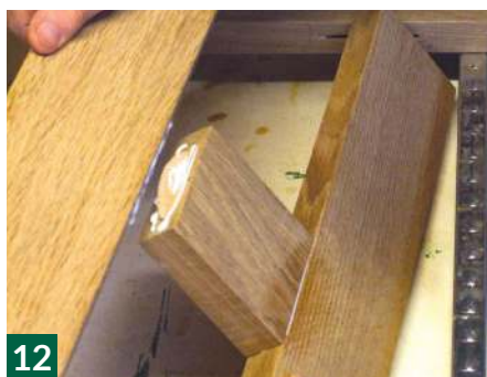
12 Use jointing biscuits and adhesive to join the centre infill to the top and bottom rails
