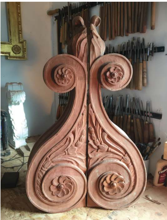
Sapele corbel brackets (800mm long) to support the porch over the front door, part of the restoration of Clinton Lodge, E.Sussex
