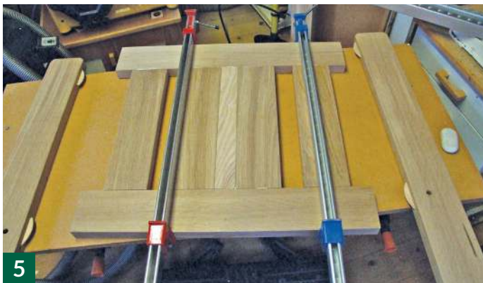
5 Cramp the assembly ensuring that the ends of the rails line up
