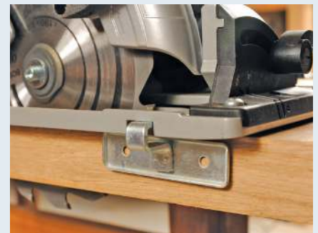
Always use a fence or guide rail
