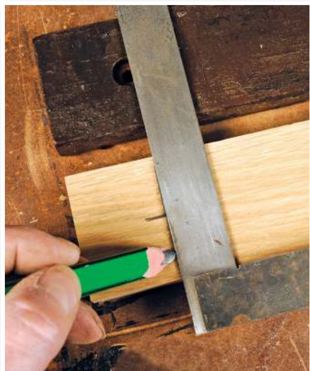
Use an existing slat to mark the bolt hole positions so they all match
