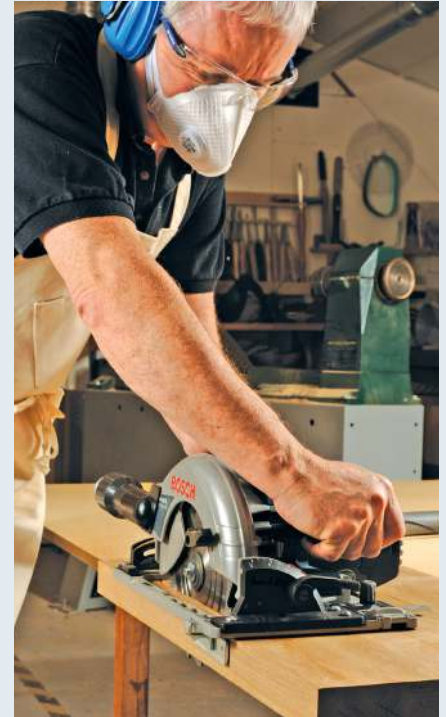
Wear PPE and stand to the side of the saw
