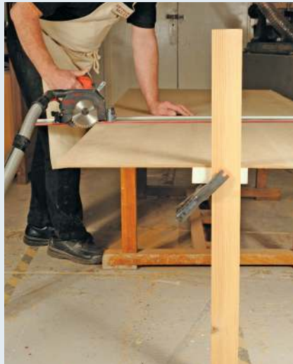
The support leg falls away when the cut is finished
