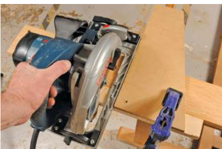
A homemade T-square makes cross-cuts easy
