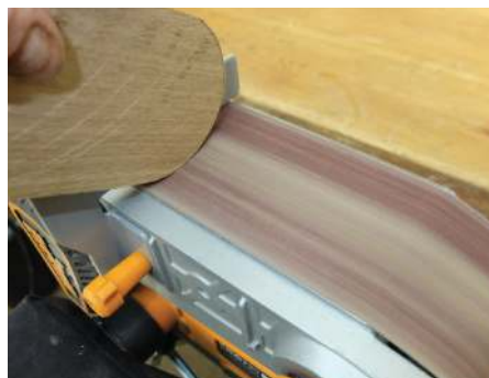
Static inverted sanding
