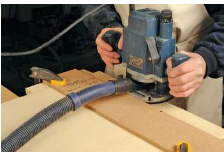
If the cut is too rough then clean up with a router afterwards
