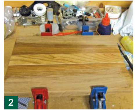
2 Apply adhesive to the biscuits and join the pieces together. Ensure that the edges are accurately lined up and cramp to set
