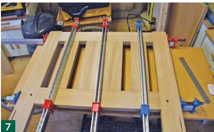
7 Attach the legs with size 20 biscuits and adhesive and cramp to set
