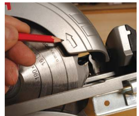
The arrow indicates tooth and cut direction
