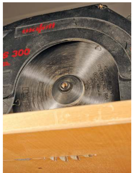
The teeth should just project when cutting faced board
