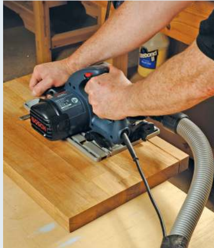
Keep the lead and trail hose out of the way
