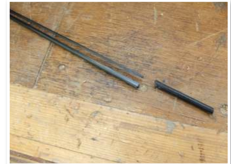
The rod failed spectacularly – note how the long section has split apart
