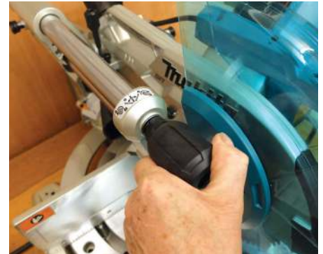
The ratchet-action bevel locking knob
