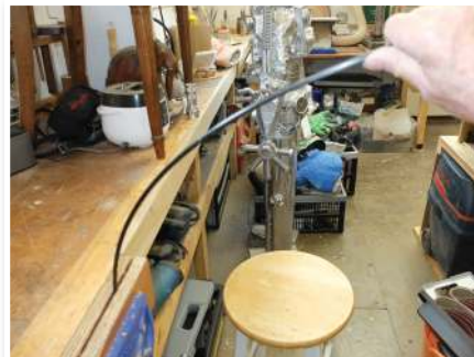
My stress test got this 6mm dia. rod to a 90° bend before breaking
