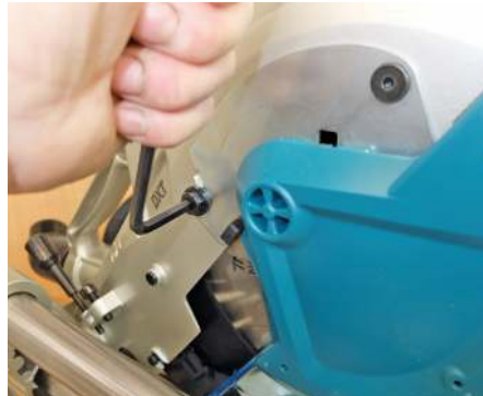
Tightening the bolt holding the guard centre plate
