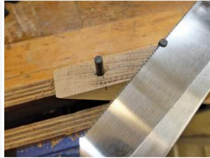
Carbon fibre is easy to cut with a fine-tooth saw
