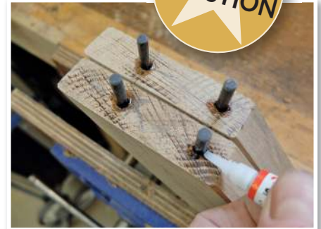
It cannot absorb wood glue so CA adhesive is the practical solution
