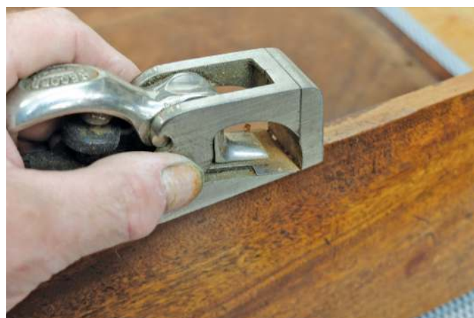
Using a bullnose rebate plane to remove most of the edge damage
