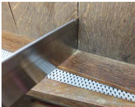
Where the drawer bottom boards were still joined, a pullsaw separated them
