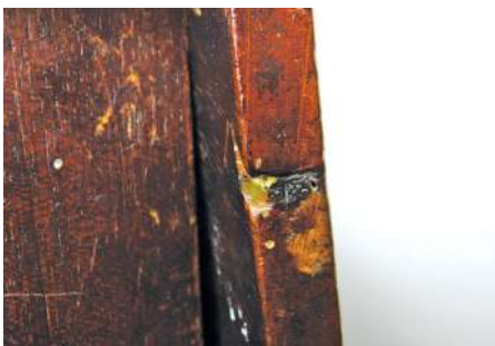
An old lump of rosin-type filler used to fill a gap in the mahogany
