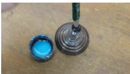
Patinating the fixing screw, the pencil point breaks the fluid surface tension
