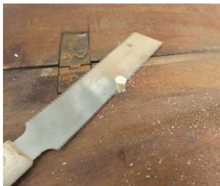
The plug trimmed off with a flexible flush-cut saw
