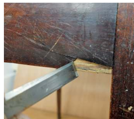
The broken area of veneer was trimmed ready for patching
