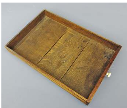
The oak drawer bottom separated into three sections by shrinkage
