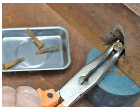
Pressing a screw tip down on a piece of cast iron while pulling with pliers
