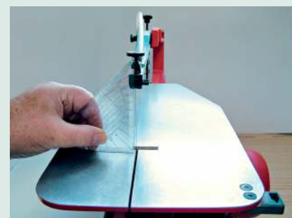
Using a set square to check blade alignment
