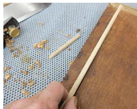
A new piece was fitted in the gap left by shrinkage and edge planing
