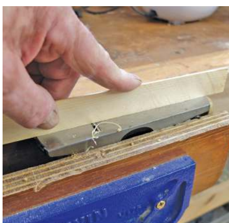
The slips were planed to width by running them over a block plane in a vice
