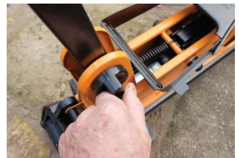
Loosening the rear leg on the SJA100XL ready to become the carry grip
