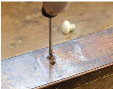
A broken-off thread removed by hacksawing a slot and using a screwdriver
