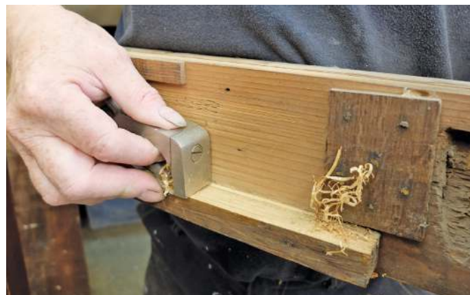
Heavily worn drawer runners were planed level again
