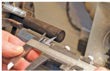
Using the internal jaws for fine measurement on the lathe
