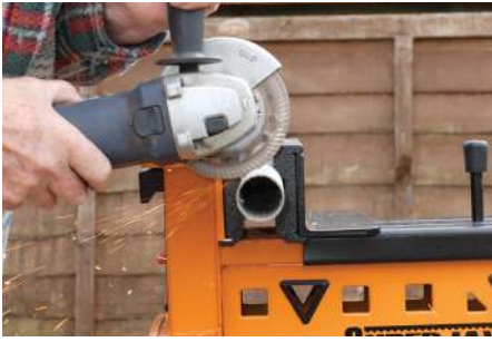
Engineers jaws on the SJA100XL being used to cut a steel pipe
