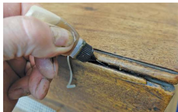
Injecting hide glue under a waggly hinge to set it firmly in place ➤
