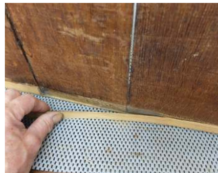
The drawer bottom slips were simply pulled away thanks to failed glue
