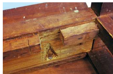
A crudely marked and cut screw pocket for a table-top screw
