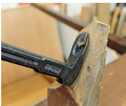
A cat's paw was used to withdraw the iron nails
