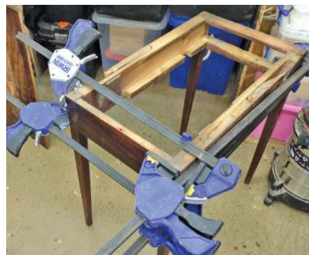
As soon as the glue-up was done the frame was clamped tight overnight
