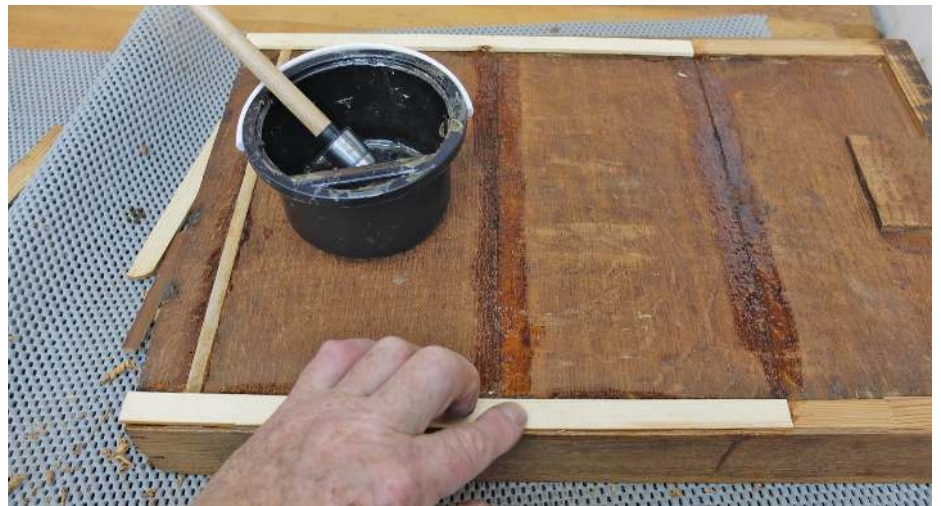
Holding a drawer slip while the glue sets. Hot water will remove any excess
