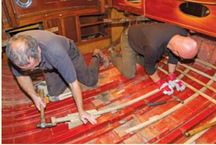
The process of steam bending the ribs to be installed in the hull
