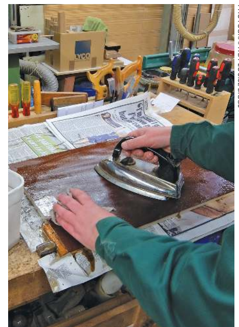
Ironing a veneer after laying to remove any bumps and cockling
