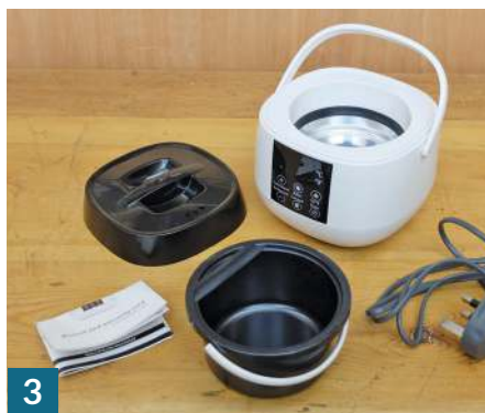
3 A cheap wax heater with lift-out pot suitable for working with hide glue
