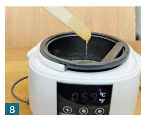
8 The freshly made glue should be fairly thin and runny to be useable
