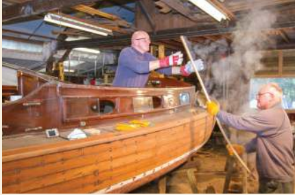
The process of steam bending the ribs to be installed in the hull
