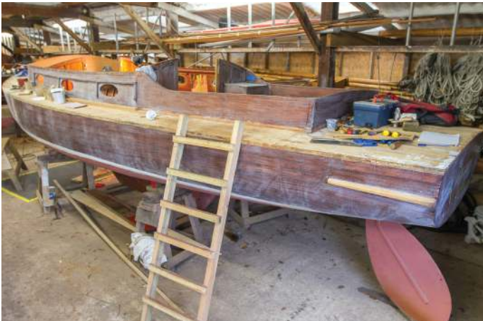
Hustler 4's decks stripped back ready for new lino to be fitted
