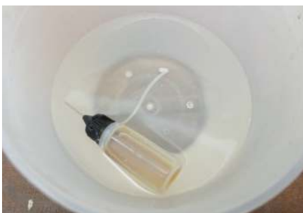
A glue-filled injector can work again if it is placed in hot water first
