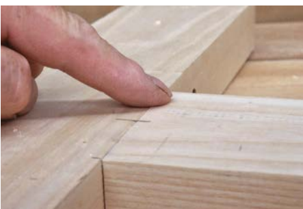
Checking by touch to make sure the joint is flush
