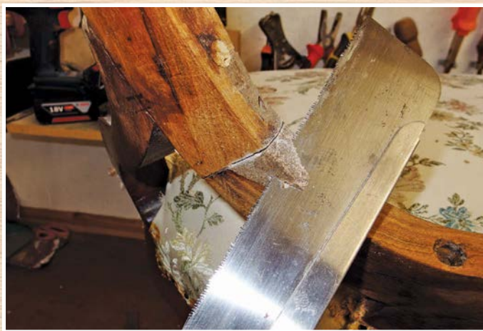
A dozuki blade being used to cut away previous filling work prior to rebuilding with a wedge of walnut
