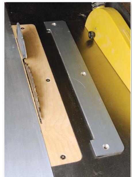
A standard insert plate replaced with a homemade zero clearance version
