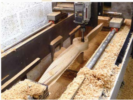
CNC machining of a wooden propeller using x,y,z axis programming
