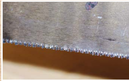
The fine, heat-treated teeth do become damaged with use but can be replaced easily
