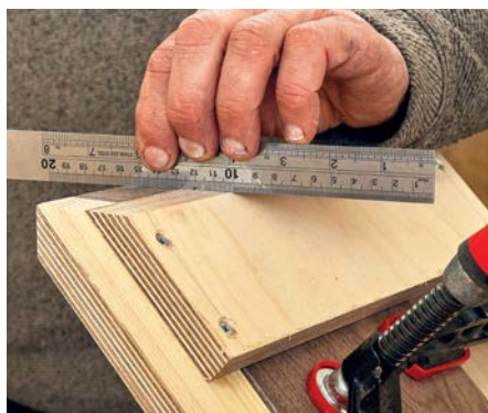
Check mitre is flush with top of jig
