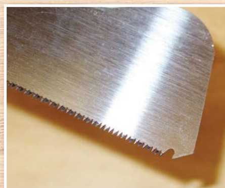
A small, 150mm dozuki-me blade with a hook tip for starting mid-panel cuts
