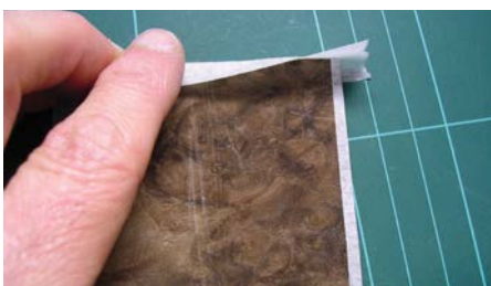
Taping the edges of your background veneer will help to protect against damage during handling
