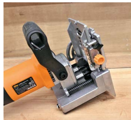
The fence height setting scale, adjustment and locking knobs
