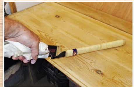
Removing an old, damaged blade. Hand protection is essential
