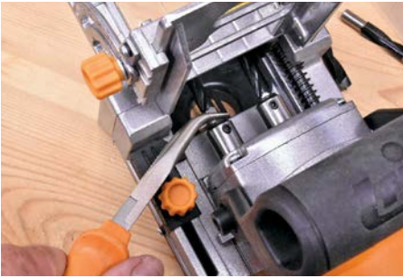
Using cranked pliers to remove a dowelling bit safely
