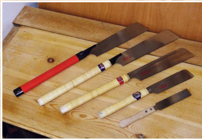
The Editor's own set of Japanese saws. From L-R: rip, kataba, dozuki, dozuki-me, flush trim
