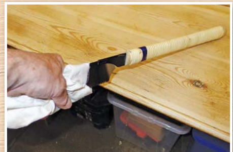
Fitting a blade by tapping home, with the vicious teeth covered for safety
