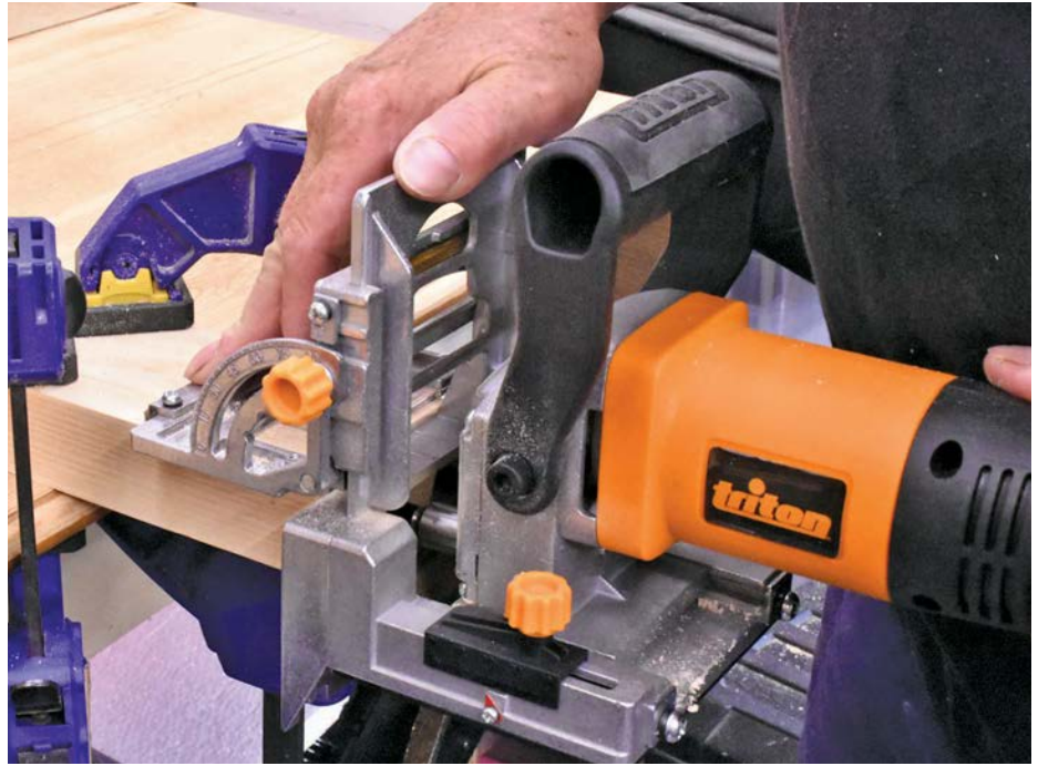
Pressing down on the fence to ensure accurate hole placement
