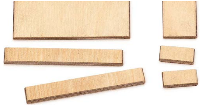
Cut splines to width minus 1mm ( \frac{1}{32} in) for wriggle room.
