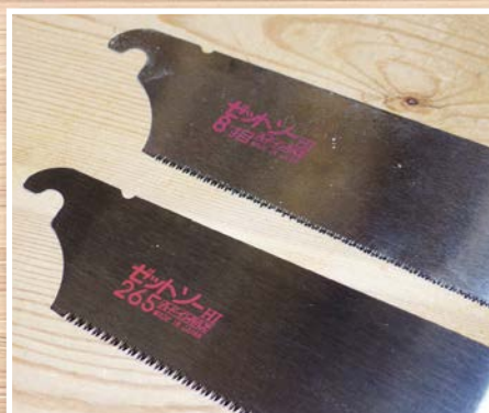
This larger toothed, slightly longer kataba blade was bought to replace the damaged blade at the top
