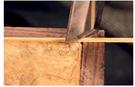
Make a test cut in some scrap wood before you attempt to fit the inlay
