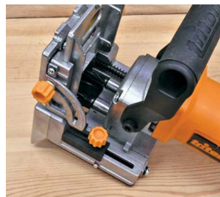
Fence tilt adjustment and drilling depth setting
