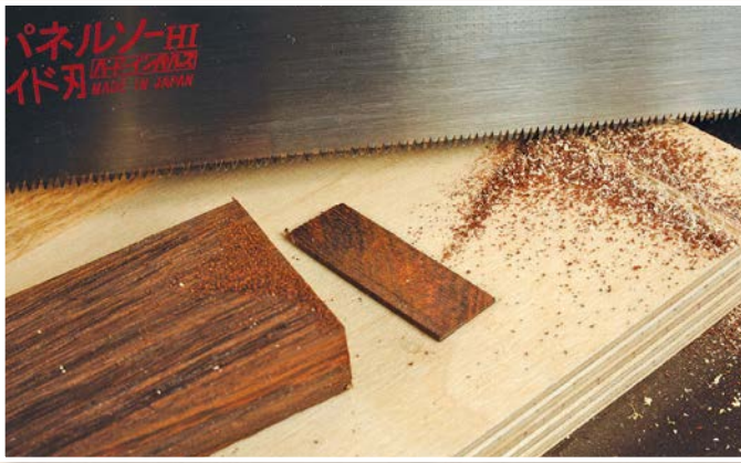
Very fine trimming cuts are possible thanks to the fine teeth and the pull action
