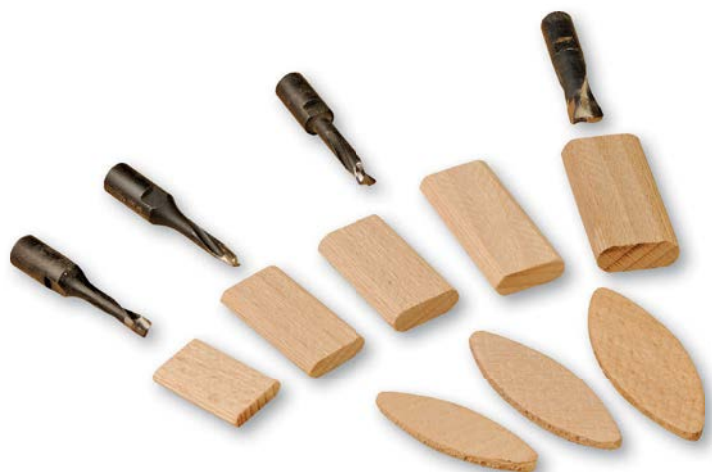
A size and shape comparison between biscuits and Dominos
