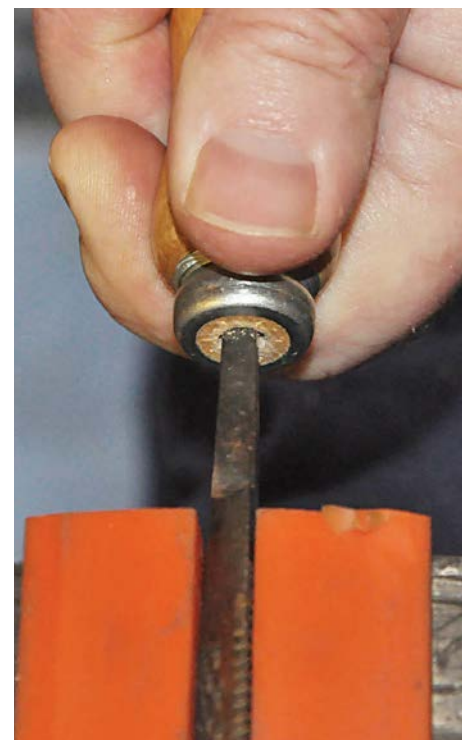
With the rasp held in soft jaws, twist and push the handle on to the tang
