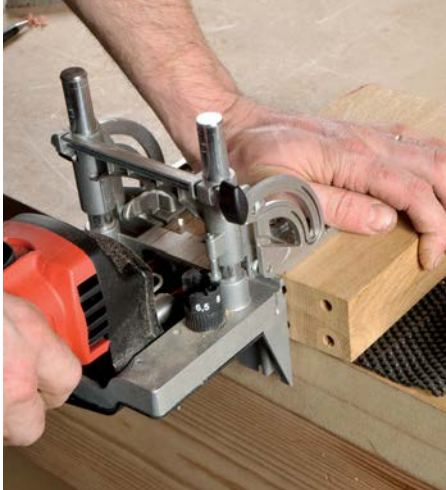
End-grain dowell machining is very accurate with the duo doweller
