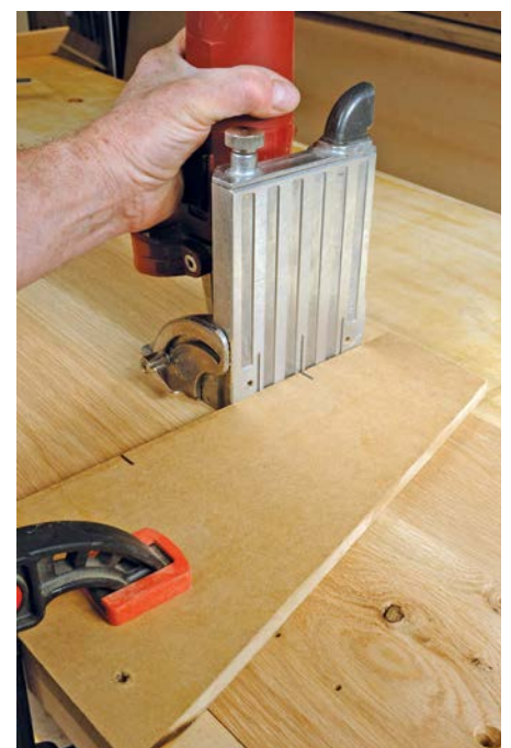
Using a T-square for cross-panel slotting for holding bookcase shelves
