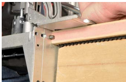
Releasing a drilling bit to change for a different size bit
