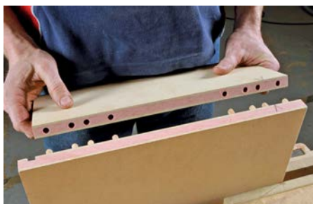
Matching up carcass corner components, note hole spacings
