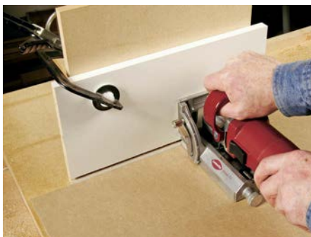
Creating a drawer-bottom panel groove with anti-slip devices retracted
