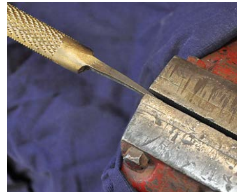
The same technique can be used to correct the tang in the other plane
