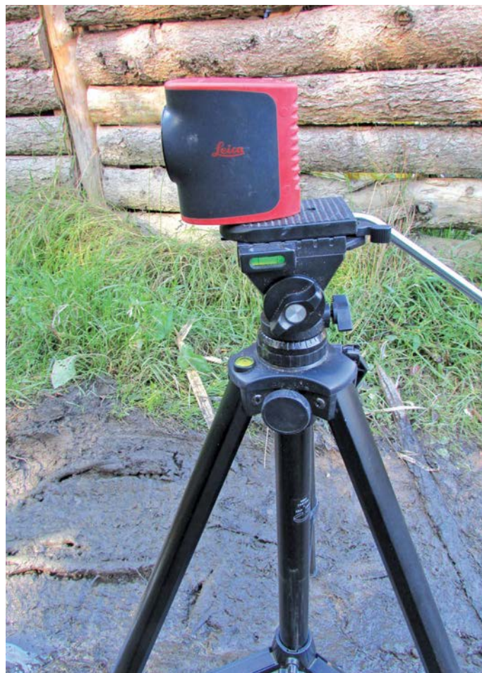
A laser and tripod for marking the levels on the posts
