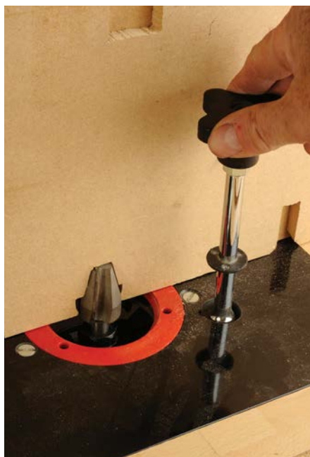
The through-fence on the router will prevent breakout
