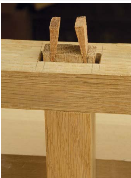
A wedged mortise and tenon. The wedges will spread the tenon
