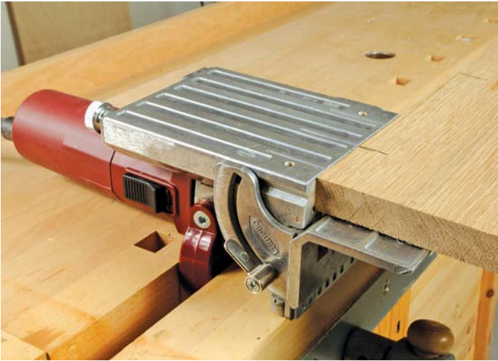
A biscuit joiner can usually be inverted in a vice as a static machine
