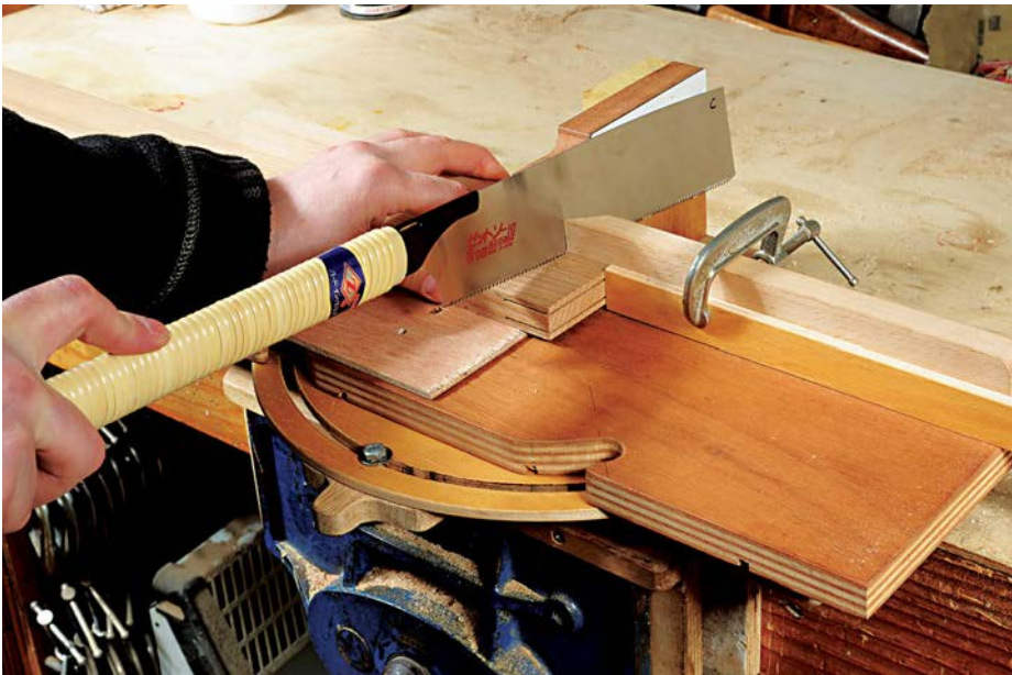
The shop-made mitre jig works well with Japanese and Western saws
