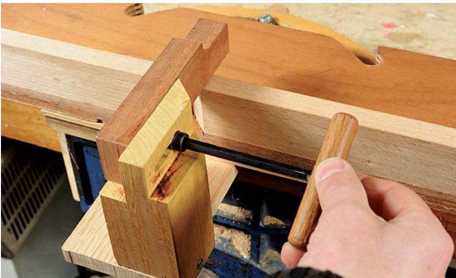
Advance or retract the magnetic guide to suit your saw
