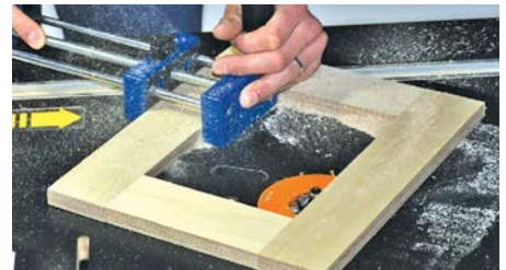
Using a Rockler routing workpiece clamp to rout the frame
