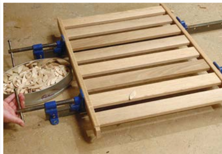
T-bar clamps holding a slatted frame
