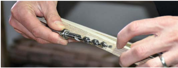
Demonstrating the angle the drill must take in the wood
