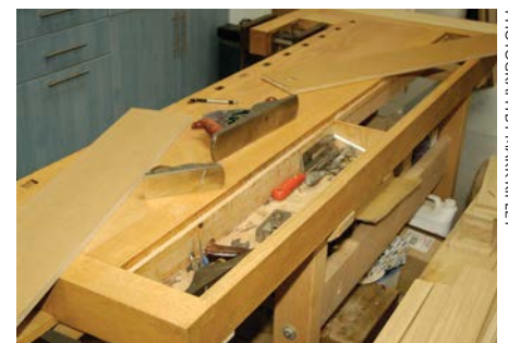
The usual untidy tool well, mitigated by having a drop-in cover board for a better working area
