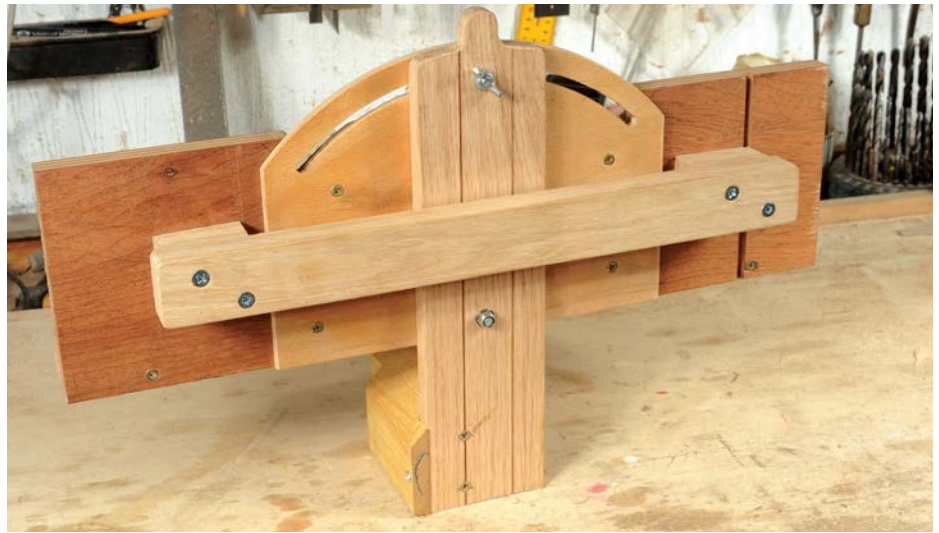
A bar beneath the saw jig allows you to secure it into a vice
