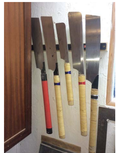
Keep your tools off the bench completely. With magnetic racks it is easy to both take and place tools out of the way
