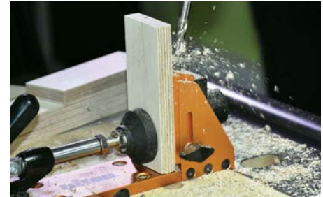
Fast drilling of a pocket hole with good chippings removal rate
