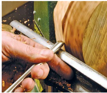
A toolrest mounted close to the blank
