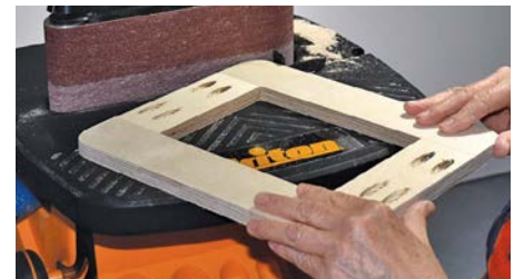
Sanding the frame corners on a Triton bench-top sander
