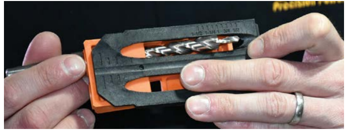
How the drill will protrude through the jig base
