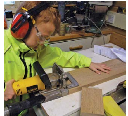
Mark and cut matching biscuit slots to join the end pieces to the assembled centrepiece.
