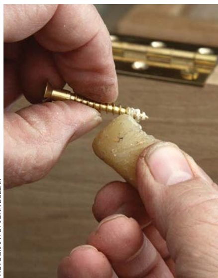
Beeswax is an easy way to help screws drive into their holes
