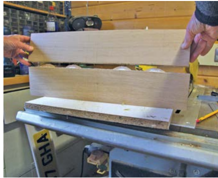
Join two pieces to form the side panels
