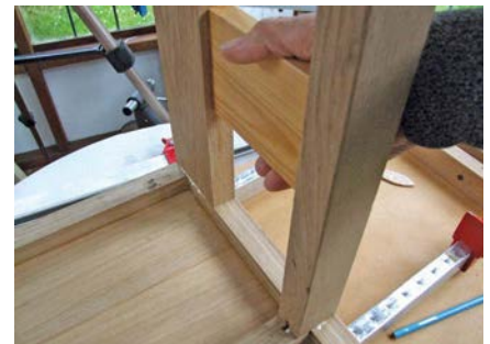
Trim biscuits to remove the outer points
