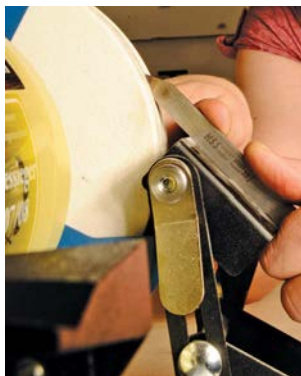
With the toolrest – or here the sharpening jig – angle set, grind off one side...
