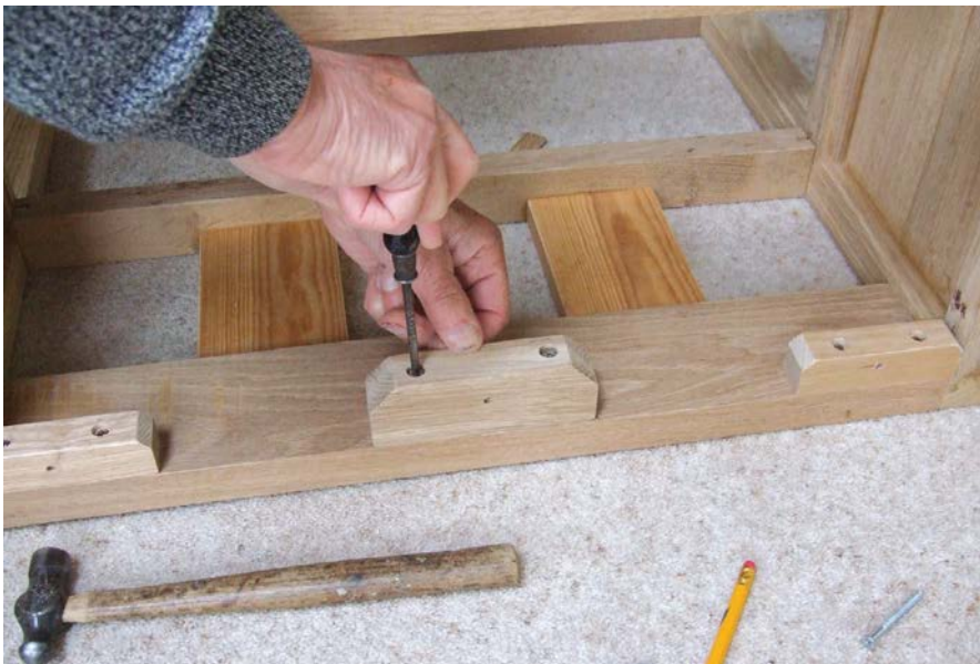
Attach blocks to the top of the rear rail for attaching the rear of the table top
