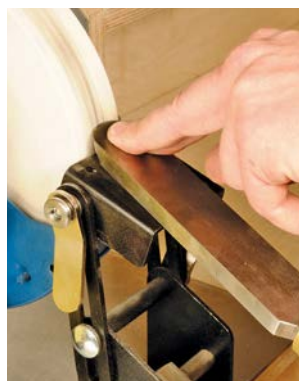
... until all of the scraper edge has been ground, creating your cutting edge
