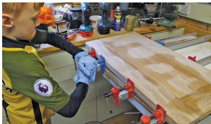
Cramp the assembly and allow to set
