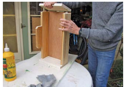
Complete the assembly and clamp. Check that the drawer is square
