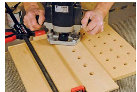
Then router drill each support hole, like this cutter storage board
