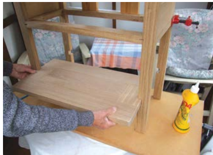
Slide the shelf into position, lining the back edge level with the rear of the leg
