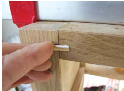
Cut ash infills to fit the slot cut by the biscuit cutter
