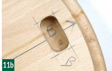
9 The underside of the mortising jig showing the bandsawn detent which allows the jig to sit properly on the curve
