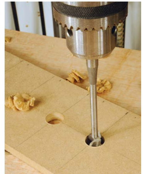
Make an accurate jig with holes to match your guidebush
