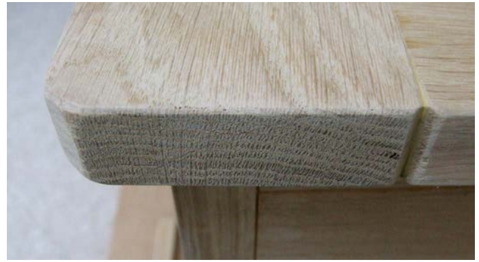
The front and rear pieces can be slightly eased at the corners
