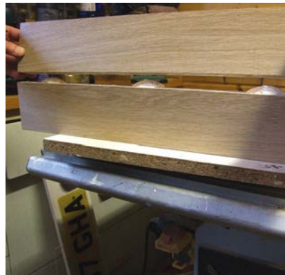
The centre part of the top panel is formed by joining two boards together using jointing biscuits
