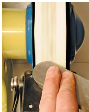
Push the scraper into the wheel at one edge first, to start the grind...
