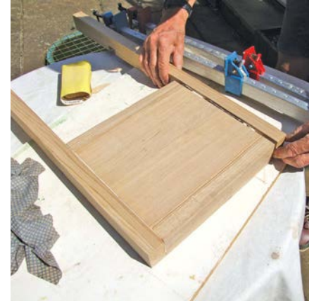
Mark and cut biscuit slots to attach the side panels to the legs
