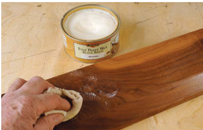
Hardening wax needs positive pressure to stick evenly to a highly finished surface
