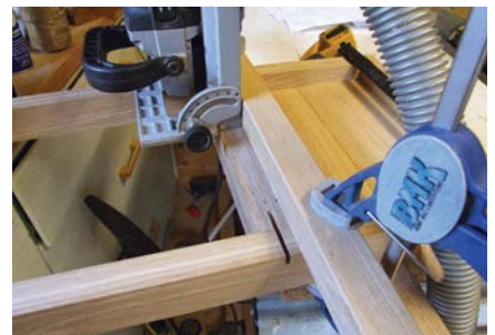
For the lower rail joints, use a guide for the biscuit cutter
