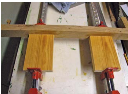
For the rear sub-assembly, attach the two lengths of pine to the lower rear rail using size 20 biscuits and adhesive
