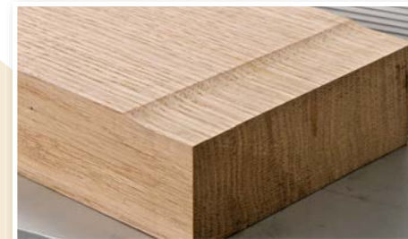
Snipe due to poor blade setting
