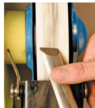
... then the other is ground. Be careful to keep both blade angles the same
