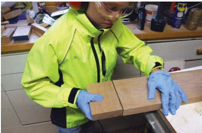
Join and cramp the end pieces to the assembled centrepiece
