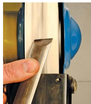
The skew is similar to the parting tool for grinding. First one side...
