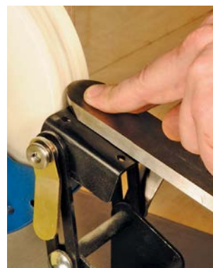
... then, with even pressure on the wheel and toolrest, sweep the handle around...
