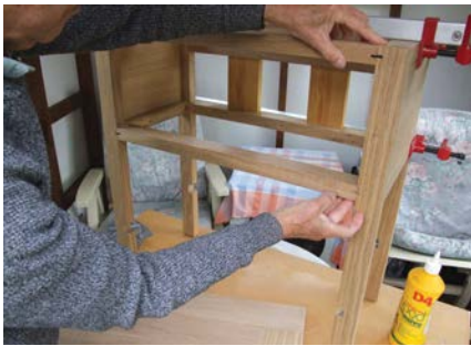
Carefully lift the part-assembly upright. Attach the front rails then clamp to set
