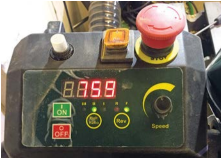
The digital speed control and speed readout unit
