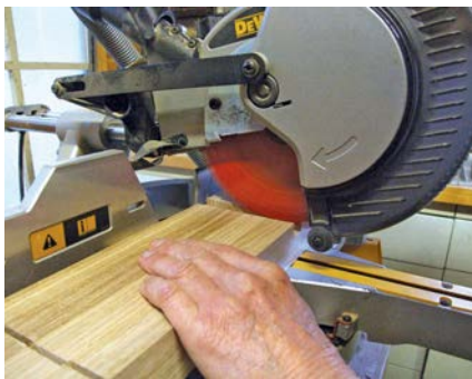
Clamp the legs together and trench out the slot required to hold the shelf in place
