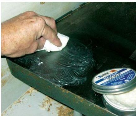
Cast-iron can be very 'dry', so waxing helps a great deal to reduce friction
