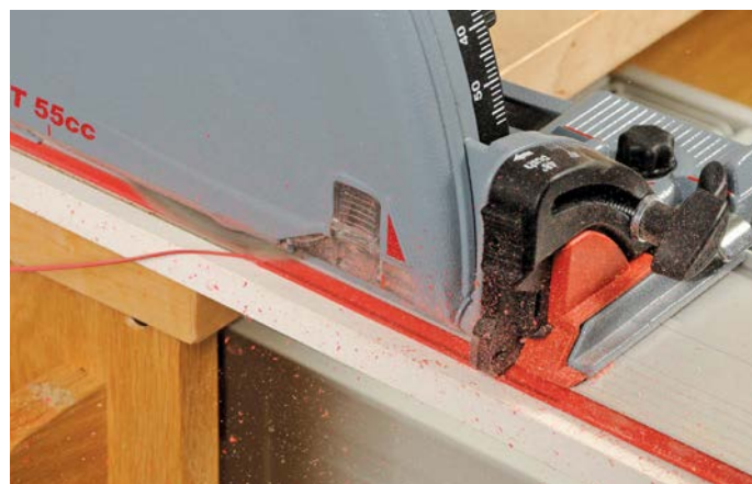
If you can afford it, a guide rail saw is ideal. The first blade trims the rubber edge which you can then mark from ■
