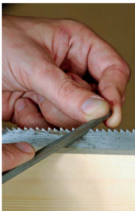
A saw file has a much sharper triangular profile than a standard metalworking file
