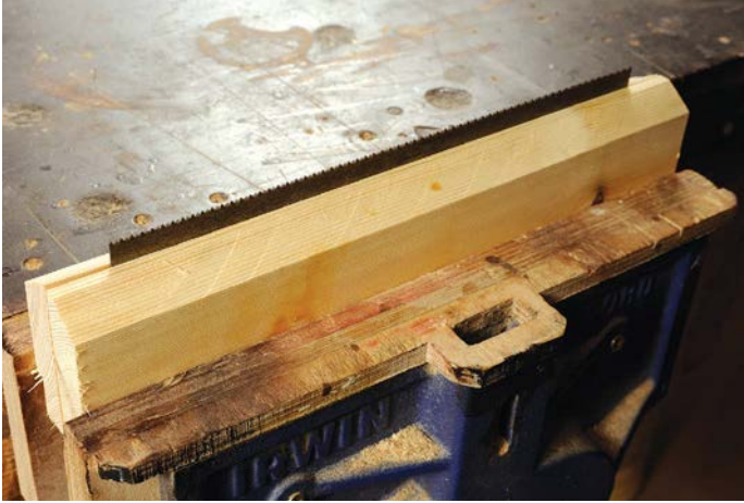
Softwood jaws made up for saw sharpening with a bevel to allow tooth filing
