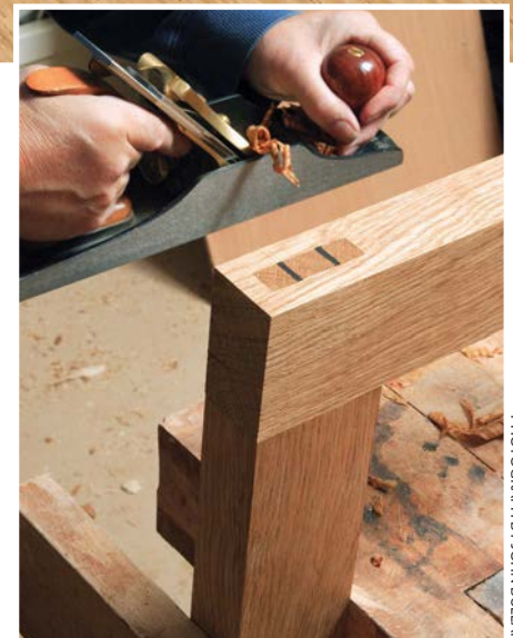
A finely set hand plane used to do the final cleaning up of an exposed joint
