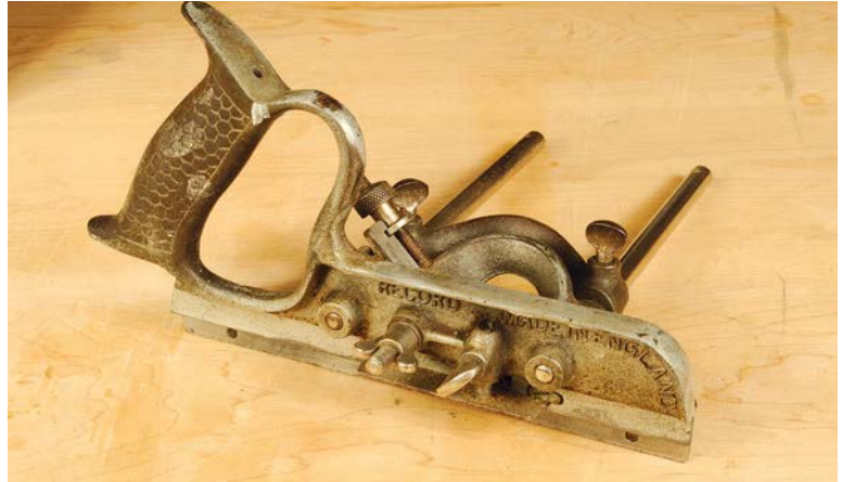
This Record 45S first appeared in the 1938 catalogue and is the same as the Stanley 45 with the addition of a simple screw adjustment to the cutter blade
