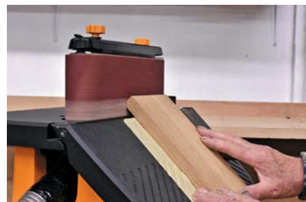
Using masking tape as a guide for chamfering
