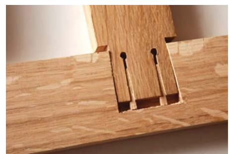
A fox-wedged joint cut through to show the joint construction
