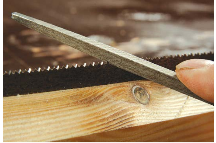
Consistency in sharpening angle and filing alternate teeth are key to success
