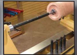
STRONGBORE™ Modular Boring Bar
