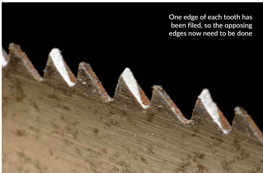
A crosscut tenon saw will saw tenon cheeks but a rip tenon saw will do it quicker
