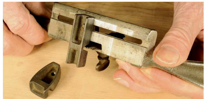
The blades are interchangeable and can be set against a choice of two fences
