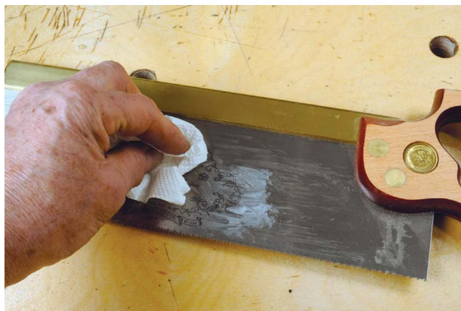
A bit of final TLC with a rub over of tallow for lubrication
