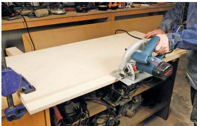
Here one cut board is acting as a fence for trimming the second board. Quick clamps make setting easy
