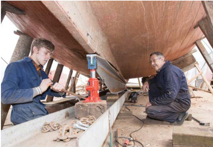
The trust's craftsmen fit a metal keel to White Moth in April 2013
