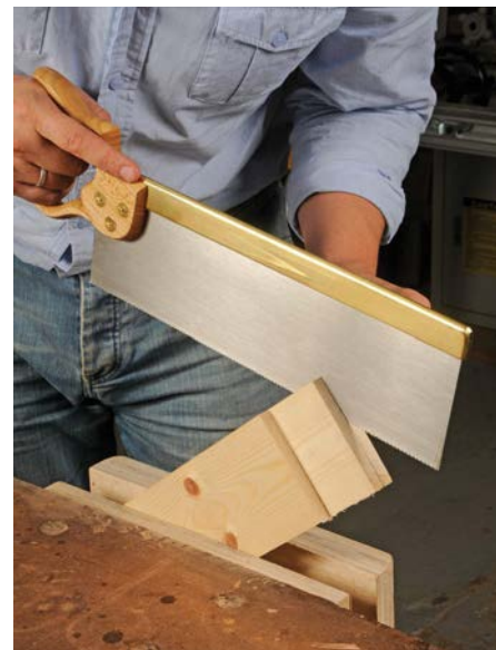
A crosscut tenon saw will saw tenon cheeks but a rip tenon saw will do it quicker
