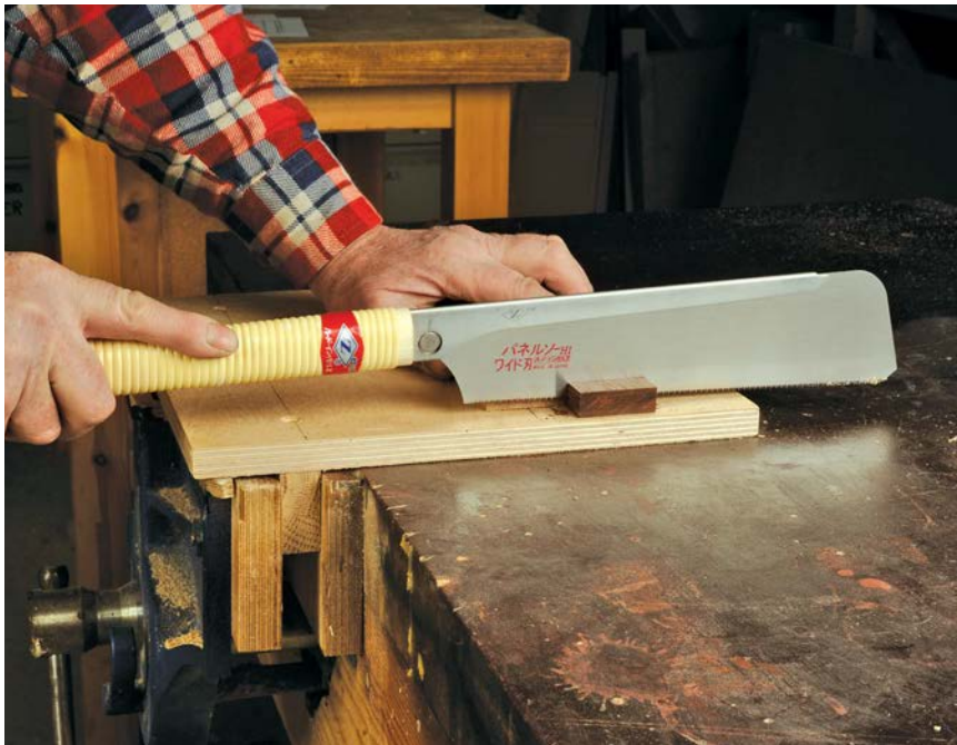
Japanese thin kerf pullsaws offer precision and control and the ability to make fine trimming cuts
