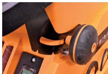
The click-stop detents allow quick repeatable angle setting
