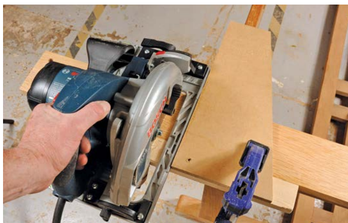
Accurate crosscutting is easy with a homemade guide but the first cut will probably trim off the end of the T-piece
