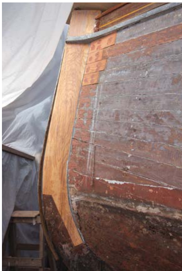
The new stem fitted during Olive's restoration can be clearly seen
