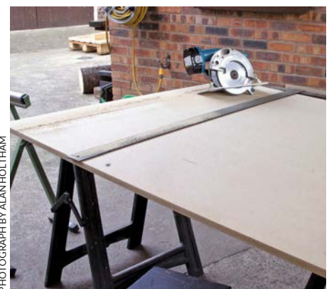
A large cut made using a giant T-square, however it needs to be very accurate before starting the cut
