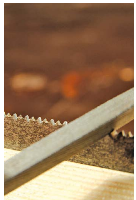
It can be tricky getting the file sitting at the correct angle in worn teeth
