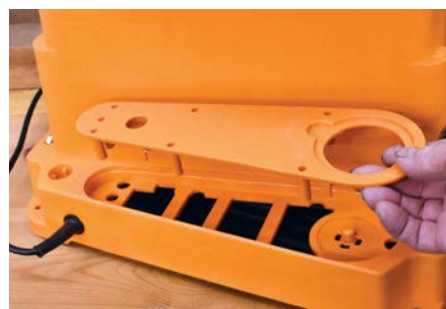
Both belt sander and bobbin insert are stowed in a special recess
