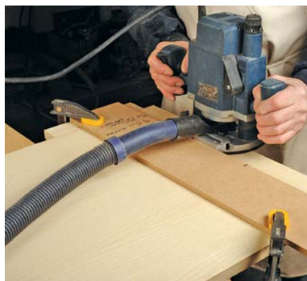
Extraction is a must, but the outlet and hose need to avoid catching on the work surface
