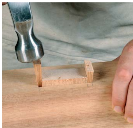
A joiner's wedge technique where they are fitted outside the tenon
