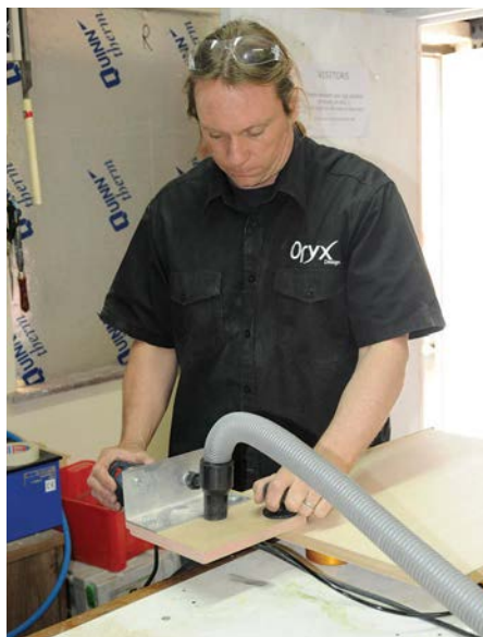
A specially made extraction device for an edge trimmer to deal with dust spraying outwards
