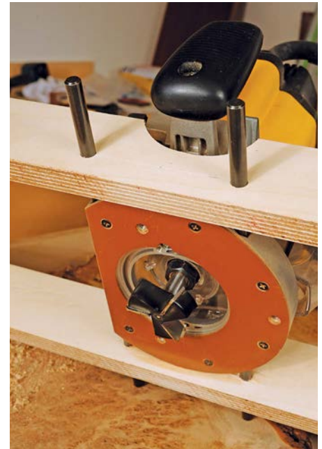
The three-winged cutter extends below the level of the skis
