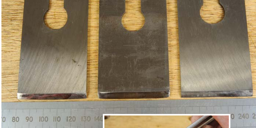
Above: Sharpened plane blades (from left) – cambered, ends rounded, straight
