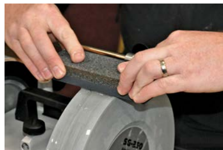
A special two-sided block prepares the same wheel for either grinding or honing, depending which side of the block is applied
