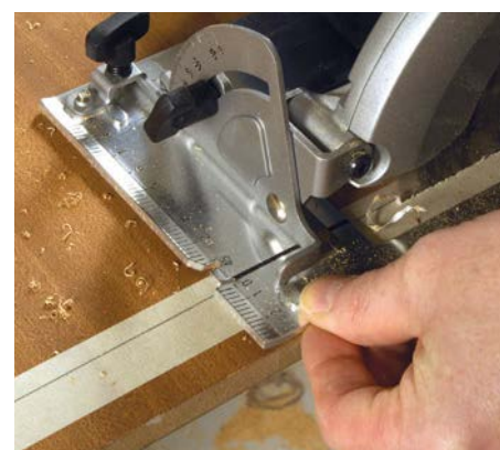
Masking tape is easy to mark cut lines on and it reduces spelching
