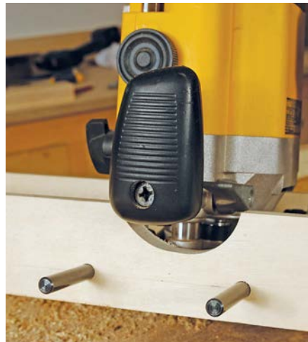
The bars need to be a tight fit so no other fixings are required
