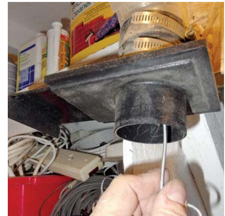
Sometimes the blast gate sheath gets blocked with dust and needs to be cleaned out
