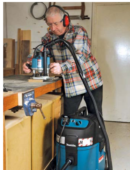
An HPLV extractor is designed for power tools rather than machines although it can give additional extraction
