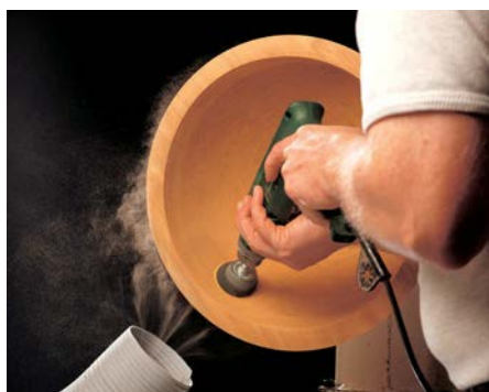
A standard extraction hose can draw off dust from turning very efficiently
