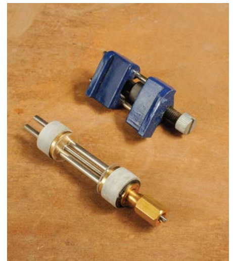
The standard type of honing guide at the rear and a more expensive and precise model in front
