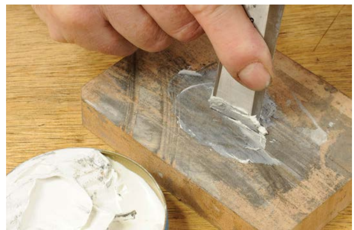
The MDF is quite indestructible, even running a blade vertically to keen the edge
