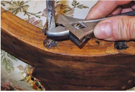
Using an adjustable spanner just above the screw head does work
