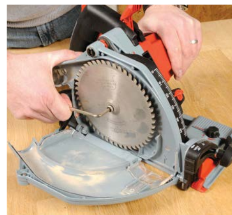
Fine teeth on this plunge saw are designed to leave a very clean-cut finish
