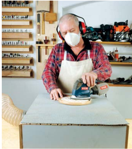
A downdraught table removes any dust not being collected by the sander itself
