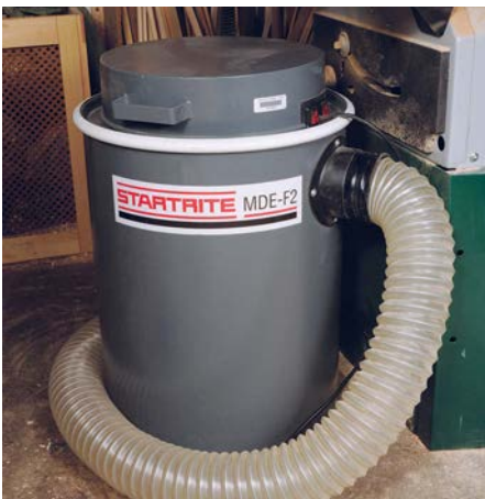
Drum-type extractors draw at a higher pressure than fan-type bag extractors
