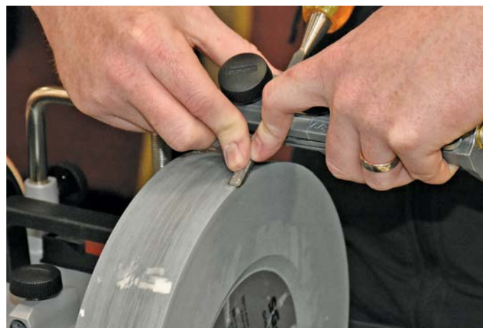
Initial grinding of a chisel on a Tormek machine, moving the blade from side to side for an even edge and to even out stone wear
