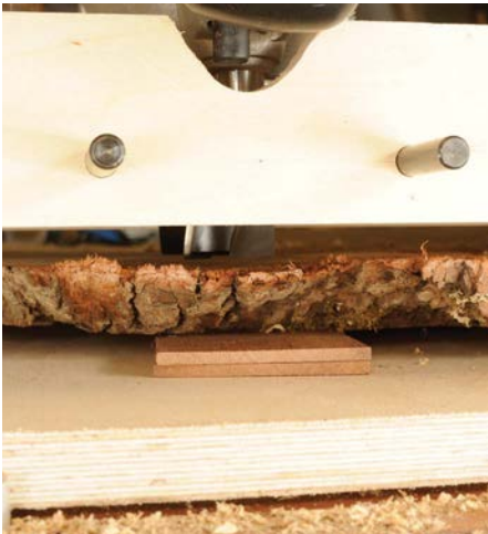
Blocks and packing are used to support the workpiece in the cradle
