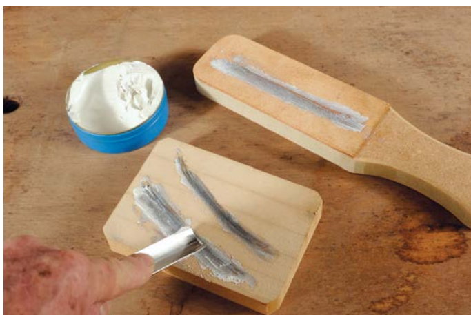
A leather strop rear, and an end-grain MDF block in use with metal polishing compound on a straight gouge
