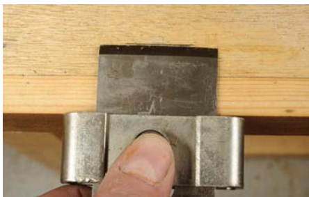
A mark on the bench top makes it easy to set blades in the guide each time. The projection is slightly different for plane blades and chisels
