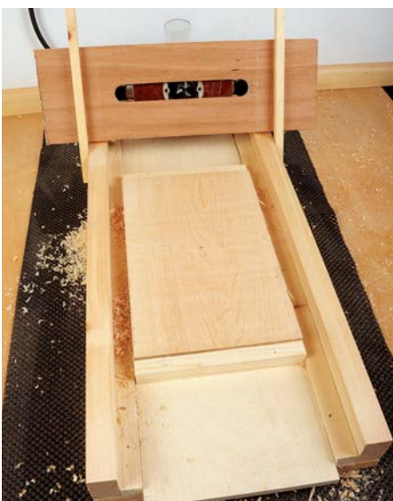
The cutter is set to skim the surface of the workpiece held in place in the jig below
