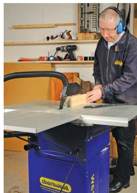
The crown guard ideally needs an HPLV power tool extractor to remove above-table dust efficiently
