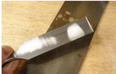
This shows just how 'unflat' even good-quality chisel blades can be, the edge still not having been touched yet
