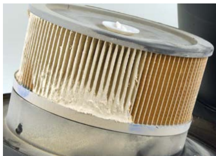
Cleaning of filters, dust bags and canisters must be done wearing a dust mask and enclosing the item in a black sack to shake it free of dust
