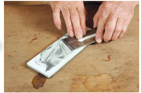
Ceramic plates give a very smooth finish to a cutting edge
