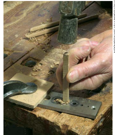
Using a ready-made plate to make dowel
