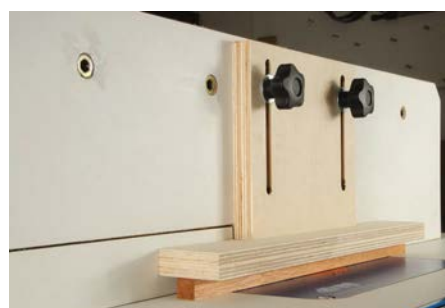
A partial tunnel for enclosing small components
