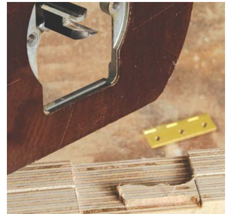
Machining the door hinge recesses
