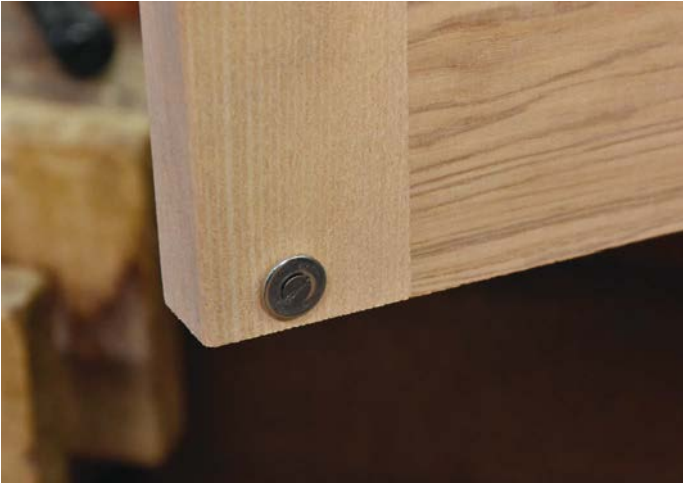
A steel washer for door closure against a magnet
