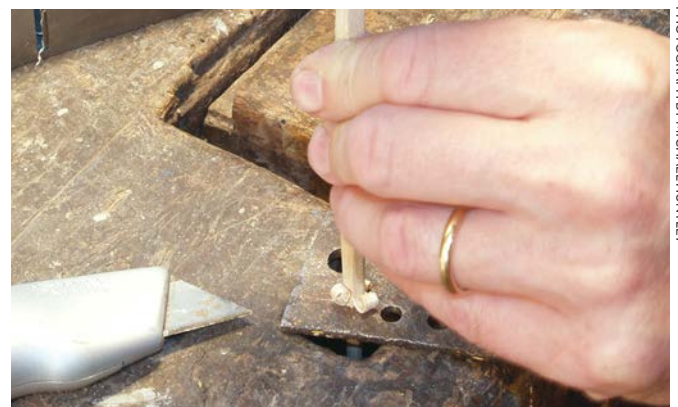
A homemade plate used for the same task – note how the waste curls away
