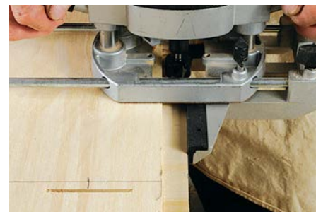
Routing the rebate to take the back panel
