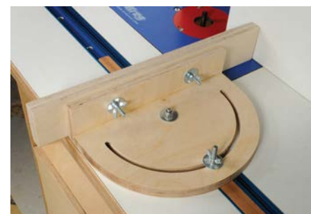
A fully adjustable mitre protractor with adjustable facing
