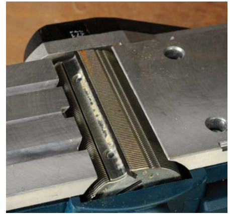
Portable planer blades are reversible and disposed of after use
