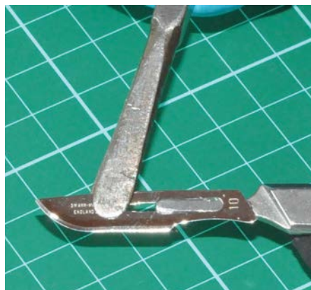
Remove the blade from the wrapping using the pliers and slide on to the handle bayonet fitting until it clicks
