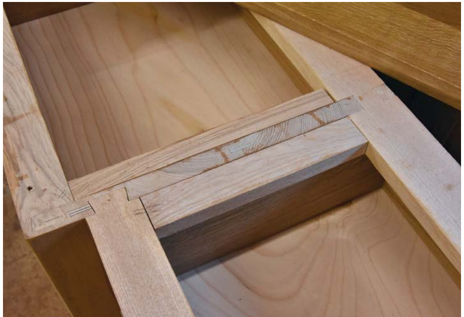
Dovetails are good for carcass strength
