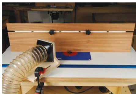
A through fence with extraction clamped in front
