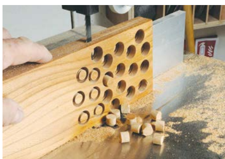
Separating the contrast plugs that cap the screw holes
