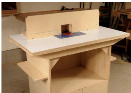
The shelves in place and also the un-faced fence
