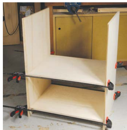
The glued up basic carcass assembly
