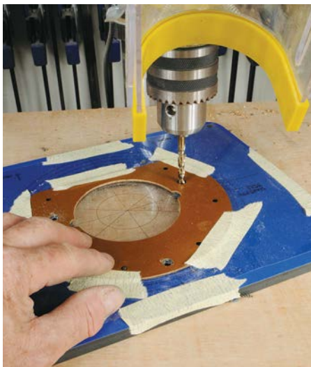
Drilling router mounting holes in the insert plate
