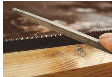
A special saw file, correctly used, can recondition a blunt handsaw
