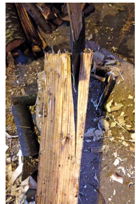
Uneven split 'running out'
