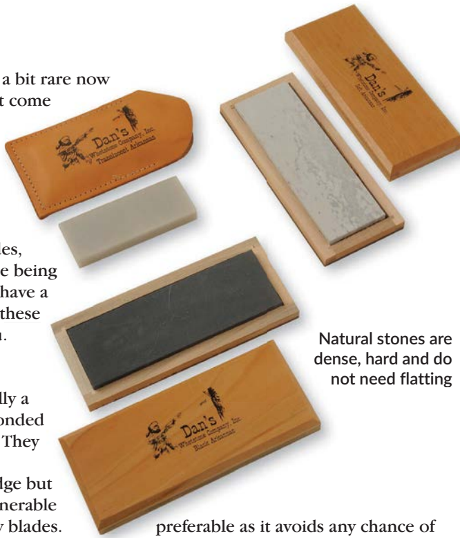
Ceramic plates give a very smooth finish to a cutting edge
