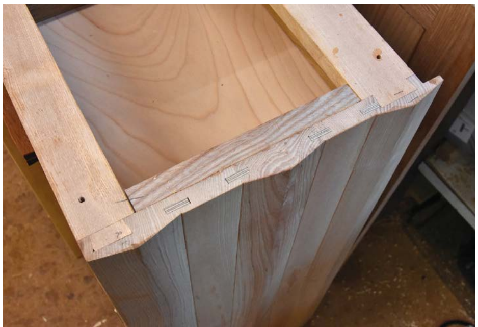
Loose tongue detail on an end panel
