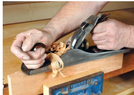
A really sharp cutting edge can produce fine, even shavings
