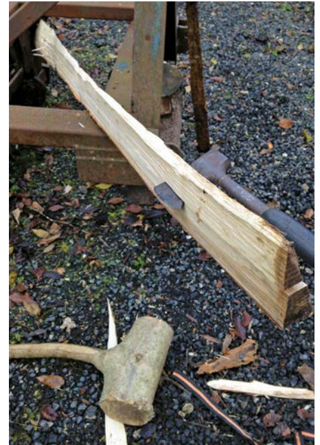
Tangential split through a longer billet
