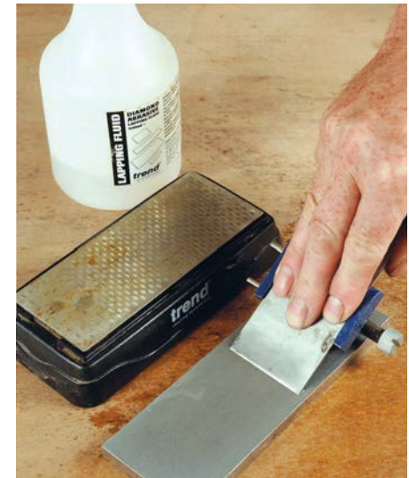
Diamond plates give a very quick result even with damaged cutting edges
