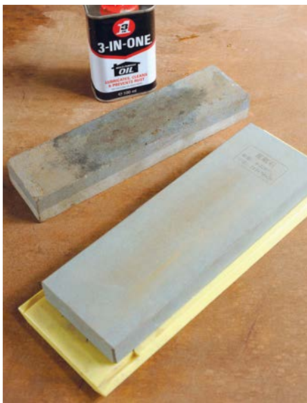
Although still available, oilstones have been largely replaced by better alternatives
