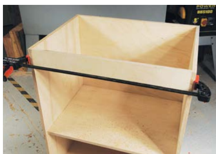
Back panel in place and top front rail biscuitied
