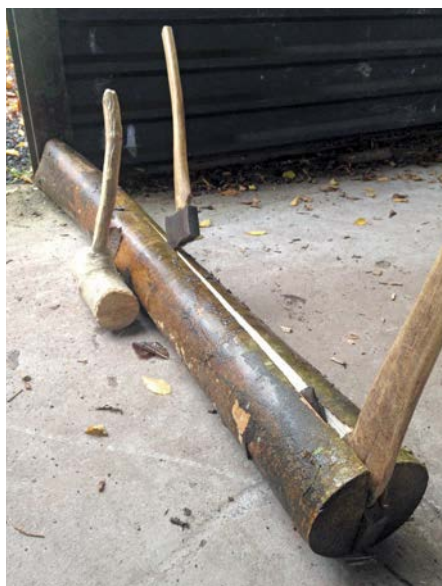
Making the first split in a clean ash log
