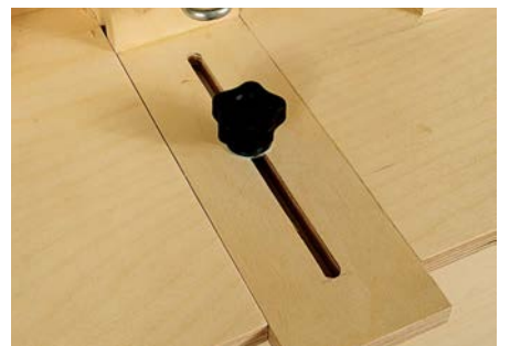
The main fence adjuster for fine movements
